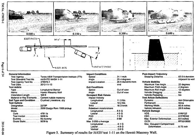
Figure 5. Summary of results for MASH test 1-11 on the Hawaii Masonry Wall.
