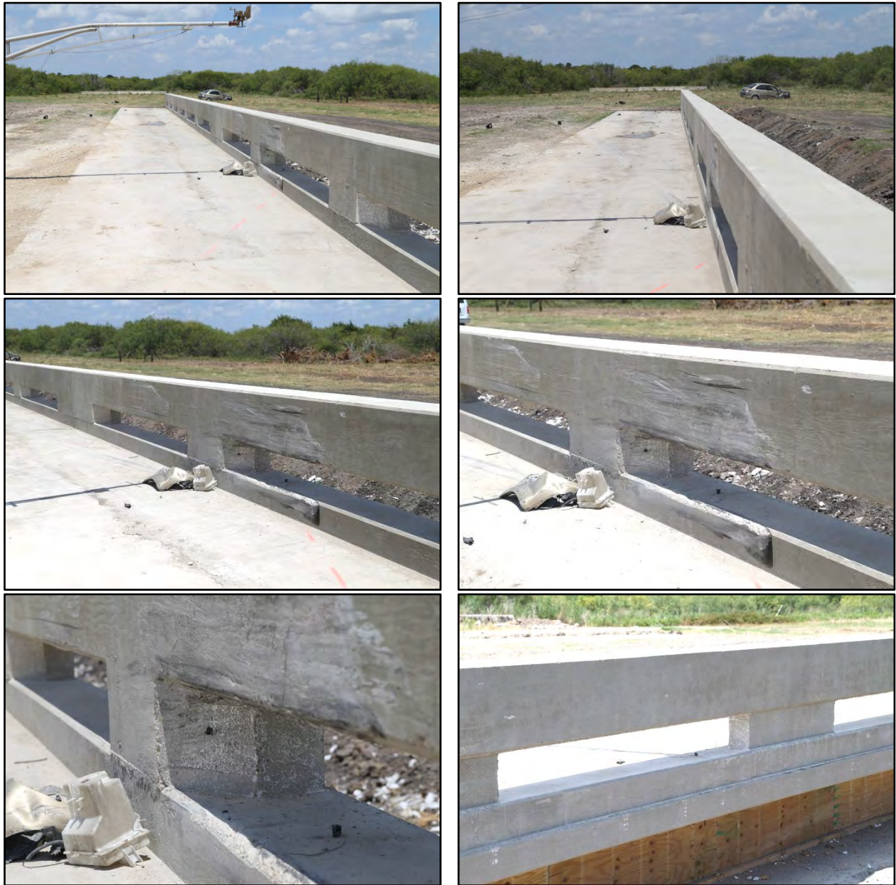
Figure 5.3. TxDOT T224 Bridge Rail after Test No. 490025-2-2.
