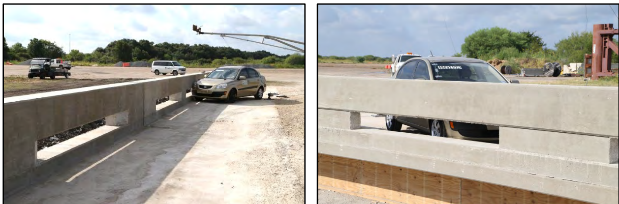
Figure 5.1. TxDOT T224 Bridge Rail/1100C Vehicle Geometrics for Test No. 490025-2-2.
