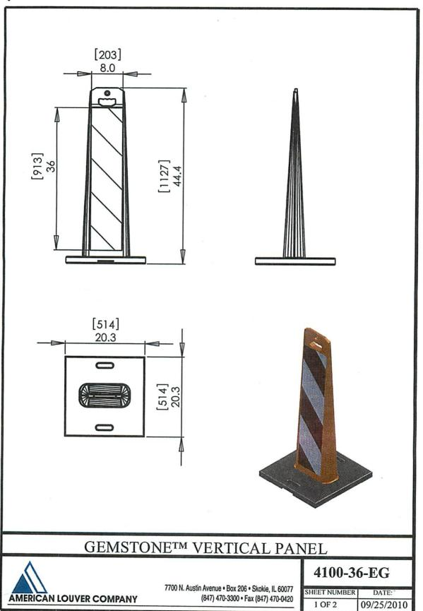
Illustration A2. Gemstone Vertical Panel Drawing (1 of 2)
