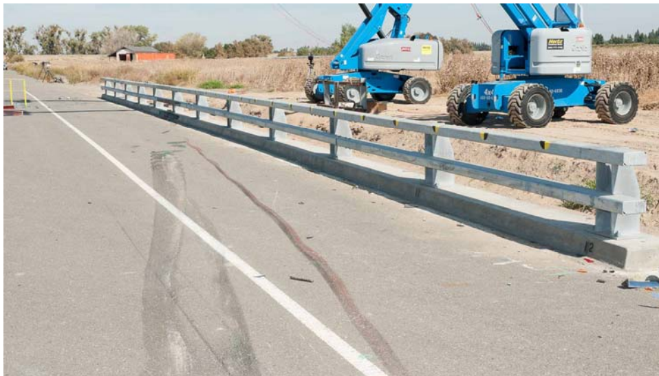
Figure 5-5 Test Article After Test 130MASH3P13-03 Looking Upstream
