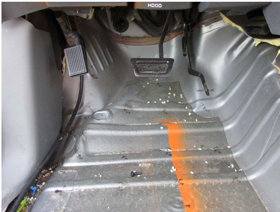
Figure 5-19 Vehicle Floorboard Post Test
