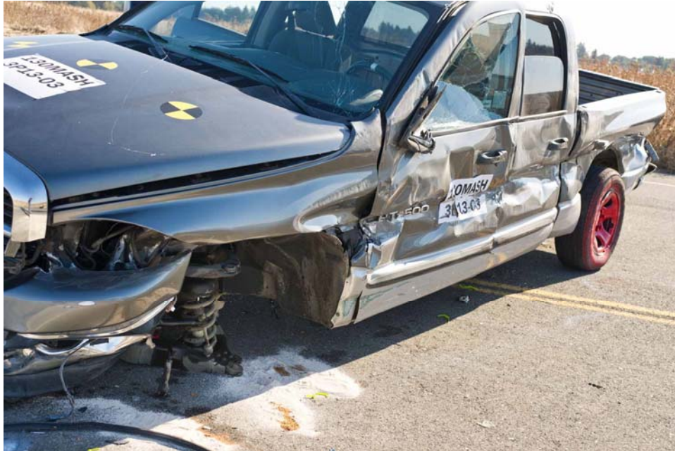
Figure 5-14 Front Corner of Upright Vehicle After Test 130MASH3P13-03
