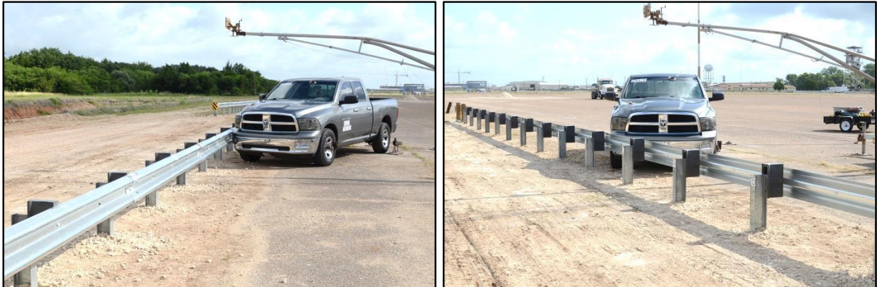
Figure 5.1. 28-inch W-Beam Guardrail System with Raised Composite Blockouts/Test Vehicle Geometrics for Test No. 608421-1.
