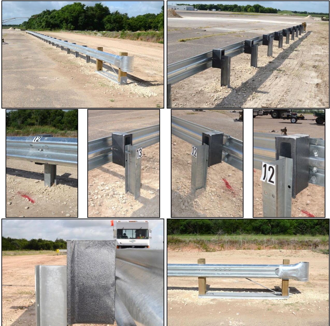
Figure 2.2. 28-inch W-Beam Guardrail System with Raised Composite Blockouts prior to Testing.
