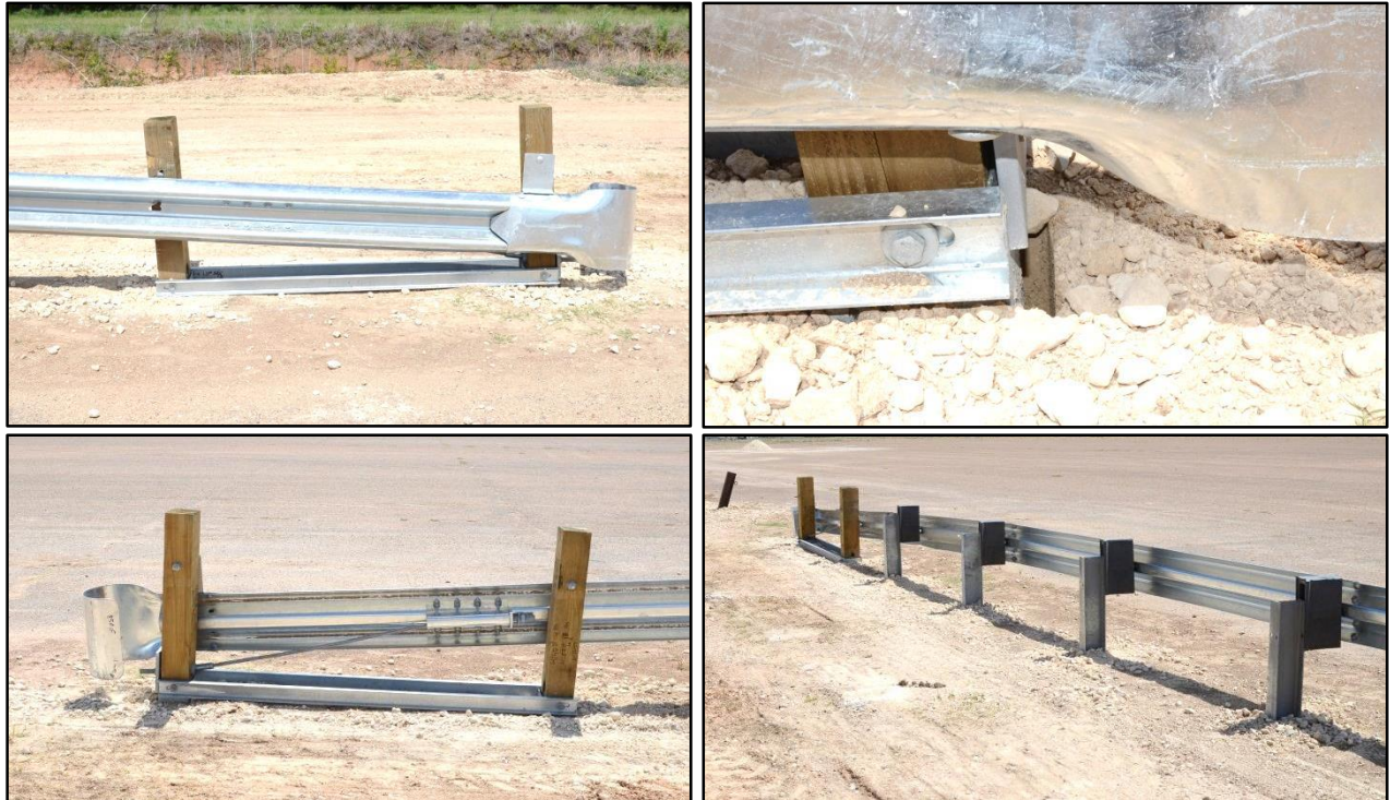
Figure 5.4. Upstream Terminal after Test No. 608421-1.
