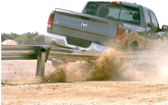
Figure D.2. Sequential Photographs for Test No. 608421-1 (Rear View).
