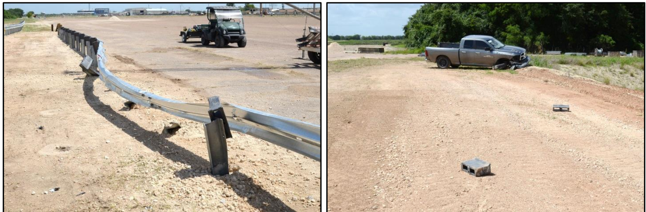
Figure 5.7. Field Side of Guardrail and Released Blockouts after Test No. 608421-1.
