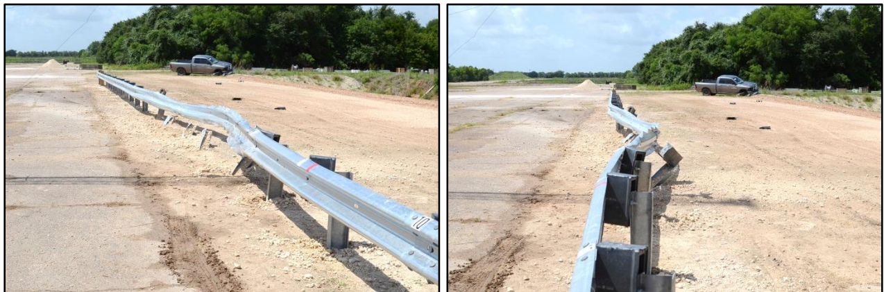
Figure 5.3. Test Vehicle and Guardrail System after Test No. 608421-1.
