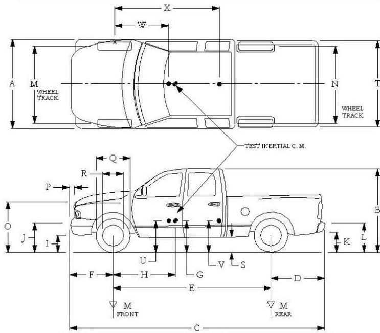
**Table C.2. Measurements of Vehicle Vertical CG for Test No. 602361-1.**
