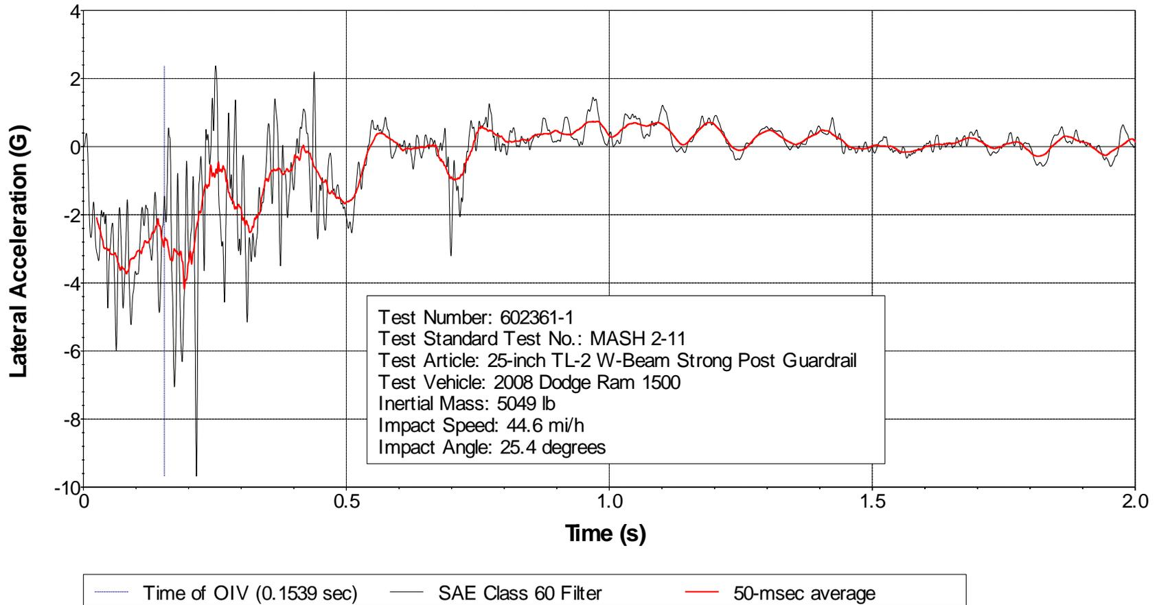
**Figure C.4. Vehicle Lateral Accelerometer Trace for Test No. 602361-1 (Accelerometer Located at Center of Gravity).**
