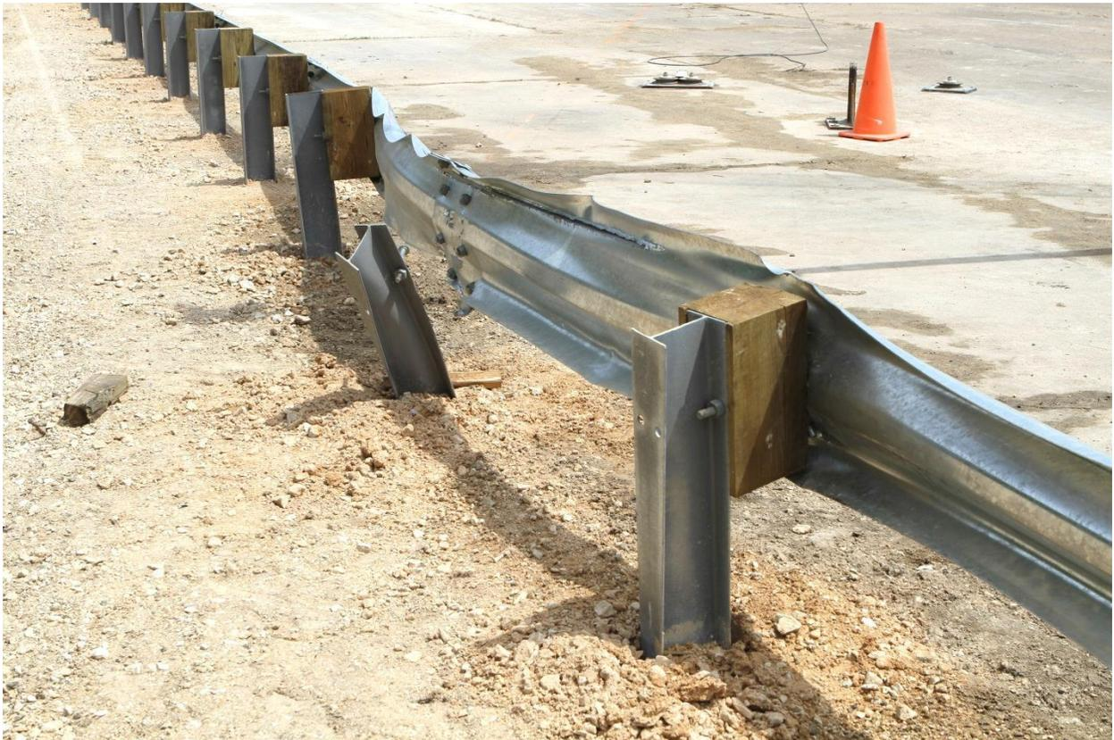
**Figure 4.6. Installation after Test No. 602361-1.**
