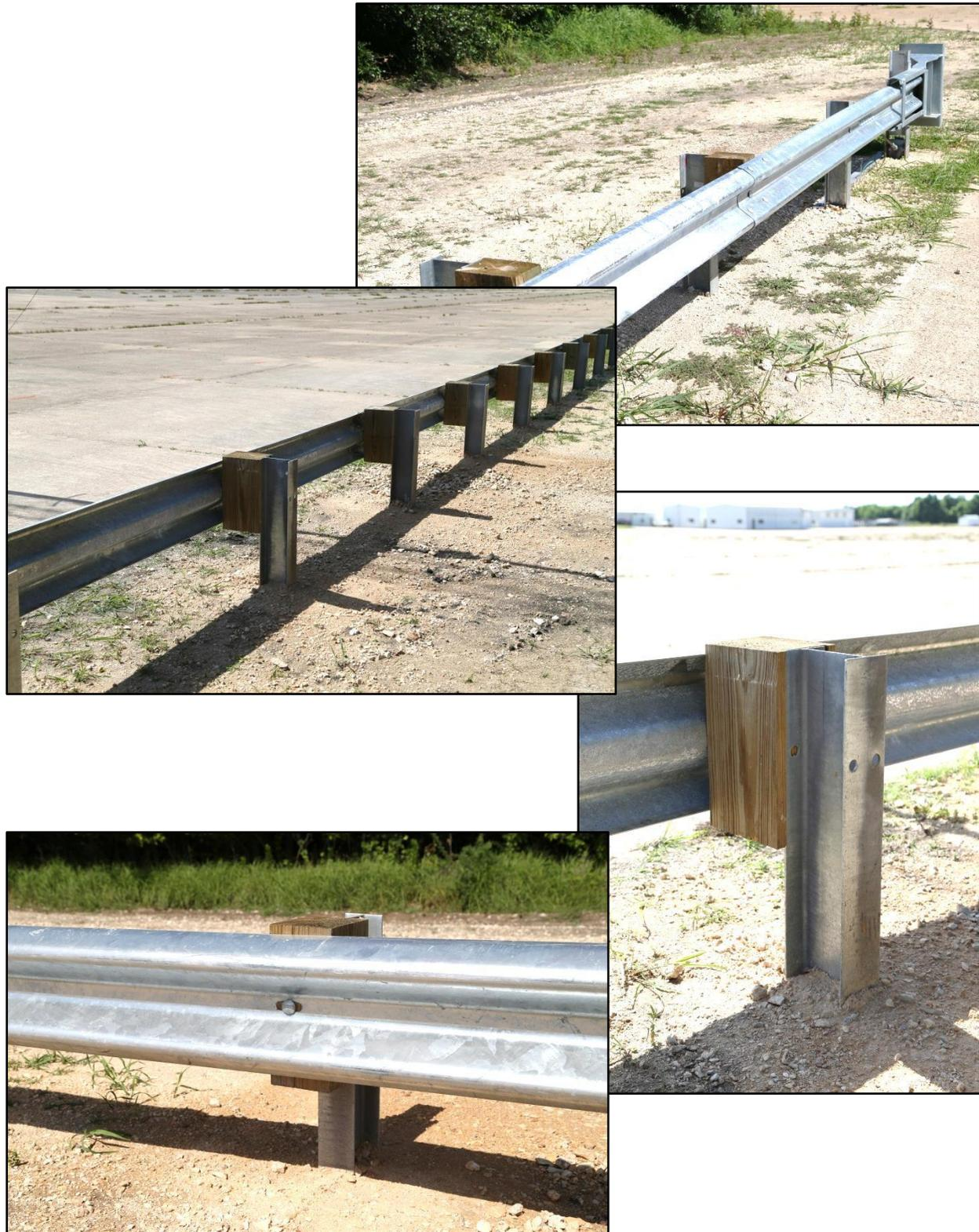
**Figure 5.2. 24-inch Tall Strong-post W-beam Guardrail prior to Testing.**
