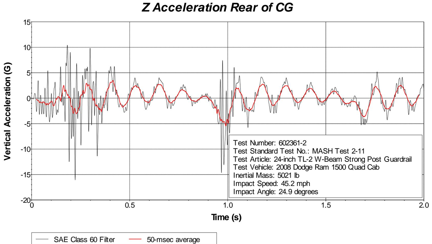
**Figure D.9. Vehicle Vertical Accelerometer Trace for Test No. 602361-2
