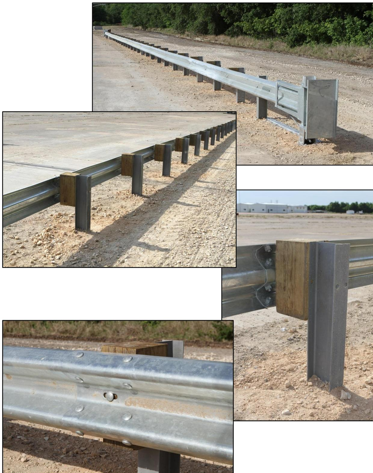
**Figure 4.2. 25-inch Tall Strong-post W-beam Guardrail Installation Prior to Testing.**
