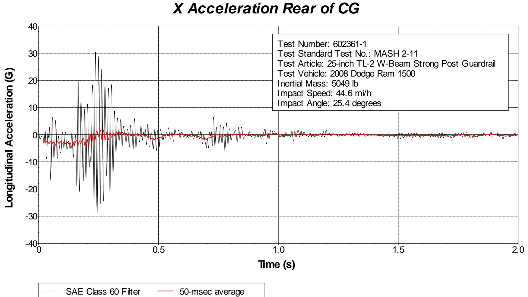
**Figure C.6. Vehicle Longitudinal Accelerometer Trace for Test No. 602361-1
