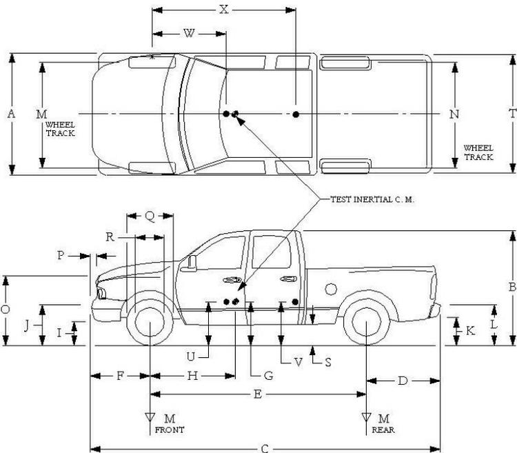
**Table D.2. Measurements of Vehicle Vertical CG for Test No. 602361-2.**
