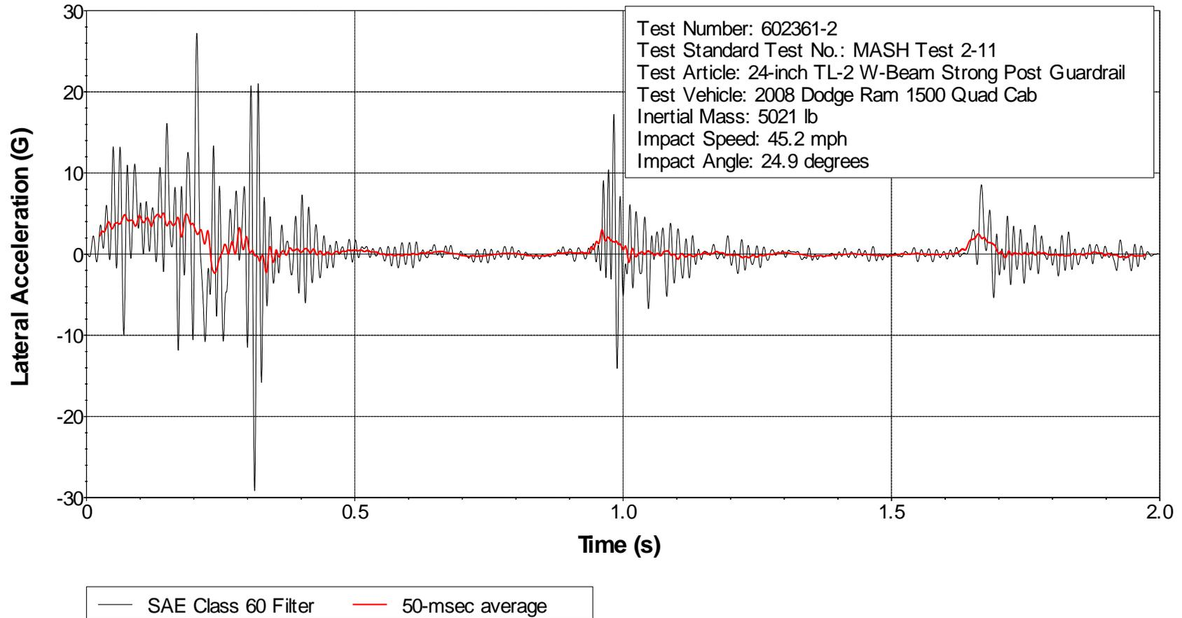
**Figure D.8. Vehicle Lateral Accelerometer Trace for Test No. 602361-2
