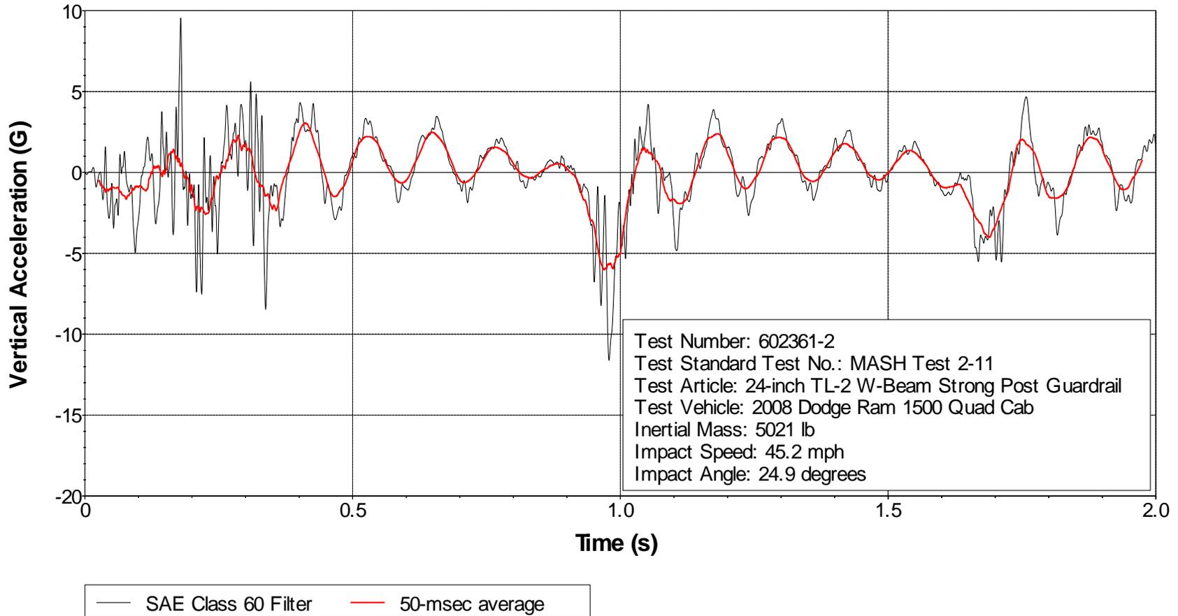
**Figure D.6. Vehicle Vertical Accelerometer Trace for Test No. 602361-2 (Accelerometer Located at Center of Gravity).**
