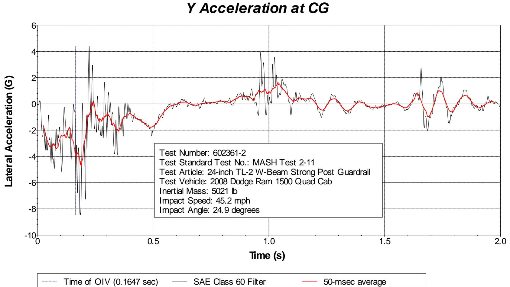
**Figure D.5. Vehicle Lateral Accelerometer Trace for Test No. 602361-2
