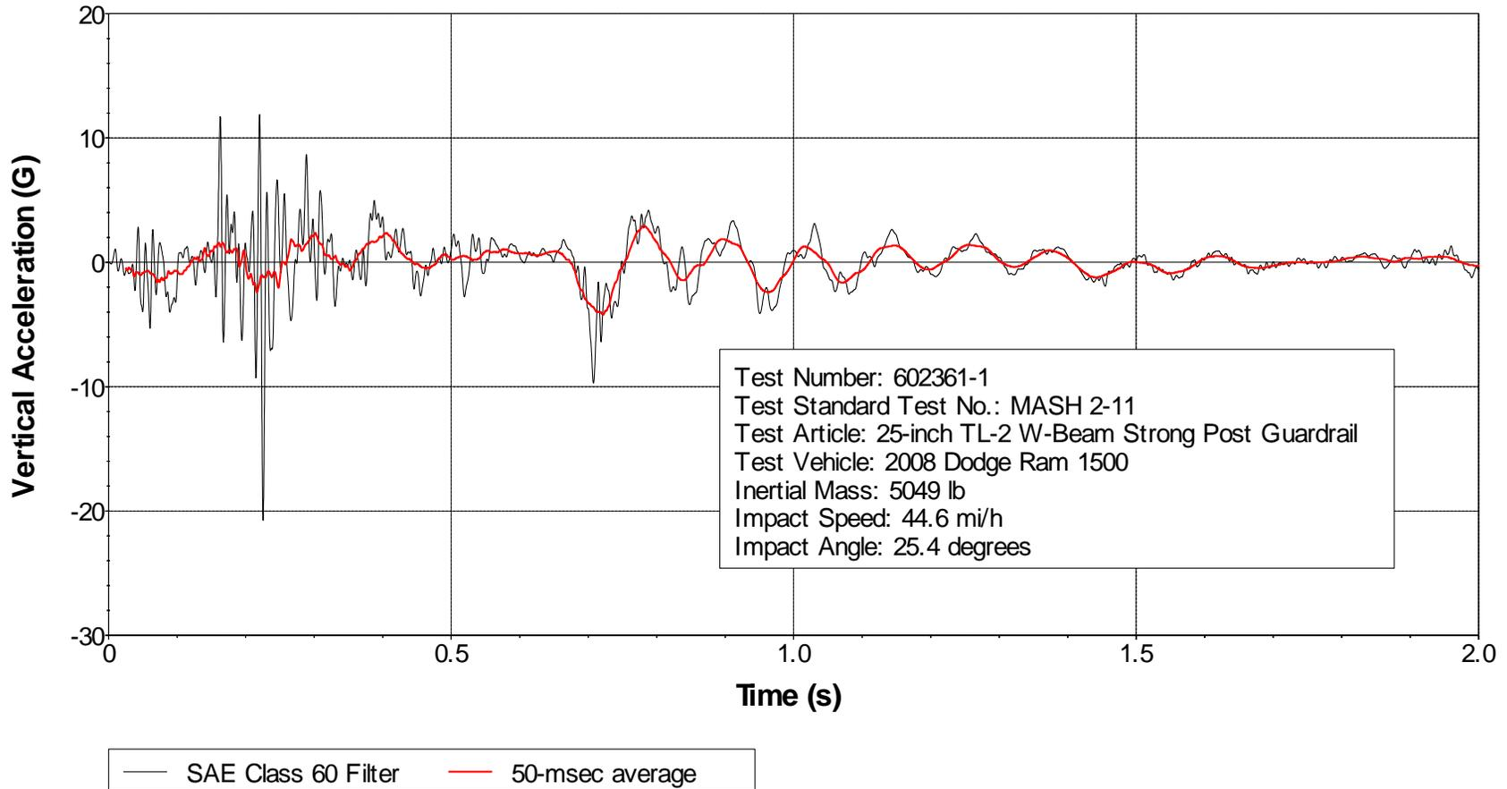
**Figure C.5. Vehicle Vertical Accelerometer Trace for Test No. 602361-1 (Accelerometer Located at Center of Gravity).**
