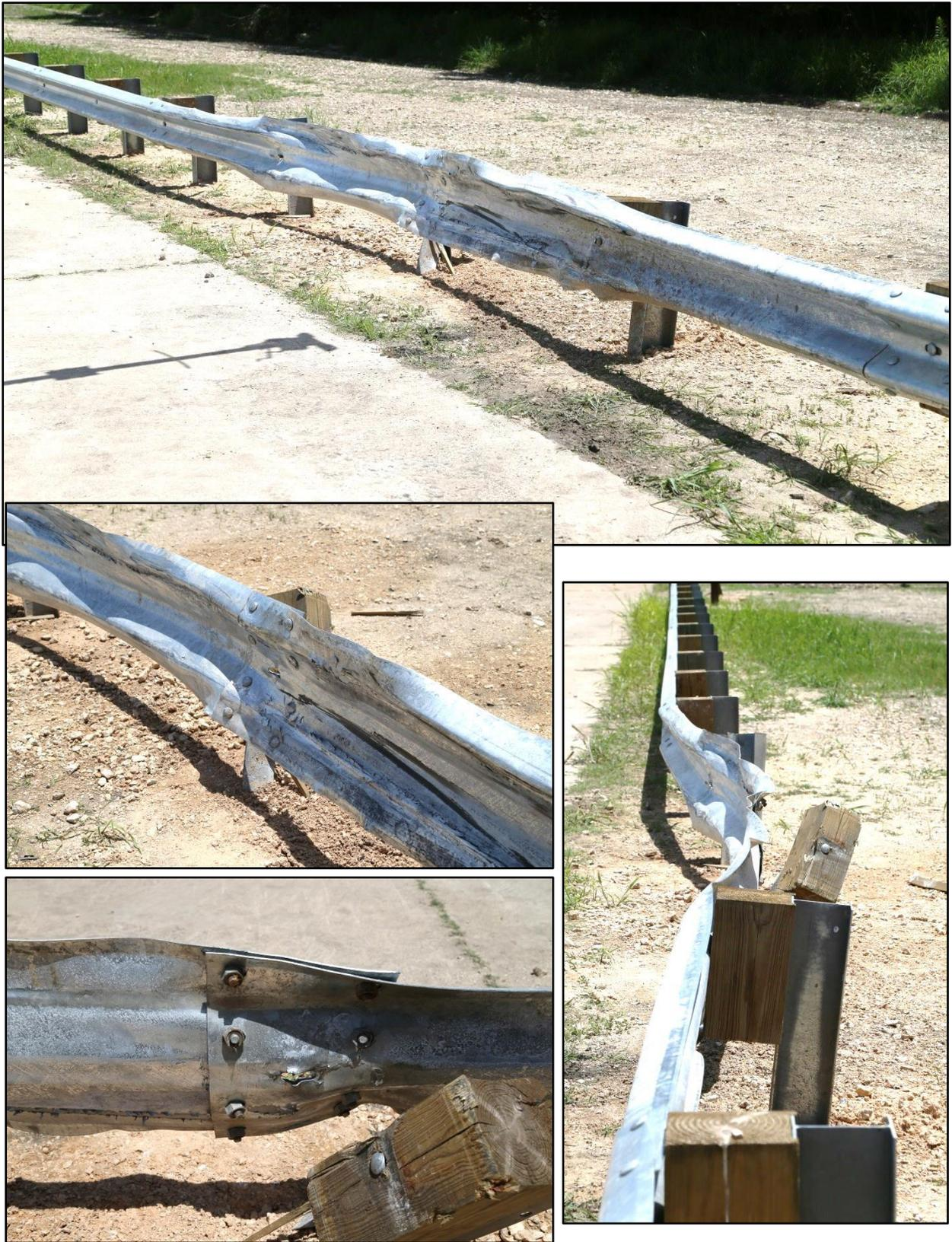
**Figure 5.6. Installation after Test No. 6012361-2.**
