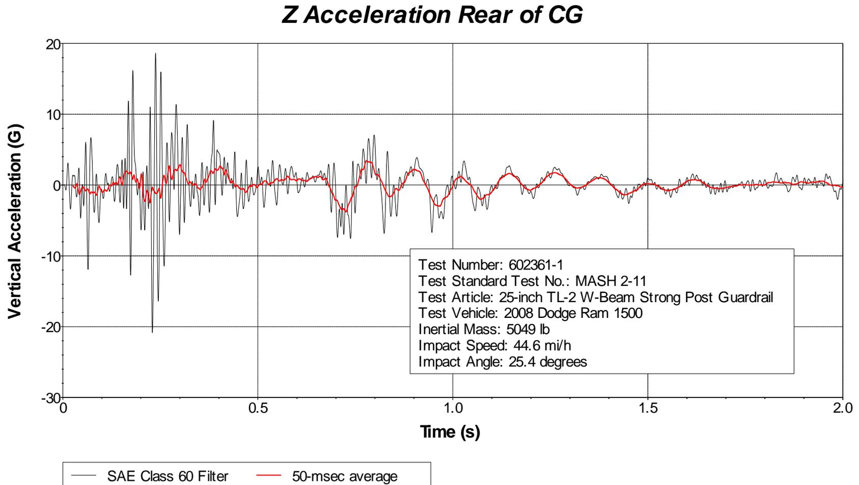
**Figure C.8. Vehicle Vertical Accelerometer Trace for Test No. 602361-1
