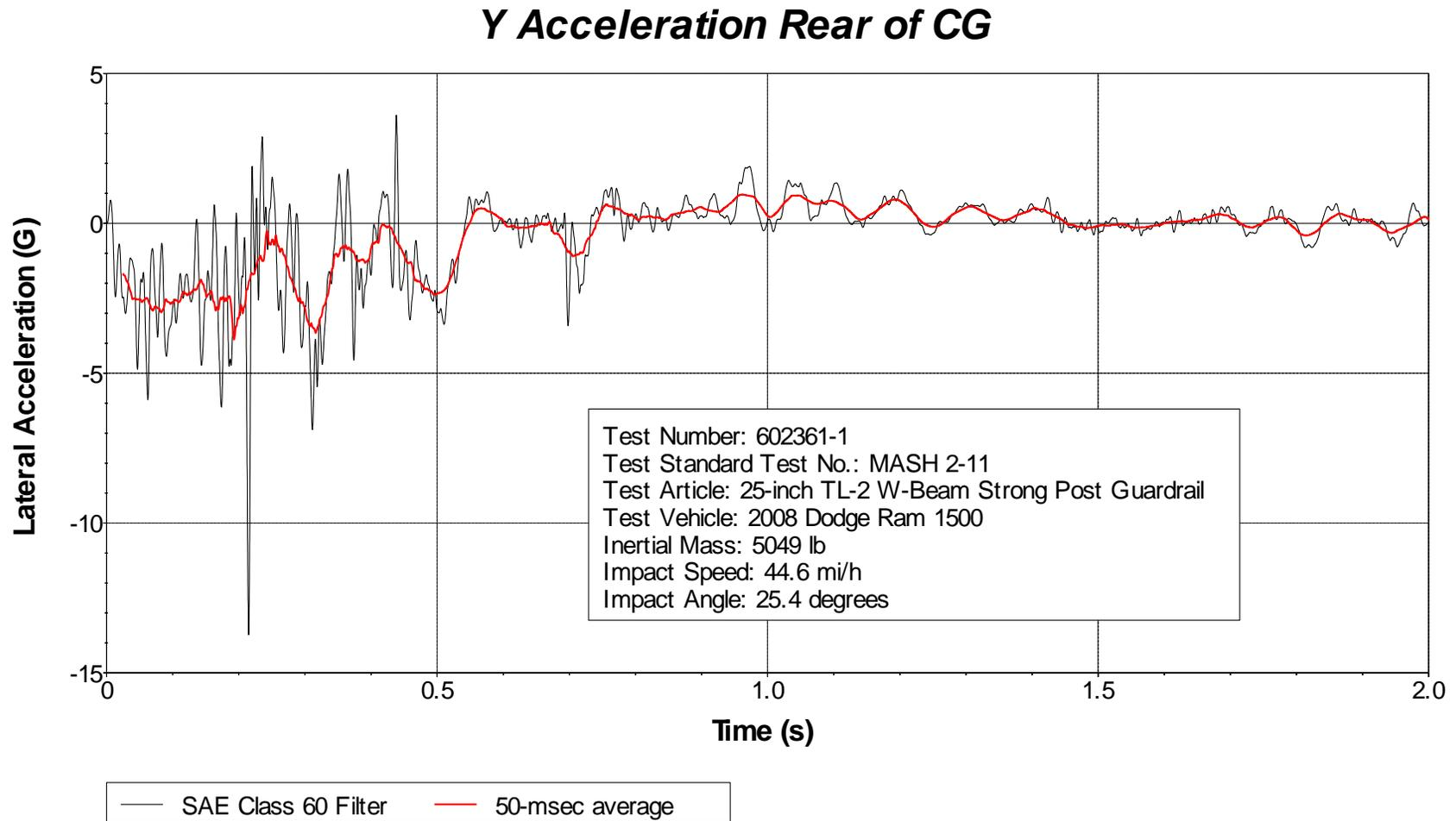
**Figure C.7. Vehicle Lateral Accelerometer Trace for Test No. 602361-1
