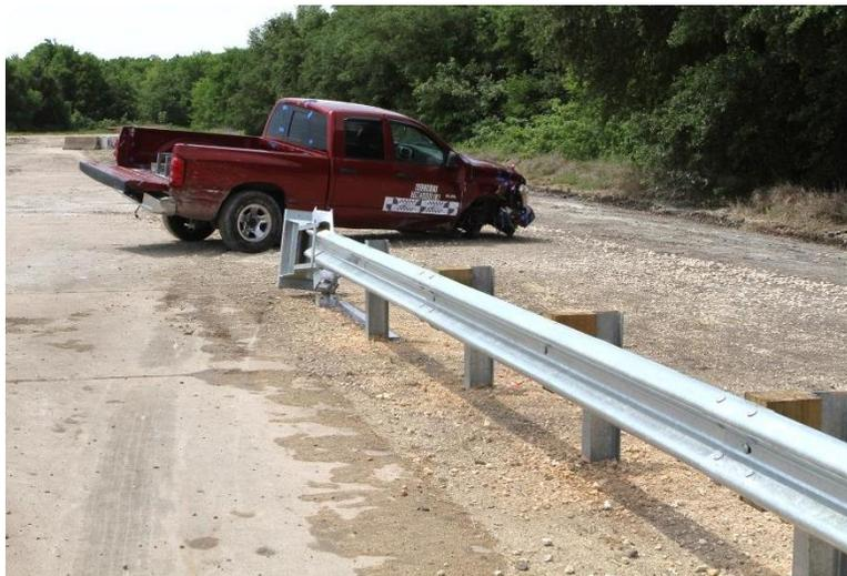
**Figure 4.5. Vehicle and 25-inch tall W-beam Guardrail after Test No. 602361-1.**
