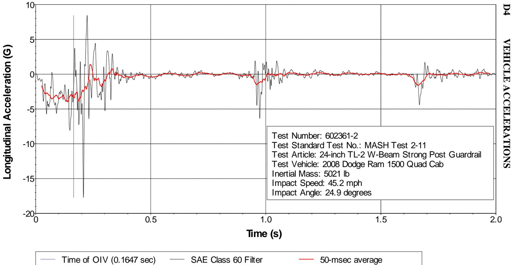
**Figure D.4. Vehicle Longitudinal Accelerometer Trace for Test No. 602361-2 (Accelerometer Located at Center of Gravity).**
