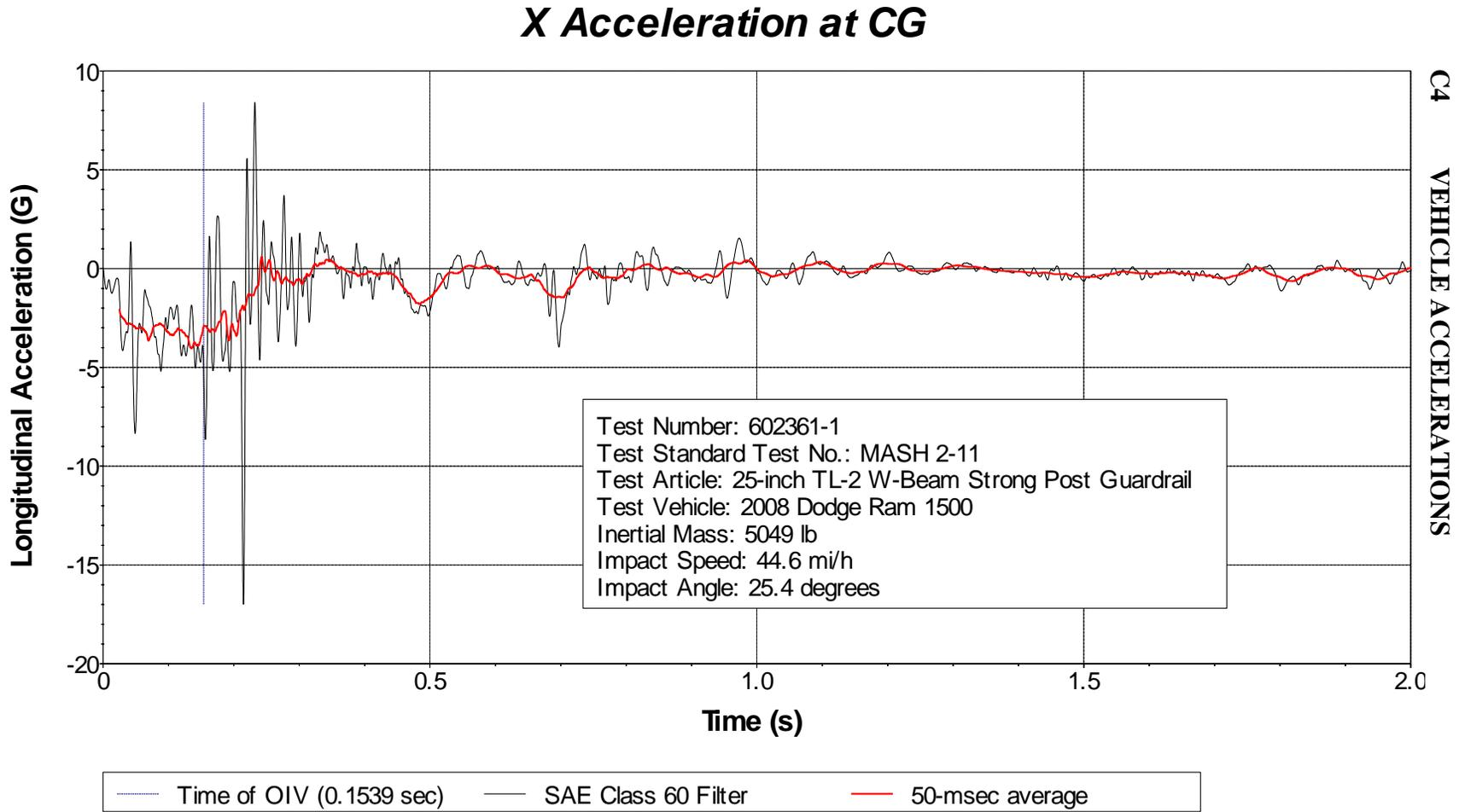
**Figure C.3. Vehicle Longitudinal Accelerometer Trace for Test No. 602361-1
