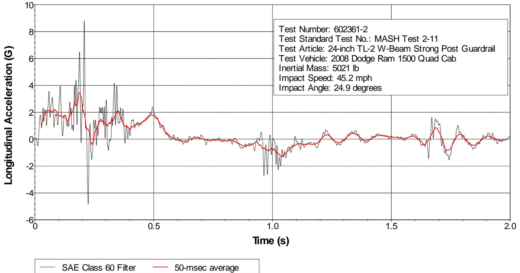
**Figure D.7. Vehicle Longitudinal Accelerometer Trace for Test No. 602361-2 (Accelerometer Located Rear of Center of Gravity).**
