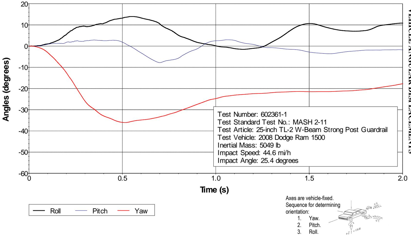
Figure C.2. Vehicle Angular Displacements for Test No. 602361-1.
