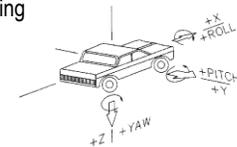
Figure D.3. Vehicle Angular Displacements for Test No. 602361-2.
