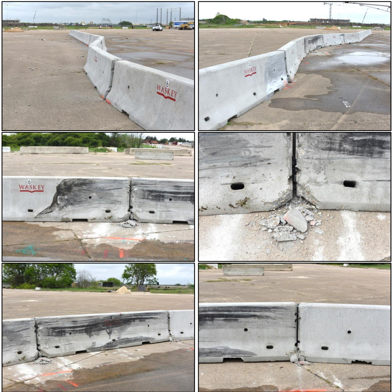
Figure 6.3. Free-Standing PCB after Test No. 607911-2.
