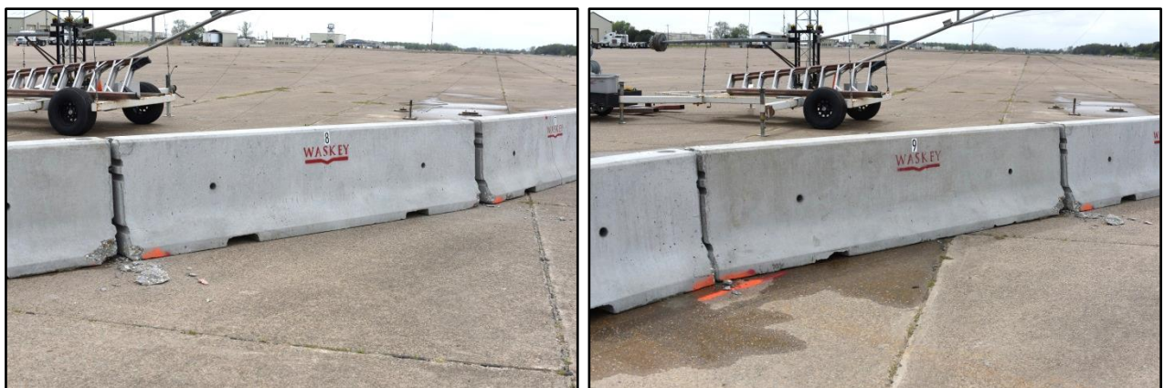
Figure 6.6. Field Side of Segments 8 and 9 after Test No. 607911-2.
