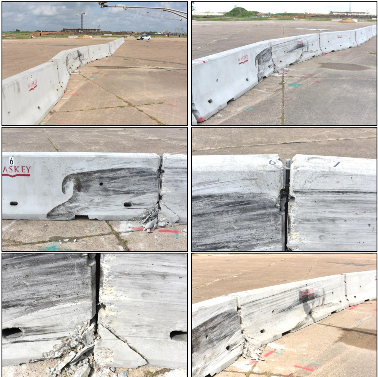
Figure 5.3. Free-Standing PCB after Test No. 607911-1.
