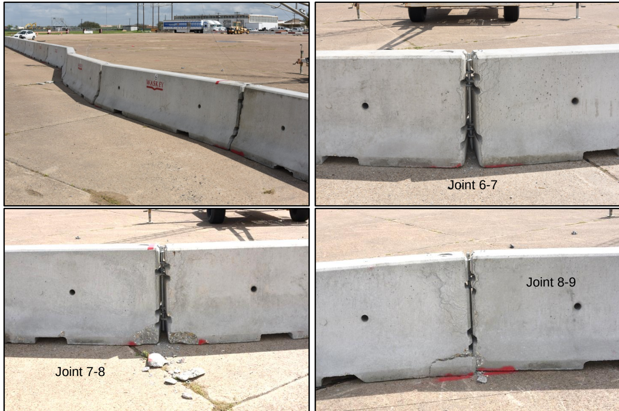
Figure 5.4. Field Side Free-Standing PCB after Test No. 607911-1.
