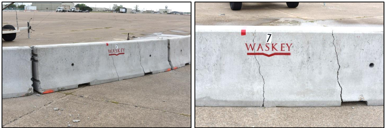
Figure 6.5. Field Side of Segment 7 after Test No. 607911-2.
