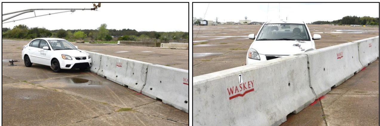
Figure 5.1. Free-Standing PCB/Test Vehicle Geometrics for Test No. 607911-1.
