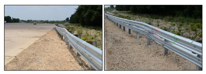
Figure 5.3. BIB Terminal after Test No. 608431-01-2.
