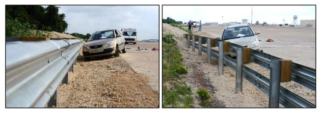
Figure 5.1. BIB Terminal/Test Vehicle Geometrics for Test No. 608431-01-2.
