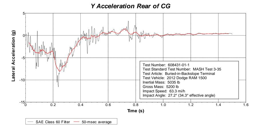
Figure D.8. Vehicle Lateral Accelerometer Trace for Test No. 608431-01-1 (Accelerometer Located Rear of Center of Gravity).
