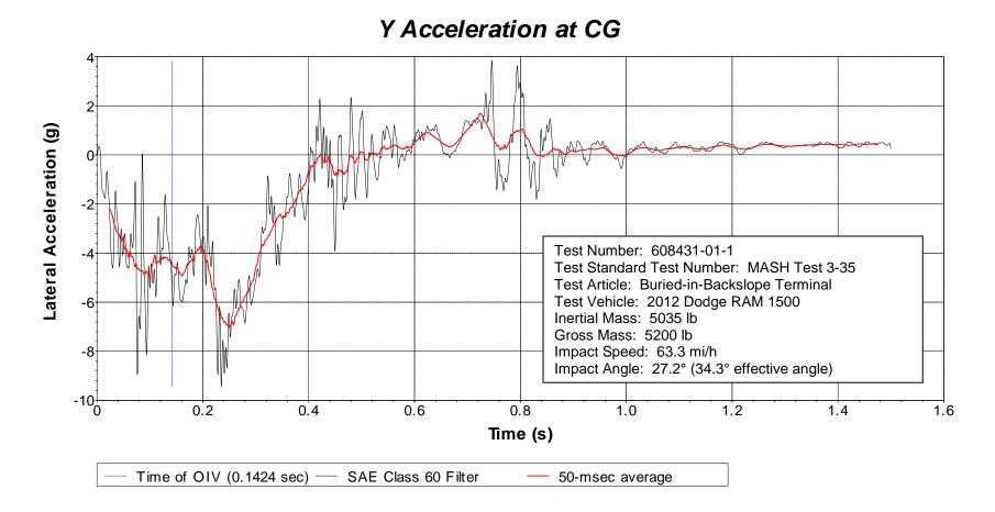
Figure D.5. Vehicle Lateral Accelerometer Trace for Test No. 608431-01-1 (Accelerometer Located at Center of Gravity).
