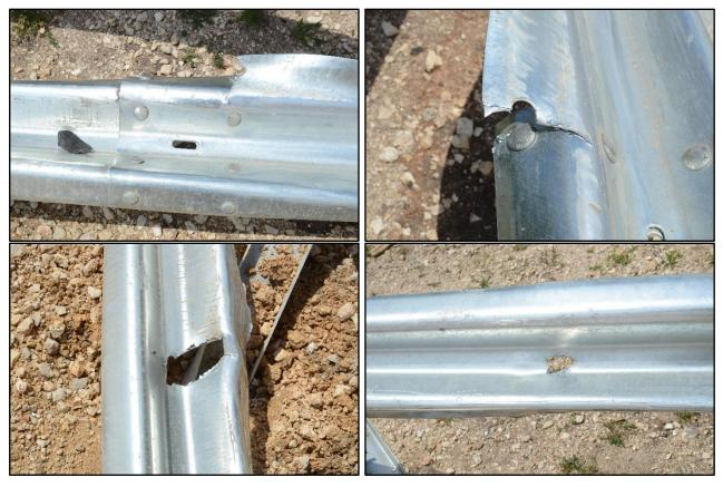
Figure 6.5. Rail Tears after Test No. 608431-01-1.
