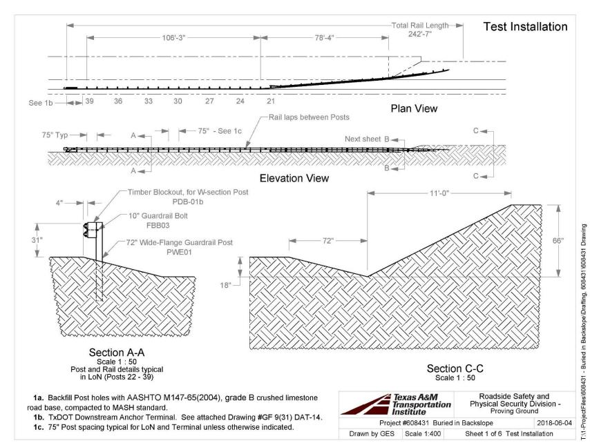
Figure 2.1. Details of the 31-inch BIB Terminal.
