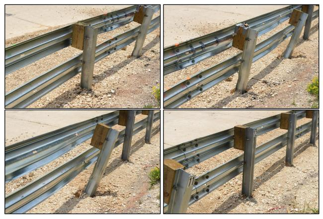
Figure 5.5. Field Side of Posts 9 through 12 after Test No. 608431-01-2.
