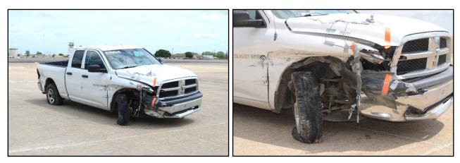
Figure 6.6. Test Vehicle after Test No. 608431-01-1.
