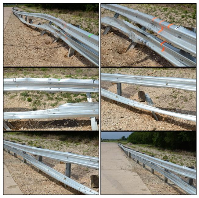
Figure 6.4. Damage at Posts 9 through 15 after Test No. 608431-01-1.
