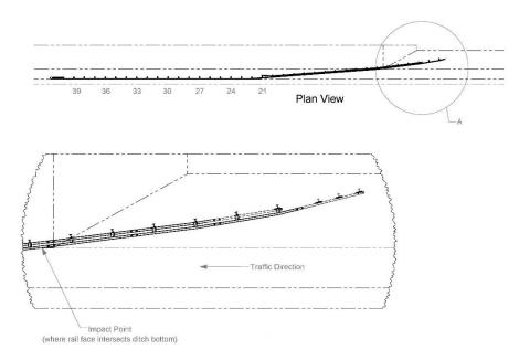
Figure 3.1. Target CIP for MASH Tests 3-34 and 3-35 on BIB Terminal.
