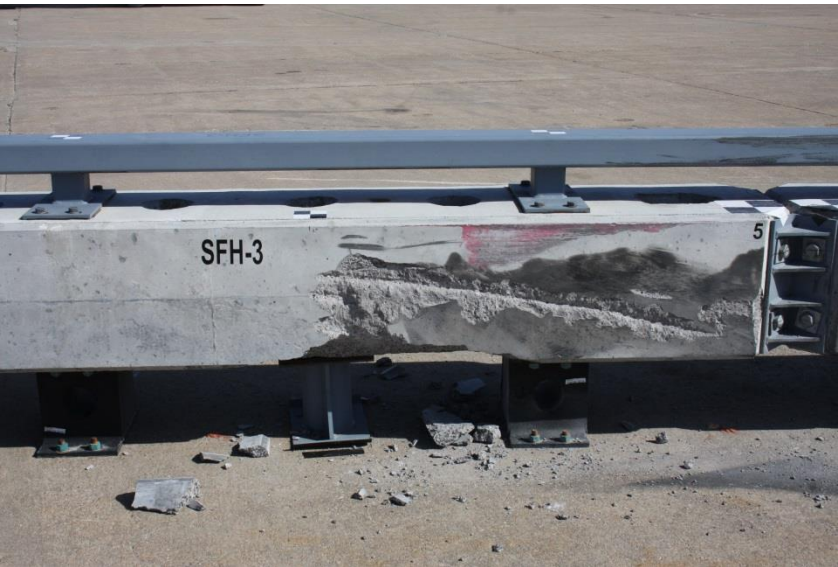
Figure 111. System Damage, Barrier No. 5 and Joint Between Barrier Nos. 5 and 6, Test No. SFH-3
