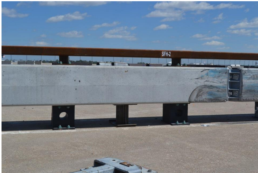
Figure 69. System Damage, Barrier No. 7, Test No. SFH-2
