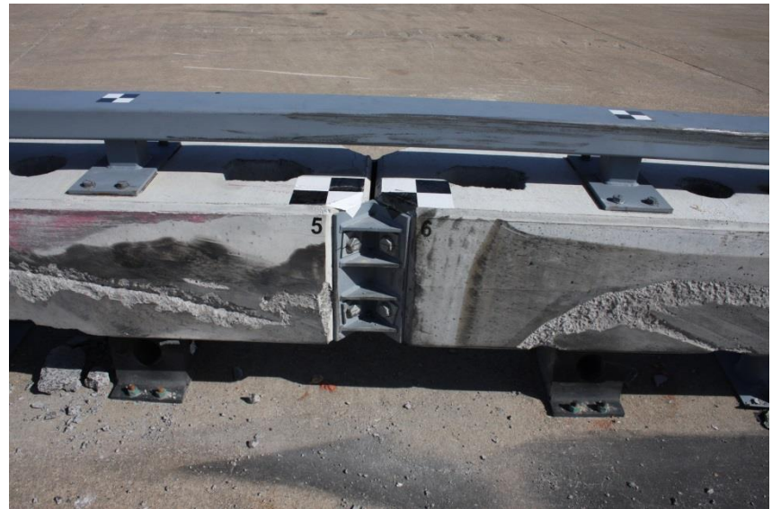
Figure 111. System Damage, Barrier No. 5 and Joint Between Barrier Nos. 5 and 6, Test No. SFH-3
