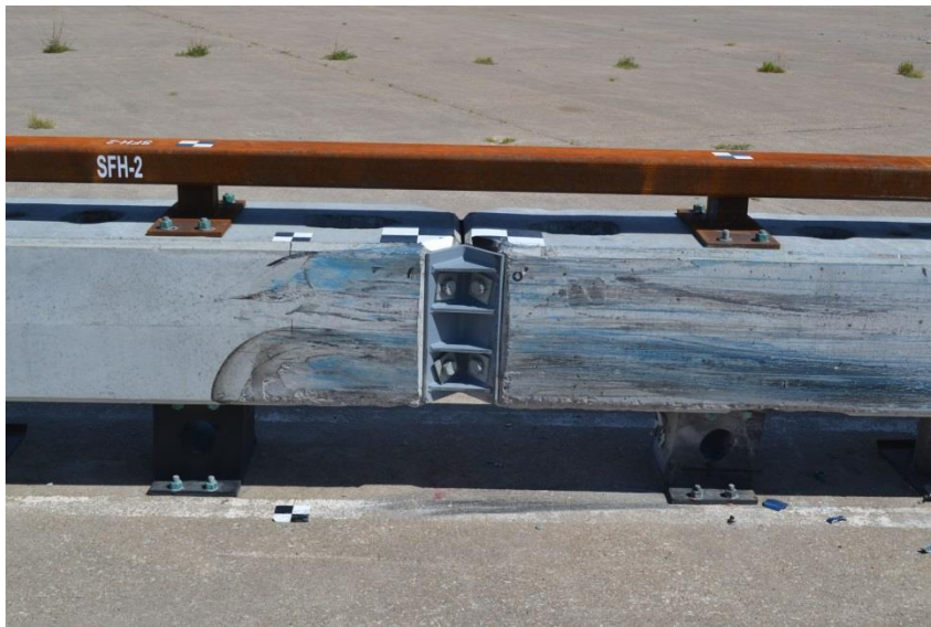
Figure 70. System Damage, Barrier No. 8, Test No. SFH-2
