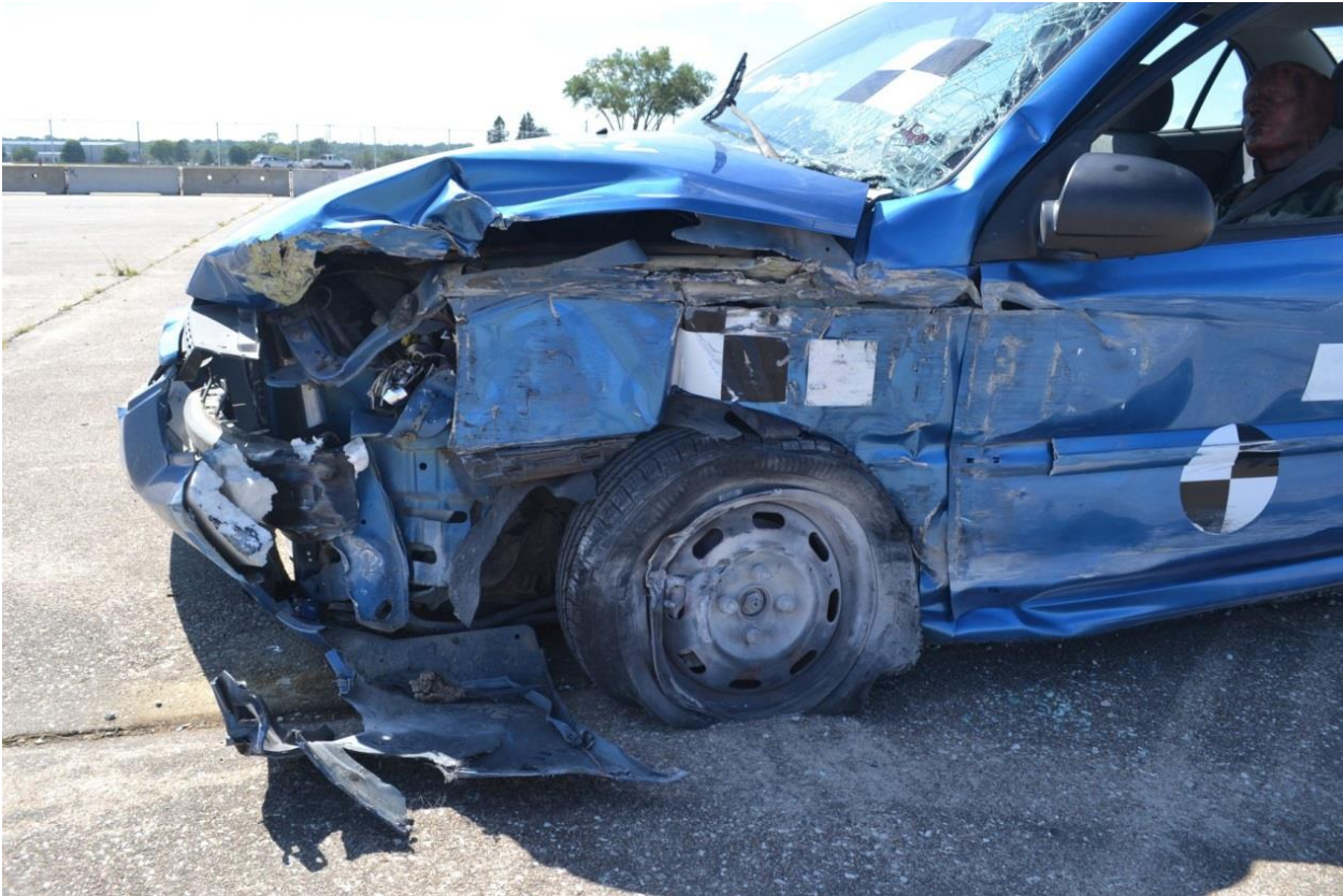
Figure 74. Vehicle Damage, Test No. SFH-2
