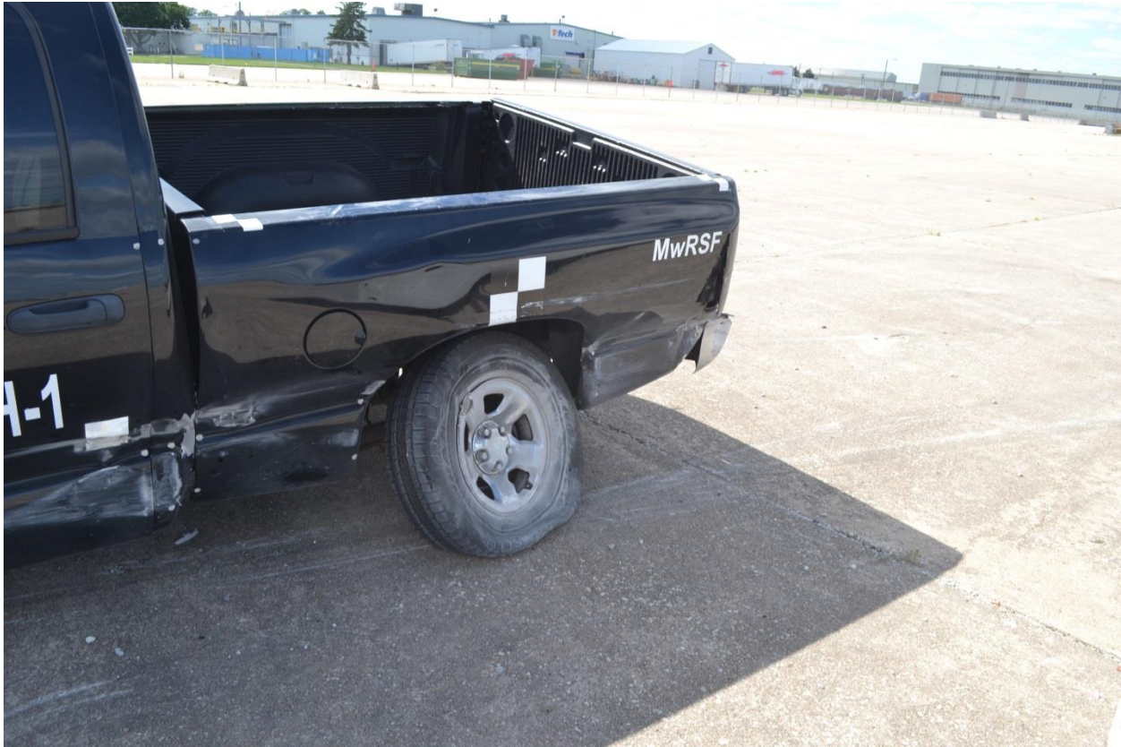
Figure 55. Vehicle Damage, Left-Front and Left-Rear Tires, Test No. SFH-1
