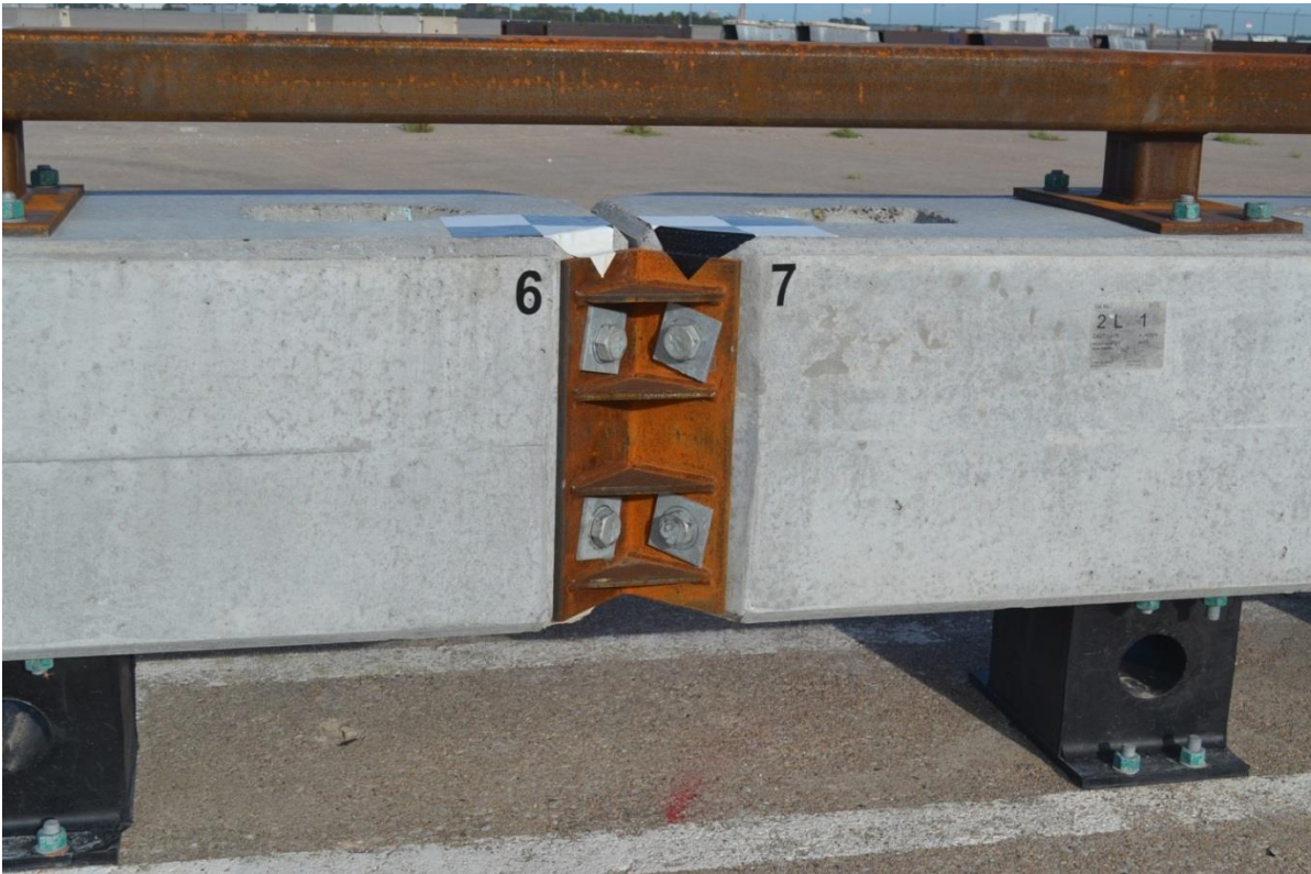
Figure 27. Test Installation Photographs, Adjustable Continuity Joint, Test Nos. SFH-1 through SFH-2
