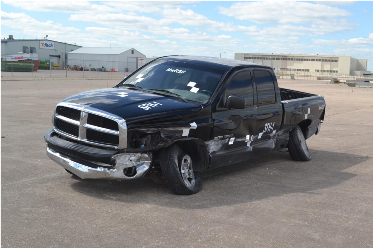
Figure 54. Vehicle Damage, Left Side, Test No. SFH-1
