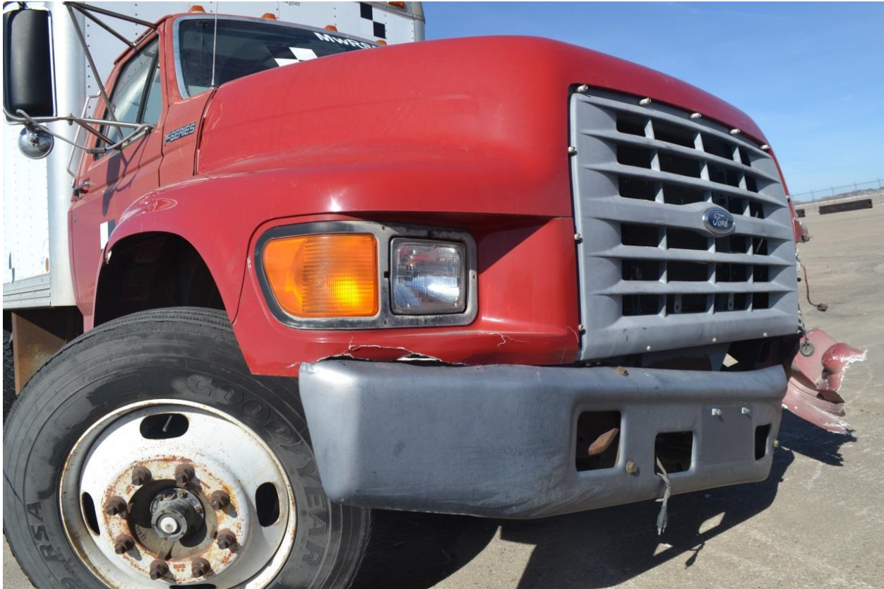
Figure 123. Vehicle Damage, Test No. SFH-3
