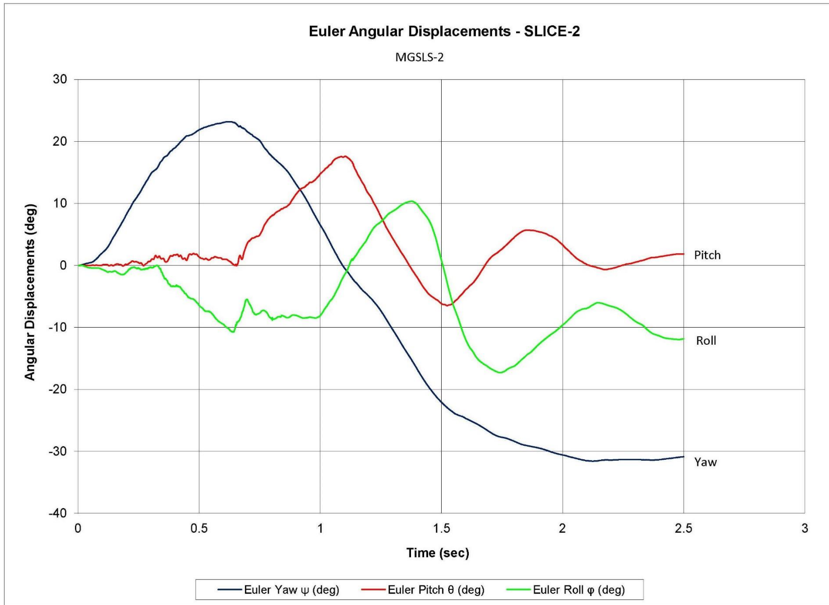
Figure F-15. Vehicle Angular Displacements (SLICE-2), Test No. MGSLs-2
