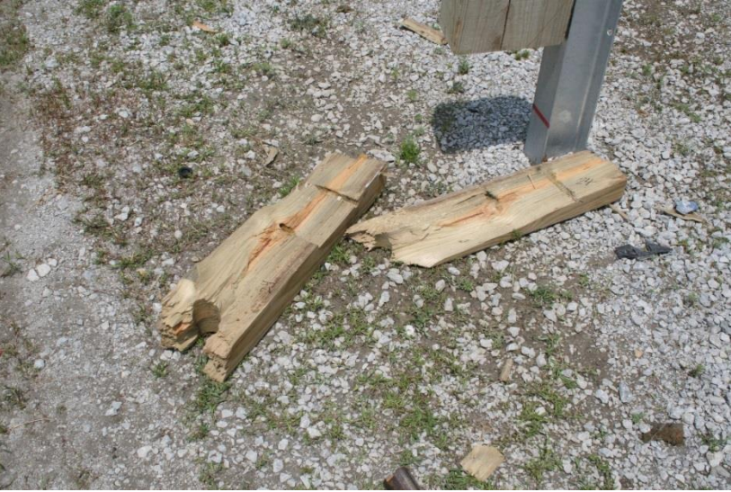
Figure 79. Damage to Post Nos. 23 through 25, Test No. MGSLs-2
