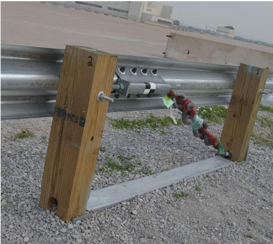
Figure 41. Test Installation Anchorage (Upstream), Test No. MGSLs-2
