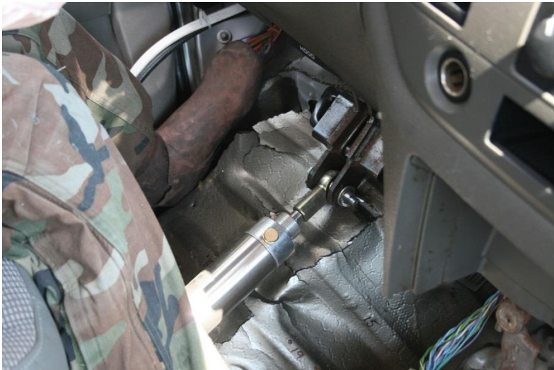
Figure 84. Occupant Compartment Damage, Test No. MGSLs-2
