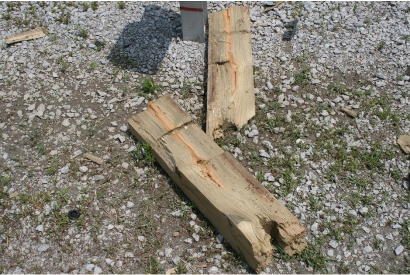
Figure 80. Downstream Anchorage Damage, Test No. MGSLS-2
