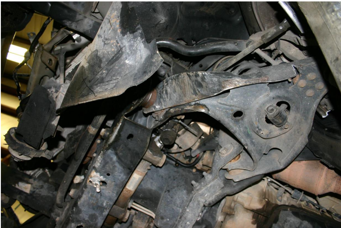
Figure 85. Vehicle Undercarriage Damage, Test No. MGSLs-2
