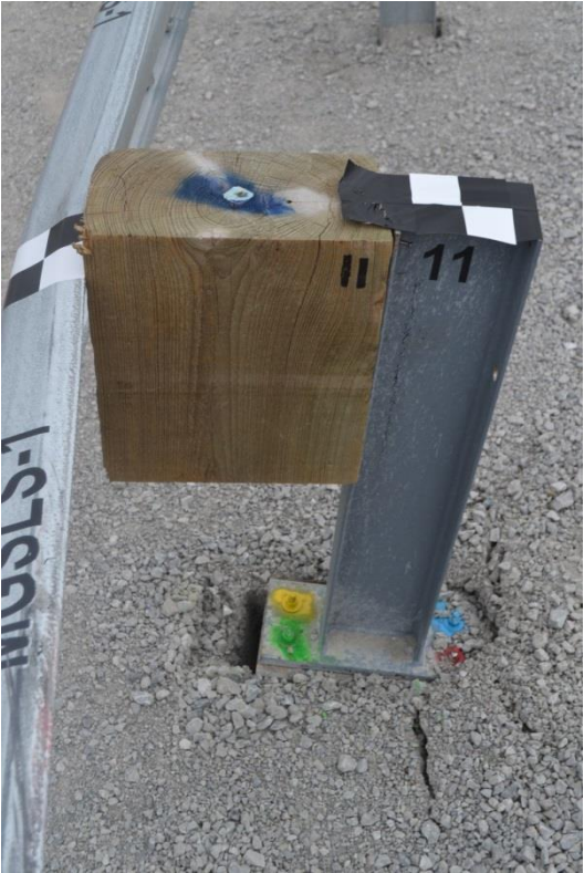
Figure 51. Damage Between Post Nos. 10 and 12, Test No. MGSL-1
