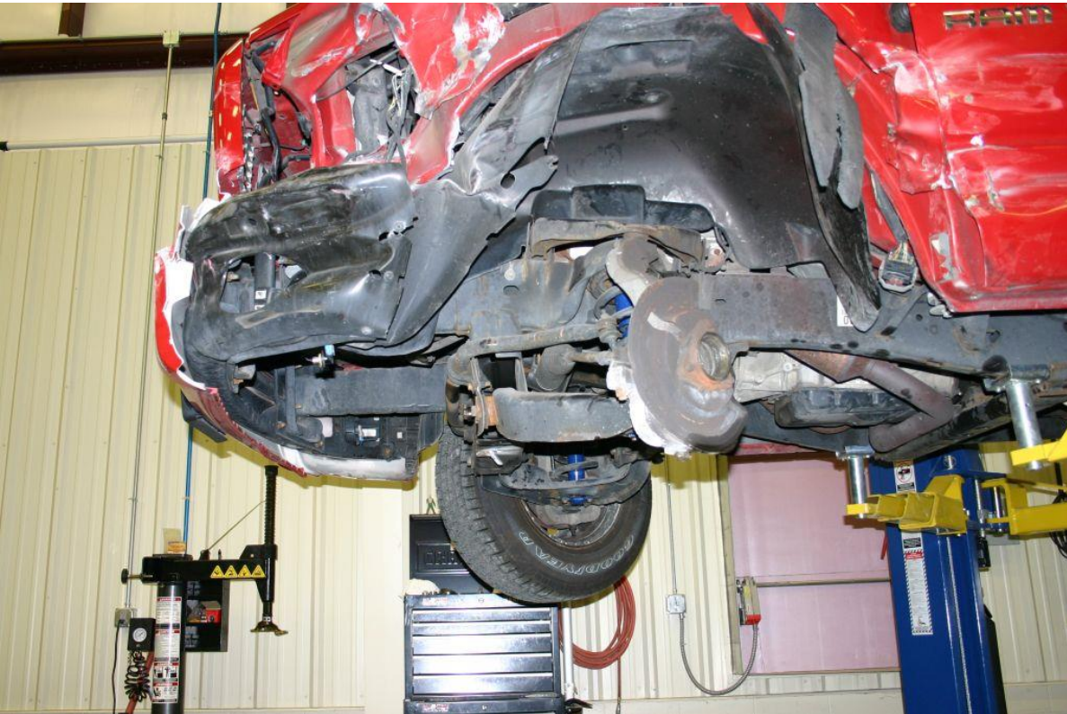
Figure 58. Vehicle Undercarriage Damage, Test No. MGSLs-1
