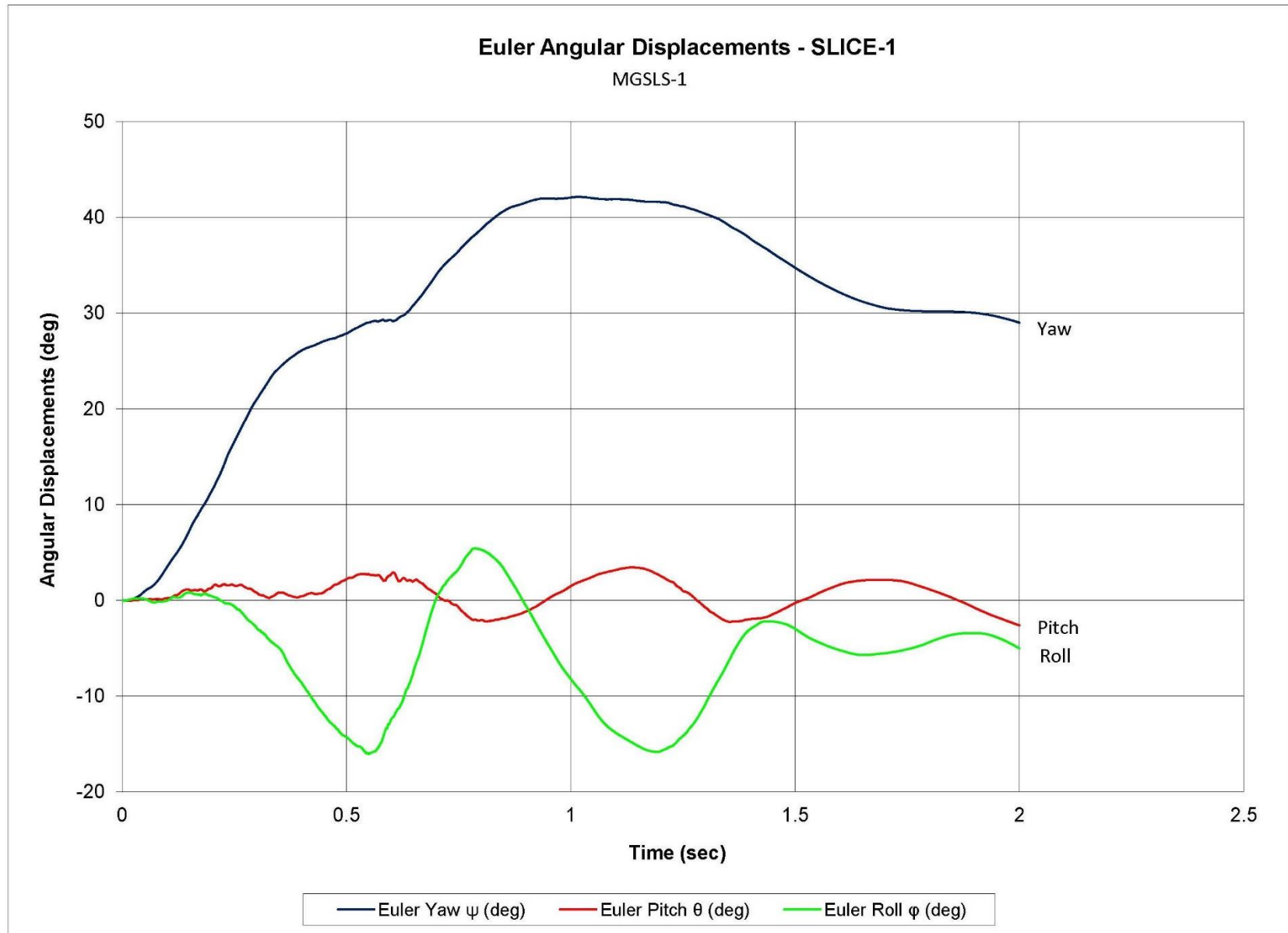
Figure E-7. Vehicle Angular Displacements (SLICE-1), Test No. MGSL-1
