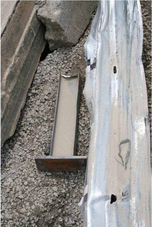
Figure 73. Damage at Post No. 14, Test No. MGSLs-2
