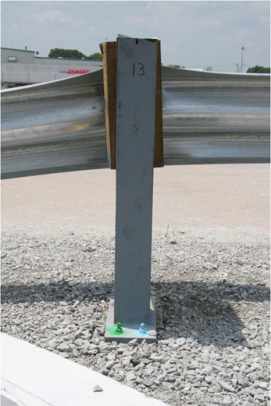
Figure 71. Damage at Post No. 13, Test No. MGSLS-2
