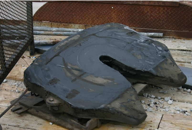
Figure 46. Fifth Wheel Plate Damage, Test No. MAN-1
