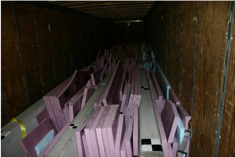
Figure 30. Test Vehicle Ballast, Test No. MAN-1
