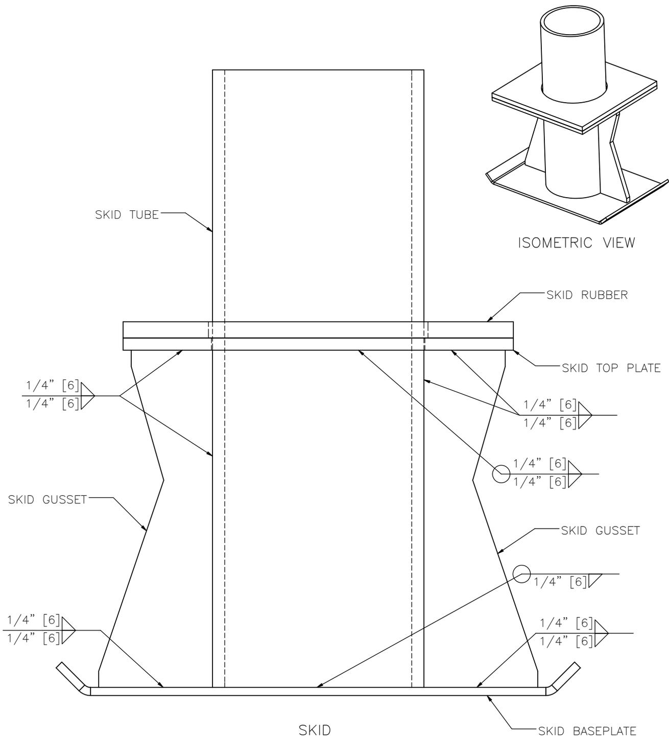
NOTE: SKID RUBBER ADDED AFTER ALL WELDING AND GALVANIZATION HAS BEEN COMPLETED.
