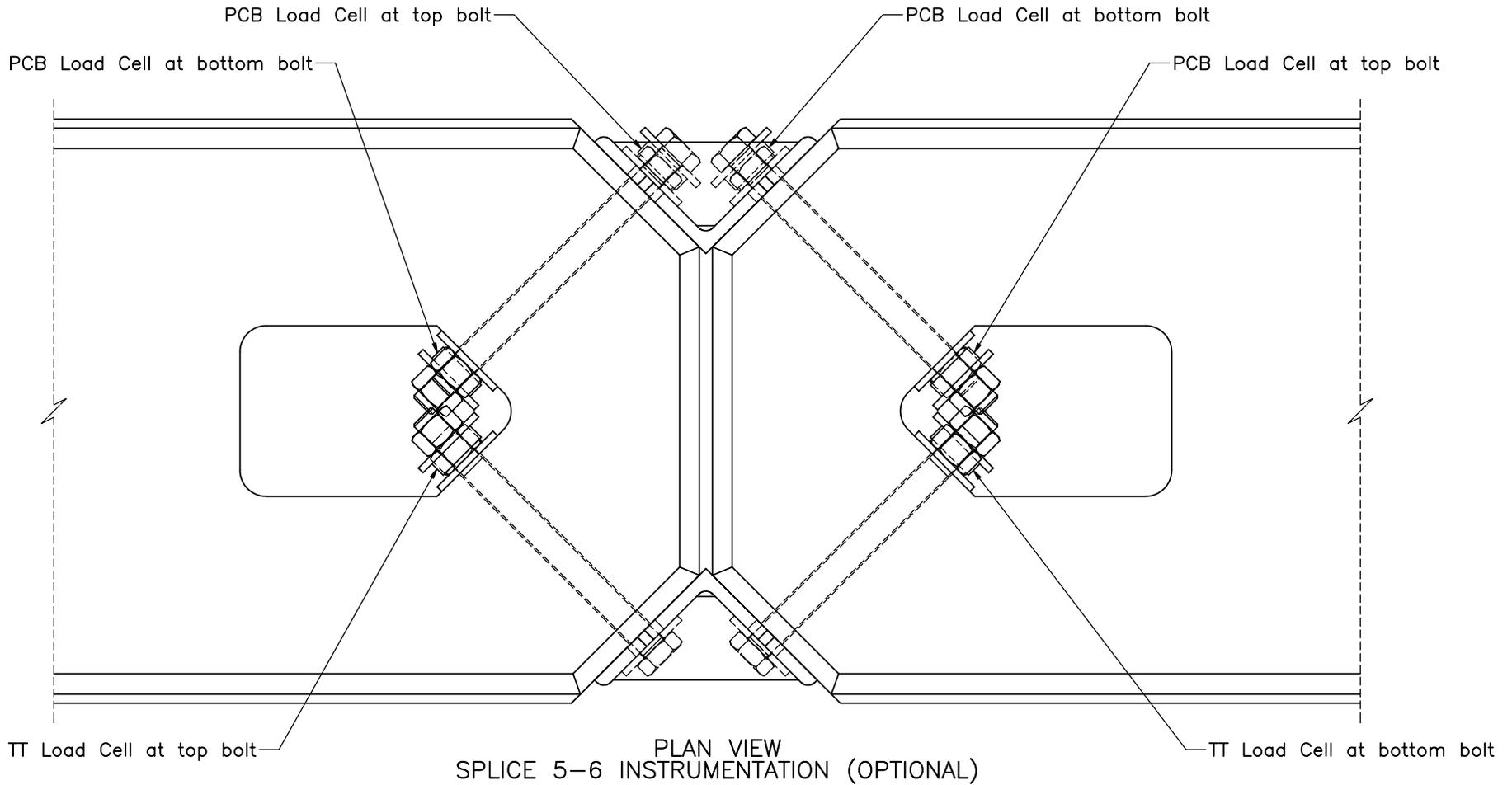
Notes: (1) Rebar, top steel tube assembly, and shear fenders removed from Plan View.
