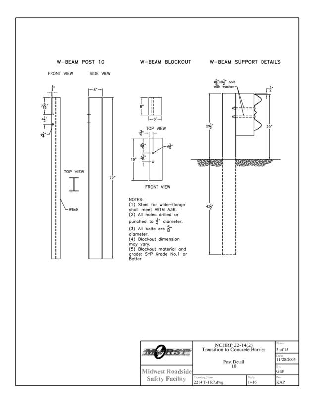
Figure A-3. Approach Guardrail Transition to Concrete Barrier Design - Post Details (English)
