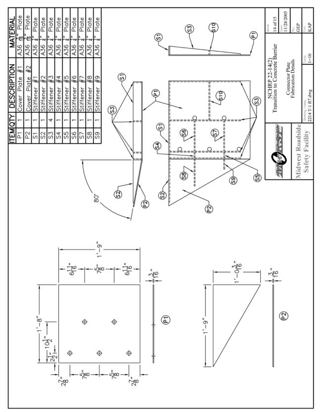
Figure A-14. Approach Guardrail Transition to Concrete Barrier Design - Connector Plate Details (English)
