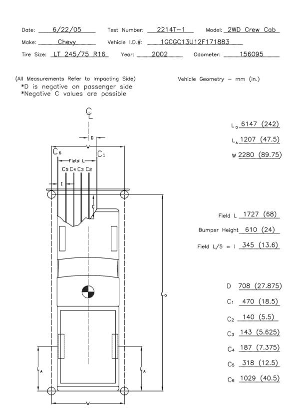
Figure C-4. NASS Crush Data, Test 2214T-1
