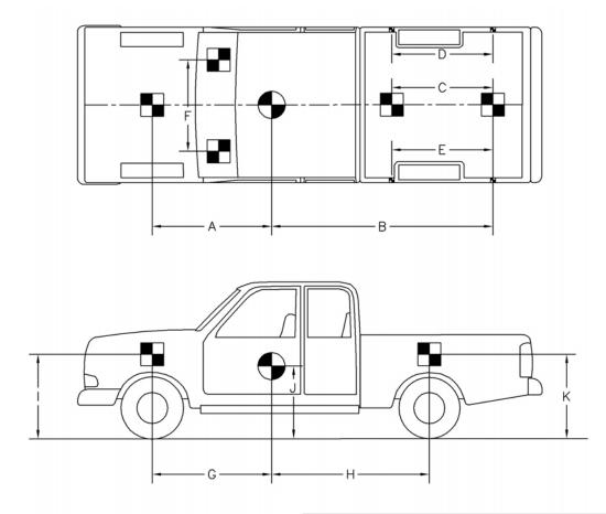
Figure 3. Vehicle Target Locations, Test 2214T-1
