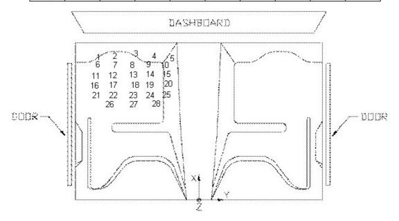
Figure C-2. Occupant Compartment Deformation Data - Set 2, Test 2214T-1
