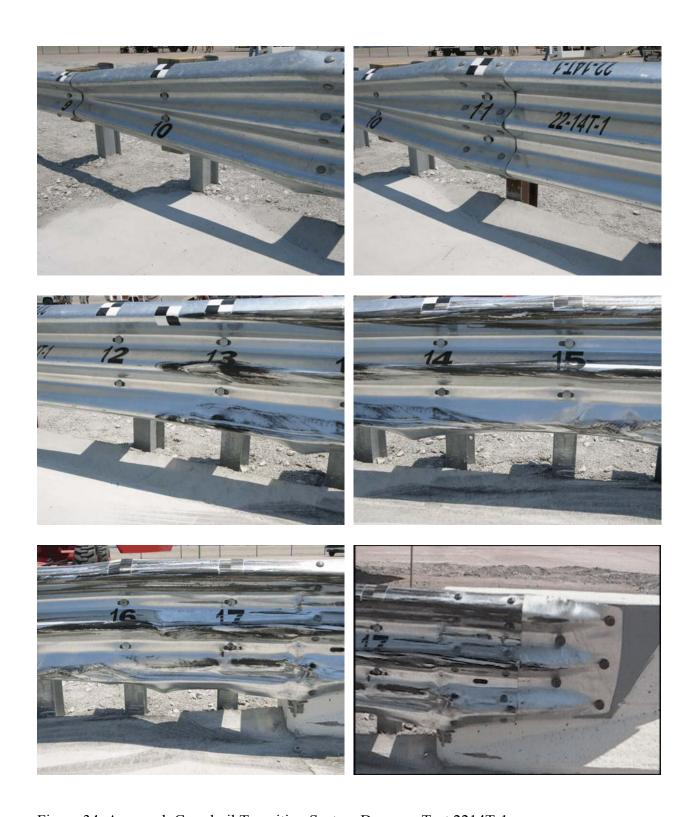
Figure 34. Approach Guardrail Transition System Damage, Test 2214T-1
