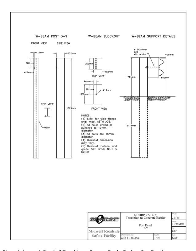
Figure 6. Approach Guardrail Transition to Concrete Barrier Design - Post Details
