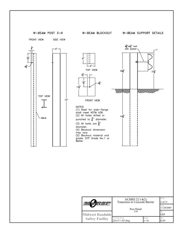
Figure A-2. Approach Guardrail Transition to Concrete Barrier Design - Post Details (English)
