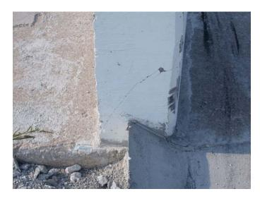
Figure 35. Concrete Barrier System Damage, Test 2214T-1
