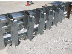
Figure 33. Approach Guardrail Transition System Damage, Test 2214T-1
