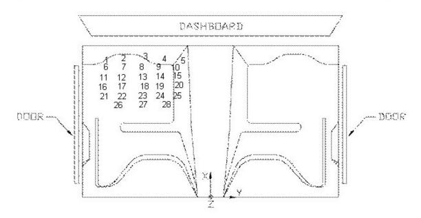
Figure C-1. Occupant Compartment Deformation Data - Set 1, Test 2214T-1
