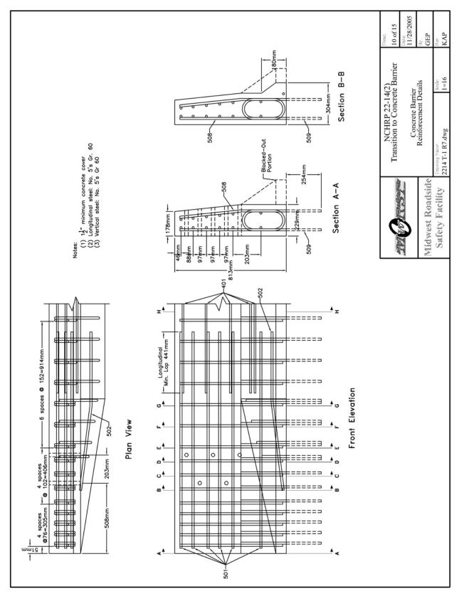
Figure 14. Approach Guardrail Transition to Concrete Barrier Design - Reinforcement Details
