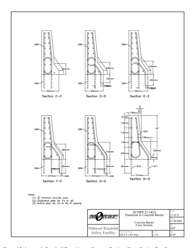
Figure 15. Approach Guardrail Transition to Concrete Barrier - Cross Section Details
