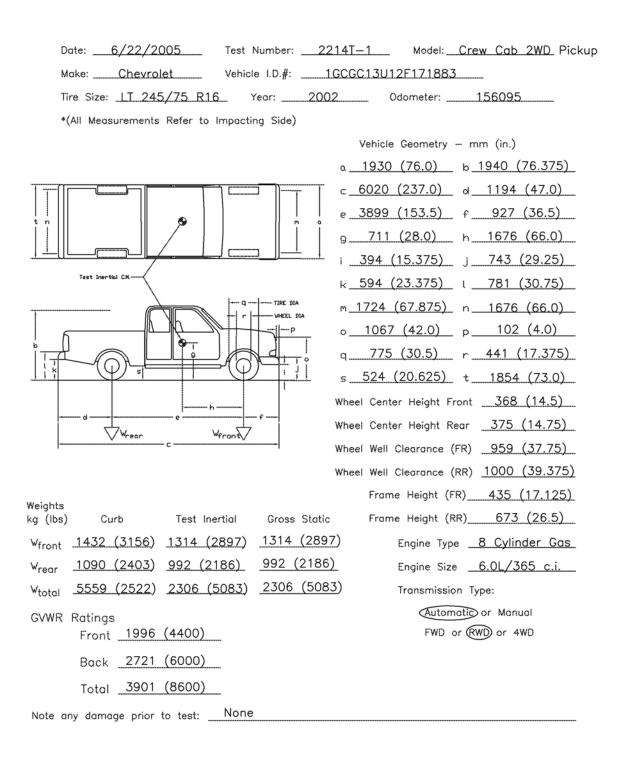
Figure 2. Vehicle Dimensions, Test 2214T-1
