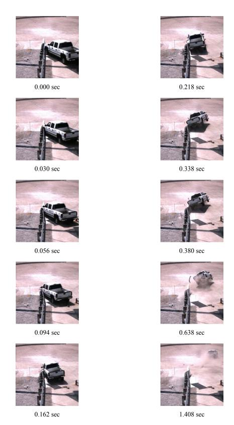
Figure 27. Additional Sequential Photographs, Test 2214T-1
