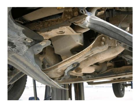
Figure 40. Vehicle Undercarriage Damage, Test 2214T-1
