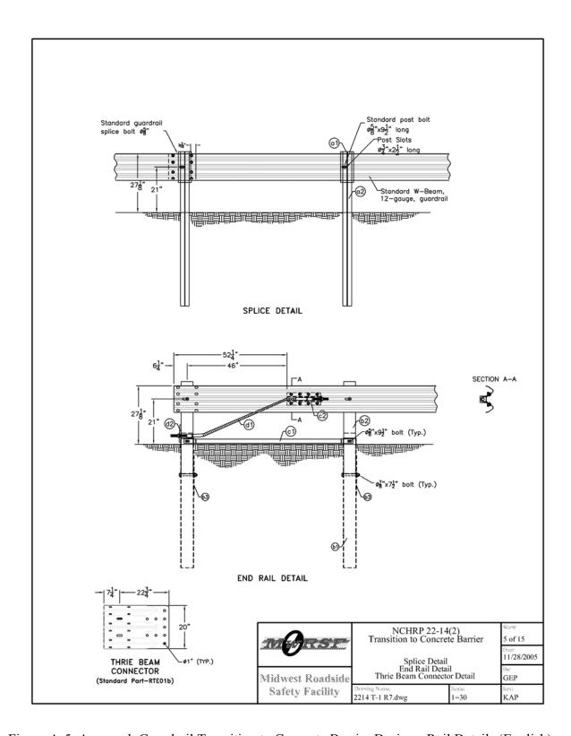
Figure A-5. Approach Guardrail Transition to Concrete Barrier Design - Rail Details (English)
