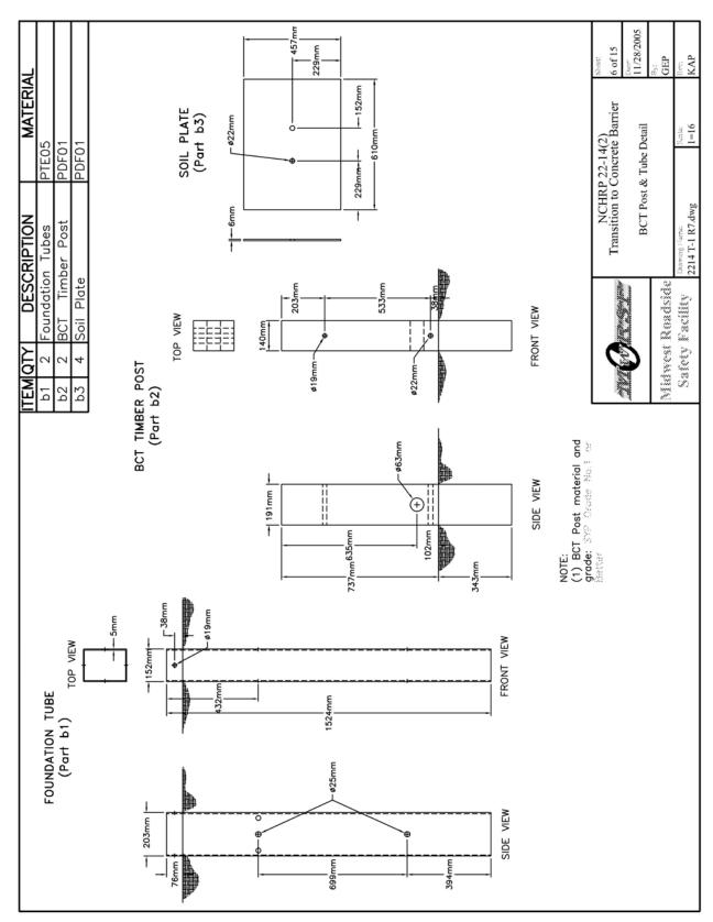
Figure 10. Approach Guardrail Transition to Concrete Barrier Design - Anchorage Details
