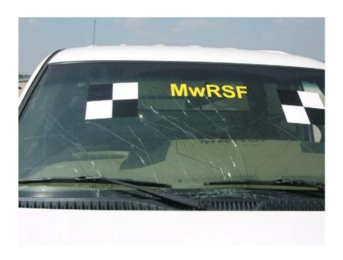
Figure 39. Vehicle Windshield Damage, Test 2214T-1
