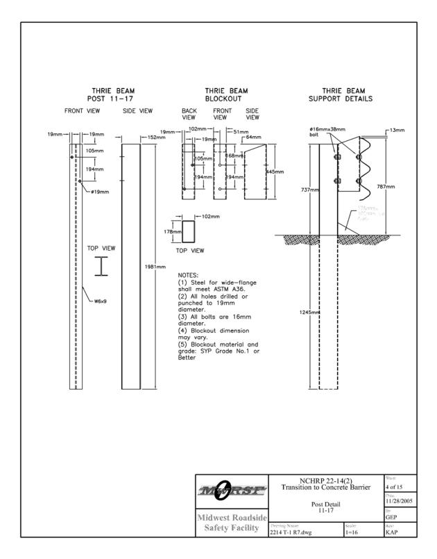
Figure 8. Approach Guardrail Transition to Concrete Barrier Design - Post Details
