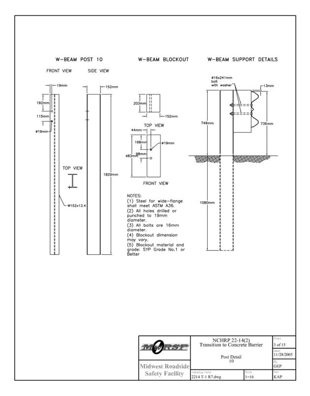
Figure 7. Approach Guardrail Transition to Concrete Barrier Design - Post Details
