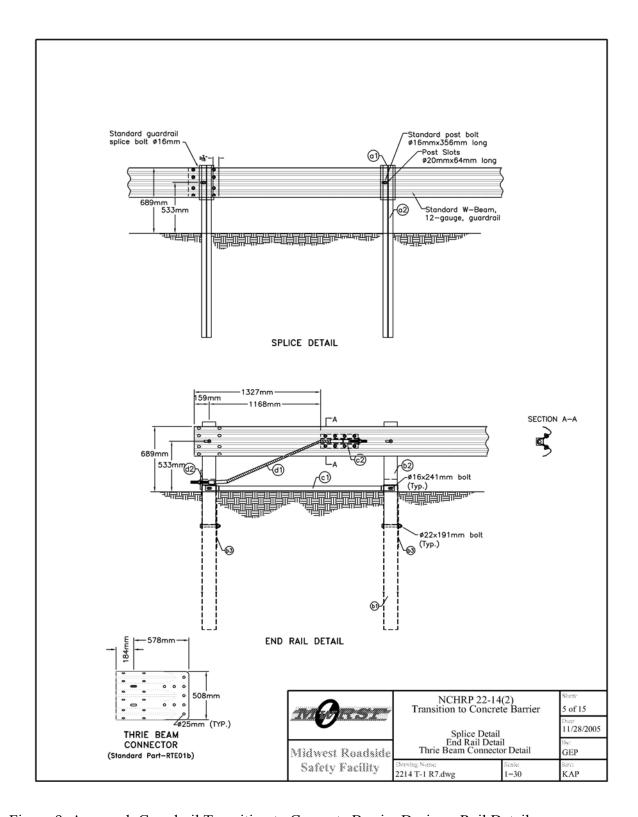
Figure 9. Approach Guardrail Transition to Concrete Barrier Design - Rail Details
