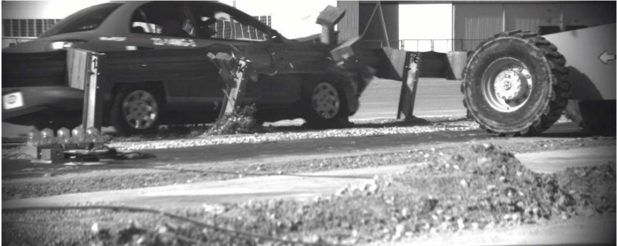
Figure 3. Test No. 2214MG-3, Wheel Snag
