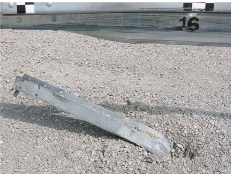
Figure 66. Post Damage, Test No. MGSMRH-2
