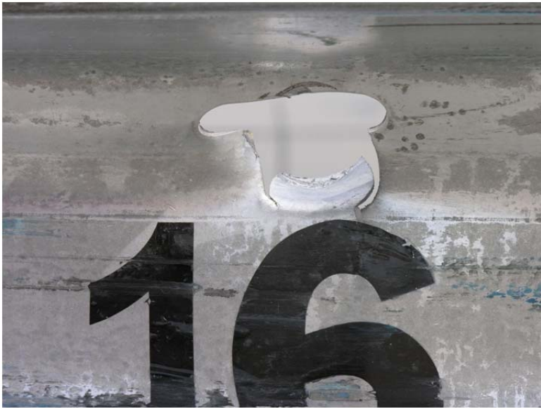
Figure 64. Post-To-Rail Bolt Hole Damage, Test No. MGSMRH-2
