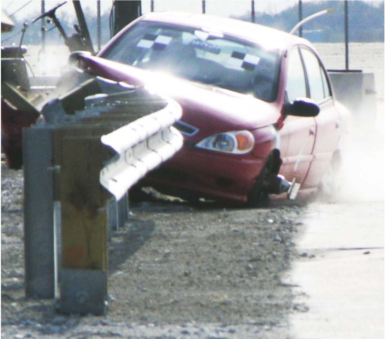
Figure 5. Test No. 2214MG-3, Rail Snags Under the Hood
