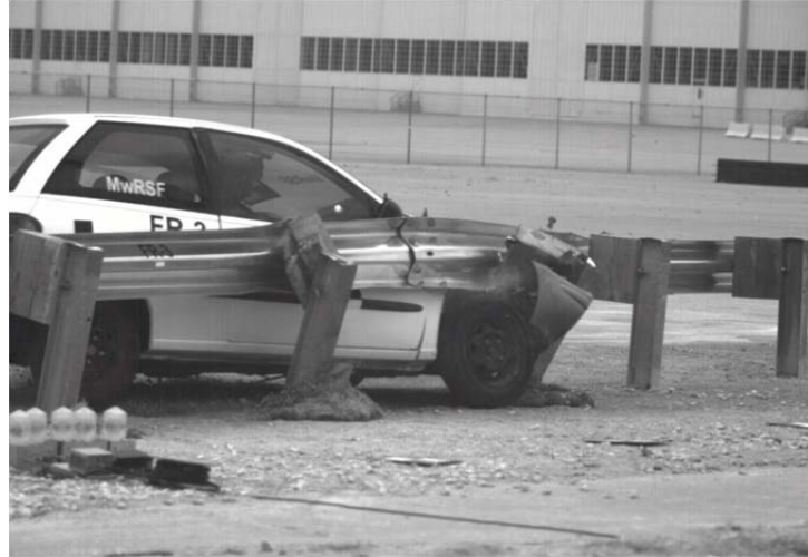
Figure 1. Test No. FR-3, Potential for Wheel Snag
