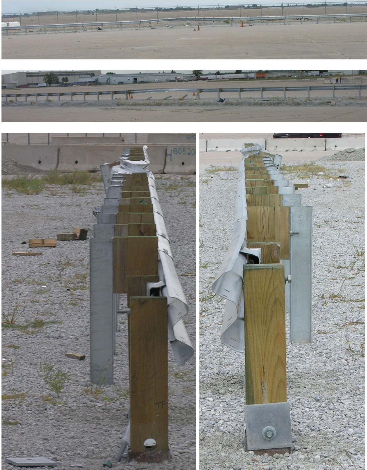
Figure 61. System Damage, Test No. MGSMRH-2
