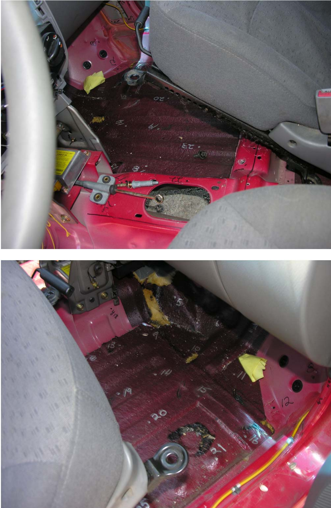
Figure 48. Occupant Compartment Damage, Test No. MGSMRH-1
