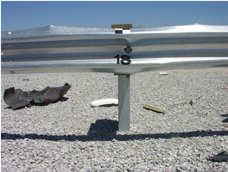
Figure 45. Post Nos. 17 and 18 Damage, Test No. MGSMRH-1
