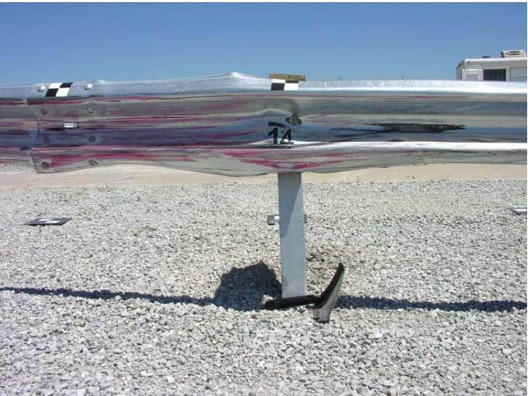
Figure 43. Post Nos. 13 and 14 Damage, Test No. MGSMRH-1
