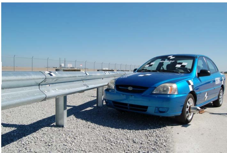
Figure 9. 1100C Next to 32-, 34-, and 36-in. (813-, 864-, and 914-mm) MGS – Front View
