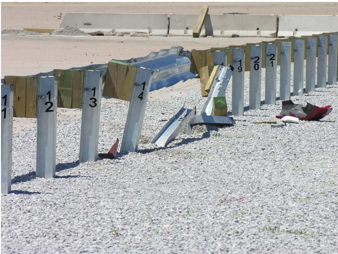
Figure 36. System Damage, Test No. MGSMRH-1
