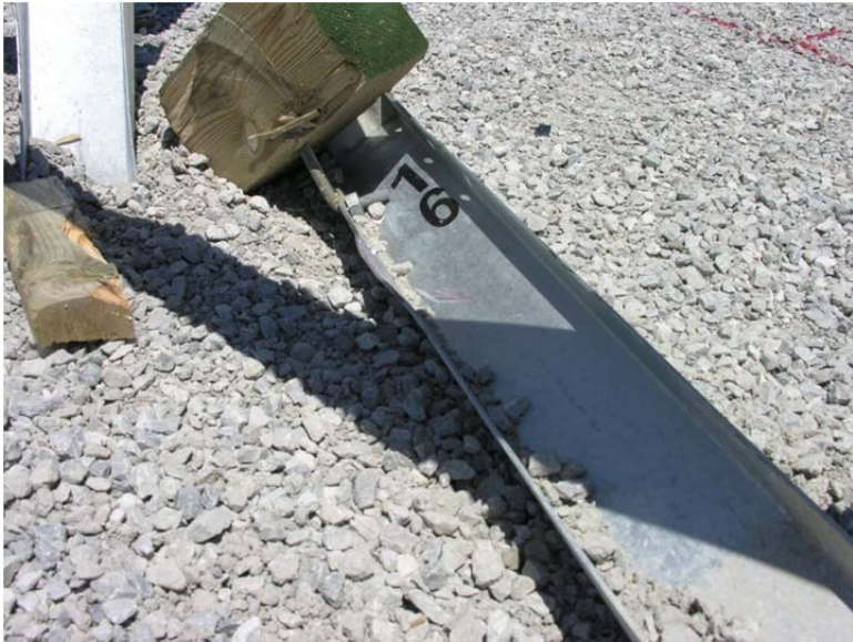
Figure 44. Post Nos. 15 and 16 Damage, Test No. MGSMRH-1
