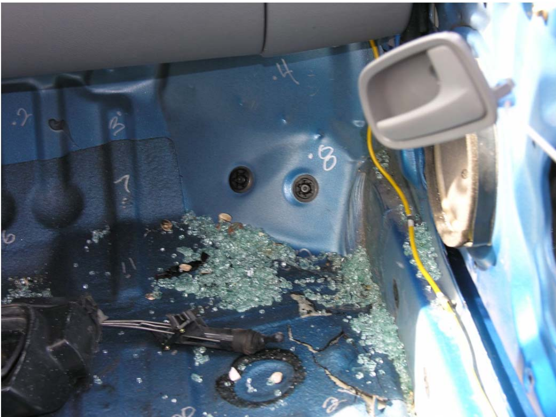
Figure 70. Occupant Compartment Damage, Test No. MGSMRH-2
