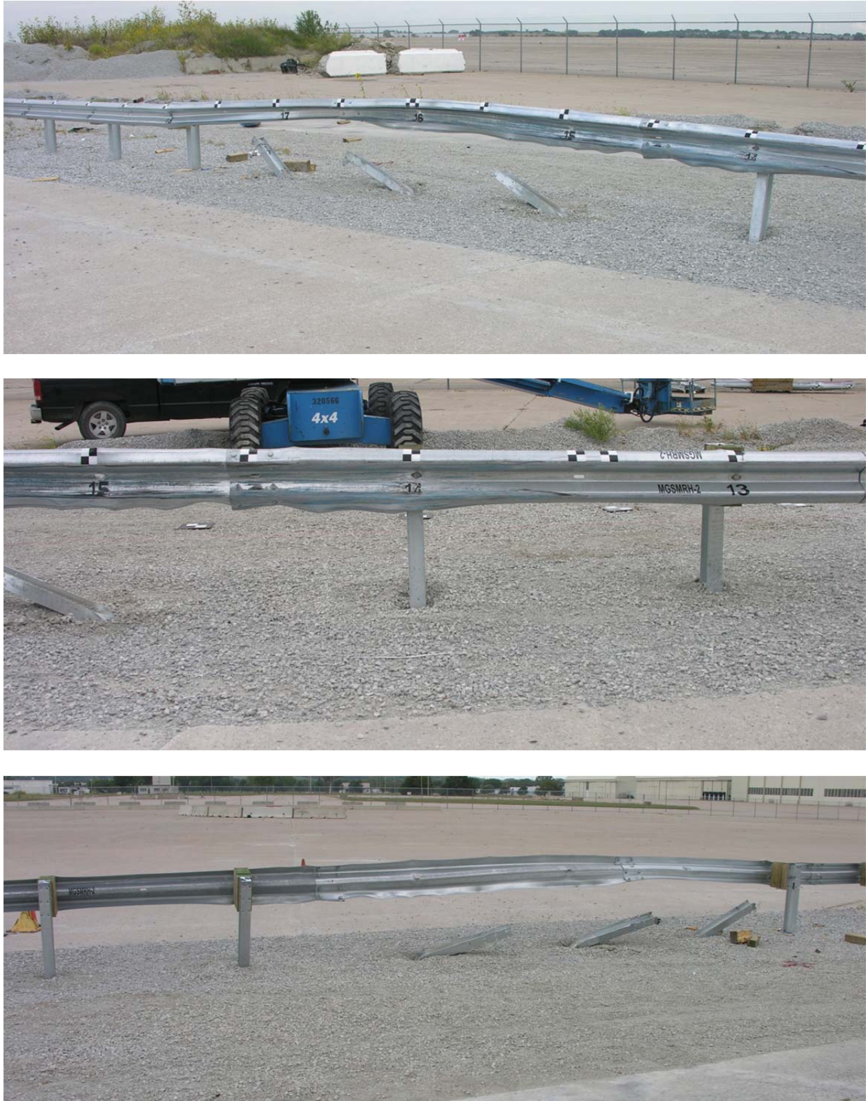
Figure 62. System Damage, Test No. MGSMRH-2
