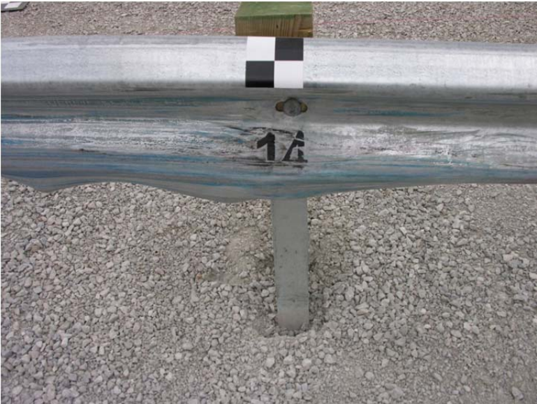
Figure 65. Post Damage, Test No. MGSMRH-2
