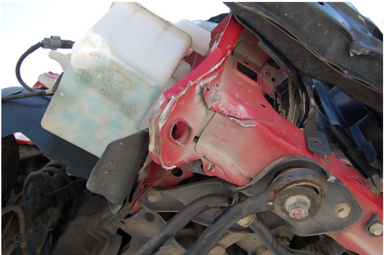
Figure 49. Undercarriage Damage, Test No. MGSMRH-1
