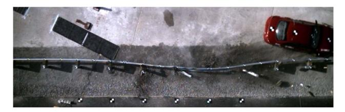
Figure 3. Vehicle Yaw Towards Barrier, test no. 2214MG-3
