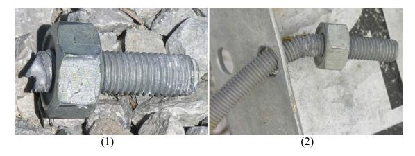
Figure 28. Blockout Bolt Failure Modes
