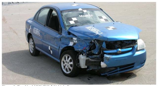
Figure 8. Test No. MGSMRH-2 Vehicle Damage
