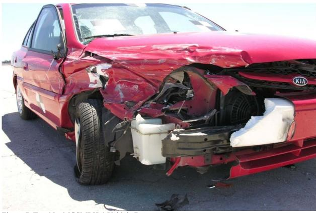
Figure 7. Test No. MGSMRH-1 Vehicle Damage
