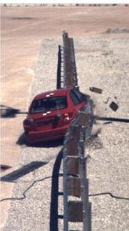
Figure 4. Test No. MGSMRH-1 Penetration
