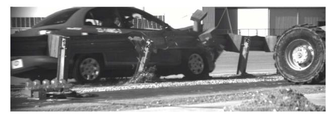
Figure 2. Underride in 1100C Impact of MGS, test no. 2214MG-3
