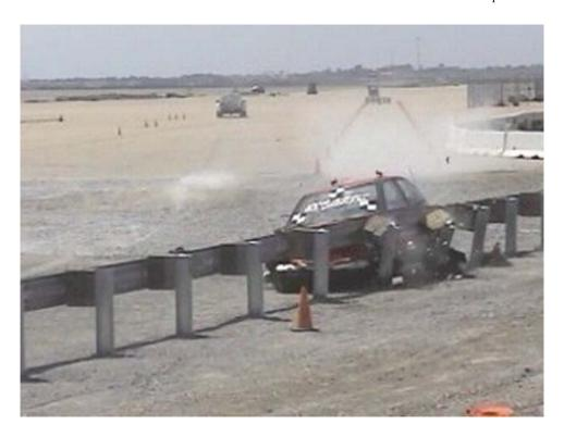
Figure 1. 820C Impact with MGS, test no. NPG-1
