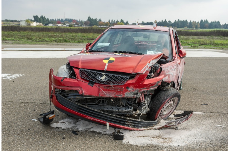
Figure 5-12 140MASH3C16-04 Kia Rio Damage (Front)
