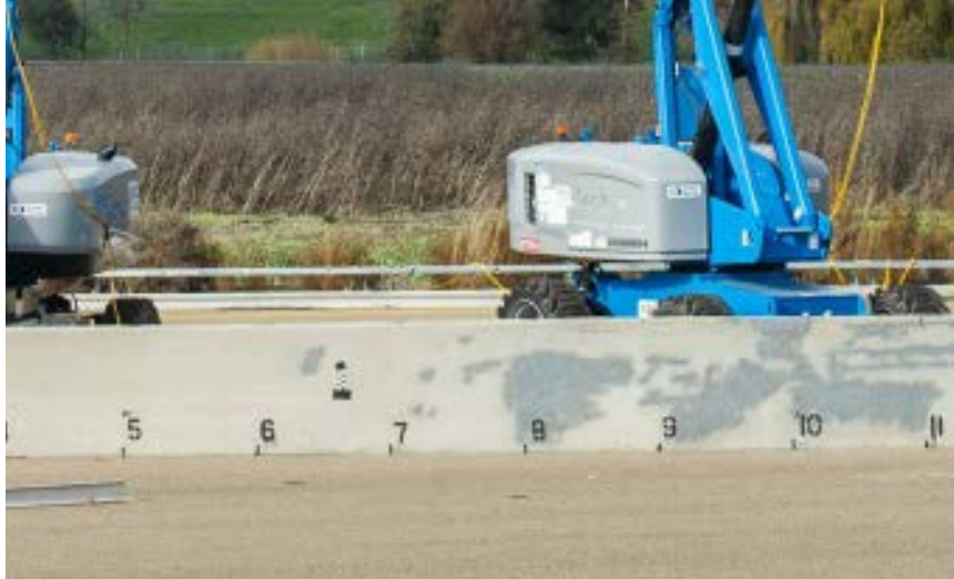
Figure 5-1 Test Article Impact Area with Checkered Tape at Impact Point
