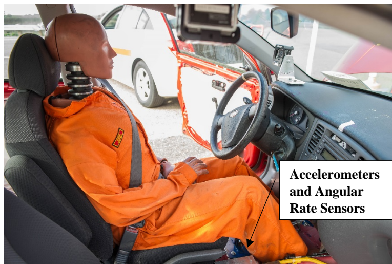
Figure 4-8 Test Vehicle Dummy and Instrumentation
