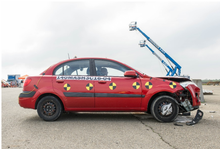
Figure 5-9 140MASH3C16-04 Kia Rio Damage (Right Side)
