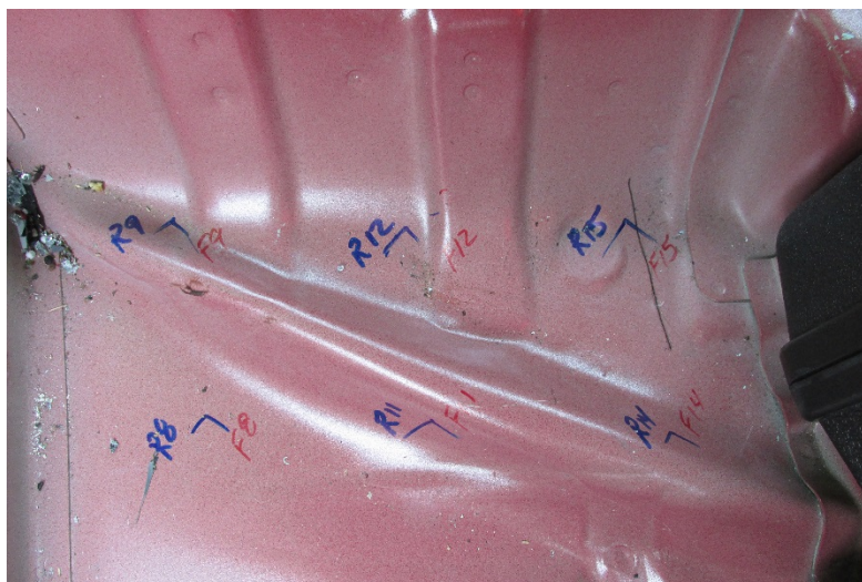
Figure 5-14 140MASH3C16-04 Kia Rio Floorboard Crease with Maximum Deformation
