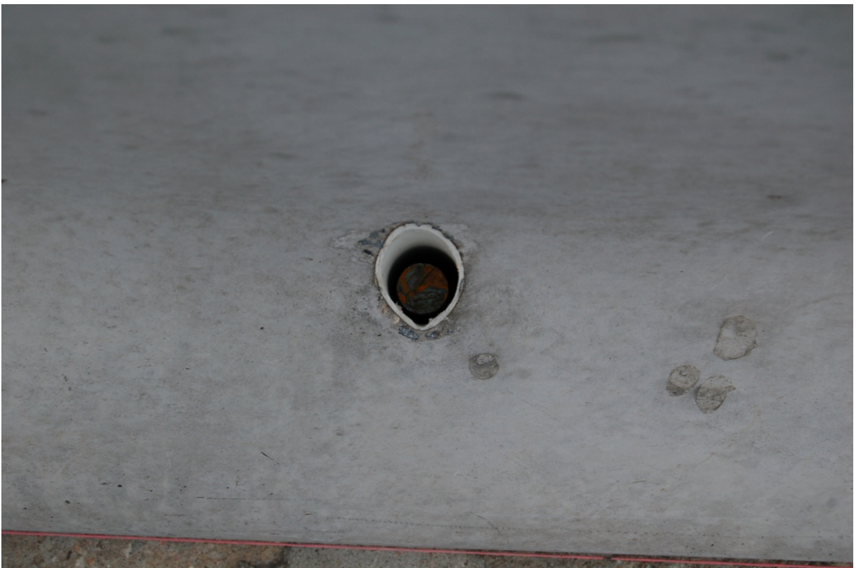
Figure 12. Temporary Concrete Barrier Section Anchor, Test No. NYTCB-5
