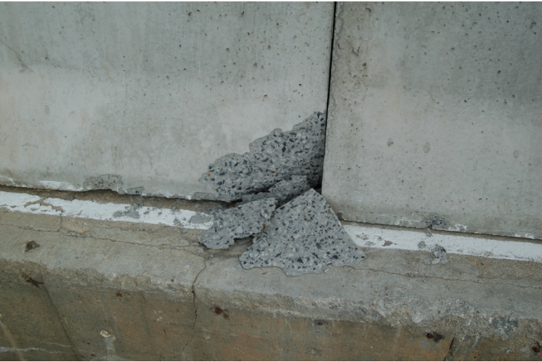
Figure 29. Barrier No. 5 Damage, Test No. NYTCB-5
