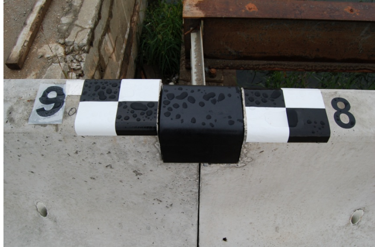
Figure 11. Temporary Concrete Barrier Sections and Connection Key, Test No. NYTCB-5
