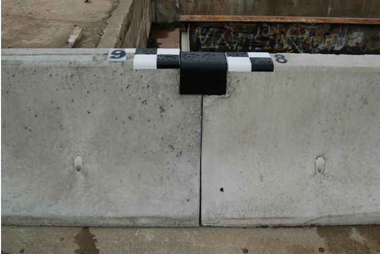
Figure 11. Temporary Concrete Barrier Sections and Connection Key, Test No. NYTCB-5
