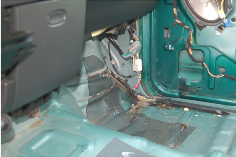
Figure 35. Occupant Compartment Deformation, Test No. NYTCB-5
