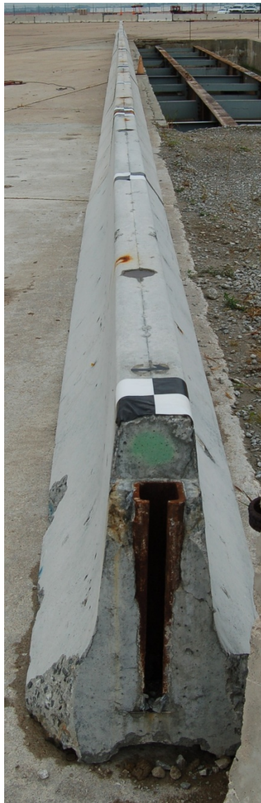
Figure 10. Pinned Temporary Concrete Barrier Test Installation, Test No. NYTCB-5
