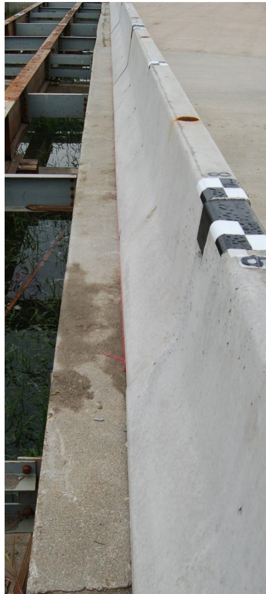
Figure 10. Pinned Temporary Concrete Barrier Test Installation, Test No. NYTCB-5
