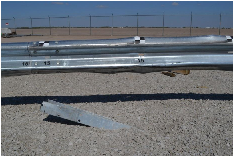
Figure 27. Post nos. 14 through 17 Damage, Test No. MGSMP-1
