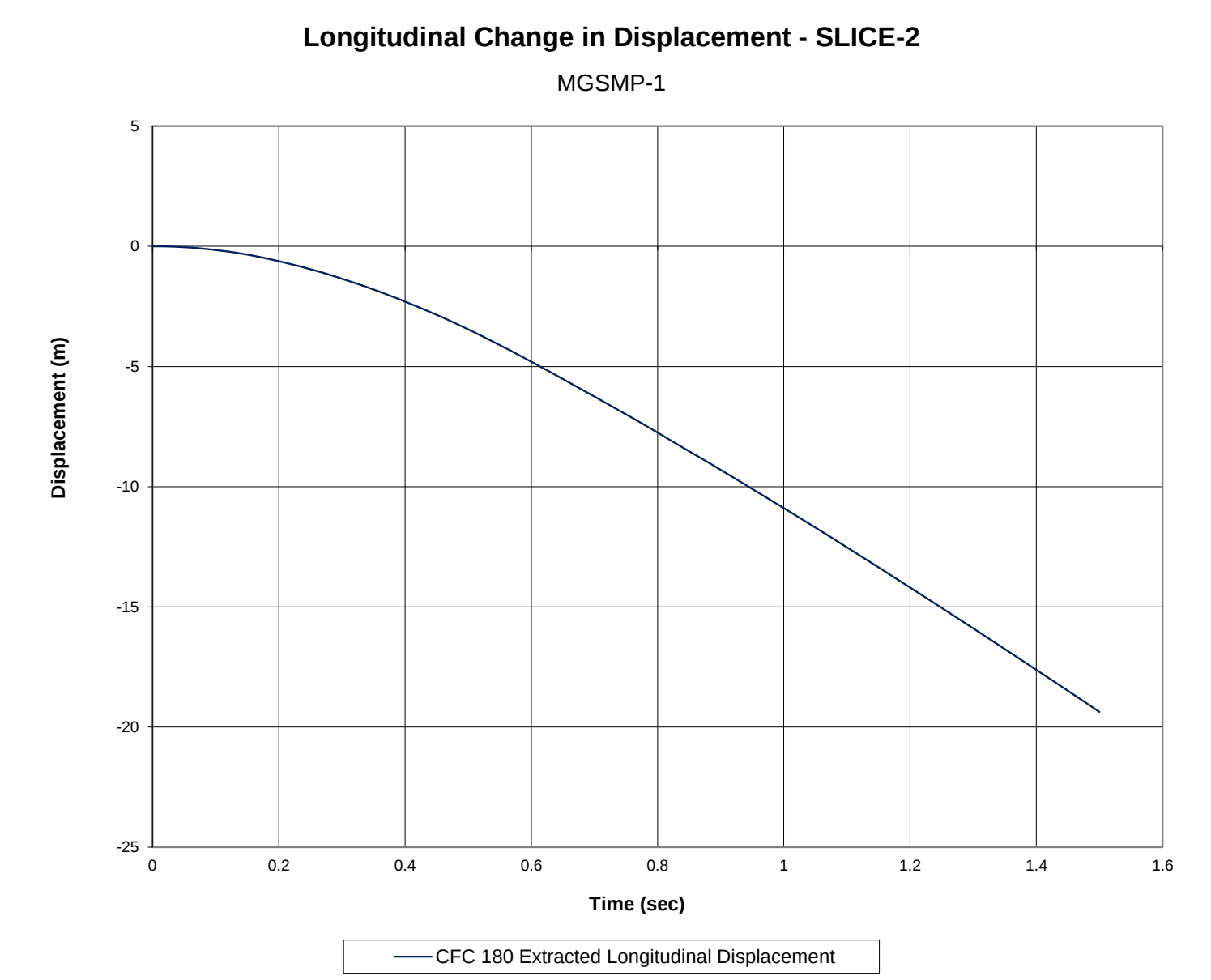
Figure E-11. Longitudinal Occupant Displacement (SLICE-2), Test No. MGSMP-1
