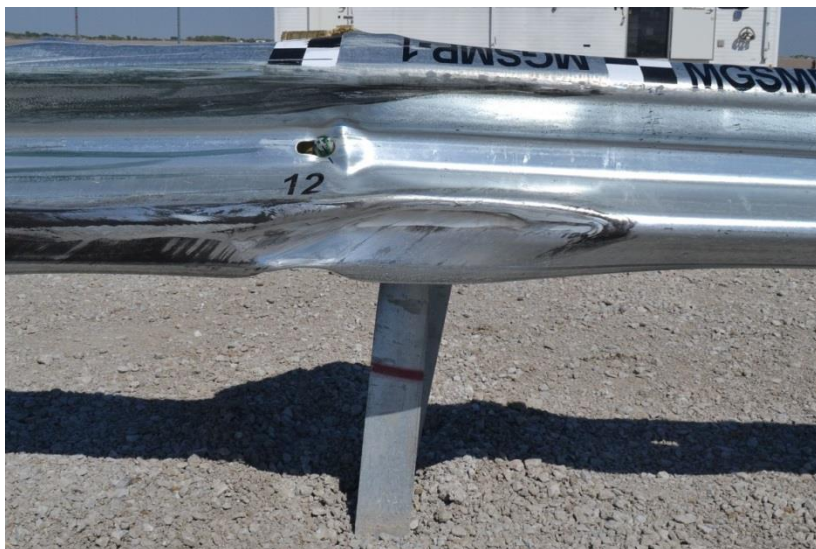
Figure 26. Post nos. 7 through 13 Damage, Test No. MGSMP-1
