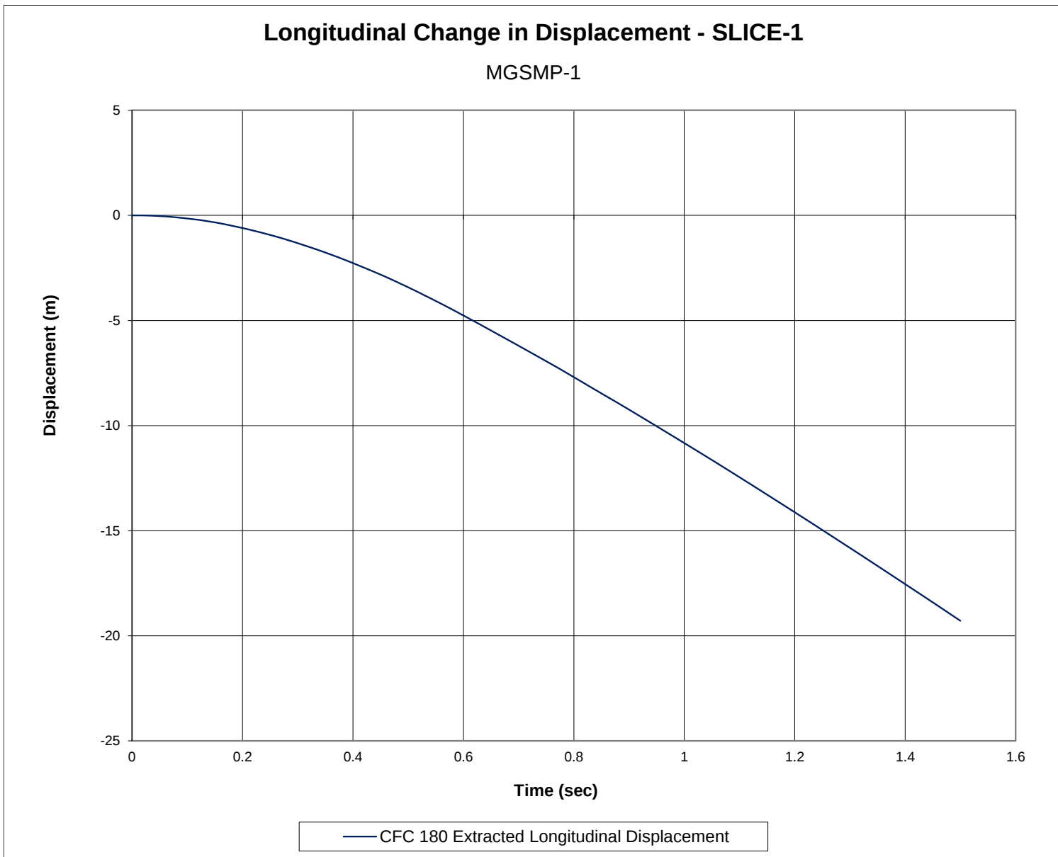
Figure E-3. Longitudinal Occupant Displacement (SLICE-1), Test No. MGSM-1
