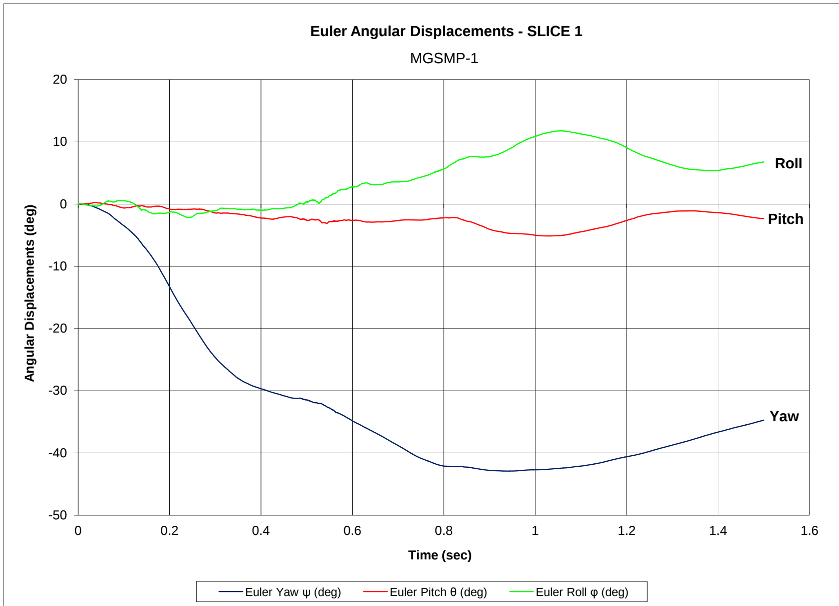
Figure E-7. Vehicle Angular Displacements (SLICE-1), Test No. MGSMP-1
