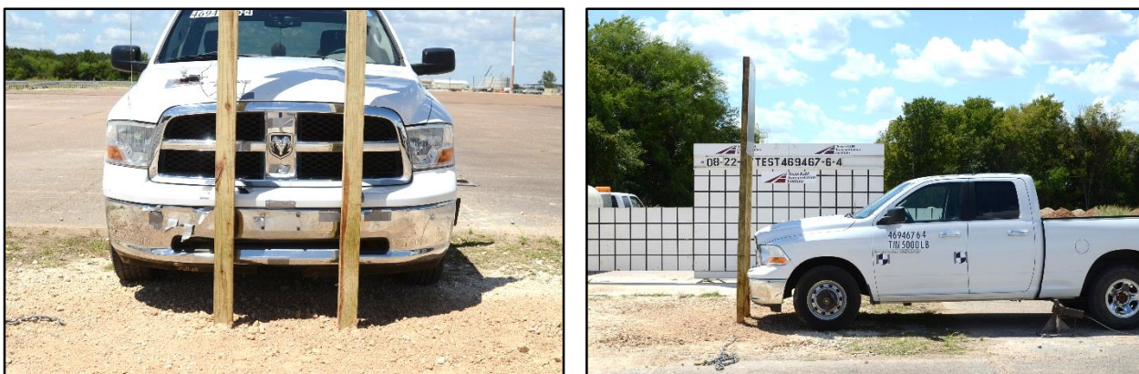
Figure 5.19. TxDOT Dual Embedded Wood Post System/Test Vehicle Geometrics for Test No. 469467-6-4.
