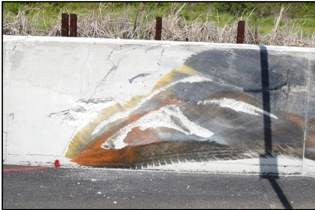
Figure 3.5. TxDOT 42-inch Tall SSCB with 1-inch ACP and Test Vehicle after Test No. 469467-3-1.
