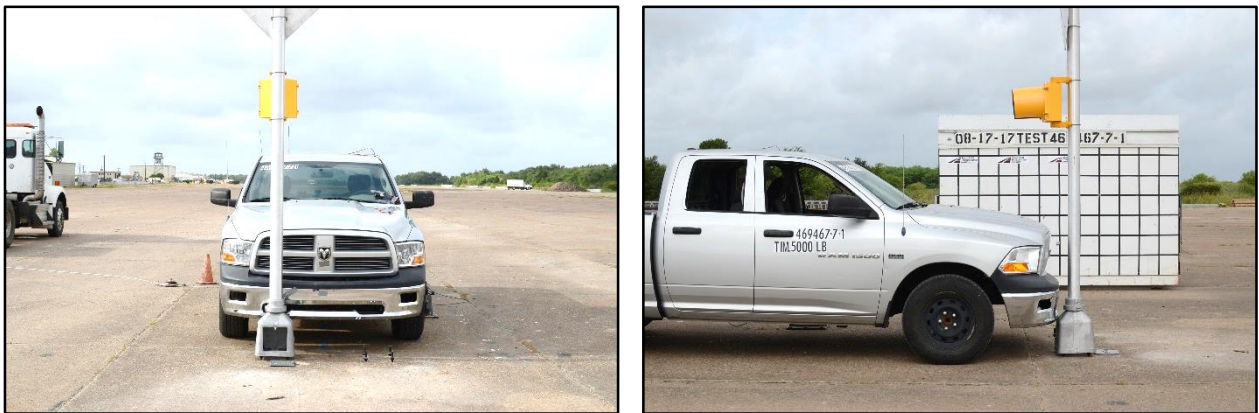
Figure 6.3. TxDOT Pedestal Pole with Beacons without Solar Assembly/Test Vehicle Geometries for Test No. 469467-7-1.
