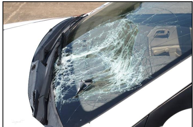
Figure 7.24. Test Vehicle Exterior Windshield Damage after Test No. 469467-8-2.
