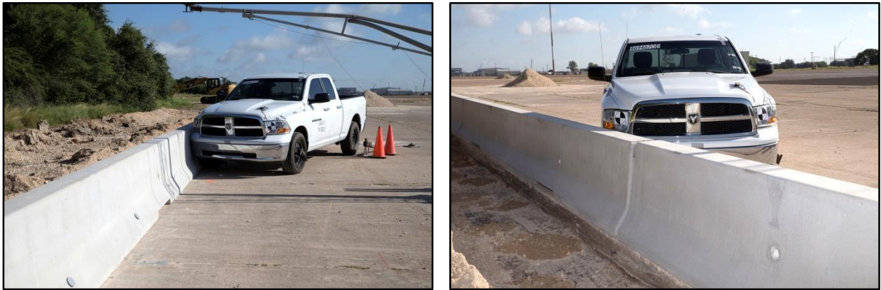
Figure 4.3. TxDOT 32-inch CSB(7)-10 Pinned to Concrete Pavement/Test Vehicle Geometries for Test No. 469467-5-1.
