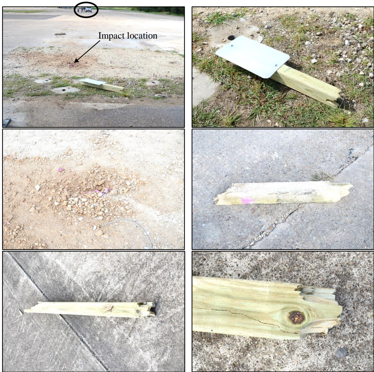
Figure 5.5. TxDOT Single Embedded Wood Post System for 0° Impact after Test No. 469467-6-1.
