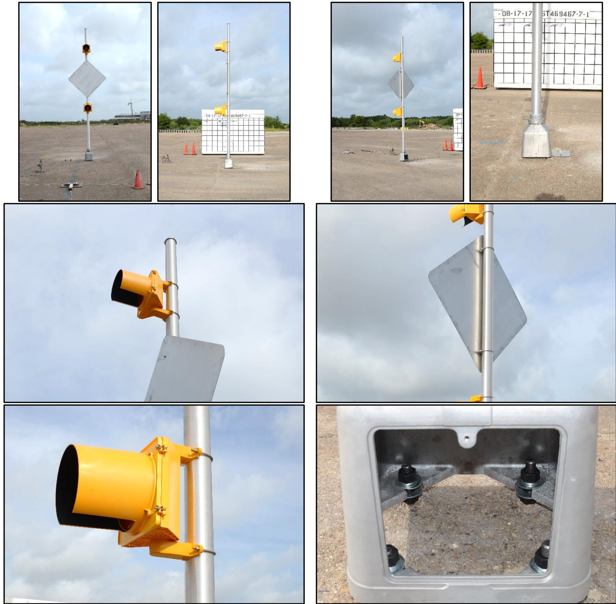
Figure 6.2. TxDOT Pedestal Pole with Beacons without Solar Assembly prior to Test No. 469467-7-1.
