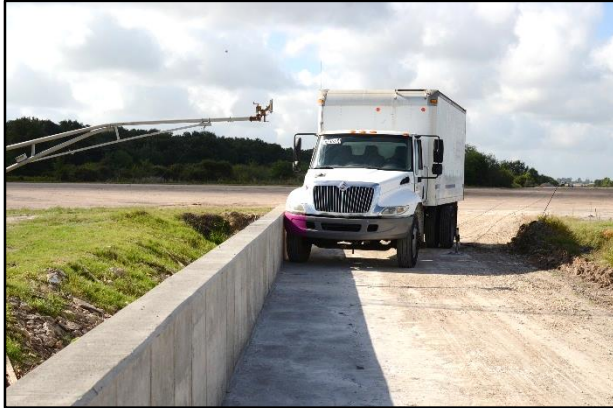
Figure 2.4. 36-inch Vertical Concrete Bridge Rail /Test Vehicle Geometrics for Test No. 469467-1-1.
