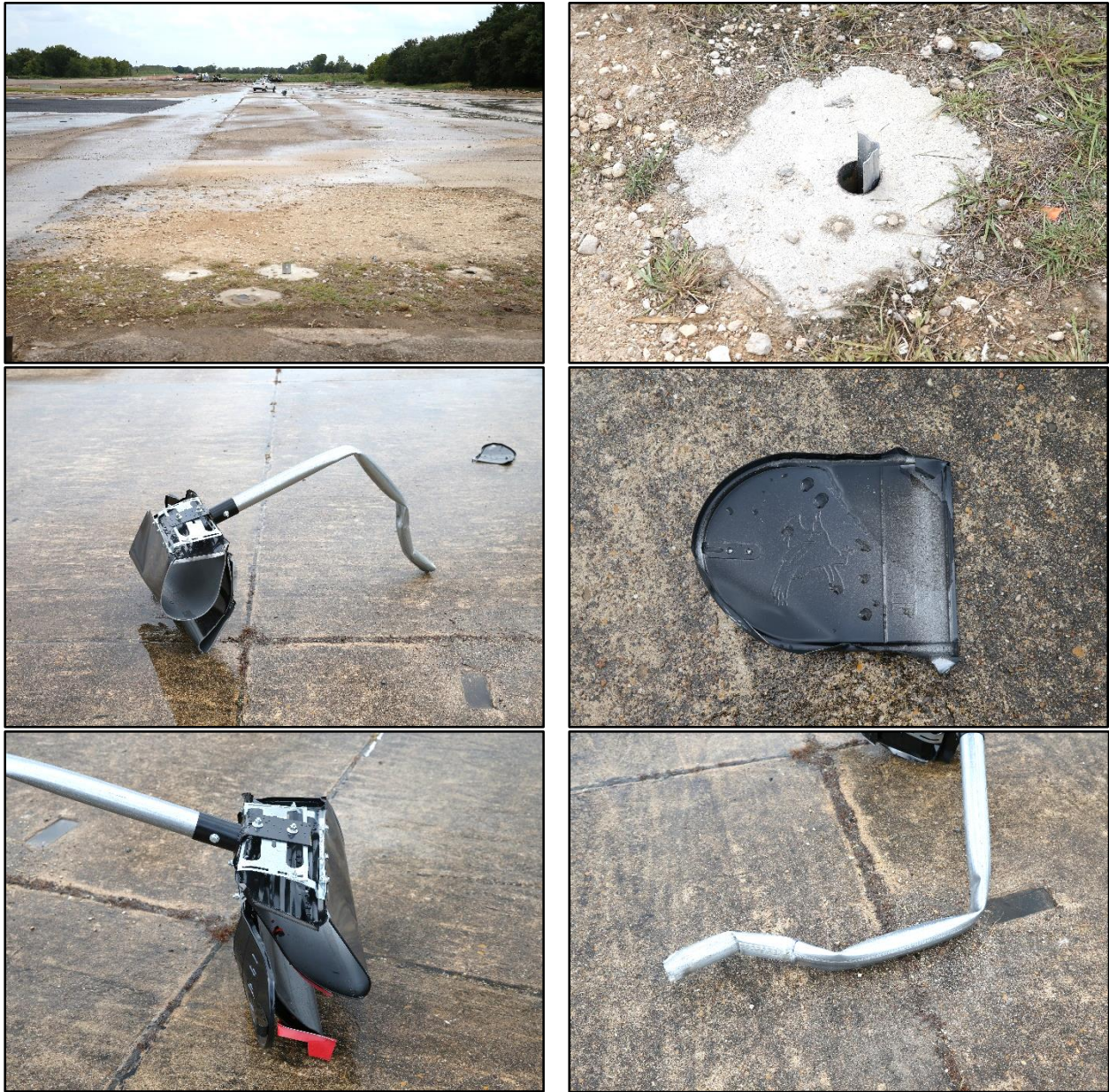
Figure 7.14. TxDOT Double Mailbox System on Thin-Walled Galvanized Tube with Type 2 Foundation after Test No. 469467-8-3.
