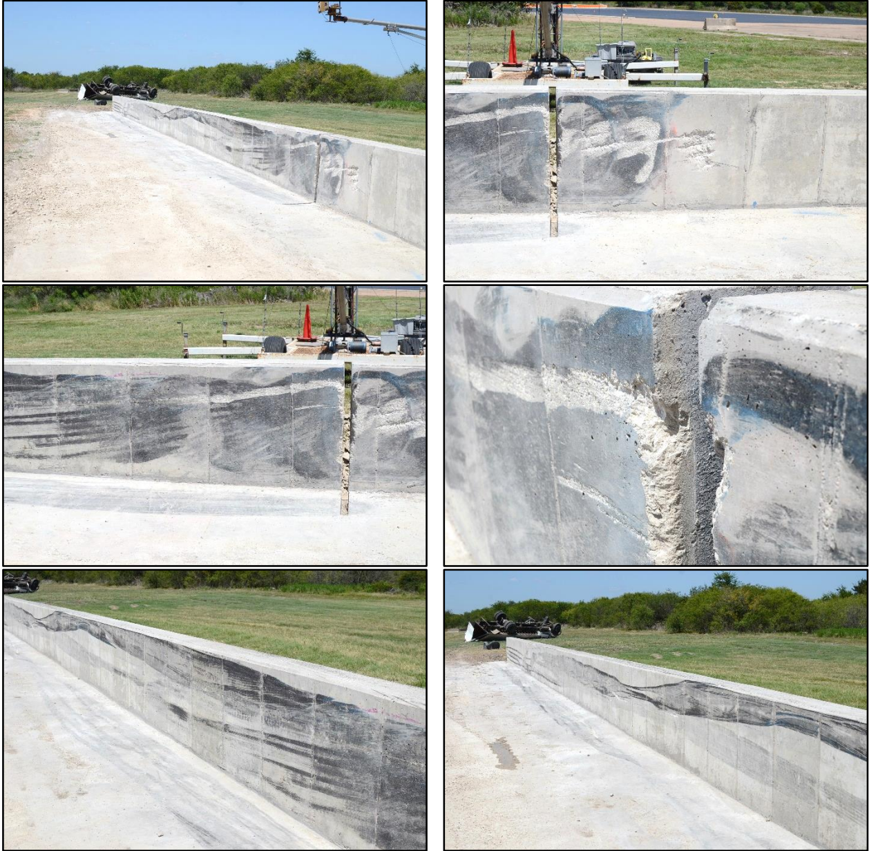
Figure 2.6. 36-inch Vertical Concrete Bridge Rail after Test No. 469467-1-1.
