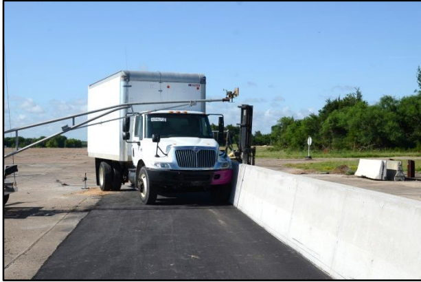
Figure 3.3. TxDOT 42-inch Tall SSCB with 1-inch ACP Overlay/Test Vehicle Geometrics for Test No. 469467-3-1.
