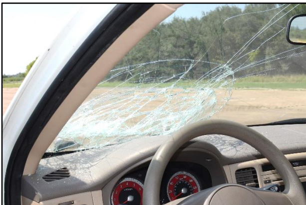
Figure 7.25. Interior Windshield Damage after Test No. 469467-8-2.
