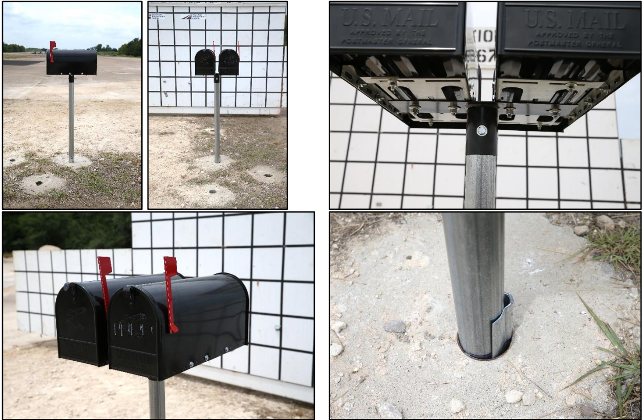
Figure 7.11. TxDOT Double Mailbox System on Thin-Walled Galvanized Tube with Type 2 Foundation prior to Testing.
