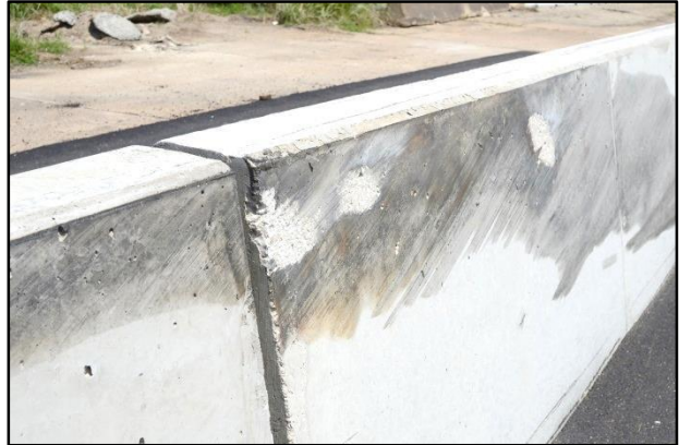
Figure 3.6. TxDOT 42-inch Tall SSCB with 1-inch ACP Overlay after Test No. 469467-3-1.
