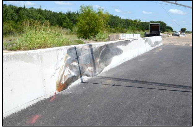
Figure 3.5. TxDOT 42-inch Tall SSCB with 1-inch ACP and Test Vehicle after Test No. 469467-3-1.
