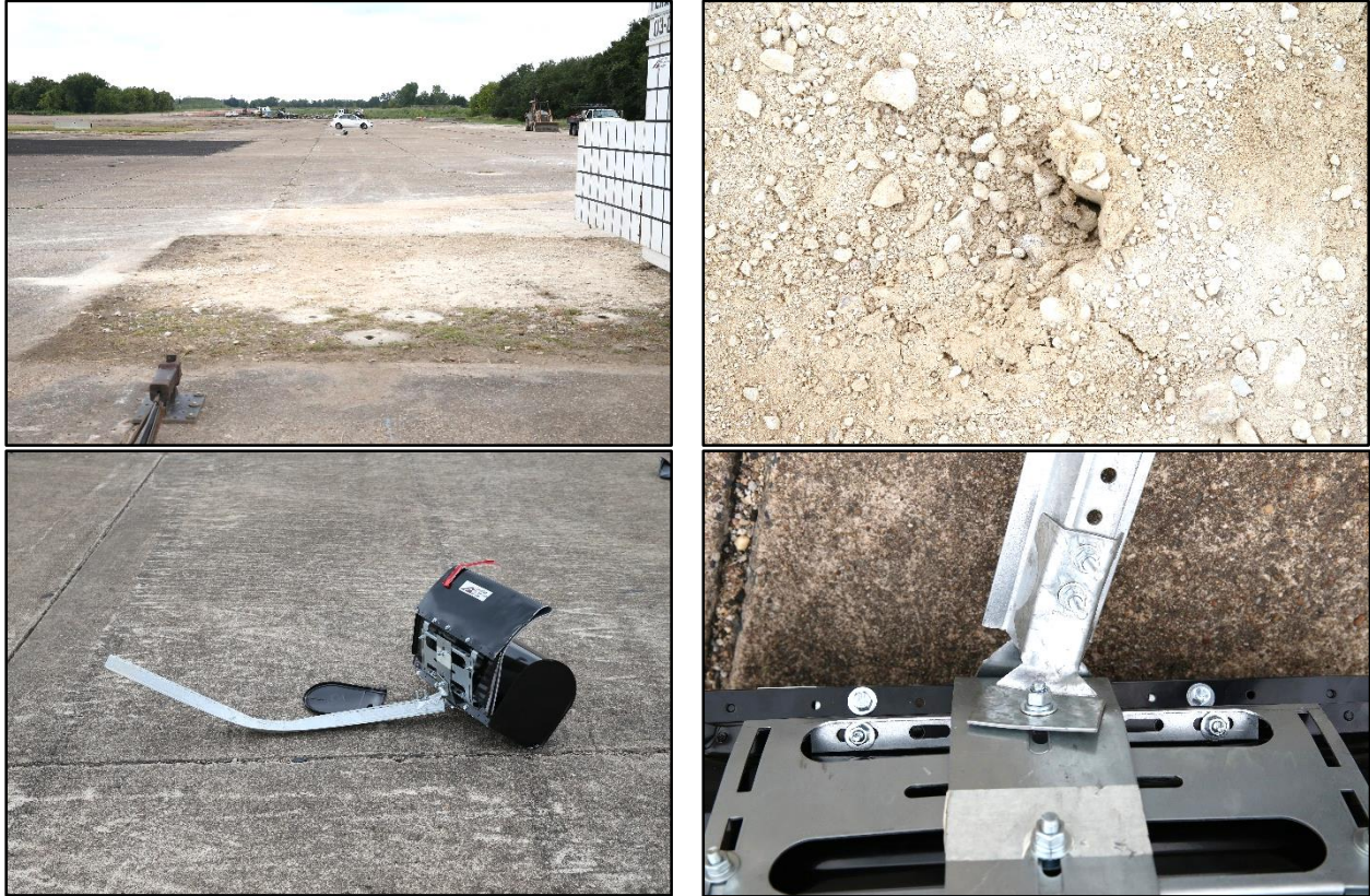
Figure 7.6. TxDOT Double Mailbox System on Winged Channel Post with Type 3 Foundation after Test No. 469467-8-4.
