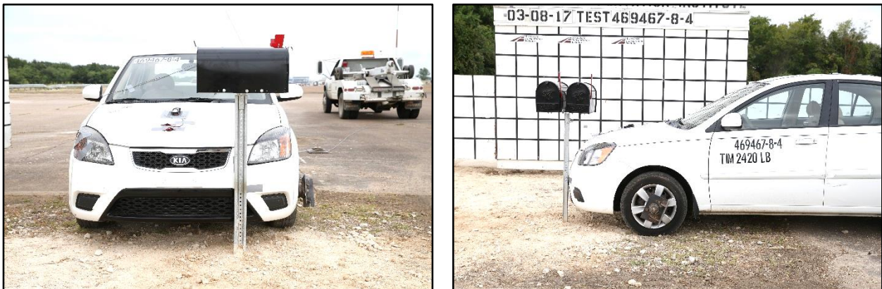
Figure 7.4. TxDOT Double Mailbox System on Winged Channel Post with Type 3 Foundation/Test Vehicle Geometrics for Test No. 469467-8-4.
