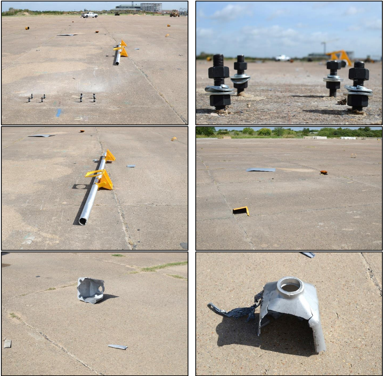
Figure 6.5. TxDOT Pedestal Pole with Beacons without Solar Assembly after Test No. 469467-7-1.
