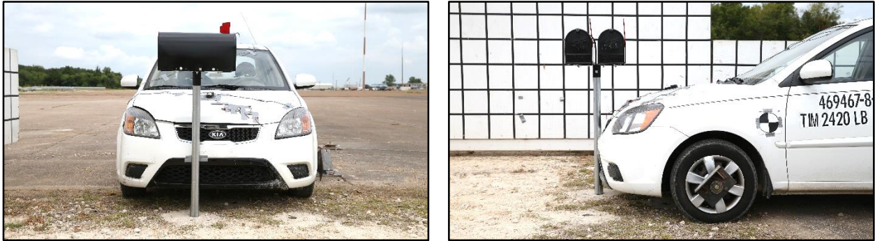
Figure 7.12. TxDOT Double Mailbox System on Thin-Walled Galvanized Tube with Type 2 Foundation/Test Vehicle Geometrics for Test No. 469467-8-3.
