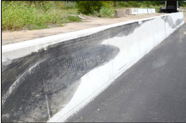
Figure 3.6. TxDOT 42-inch Tall SSCB with 1-inch ACP Overlay after Test No. 469467-3-1.
