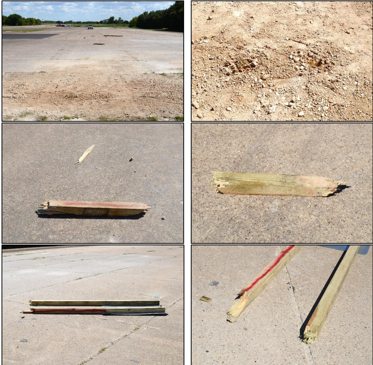
Figure 5.21. TxDOT Single Embedded Wood Post System after Test No. 469467-6-4.
