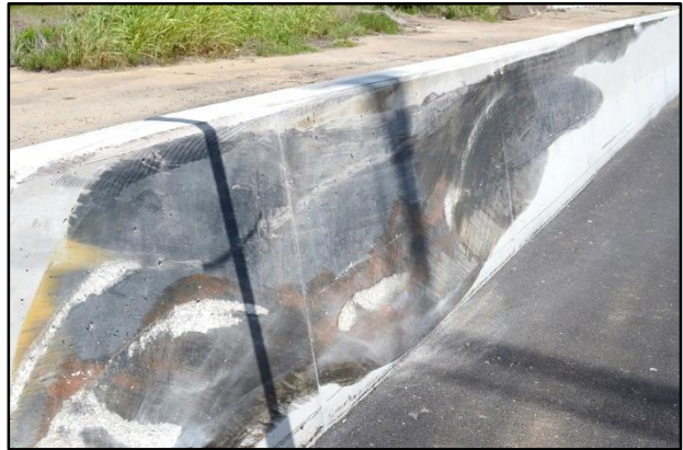
Figure 3.5. TxDOT 42-inch Tall SSCB with 1-inch ACP and Test Vehicle after Test No. 469467-3-1.
