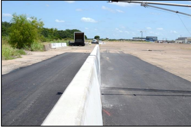
Figure 3.5. TxDOT 42-inch Tall SSCB with 1-inch ACP and Test Vehicle after Test No. 469467-3-1.
