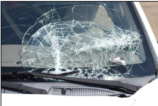
Figure 7.24. Test Vehicle Exterior Windshield Damage after Test No. 469467-8-2.
