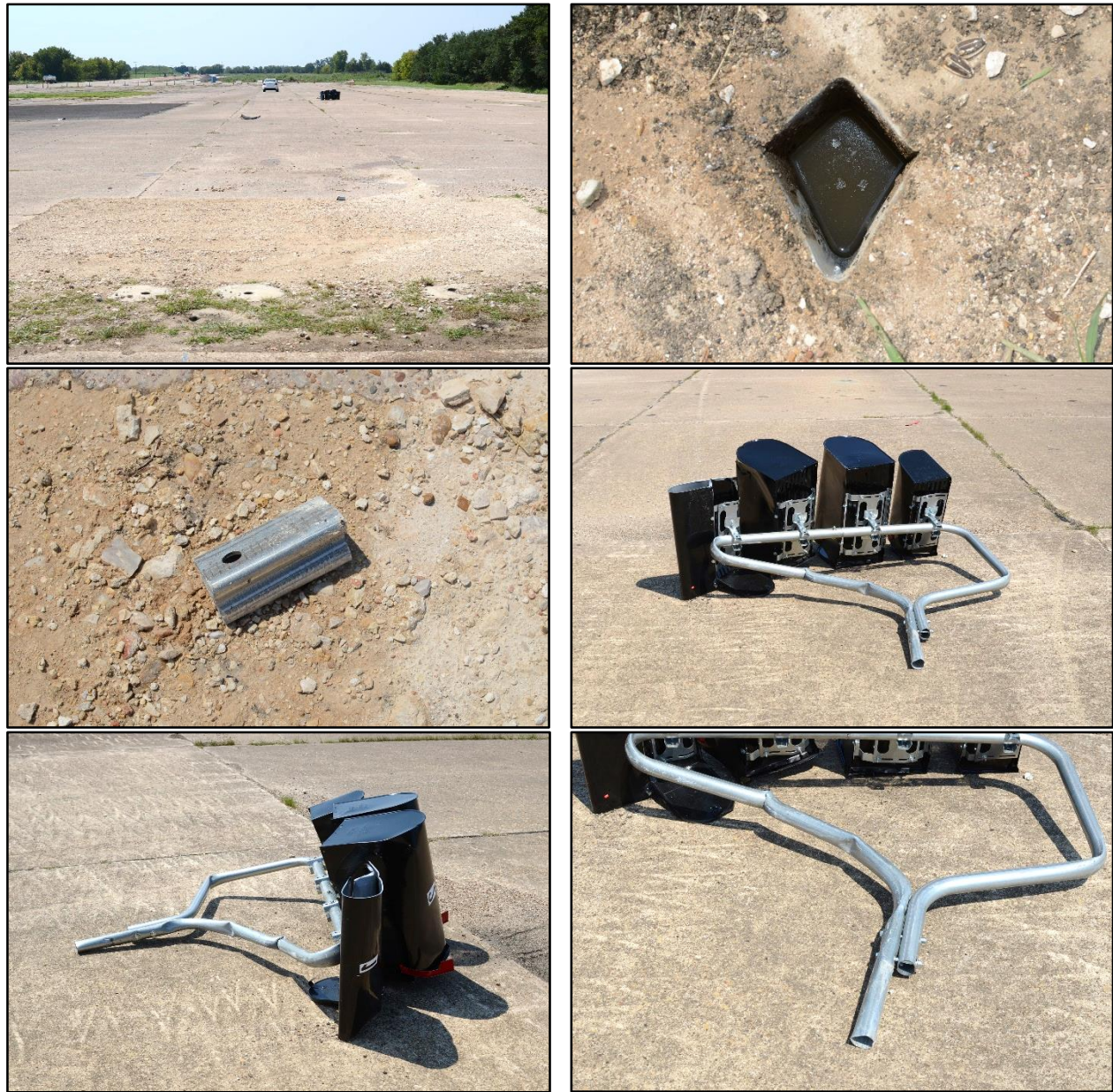
Figure 7.22. TxDOT Multiple Mailbox System on 56-inch Hanger-Type Thin-Walled Galvanized Tube with Type 1 Foundation after Test No. 469467-8-2.
