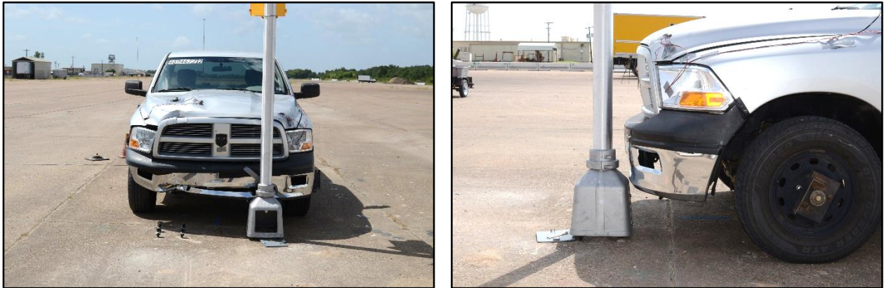
Figure 6.11. TxDOT Pedestal Pole with Beacons and Solar Assembly/Test Vehicle Geometries for Test No. 469467-7-2.
