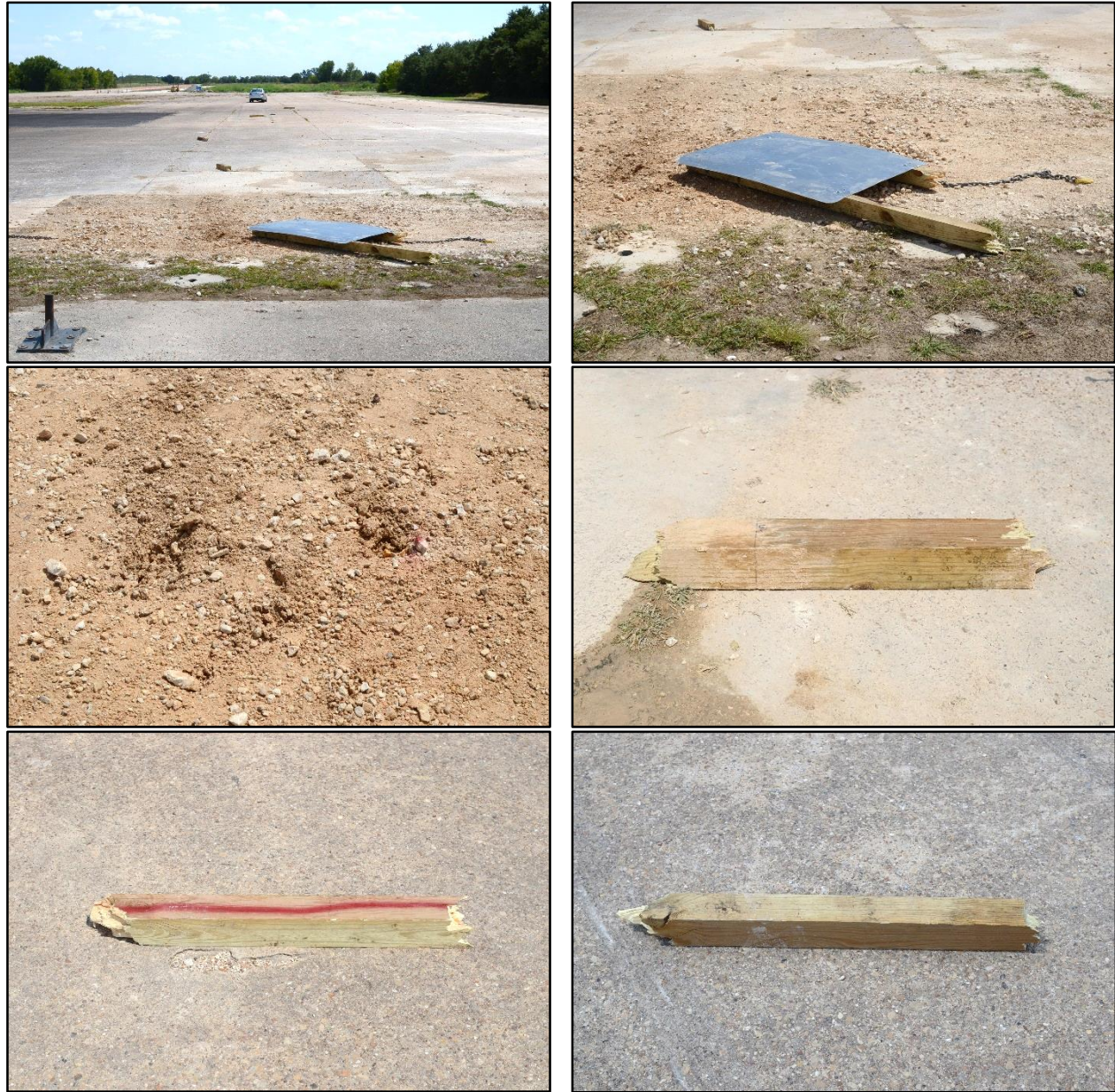
Figure 5.28. TxDOT Dual Embedded Wood Post System after Test No. 469467-6-2.
