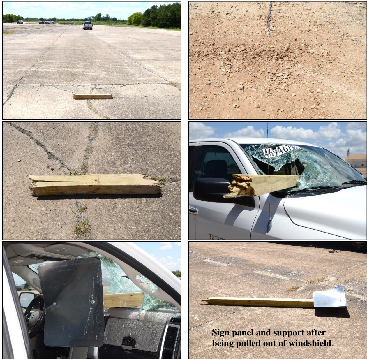
Figure 5.13. TxDOT Single Embedded Wood Post System for 90° Impact after Test No. 469467-6-3.
