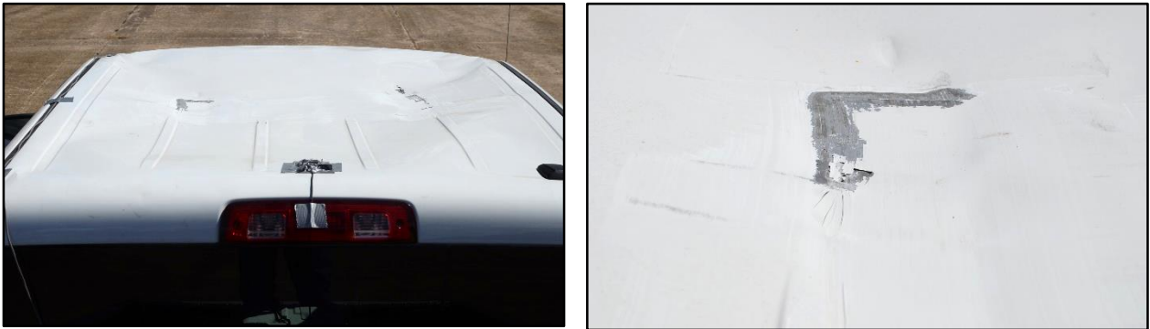
Figure 5.23. Test Vehicle Roof Damage after Test No. 469467-6-4.
