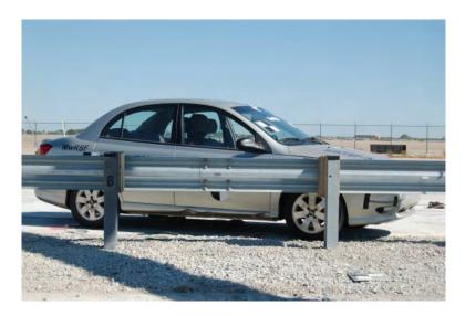
Figure 83. Impact Location. Test No. MWTSP-3
