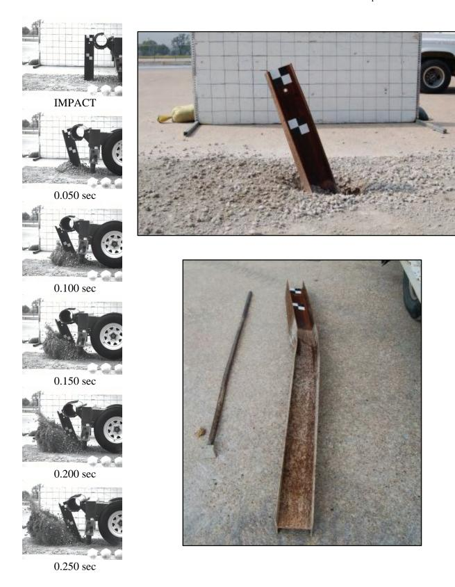
Figure 4. Time Sequential and Post-Impact Photographs, Test No. MGSATB-1
