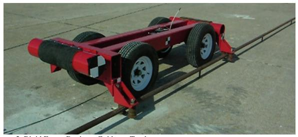
Figure 2. Rigid Frame Bogie on Guidance Track
