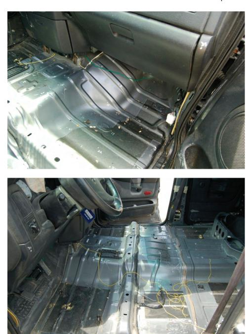
Figure 78. Occupant Compartment Damage, Test No. MWTSP-2
