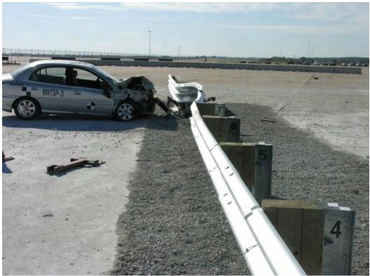
Figure 84. Vehicle Trajectory and Final Position, Test No. MWTSP-3
