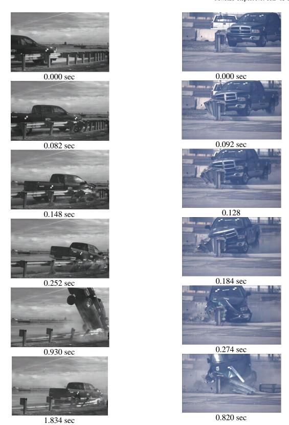
Figure 51. Additional Sequential Photographs, Test No. MWTSP-1
