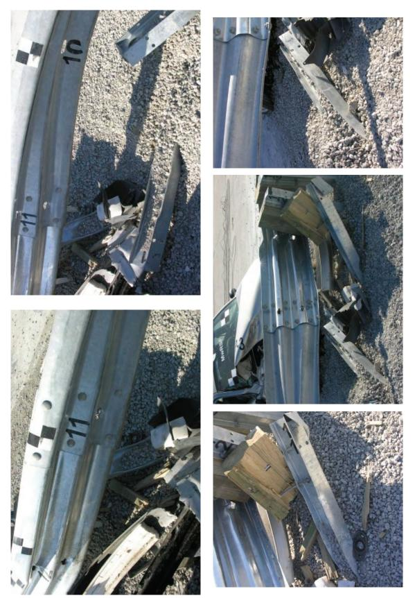
Figure 87. Posts Nos. 10 and 11 Damage, Test No. MWTSP-3
