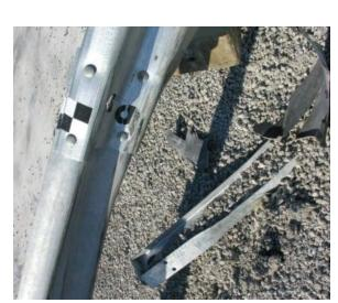
Figure 86. Posts Nos. 7 through 9 Damage, Test No. MWTSP-3
