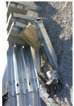
Figure 88. Post Nos. 12 through 14 Damage, Test No. MWTSP-3
