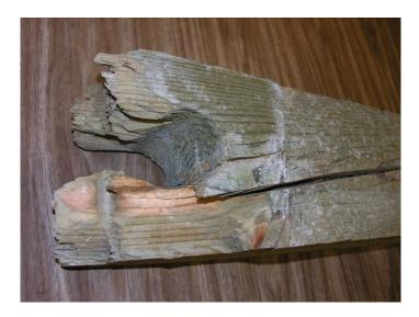
Figure 61. Anchorage Post No. 1 Damage, Test No. MWTSP-1
