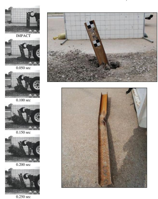
Figure 6. Time Sequential and Post-Impact Photographs, Test No. MGSATB-2
