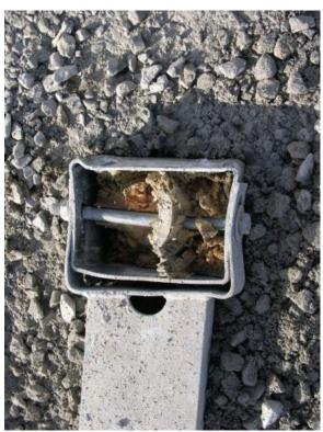
Figure 60. Upstream Anchorage Damage, Test No. MWTSP-1
