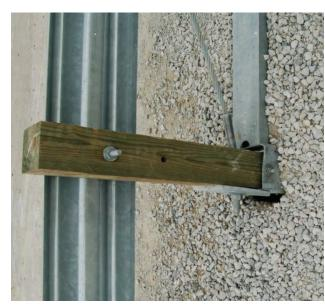
Figure 71. Upstream Anchorage Damage, Test No. MWTSP-2
