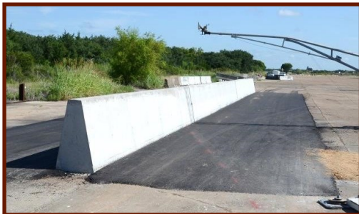
TxDOT 42" SSCB with 1" ACP prior to testing
