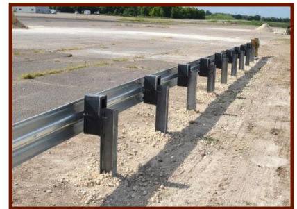
28" W-Beam System with Raised Composite Blockouts prior to Testing
