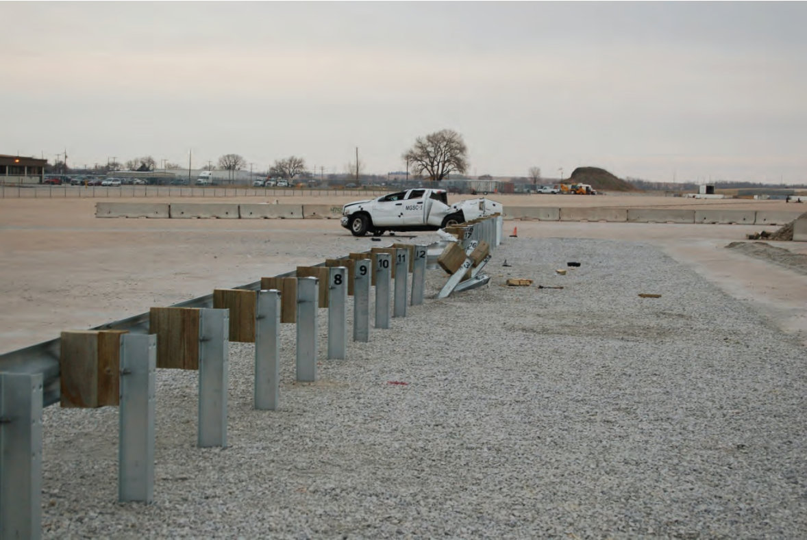
Figure 26. Vehicle Final Position and Trajectory Marks, Test No. MGSC-5
