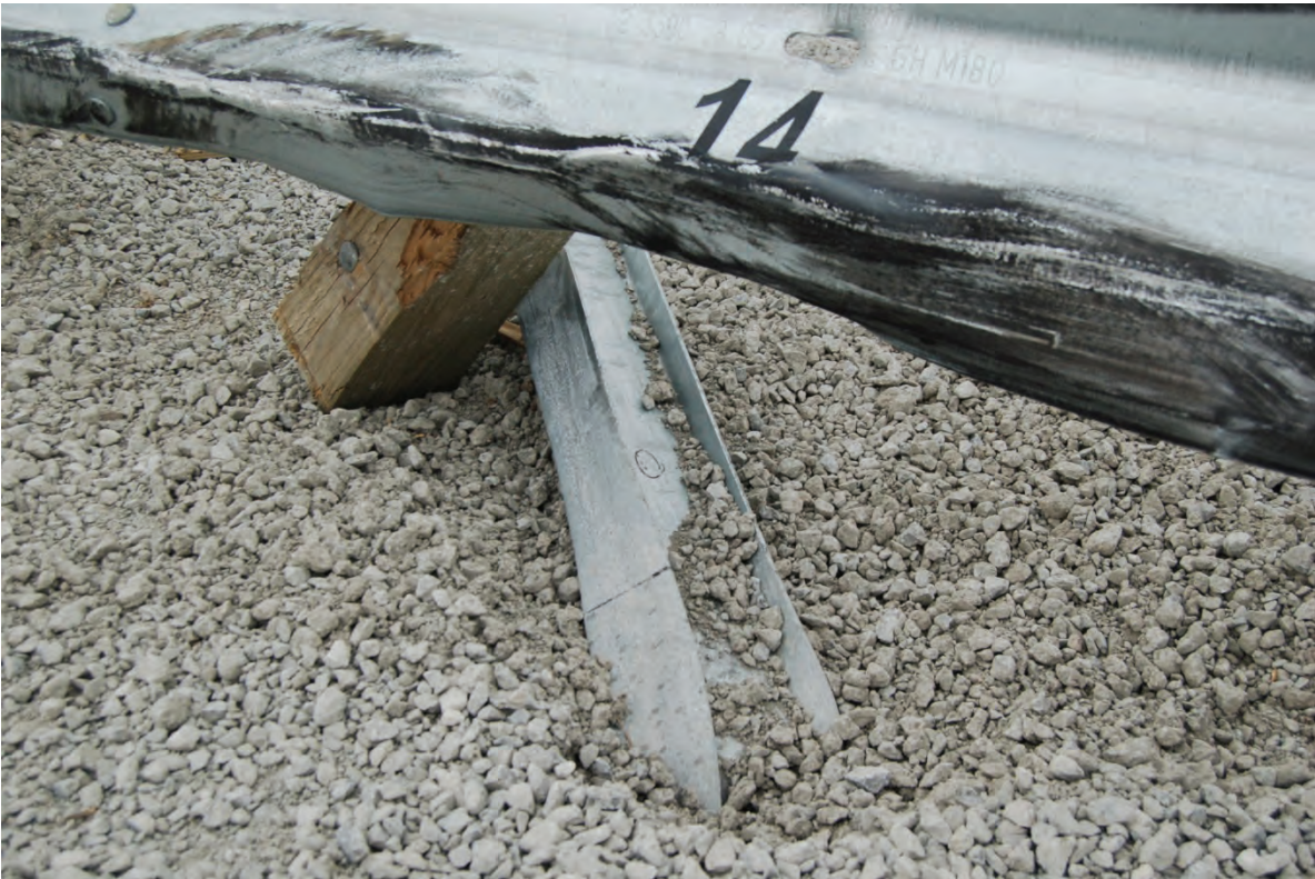
Figure 34. Post Nos. 13 and 14 Damage, Test No. MGSC-5
