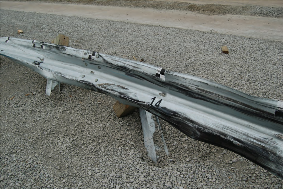
Figure 30. Rail Damage, Post Nos. 14 and 15, Test No. MGSC-5
