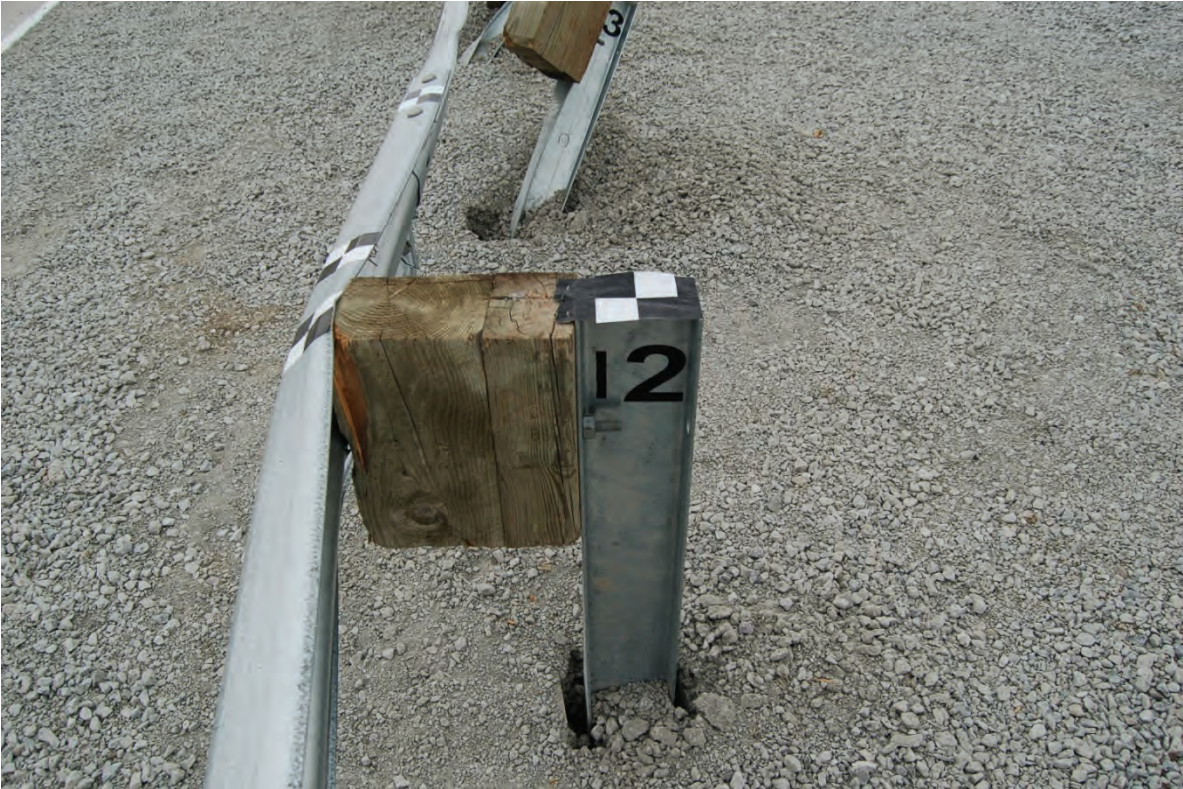
Figure 33. Post Nos. 11 and 12 Damage, Test No. MGSC-5
