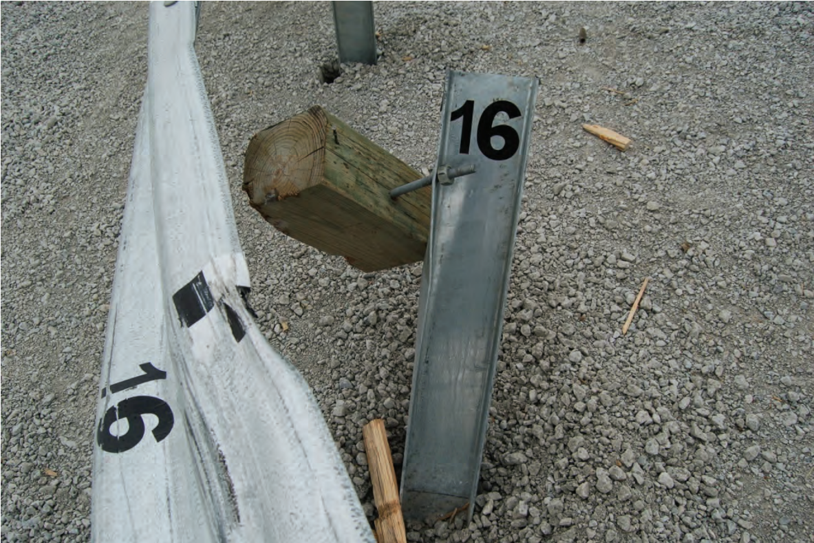
Figure 35. Post Nos. 15 and 16 Damage, Test No. MGSC-5
