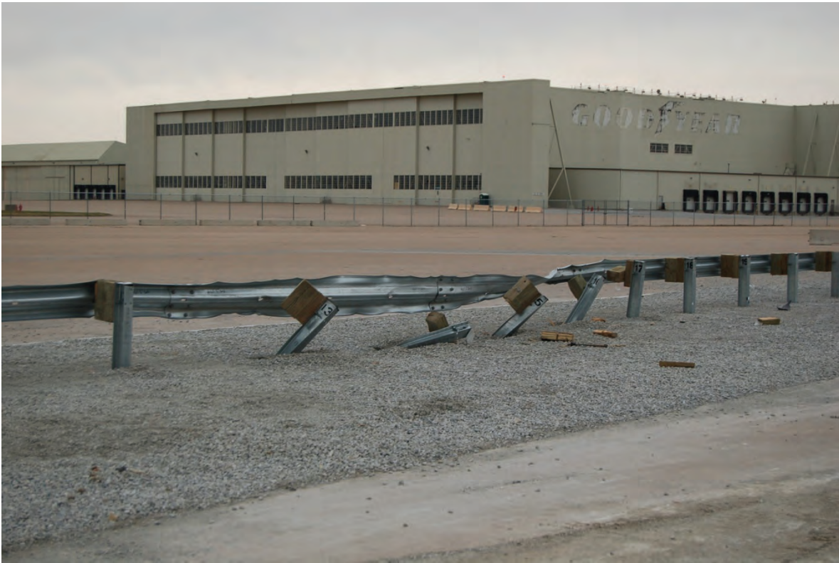
Figure 27. System Damage, Test No. MGSC-5
