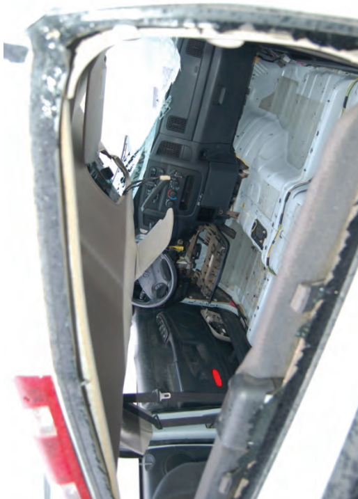
Figure 43. Occupant Compartment Damage, Test No. MGSC-5
