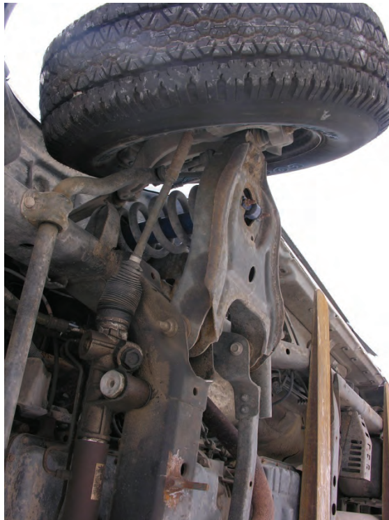
Figure 42. Undercarriage Damage, Test No. MGSC-5
