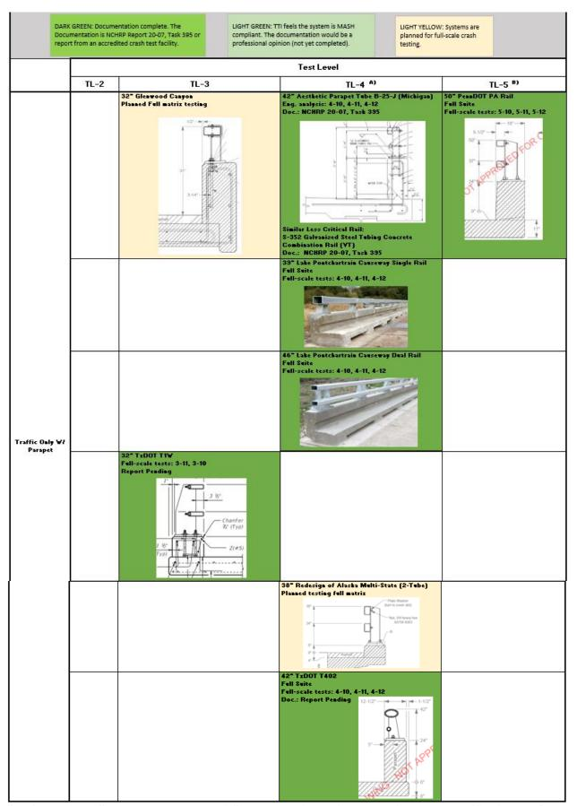
MASH Compliant Systems or under MASH Evaluation: Concrete & Metal Traffic Only w/ Parapet
