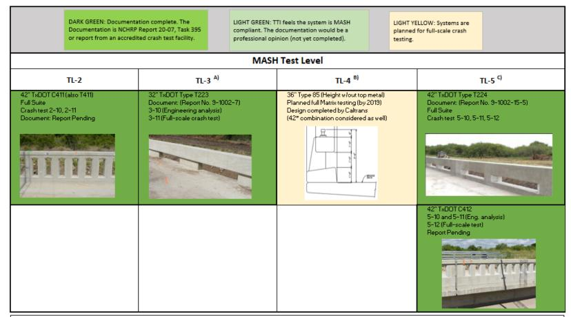
Evaluation for Post-and-Beam concrete system is individual, considering that each system is characterirized by specific geometrics (opening sizes ), which affect stability of the impacting vehicles.
