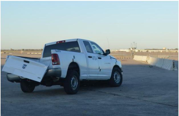
Figure 29. Vehicle Final Position and Trajectory Marks, Test No. NJPCB-4
