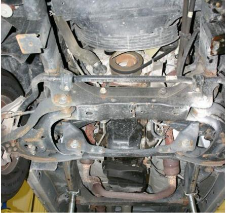
Figure 41. Undercarriage Damage, Test No. NJPCB-4
