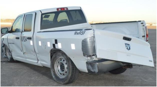
Figure 39. Vehicle Windshield, Quarter Panel, and Tailgate Damage, Test No. NJPCB-4
