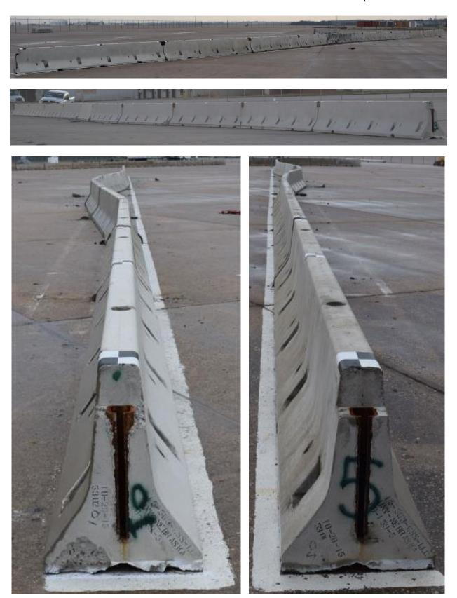
Figure 30. System Damage – Front, Back, Upstream, and Downstream End, Test No. NJPCB-4
