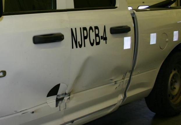
Figure 38. Vehicle Damage, Test No. NJPCB-4
