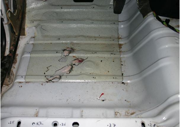
Figure 40. Occupant Compartment Deformation, Test No. NJPCB-4
