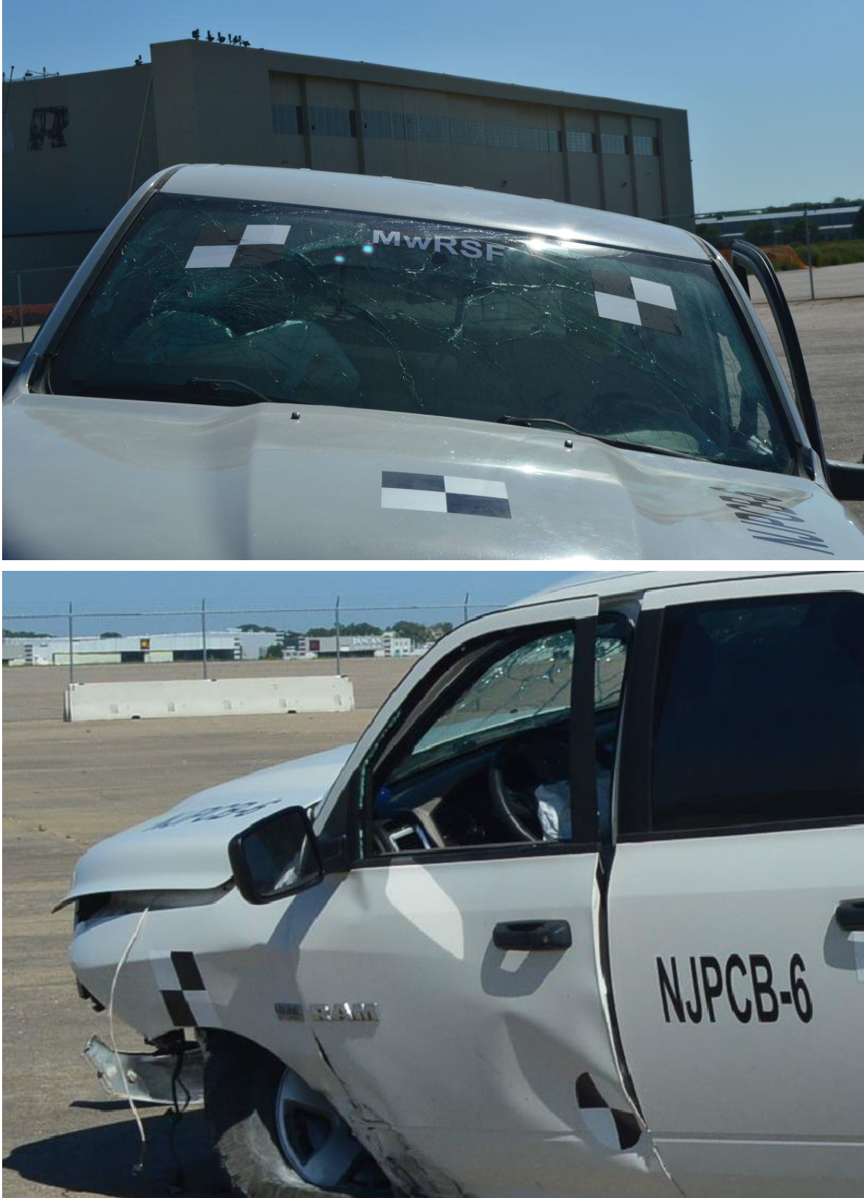
Figure 42. Vehicle Windshield and Side Window Damage, Test No. NJPCB-6
