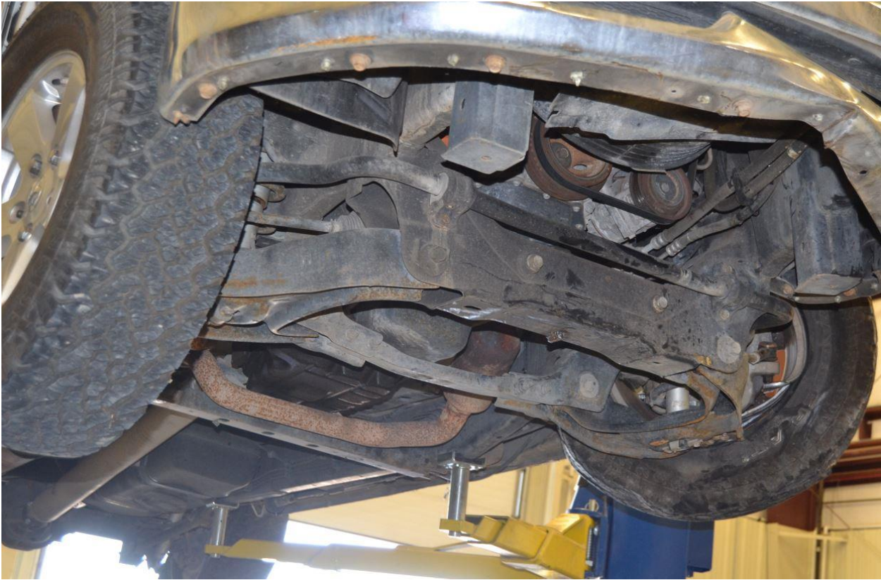
Figure 44. Undercarriage Damage, Test No. NJPCB-6
