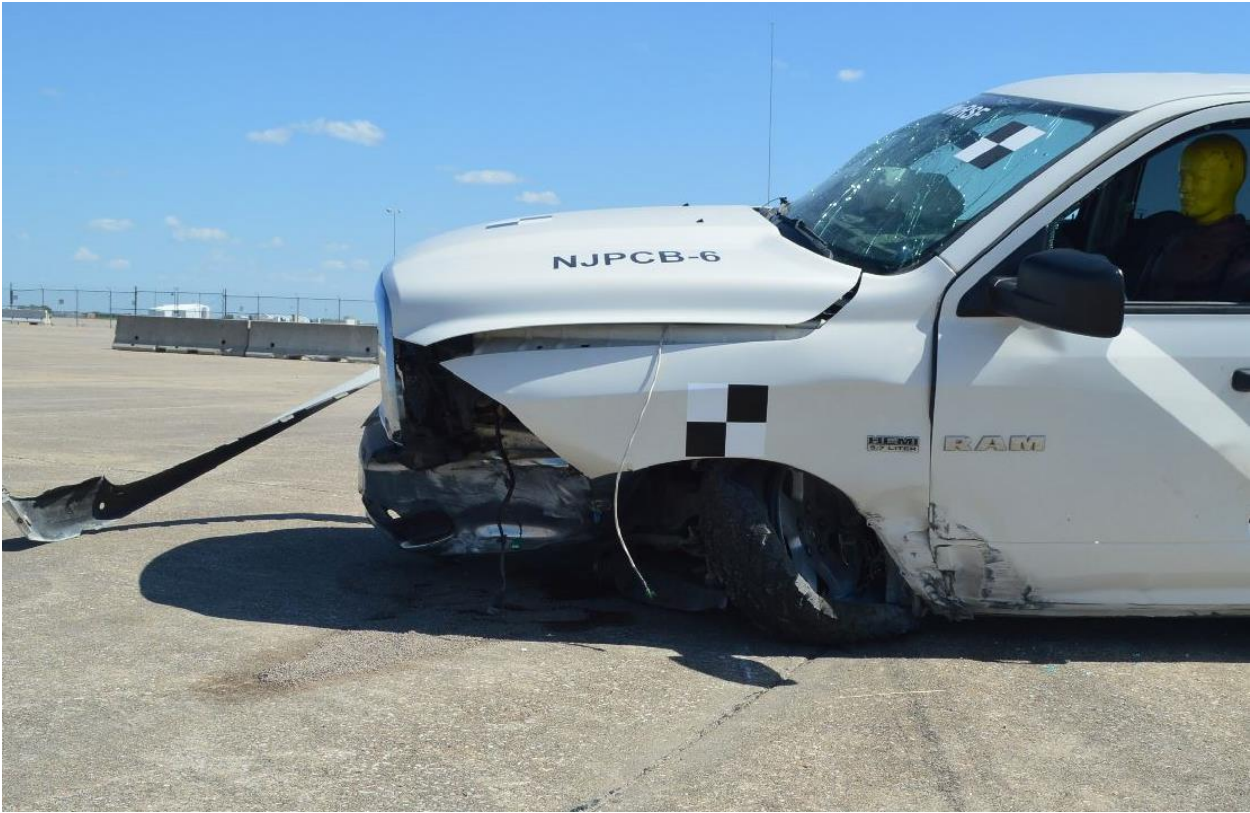
Figure 41. Vehicle Damage on Impact Side, Test No. NJPCB-6
