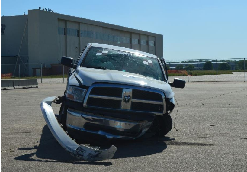
Figure 40. Vehicle Damage, Test No. NJPCB-6
