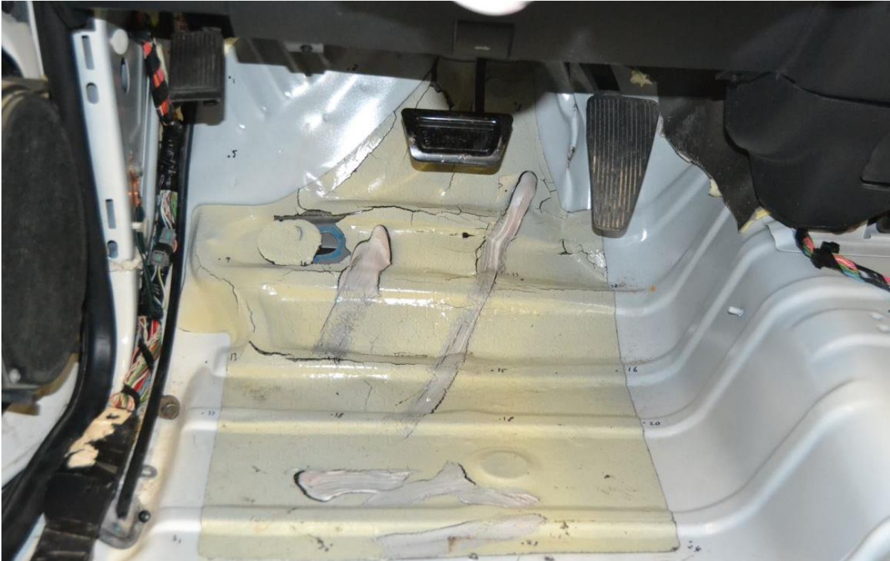
Figure 43. Occupant Compartment Deformation, Test No. NJPCB-6
