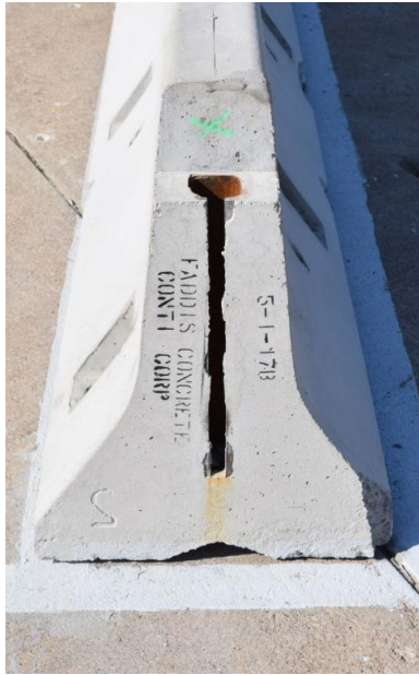
Figure 16. PCB Connection Key and Connection Socket, Test No. NJPCB-6
