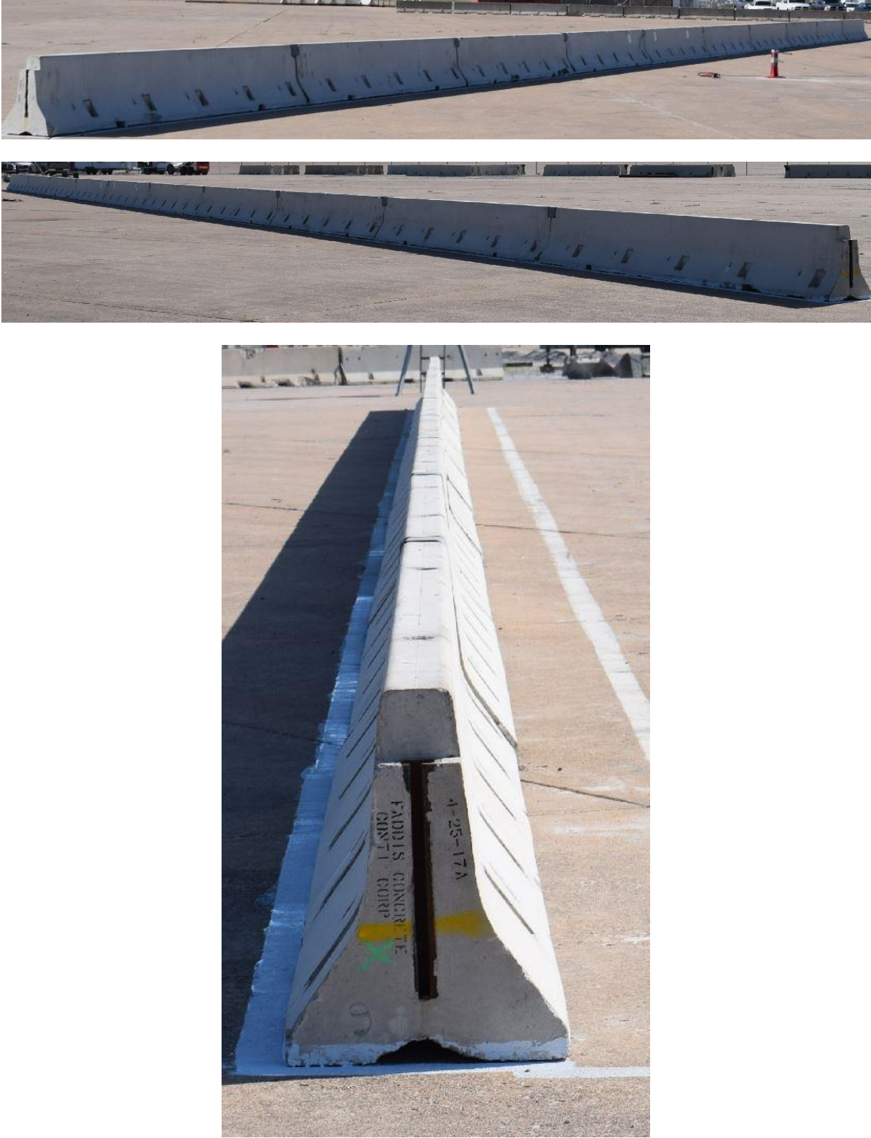
Figure 15. NJDOT PCB with Back-Side Pinned Configuration and Grouted Toes Test Installation, Test No. NJPCB-6
