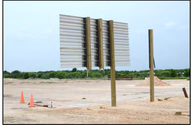
Figure 4.8. Direct Embedded Wood Support Temporary Guide Sign System after Test No. 467823-2.
