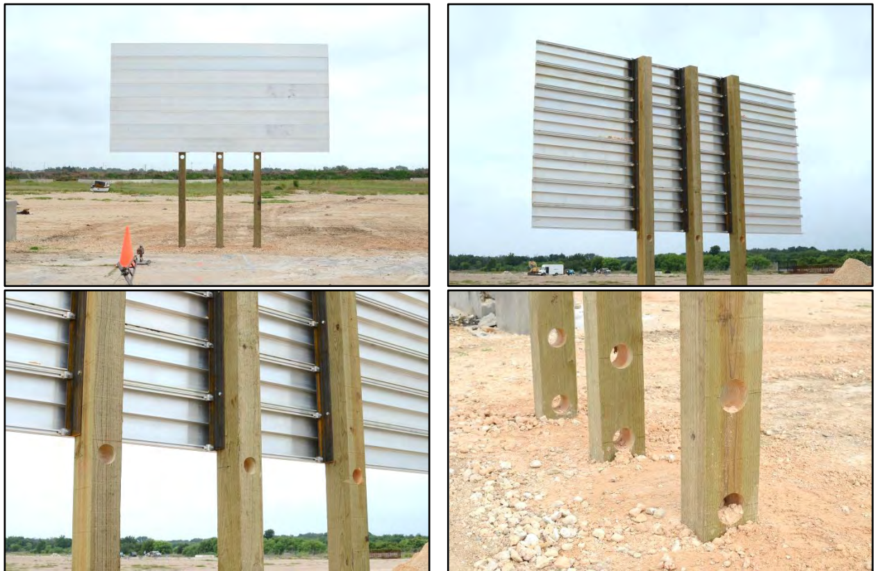
Figure 4.2. Direct Embedded Wood Support Temporary Guide Sign System before Test Nos. 467823-1 and 467823-2.
