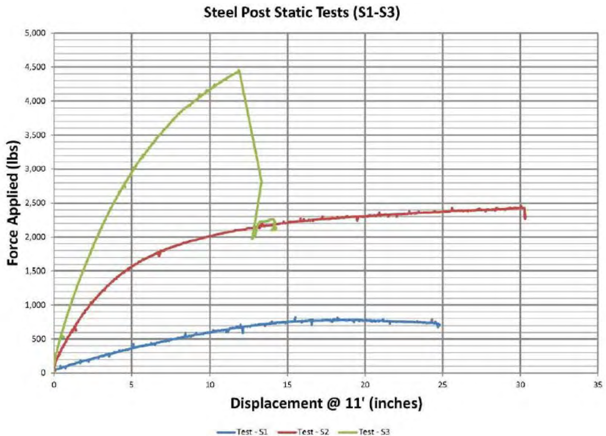
Figure 5.1. Static Test Results for S3x5.7 (Test S1), W6x9 (Test S2), and W8x18 (Test S3).
