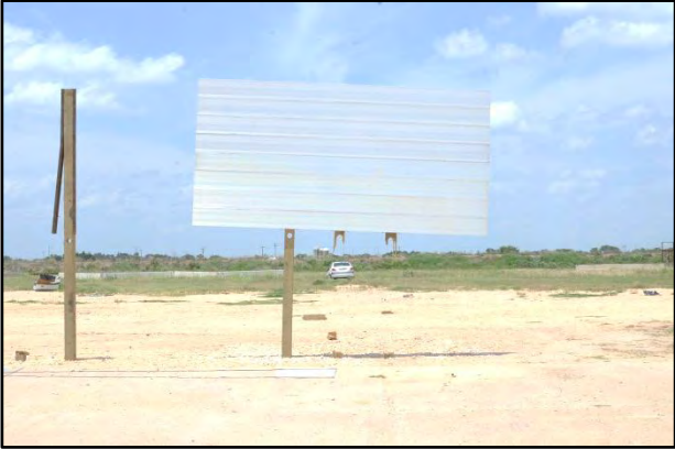
Figure 4.8. Direct Embedded Wood Support Temporary Guide Sign System after Test No. 467823-2.
