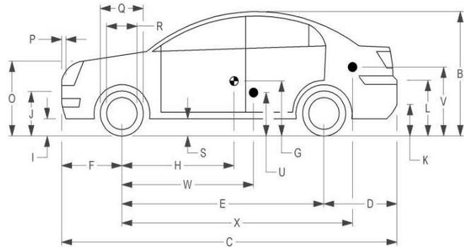
**Table C.2. Exterior Crush Measurements for Test No. 608431-01-2.**
