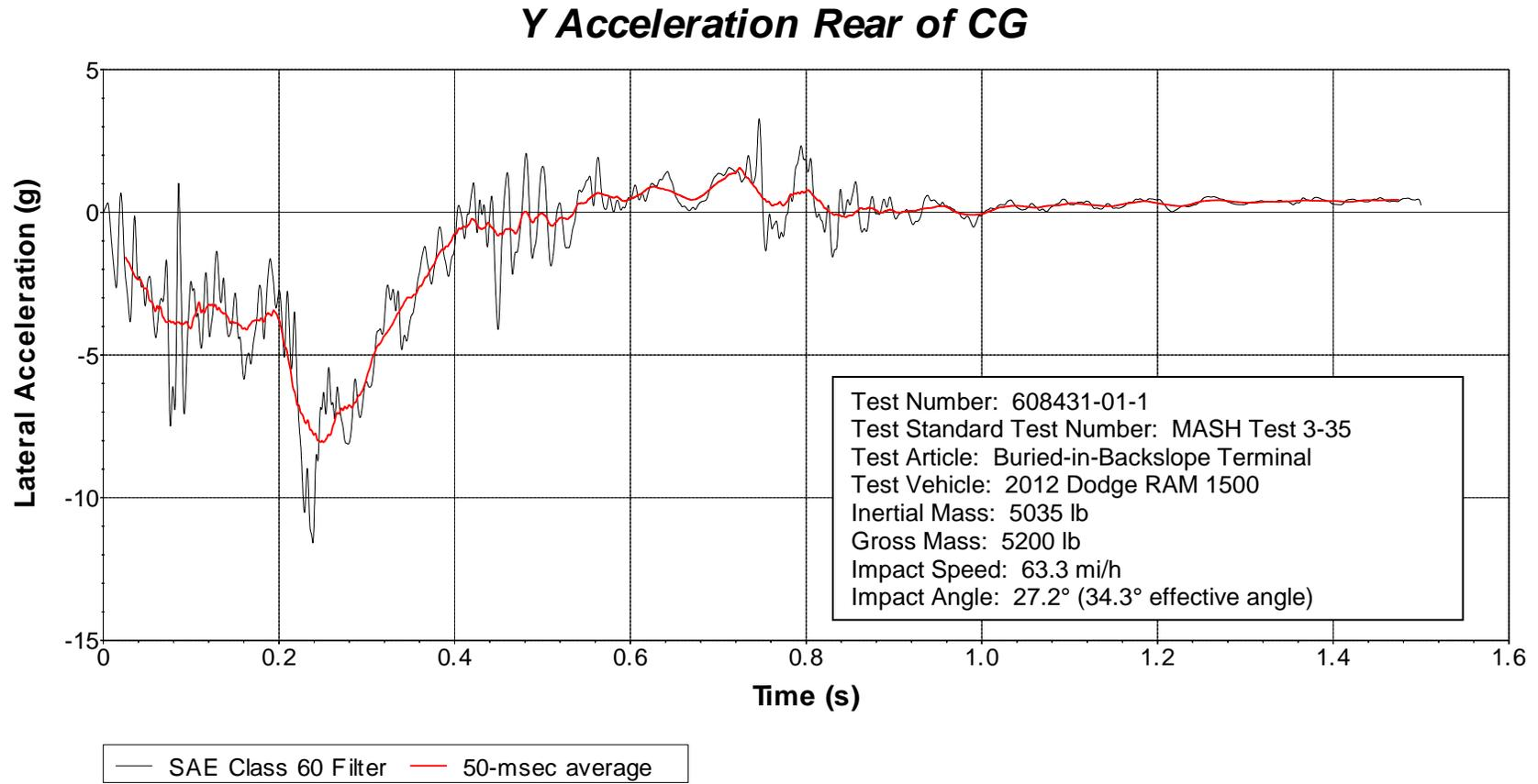
**Figure D.8. Vehicle Lateral Accelerometer Trace for Test No. 608431-01-1
