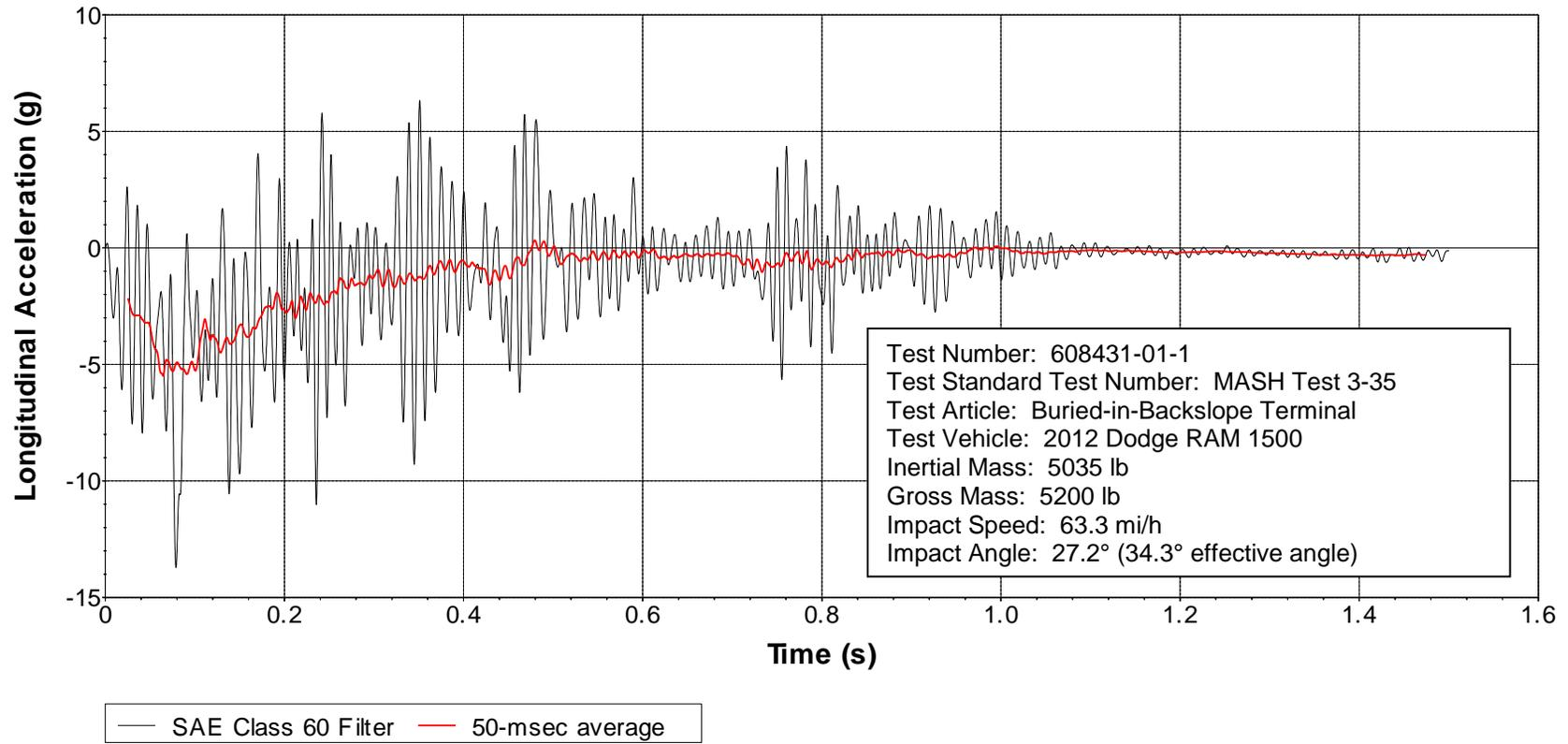
**Figure D.7. Vehicle Longitudinal Accelerometer Trace for Test No. 608431-01-1 (Accelerometer Located Rear of Center of Gravity).**
