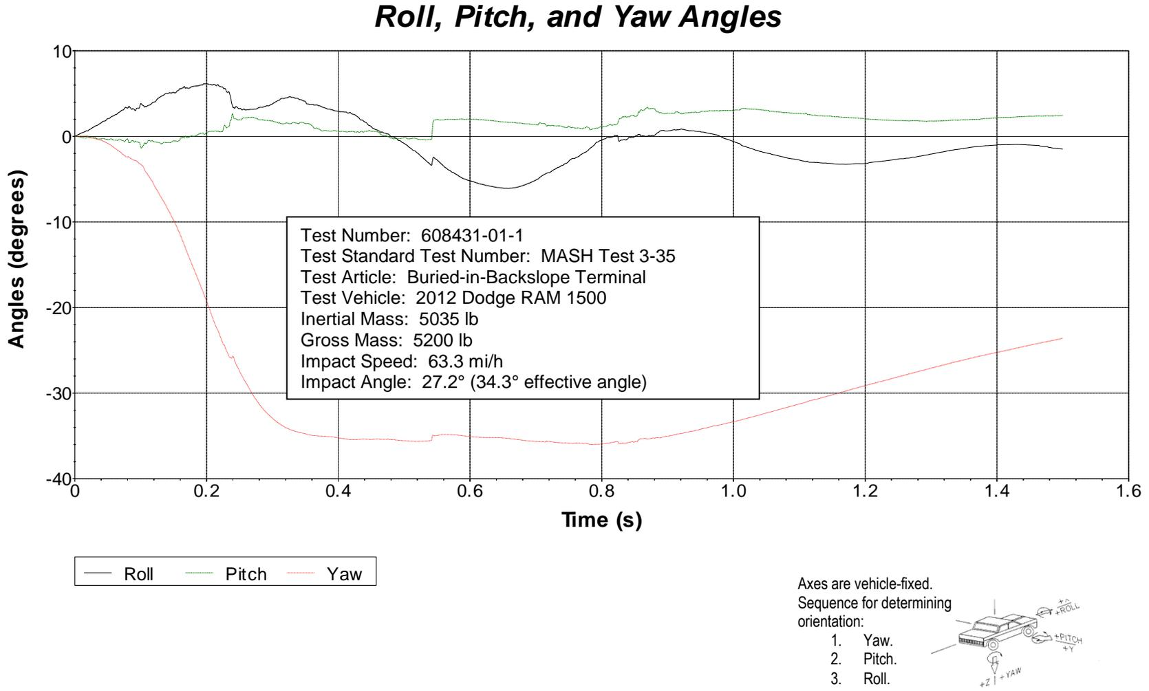
**Figure D.3. Vehicle Angular Displacements for Test No. 608431-01-1.**
