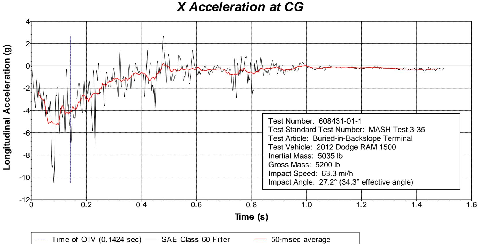
**Figure D.4. Vehicle Longitudinal Accelerometer Trace for Test No. 608431-01-1 (Accelerometer Located at Center of Gravity).**
