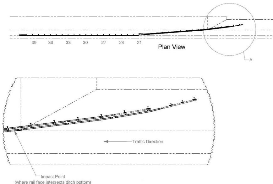
**Figure 3.1. Target CIP for *MASH* Tests 3-34 and 3-35 on BIB Terminal.**
