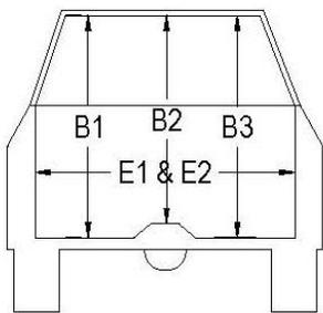
**OCCUPANT COMPARTMENT DEFORMATION MEASUREMENT**
