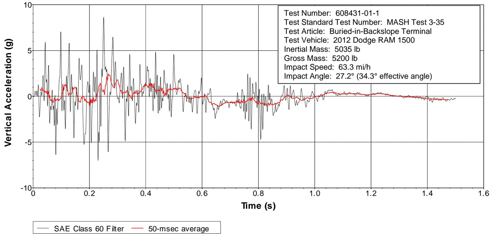
**Figure D.6. Vehicle Vertical Accelerometer Trace for Test No. 608431-01-1 (Accelerometer Located at Center of Gravity).**
