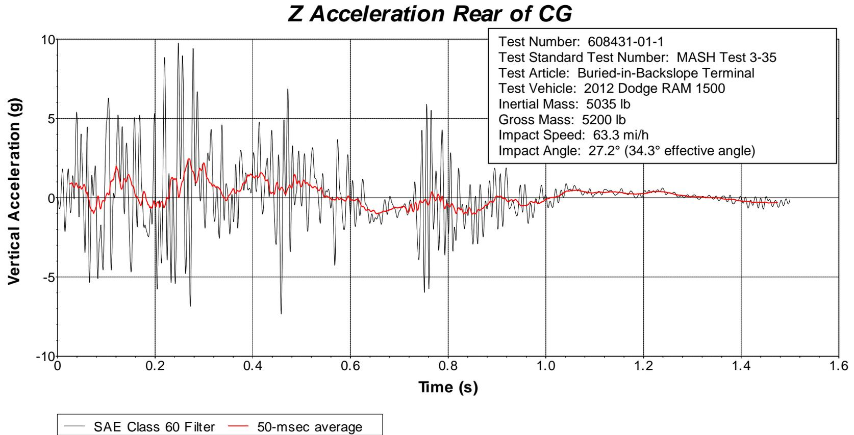
**Figure D.9. Vehicle Vertical Accelerometer Trace for Test No. 608431-01-1
