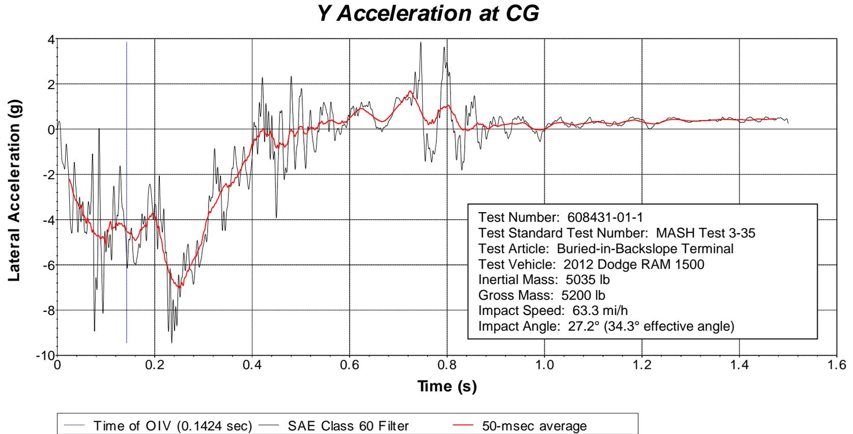
**Figure D.5. Vehicle Lateral Accelerometer Trace for Test No. 608431-01-1
