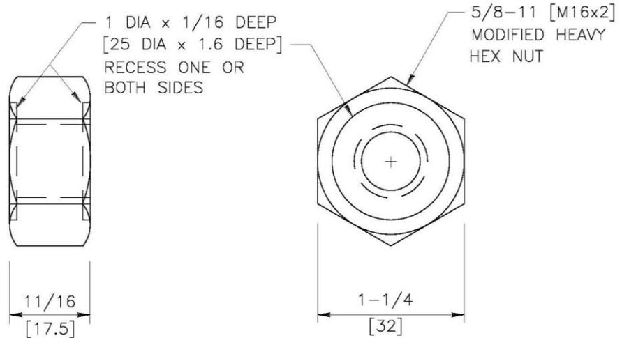
GUARDRAIL BOLT AND RECESSED NUT
