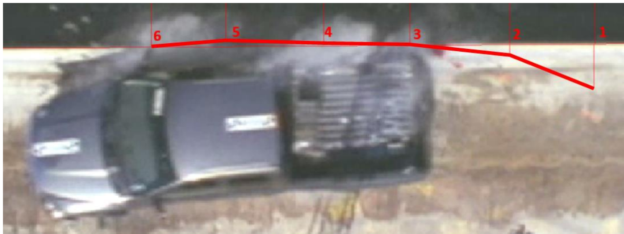
Figure 2.21. Sketch of Vehicle Extension (Side View Mirror) over Barrier (TTI Test Number 420020-3)
