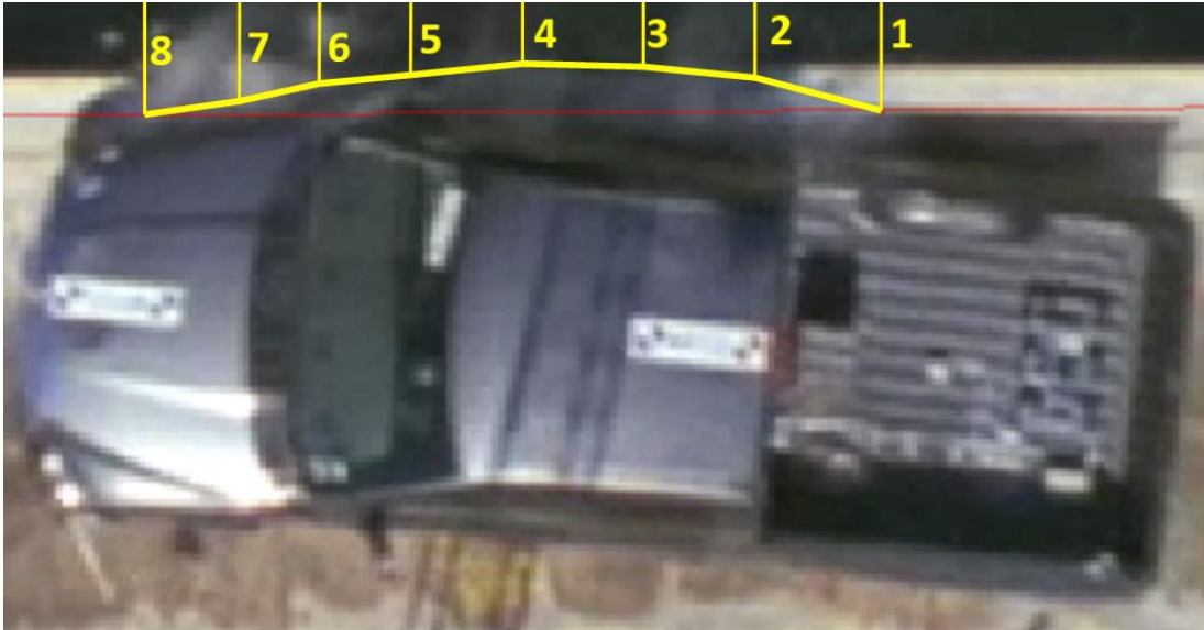
Figure 2.22. Sketch of Vehicle Extension (Front Passenger Corner) over Barrier (TTI Test Number 420020-3)
