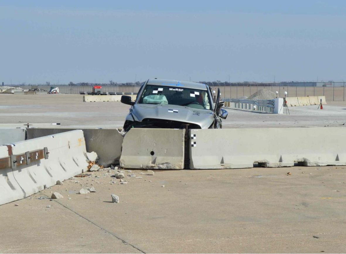
Figure 45. Vehicle Final Position and Trajectory Marks, Test No. 34AGT-1
