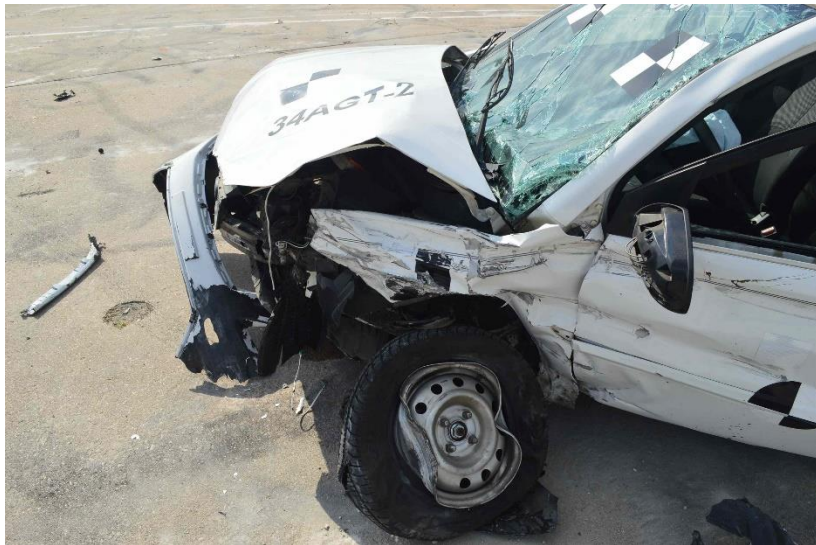
Figure 65. Vehicle Damage, Test No. 34AGT-2
