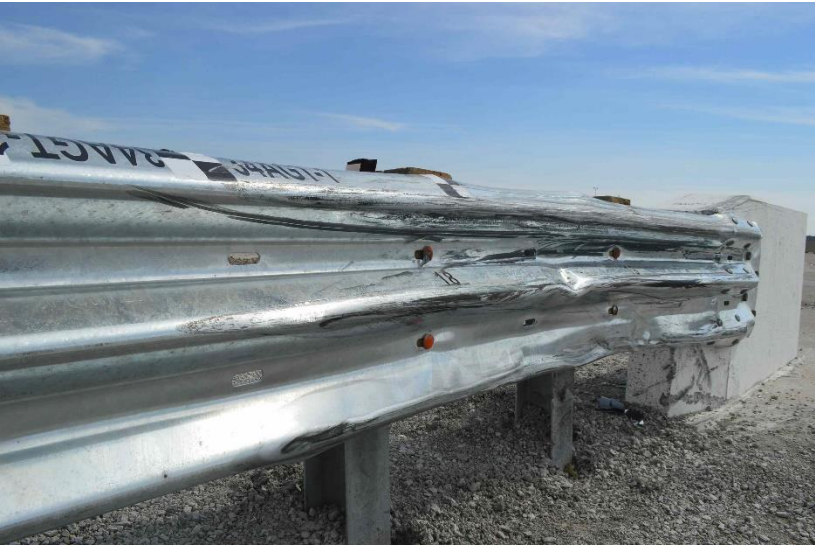
Figure 46. System Damage, Test No. 34AGT-1
