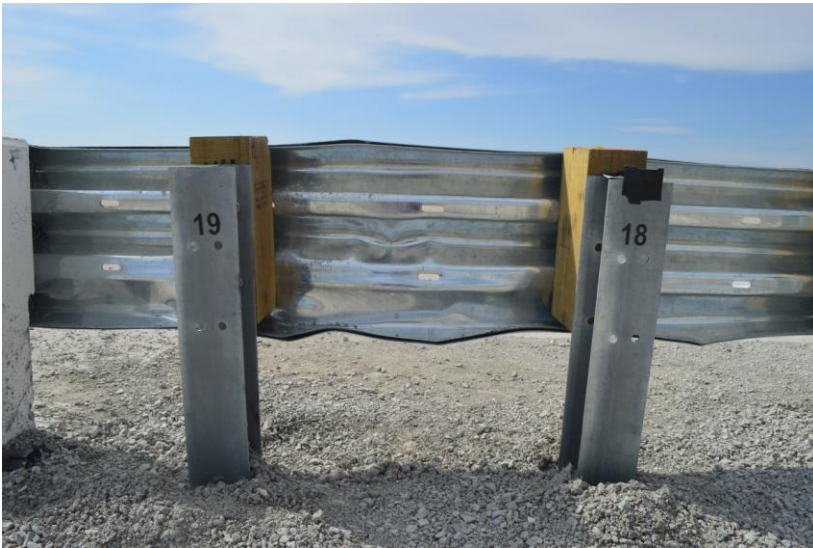
Figure 48. System Damage, Post No. 19 and Rail Connection Terminal, Test No. 34AGT-1
