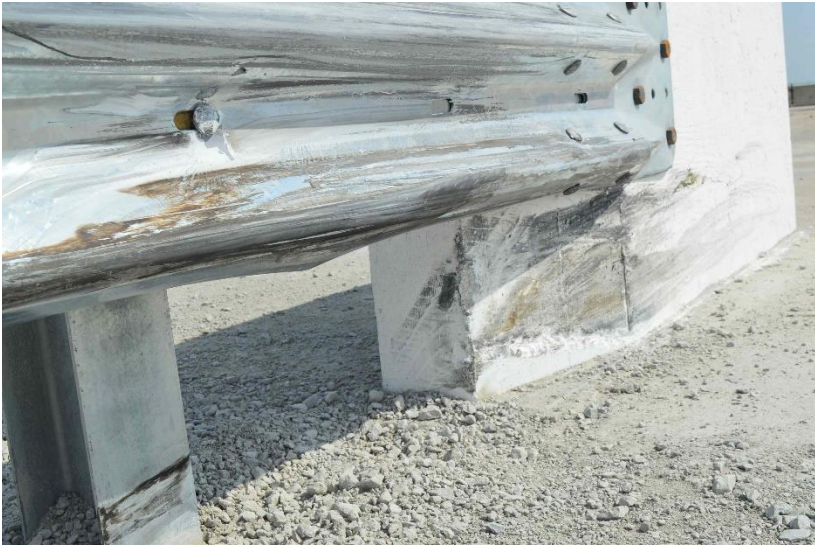
Figure 62. System Damage, Concrete Buttress, Test No. 34AGT-2
