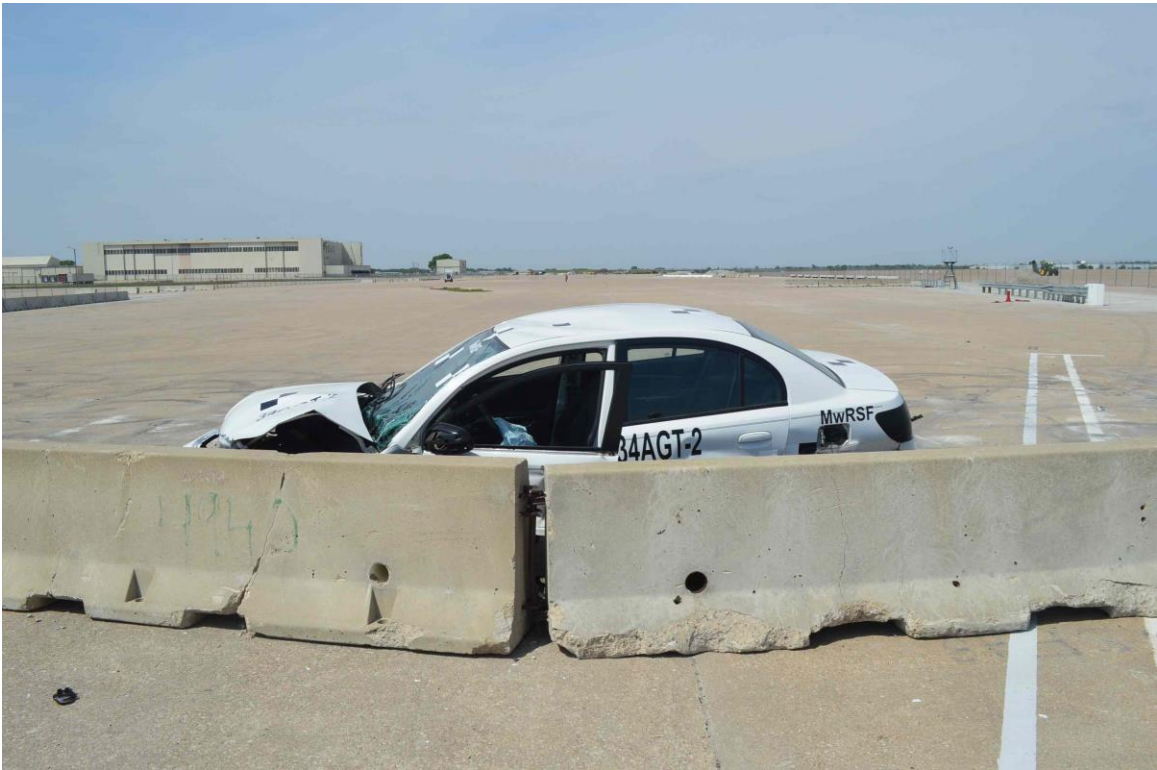
Figure 59. Vehicle Final Position and Trajectory Marks, Test No. 34AGT-2
