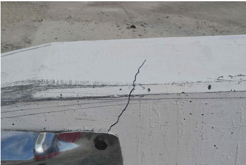
Figure 49. Buttress Damage, Test No. 34AGT-1
