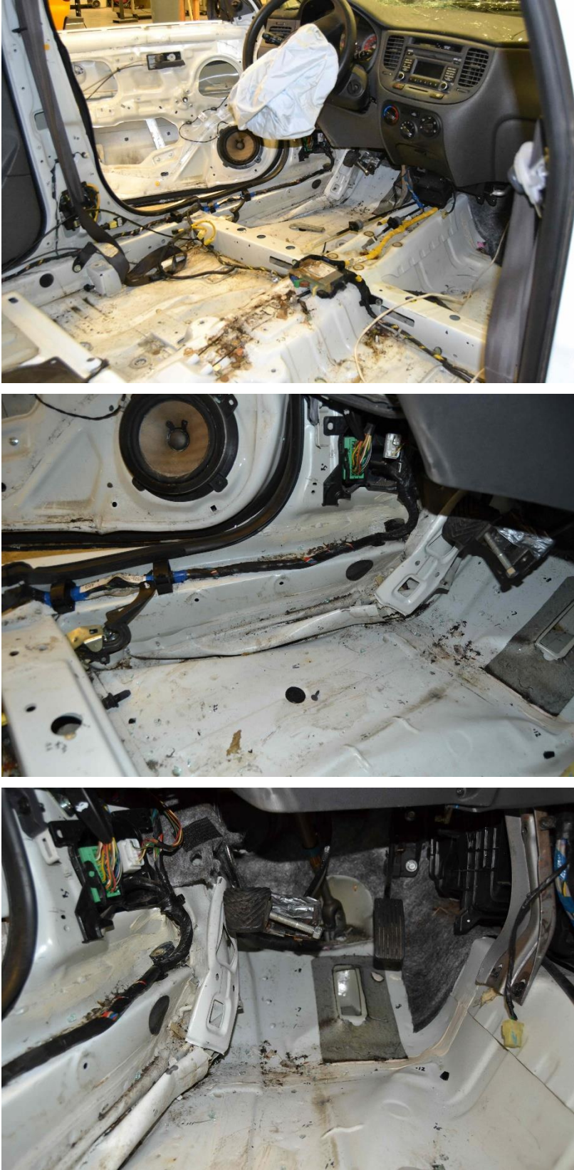
Figure 67. Occupant Compartment Deformation, Test No. 34AGT-2
