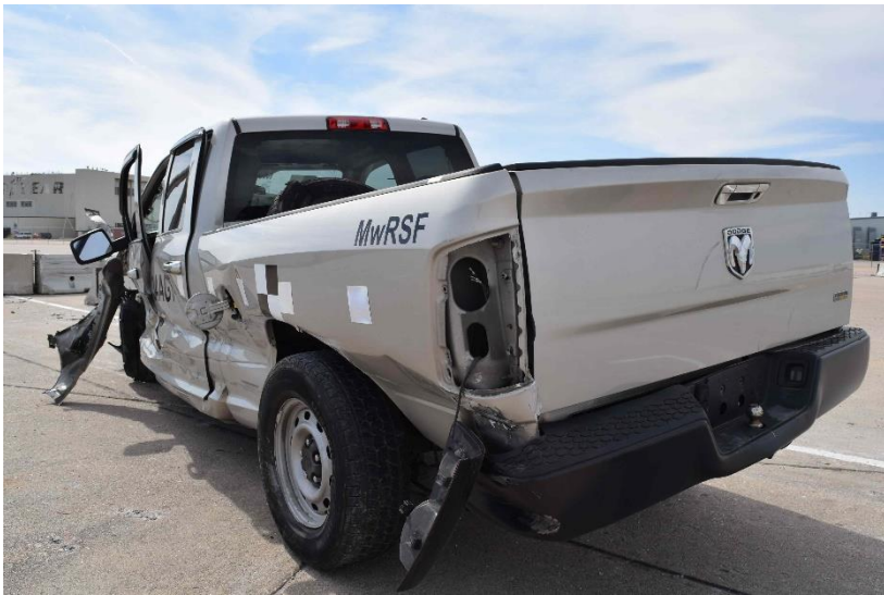
Figure 51. Vehicle Damage, Test No. 34AGT-1
