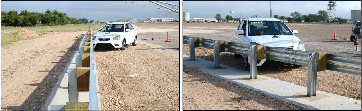
**Figure 6.3. Guardrail/Test Vehicle Geometries for Test No. 608551-3.**
