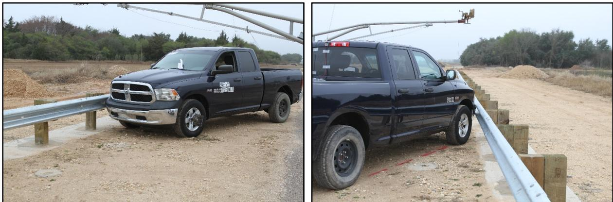
**Figure 5.3. Guardrail in Mow Strip/Test Vehicle Geometrics for Test No. 608551-5.**
