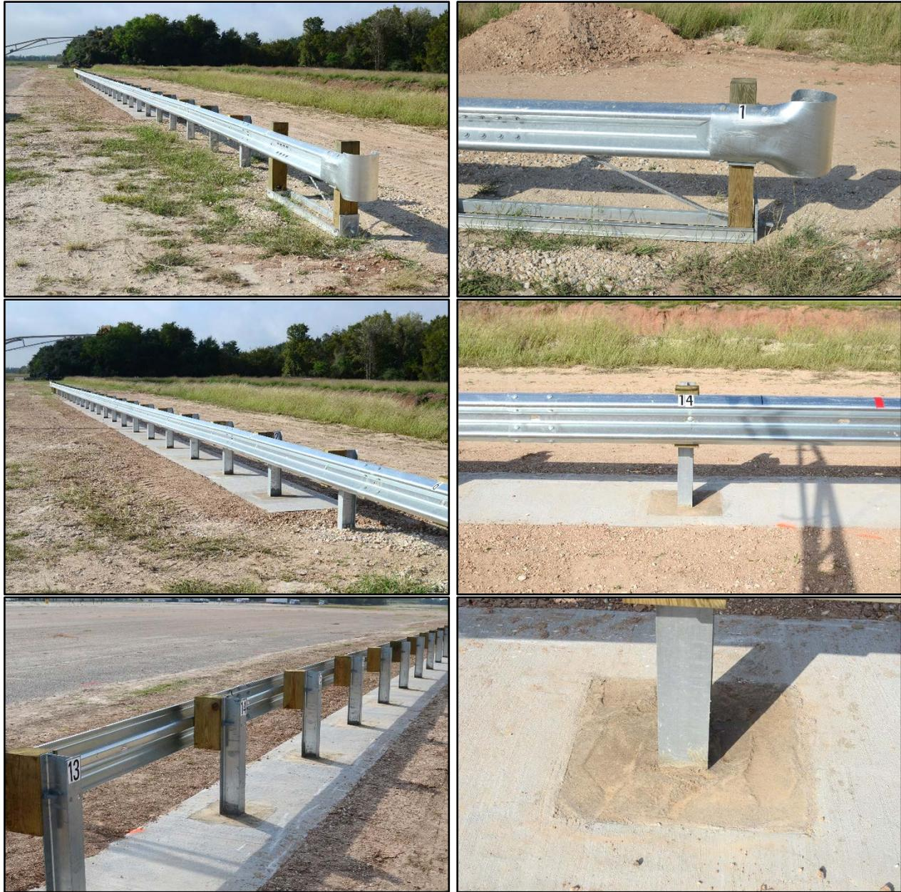
**Figure 6.2. 31-inch W-Beam Guardrail on Steel Posts in Concrete Mow Strip prior to Testing.**
