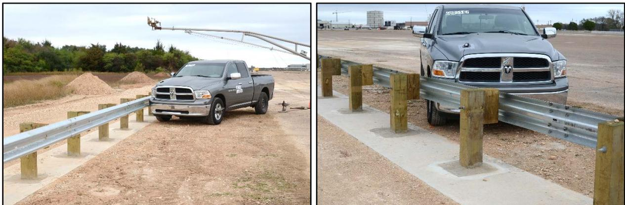
Figure 4.10. Guardrail in Mow Strip/Test Vehicle Geometrics for Test No. 608551-2.
