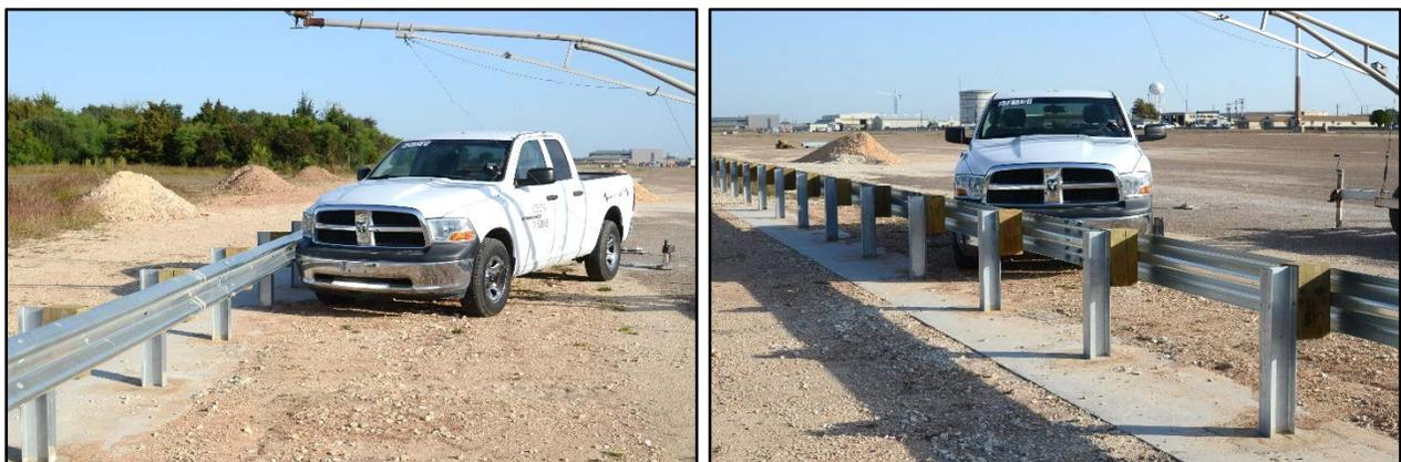
**Figure 6.10. Guardrail/Test Vehicle Geometrics for Test No. 608551-4.**
