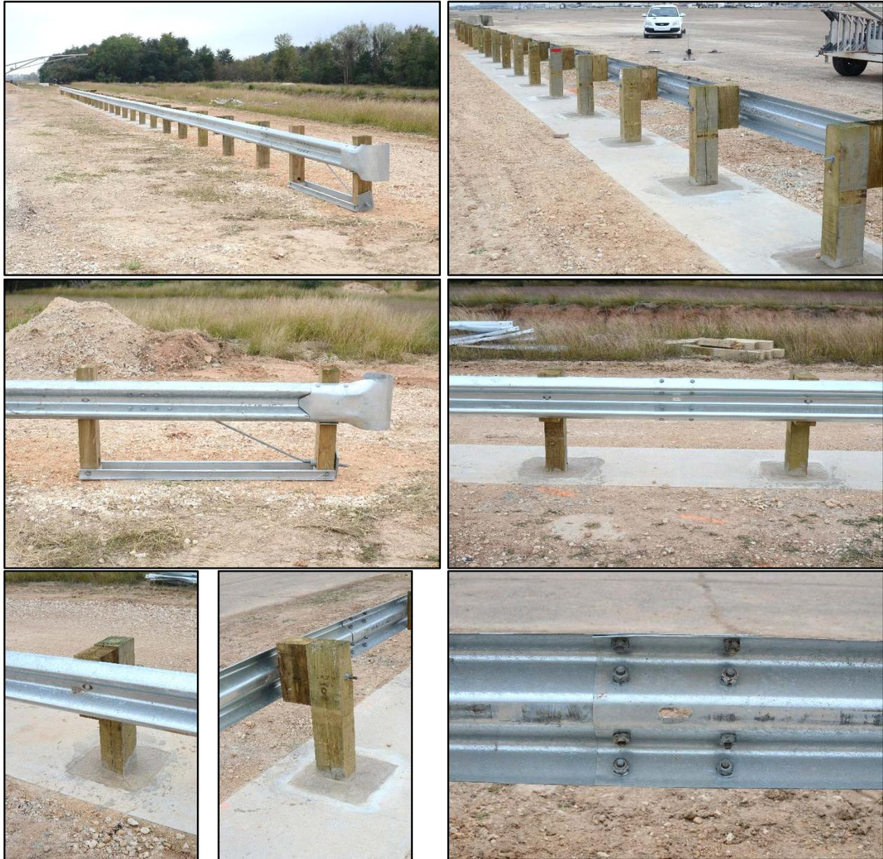
**Figure 4.2. 31-inch W-Beam Guardrail on Wood Posts in Concrete Mow Strip prior to Test Nos. 608551-1 and 2.**
