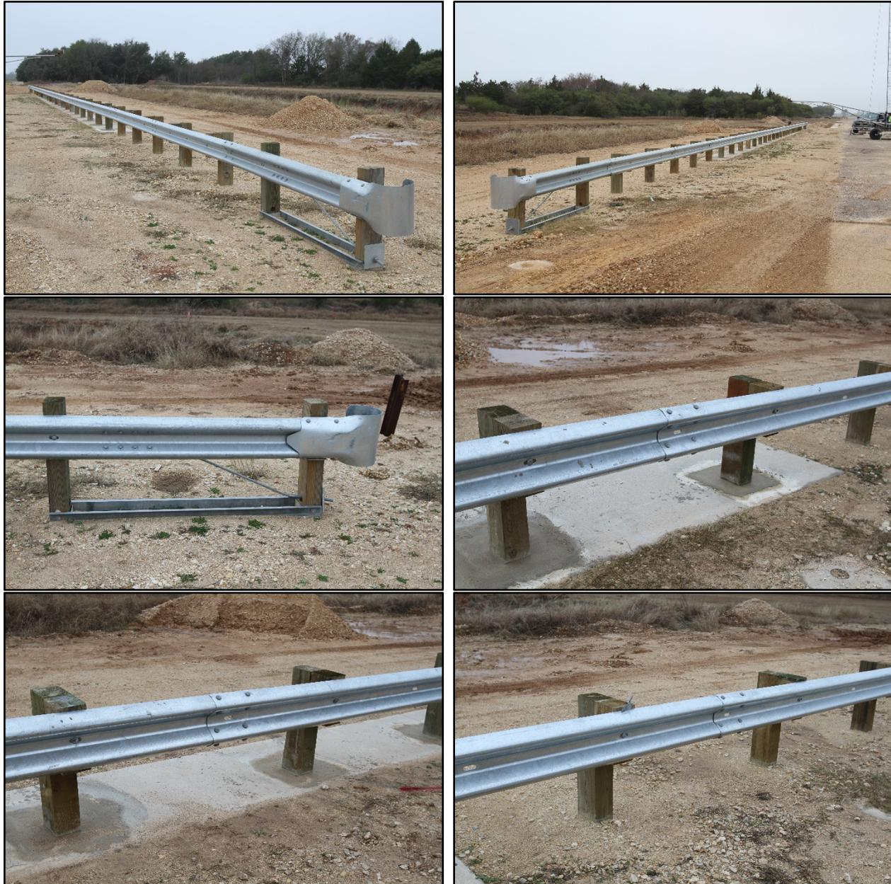
**Figure 5.2. 31-inch W-Beam Guardrail on Wood Posts with Reduced Embedment in Concrete Mow Strip prior to Test No. 608551-5.**
