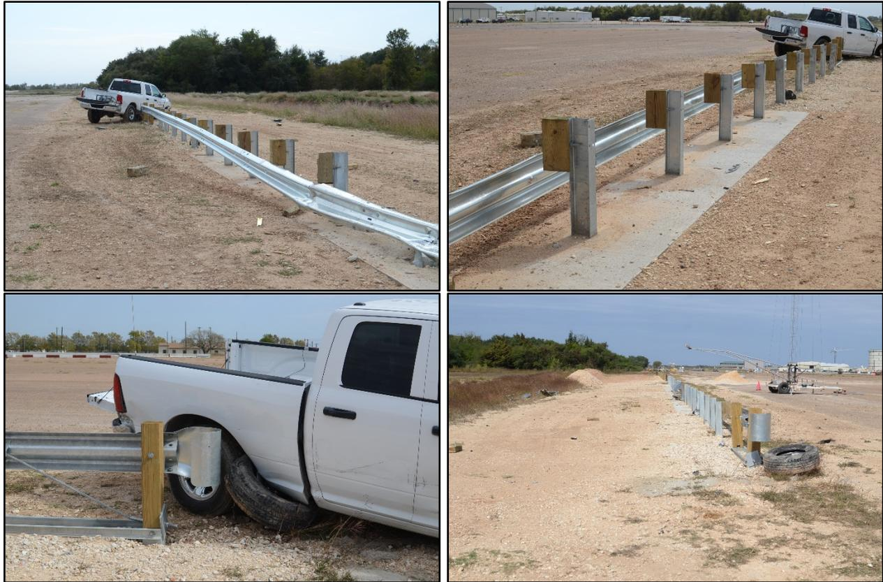
**Figure 6.14. Guardrail Downstream of Impact Area after Test No. 608551-4.**
