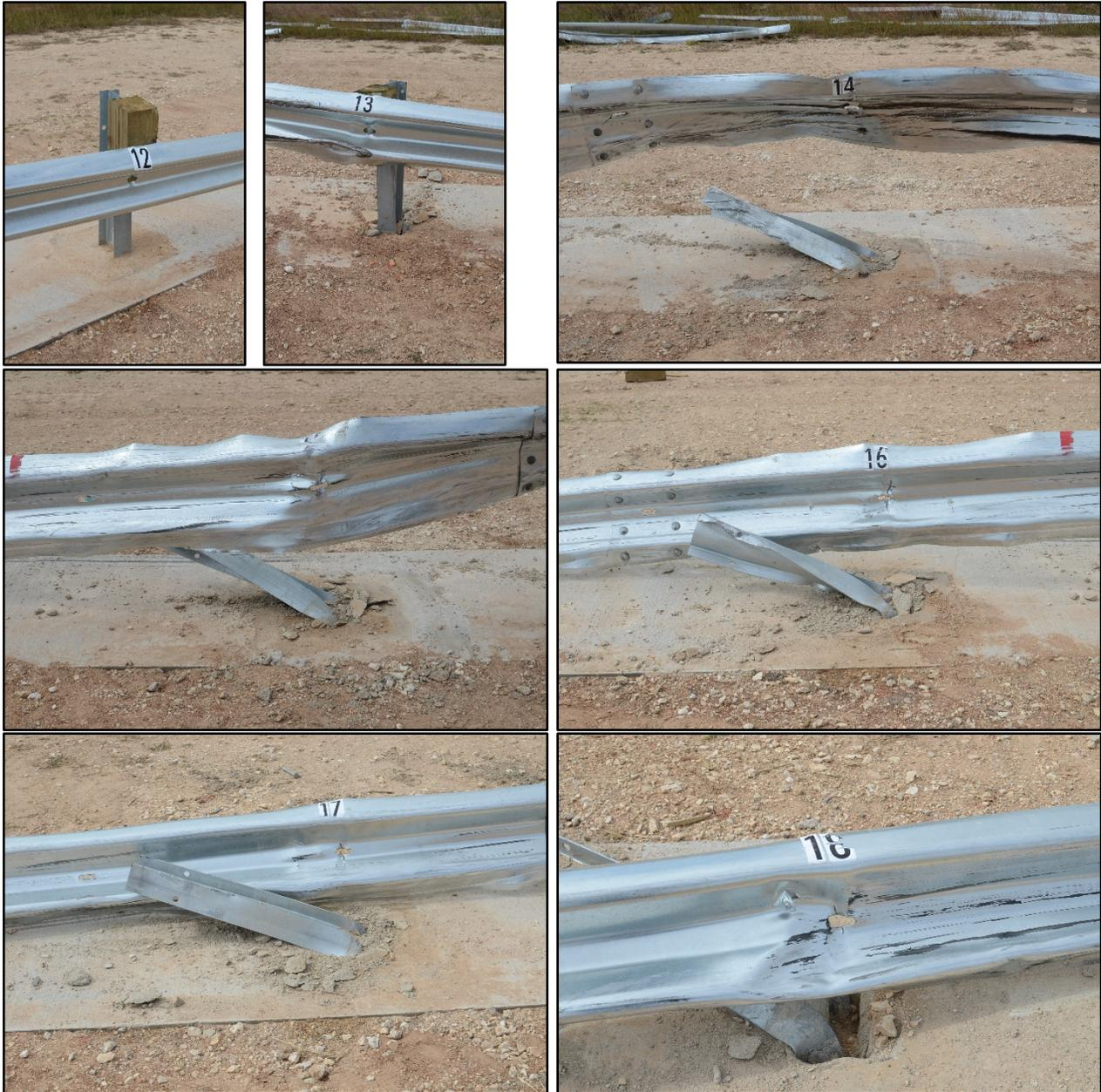
**Figure 6.13. Posts 12-18 after Test No. 608551-4.**
