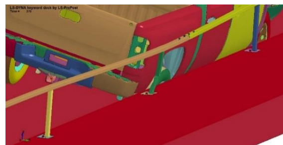
Figure 81. Post Snag Sequential Views, Impact 1.7 ft (0.5 m) US from Post No. 7 Simulation
