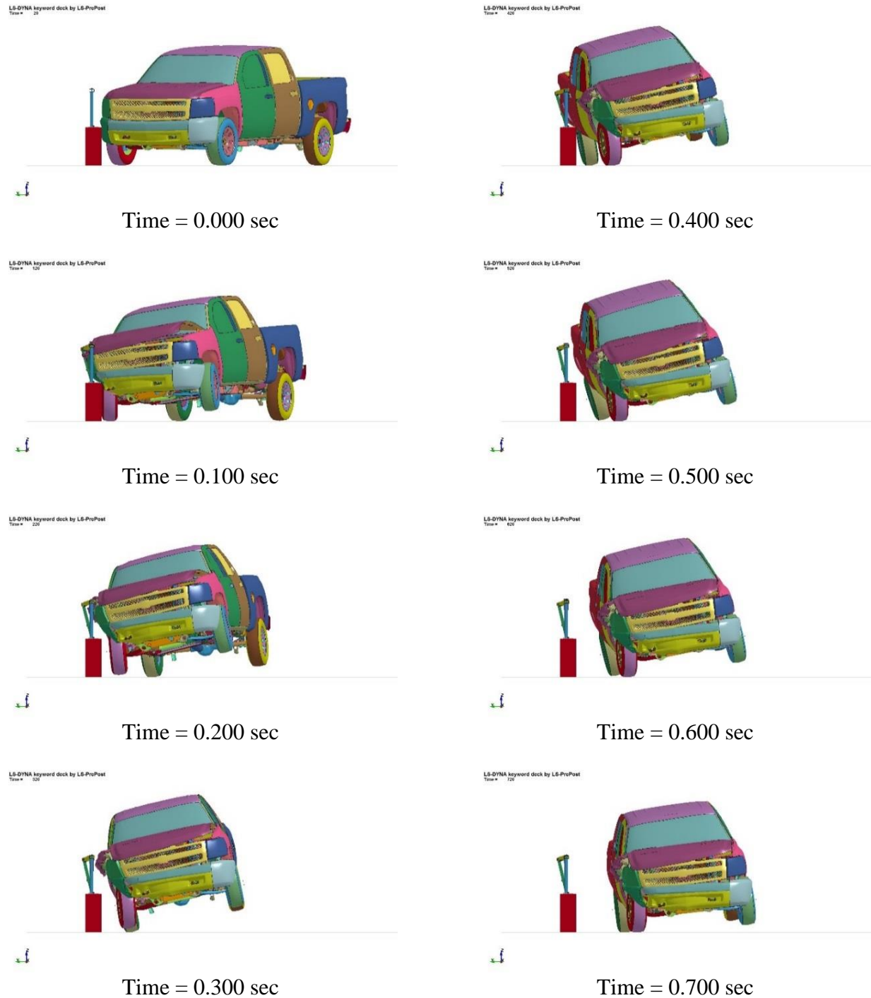
Figure 80. Downstream Sequential Views, Impact 1.7 ft (0.5 m) US from Post No. 7 Simulation
