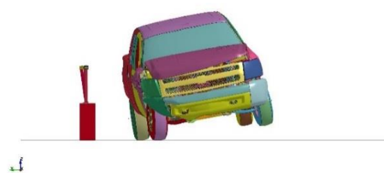
Figure 83. Downstream Sequential Views, Impact 2.6 ft (0.8 m) US from Splice Reversed Simulation
