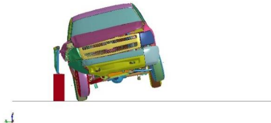
Figure 76. Downstream Sequential Views, Impact 4.3 ft (1.3 m) US from Post No. 7 Simulation
