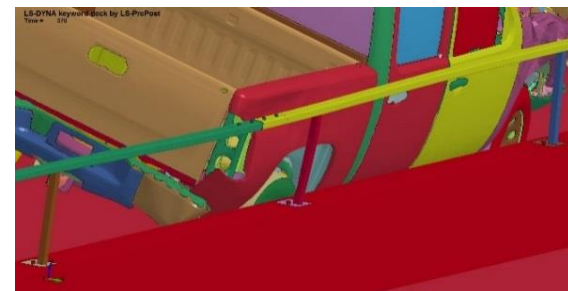
Figure 84. Post Snag Sequential Views, Impact 2.6 ft (0.8 m) US from Splice Reversed Simulation
