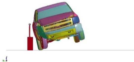
Figure 83. Downstream Sequential Views, Impact 2.6 ft (0.8 m) US from Splice Reversed Simulation
