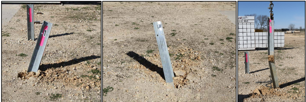
Figure 3.5. Direct Embedded Post after Test No. 611011-B1.
