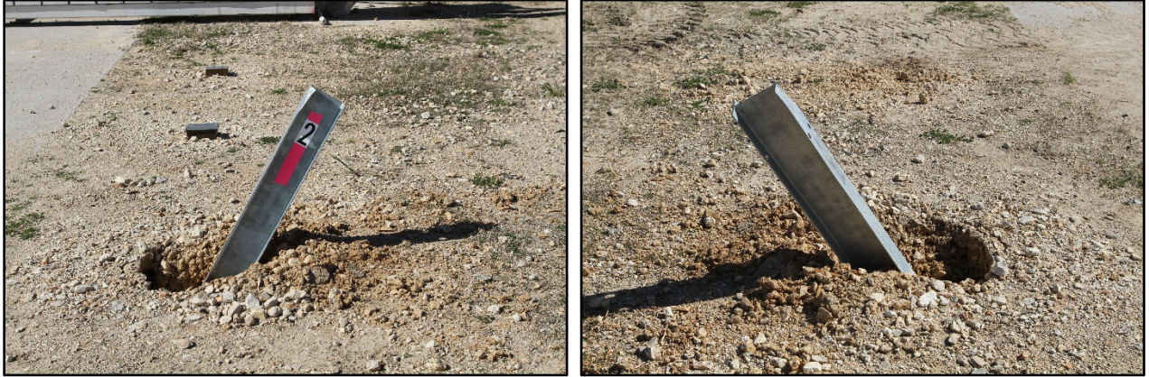
Figure 3.10. Direct Embedded Post after Test No. 611011-B2.
