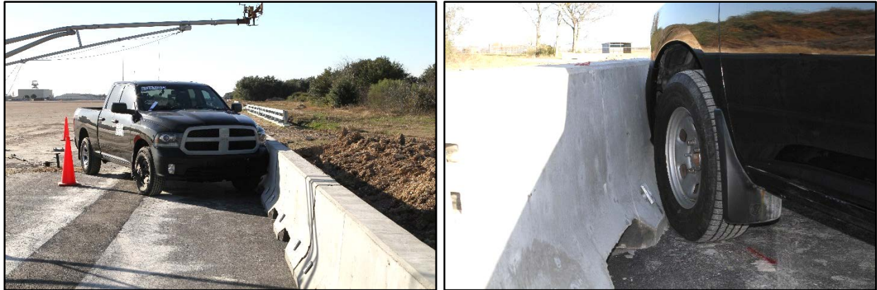
Figure 4.3. Barrier/Test Vehicle Geometrics for Test No. 612831-01-1.
