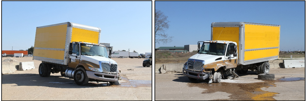
Figure 6.6. Test Vehicle after Test No. 612831-01-3.
