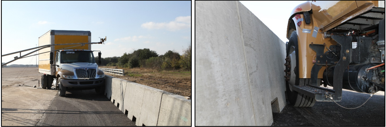
Figure 6.3. Embedded Single-Slope Barrier with Drainage Scuppers/Test Vehicle Geometrics for Test No. 612831-01-3.
