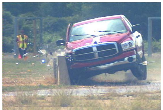
Figure E1. Sequential Photographs for Test No. 490022-4 (Overhead and Frontal Views).
