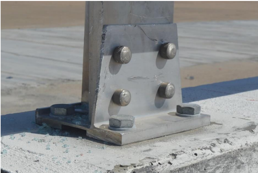
Figure 57. Rail and Post No. 11 Damage, Test No. NCBR-1
