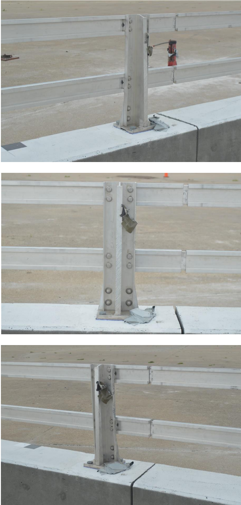
Figure 78. Post No. 6 Backside Damage, Test No. NCBR-2
