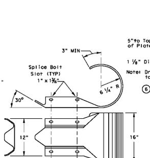
**9 W-BEAM END SECTION (ROUNDED) (12 GA.)**
