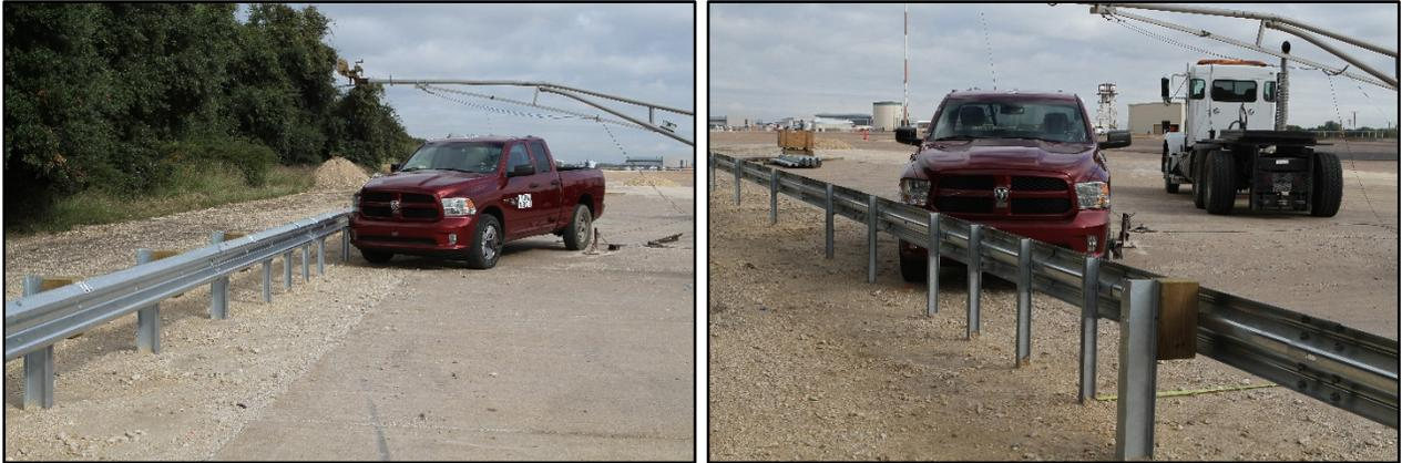
**Figure 5.1. Transition/Test Vehicle Geometrics for Test No. 612051-02-1.**
