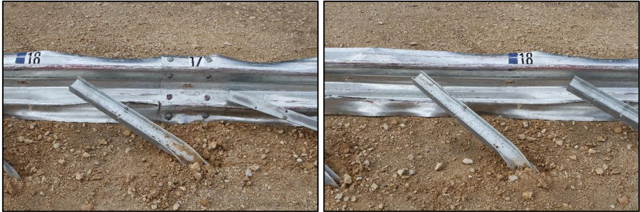
**Figure 5.5. Posts 17 and 18 after Test No. 612051-02-1.**
