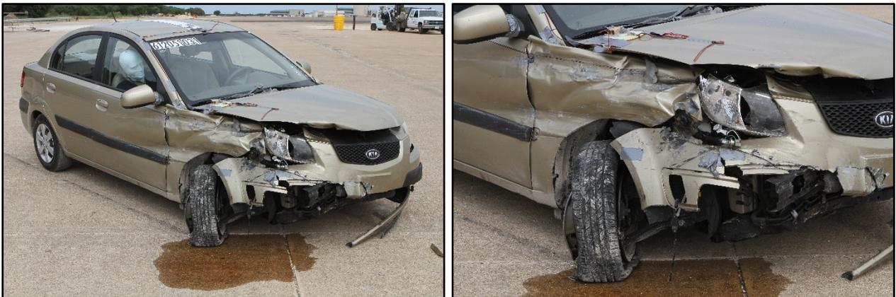
**Figure 6.4. Test Vehicle after Test No. 612051-03-1.**
