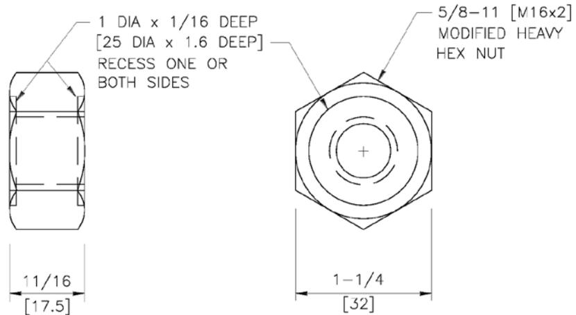
GUARDRAIL BOLT AND RECESSED NUT
