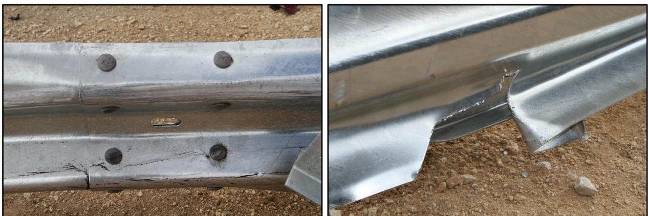
**Figure 5.7. Partial Tear of Rail Element after Test No. 612051-02-1.**
