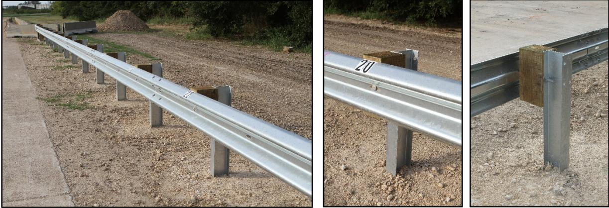
**Figure 2.4. MGS Strong Post System prior to Testing.**
