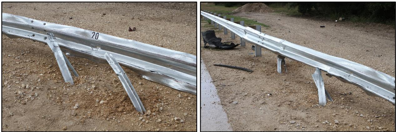
**Figure 5.6. Posts 19 through 25 after Test No. 612051-02-1.**
