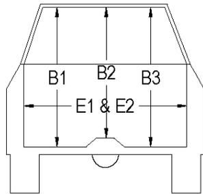
**OCCUPANT COMPARTMENT DEFORMATION MEASUREMENT**
