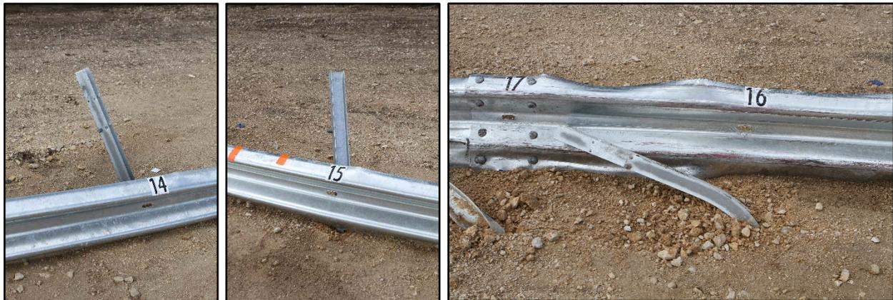
**Figure 5.4. Posts 14 through 16 after Test No. 612051-02-1.**
