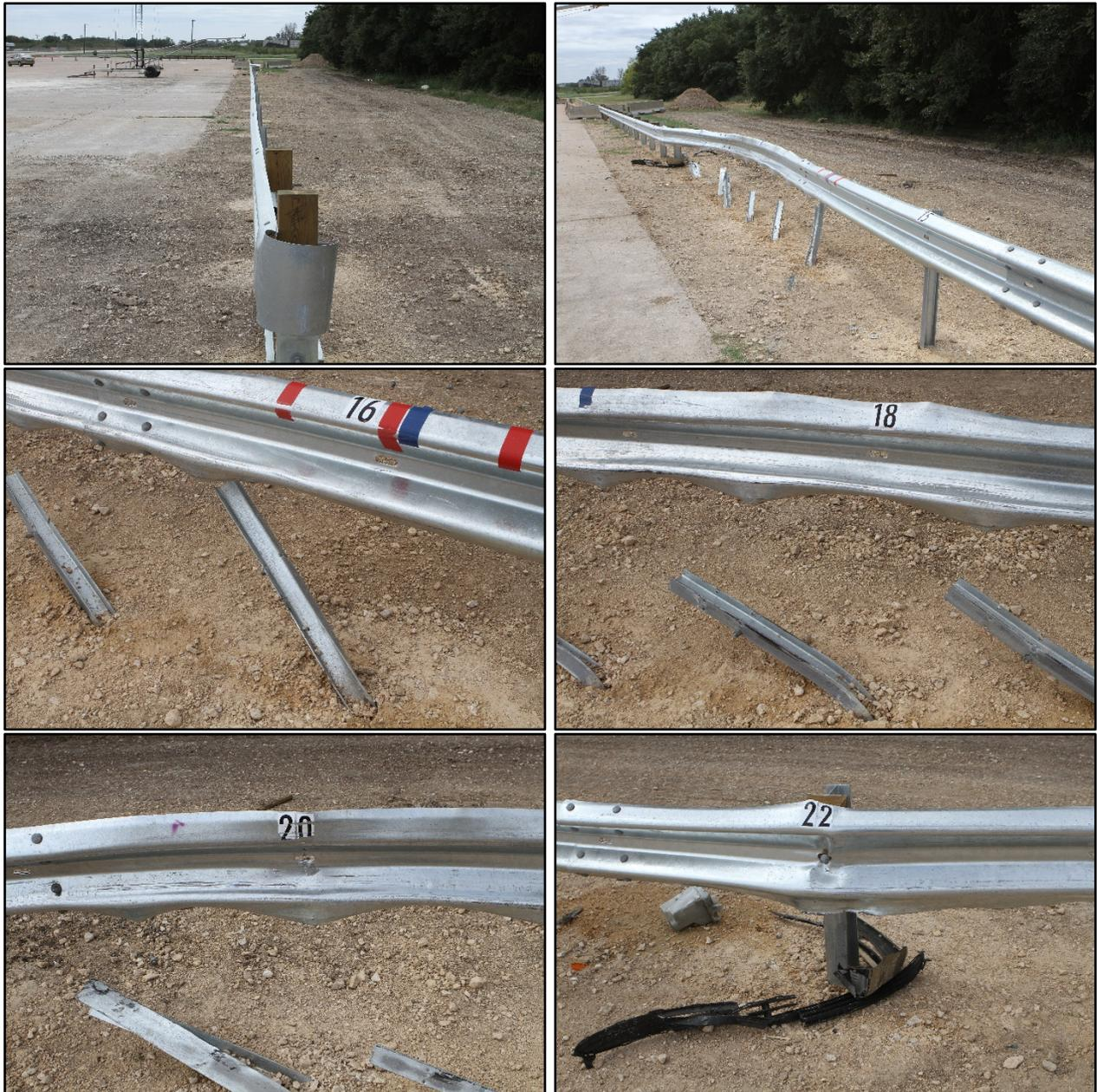
**Figure 6.3. Transition after Test No. 612051-03-1.**
