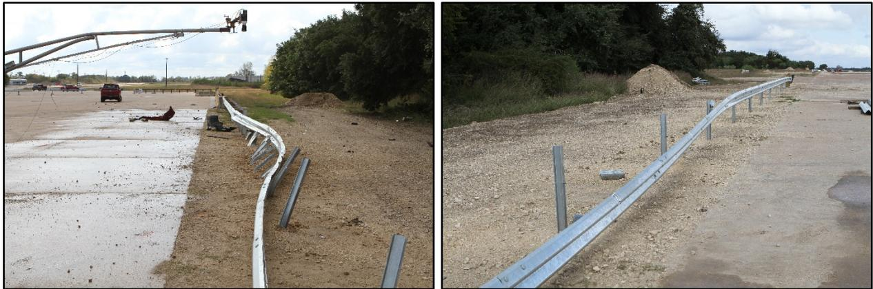
**Figure 5.3. Transition after Test No. 612051-02-1.**
