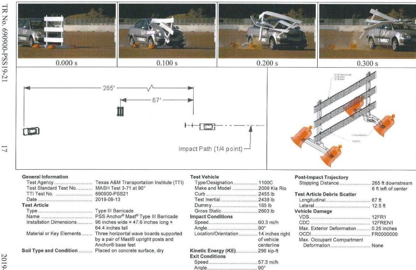
Figure 5.6. Summary of Results for MASH Test 3-71 at 90° on PSS Anchor® Mast® Type III Barricade.
