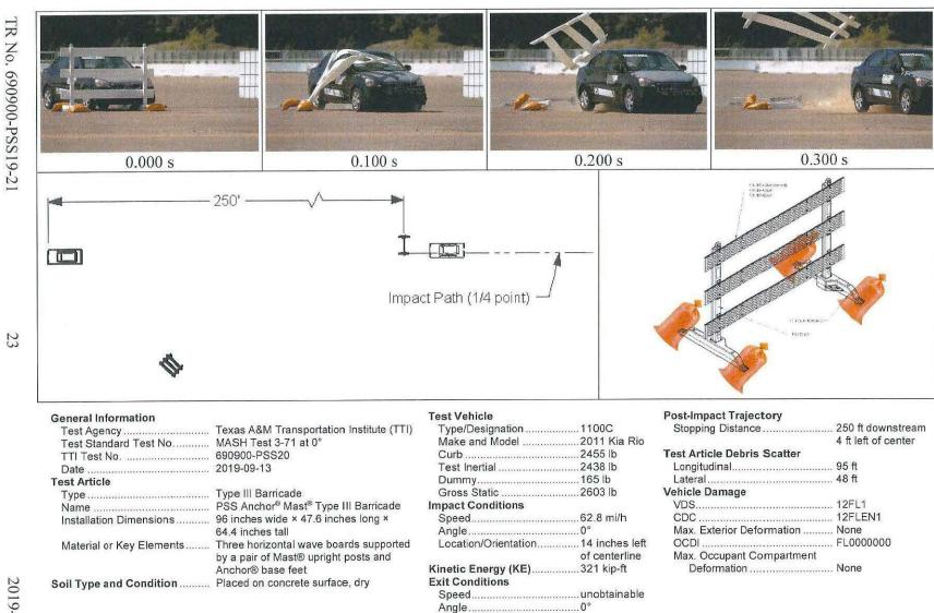
Figure 6.6. Summary of Results for MASH Test 3-71 at 0° on PSS Anchor® Mast® Type III Barricade.
