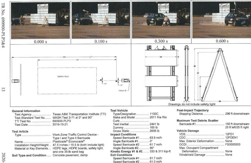
Figure 5.6. Summary of Results for MASH Test 3-71 at 0° and 90° on Plasticade® Econocade® Type I and Type II Barricades
