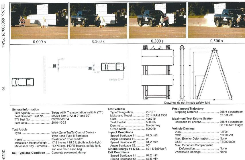
Figure 6.7. Summary of Results for MASH Test 3-72 at 0° and 90° on Plasticade® Econocade® Type I and Type II Barricades.
