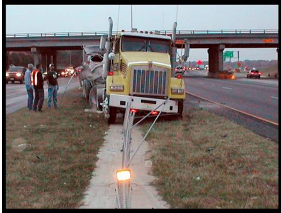
Figure 5. Large Truck Stopped by Cable Median Barrier System in Oklahoma [20]
