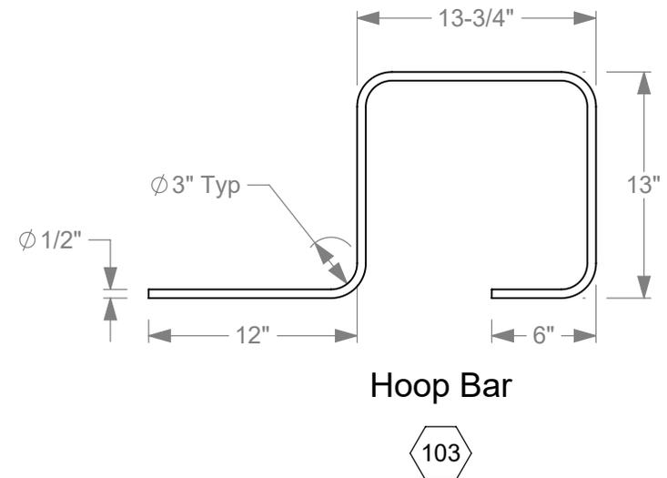
**7a.** All bent bars, and all longitudinal bars in the Curb, Deck and Wall shall be epoxy coated. All bars are grade 60..
