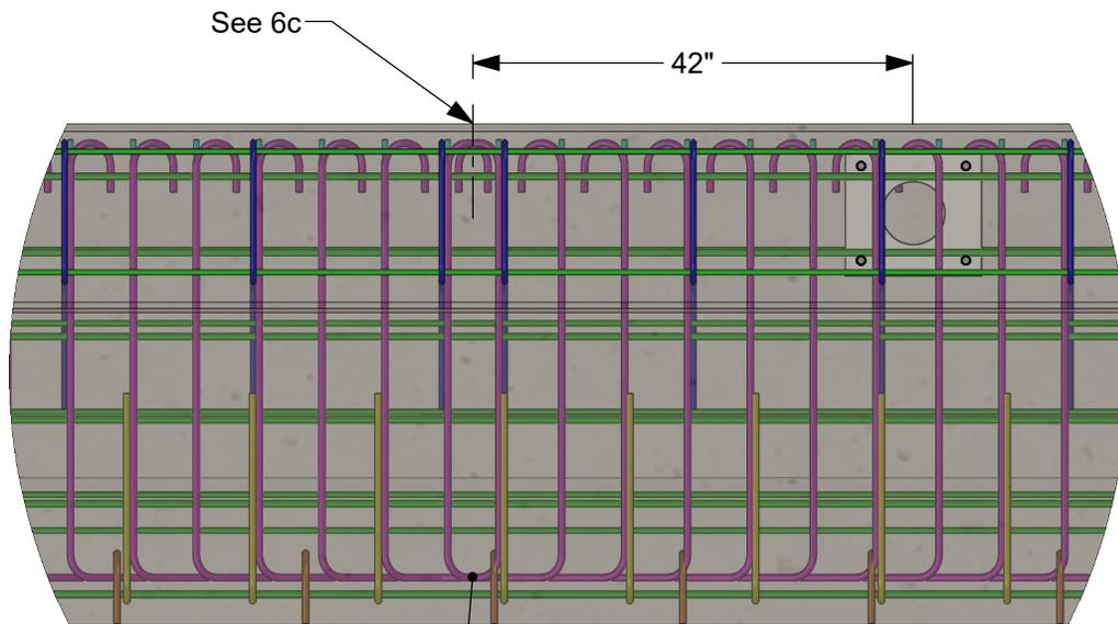
Offset Hook Bars as needed to avoid interference.
