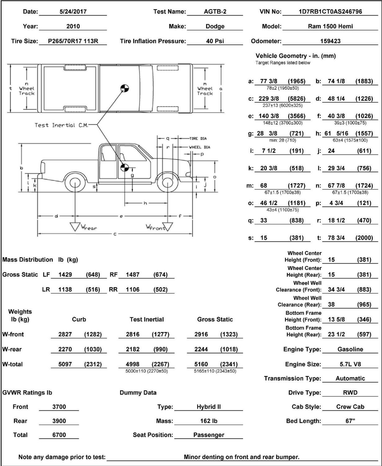
Figure 31. Vehicle Dimensions, Test No. AGTB-2
