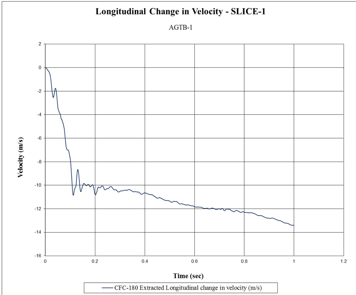
Figure E-2. Longitudinal Occupant Impact Velocity (SLICE-1), Test No. AGTB-1
