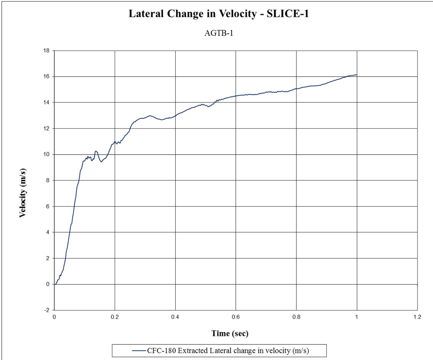
Figure E-5. Lateral Occupant Impact Velocity (SLICE-1), Test No. AGTB-1
