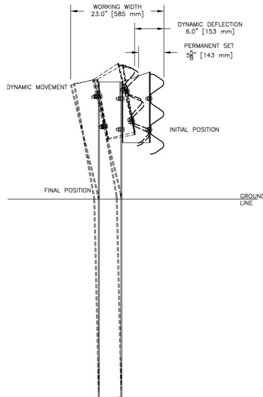
Figure 43. Maximum Dynamic Deflection and Working Width, Test No. AGTB-1
