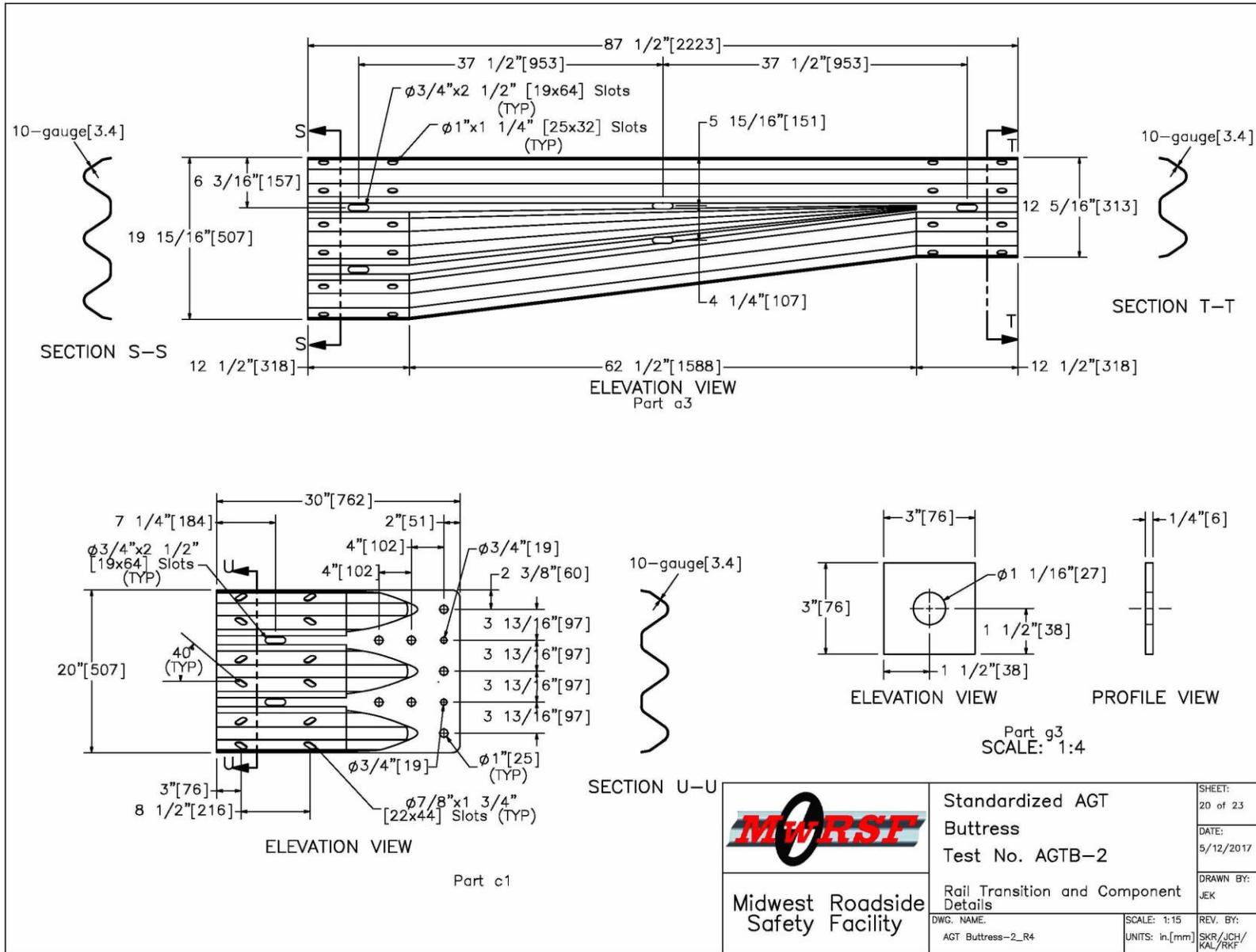
Figure 67. Rail Transition and Component Details, Test No. AGTB-2
