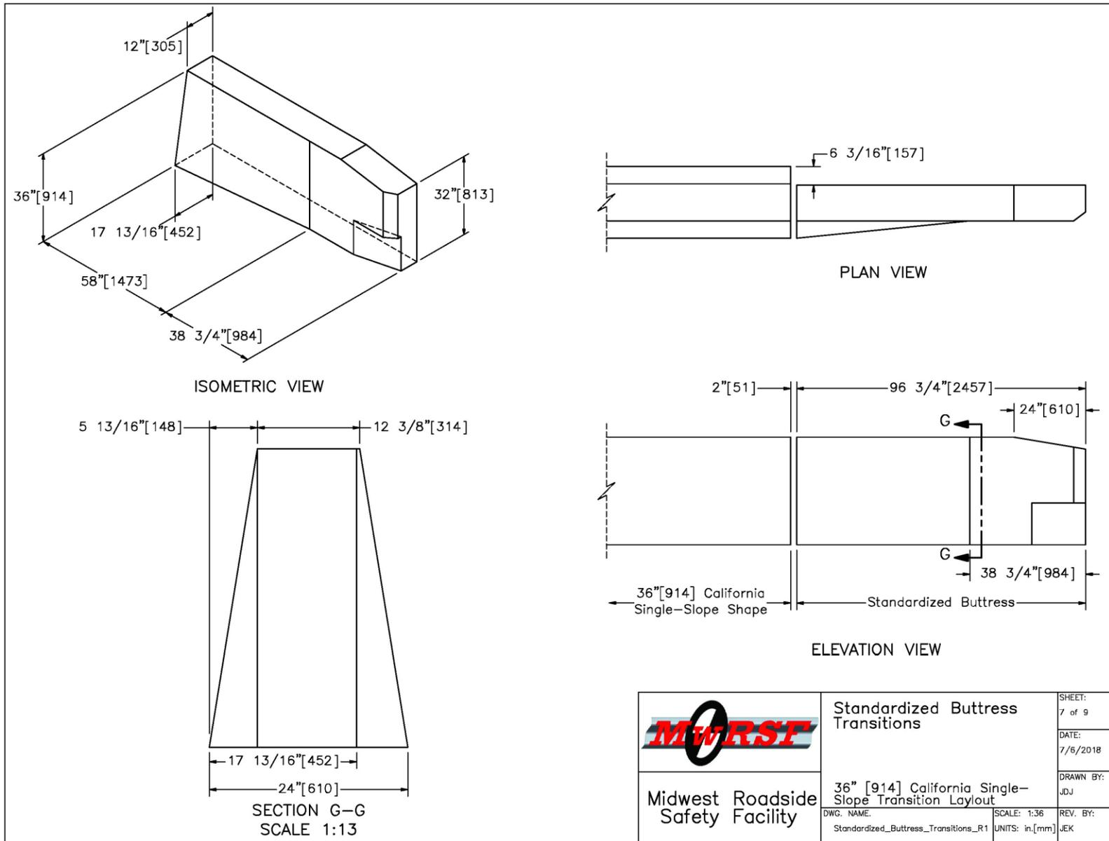
Figure 92. Buttress Shape Transition to 36-in. Tall California Single Slope Barrier
