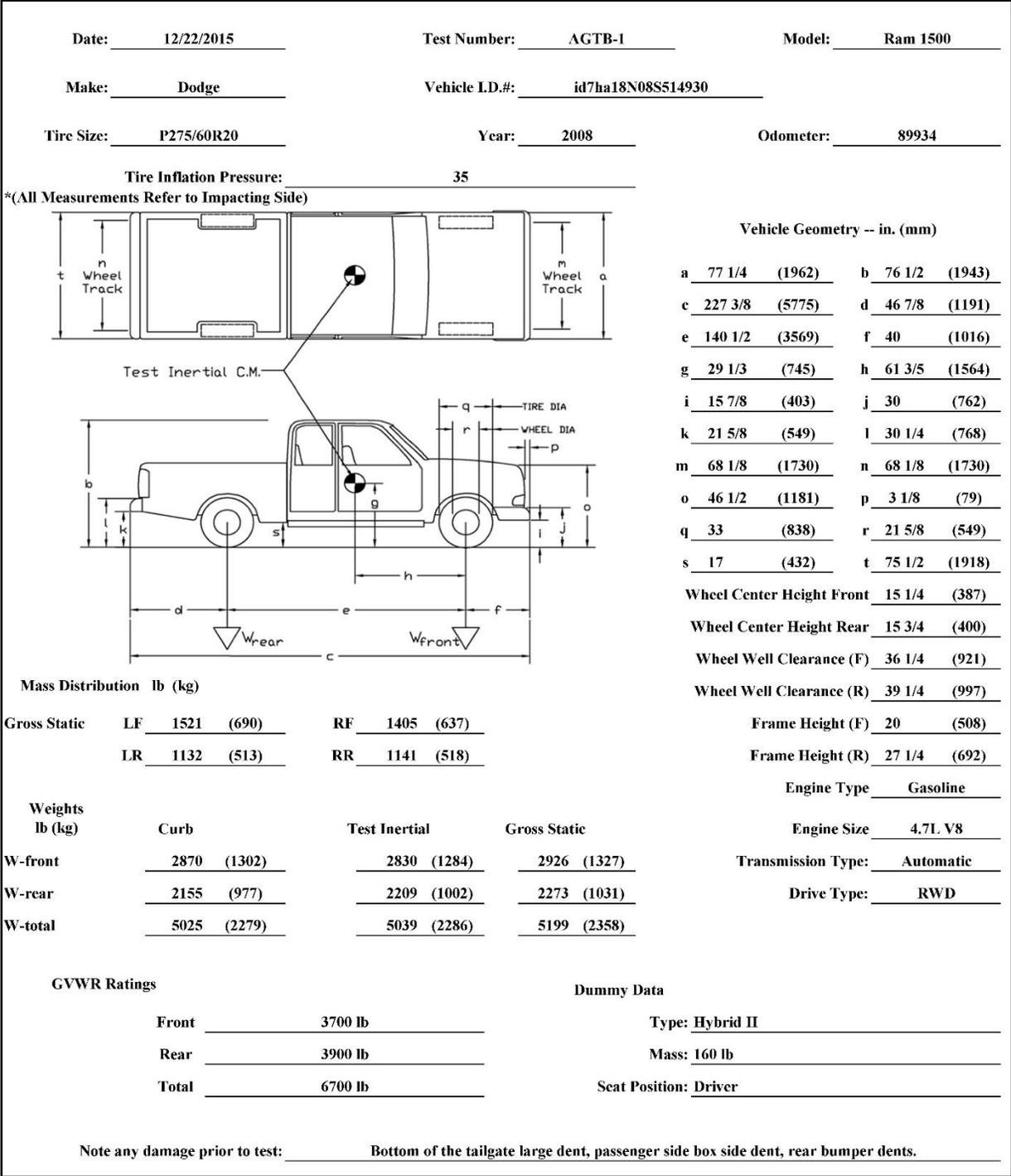
Figure 29. Vehicle Dimensions, Test No. AGTB-1
