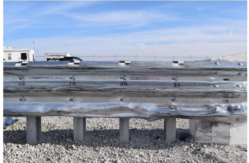
Figure 41. System Damage, Test No. AGTB-1
