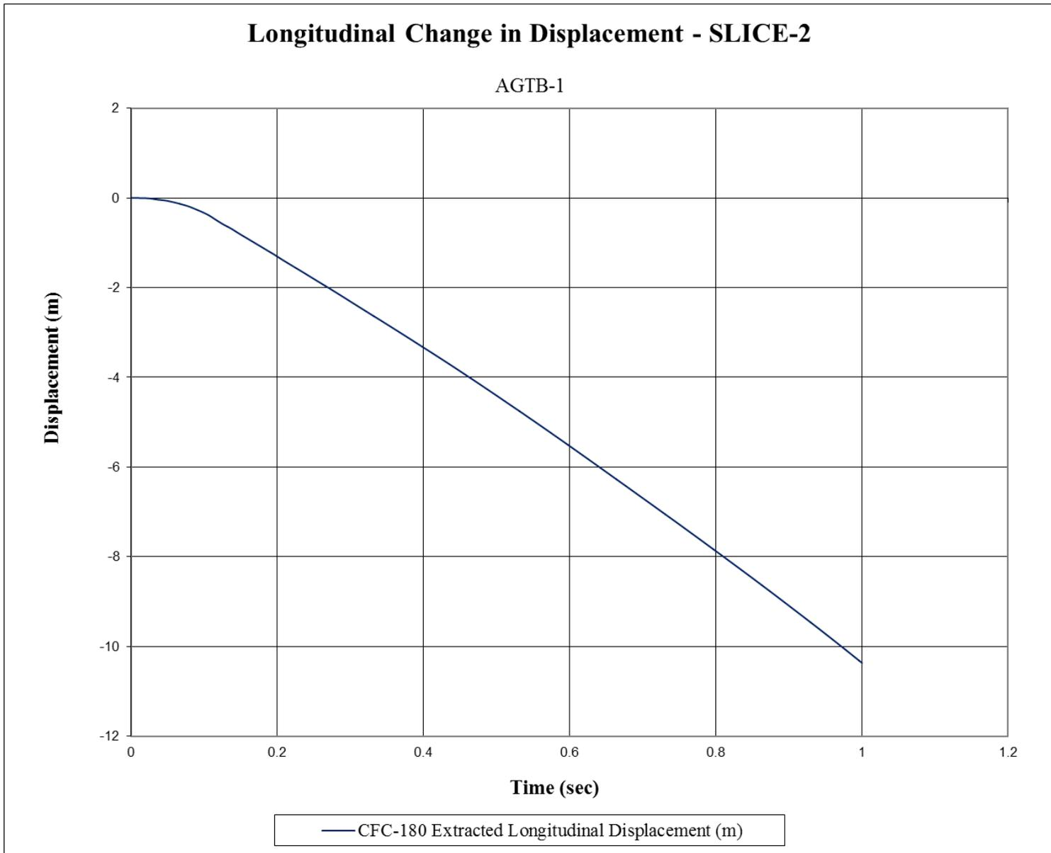
Figure E-11. Longitudinal Occupant Displacement (SLICE-2), Test No. AGTB-1
