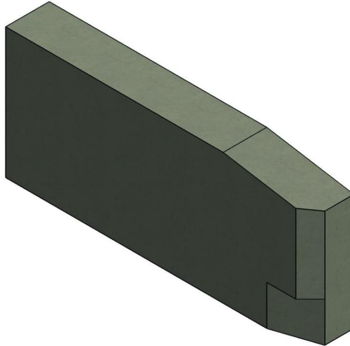
Figure 1. General Shape of Standardized Buttress Incorporating Dual Tapered Front Edge
