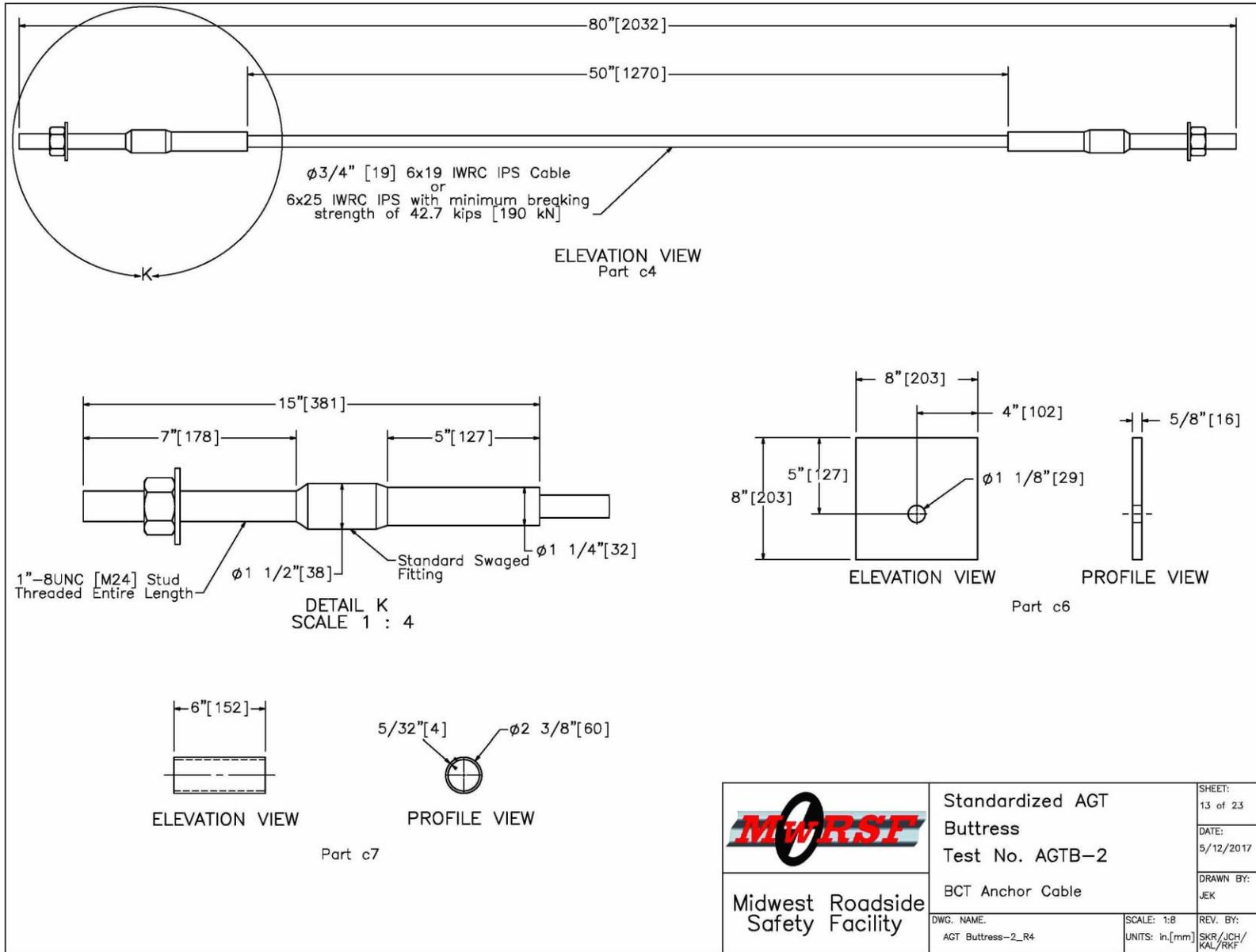
Figure 60. BCT Anchor Cable, Test No. AGTB-2
