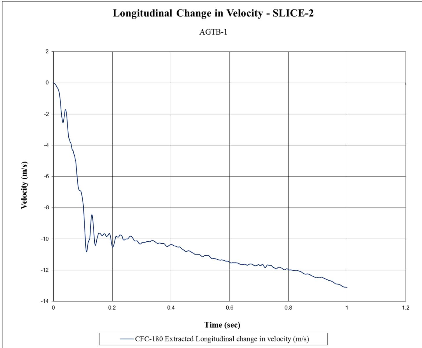
Figure E-10. Longitudinal Occupant Impact Velocity (SLICE-2), Test No. AGTB-1
