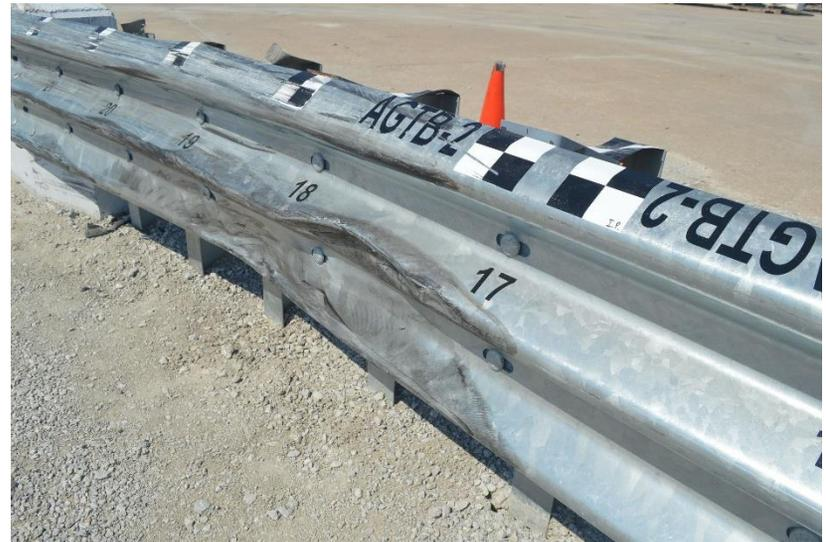
Figure 76. System Damage, Test No. AGTB-2
