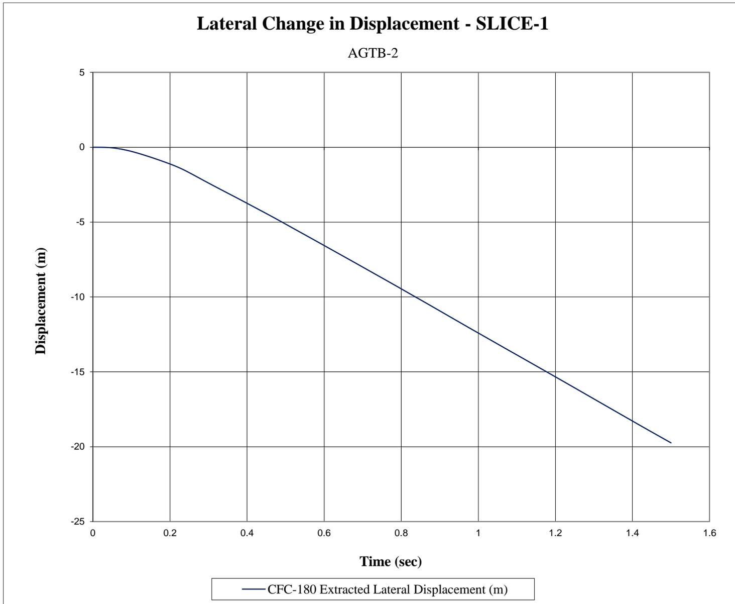
Figure F-6. Lateral Occupant Displacement (SLICE-1), Test No. AGTB-2
