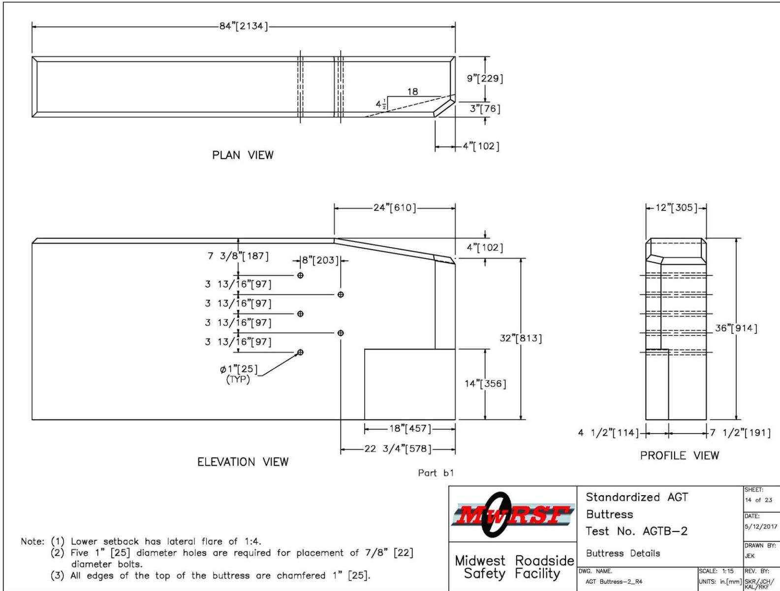
Figure 61. Buttress Details, Test No. AGTB-2
