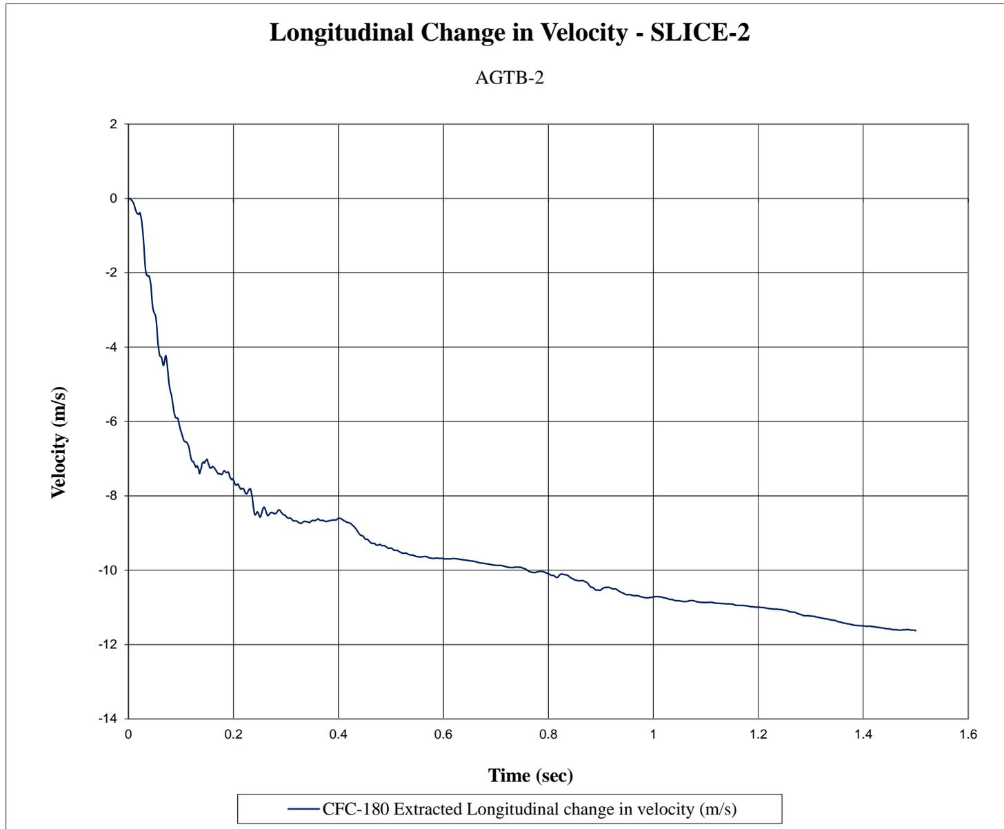
Figure F-10. Longitudinal Occupant Impact Velocity (SLICE-2), Test No. AGTB-2
