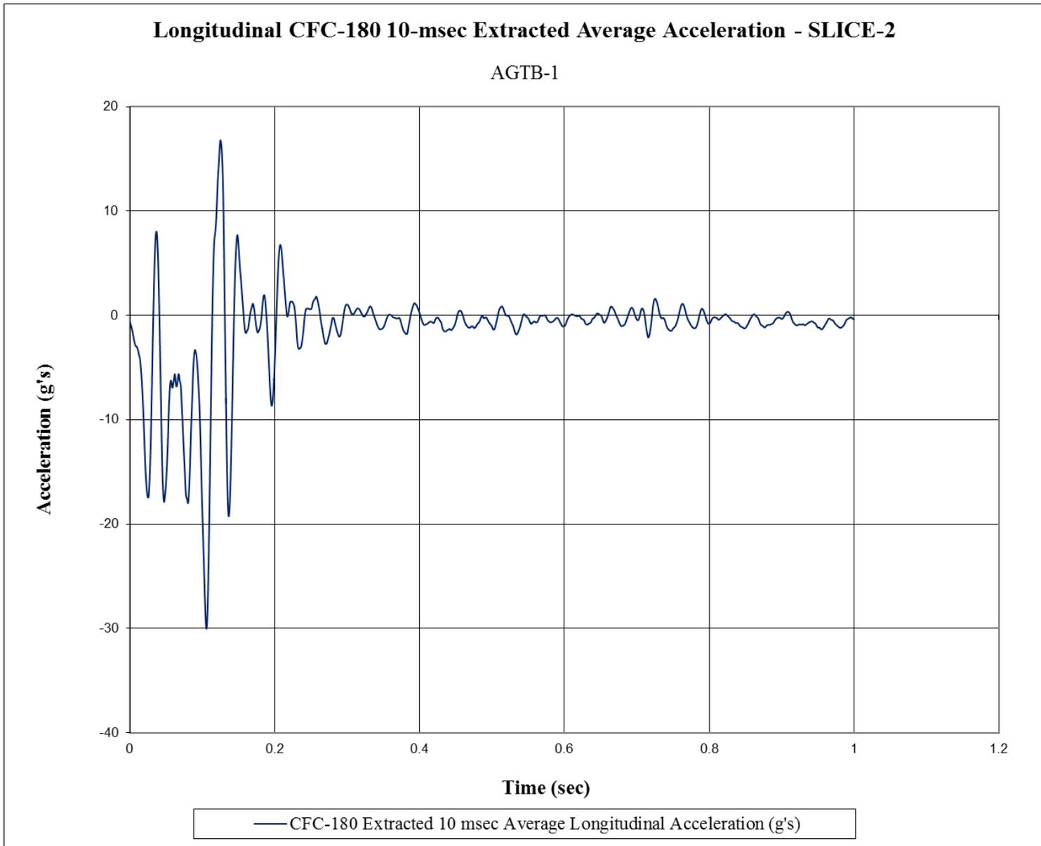
Figure E-9. 10-ms Average Longitudinal Deceleration (SLICE-2), Test No. AGTB-1
