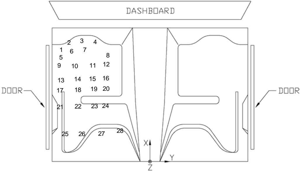
Figure D-2. Floor Pan Deformation Data – Set 2, Test No. AGTB-1
