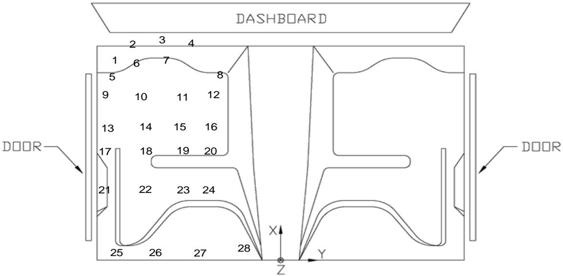
Figure D-1. Floor Pan Deformation Data – Set 1, Test No. AGTB-1
