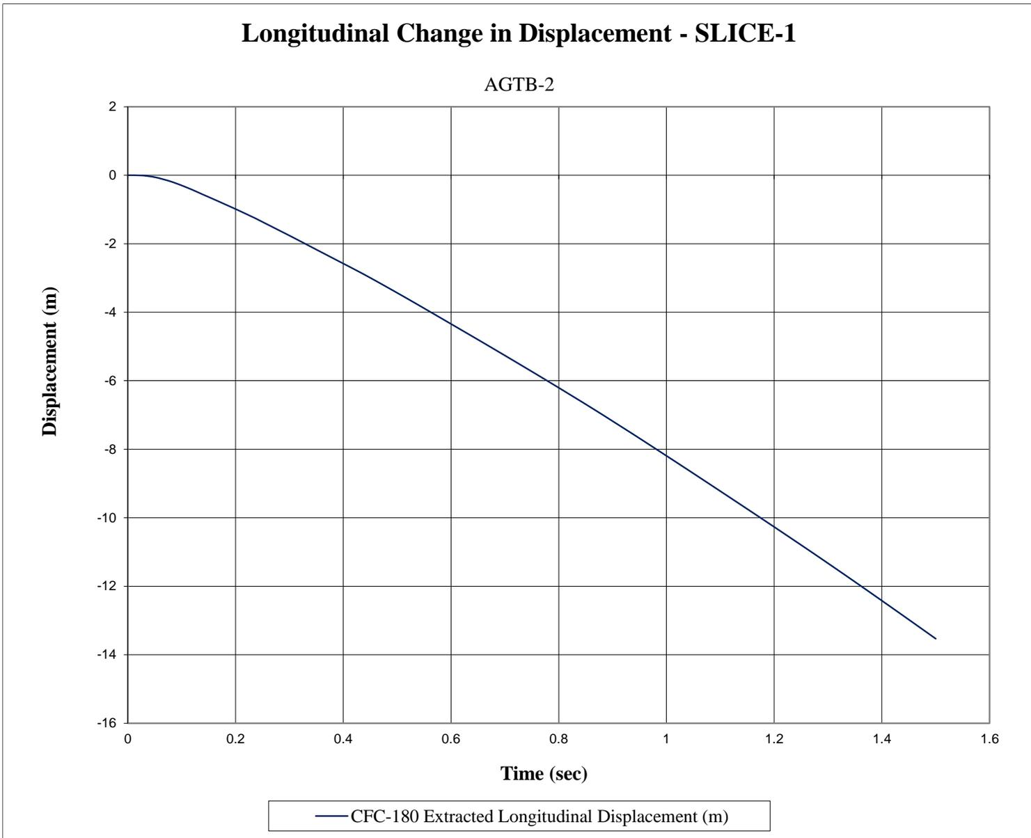
Figure F-3. Longitudinal Occupant Displacement (SLICE-1), Test No. AGTB-2
