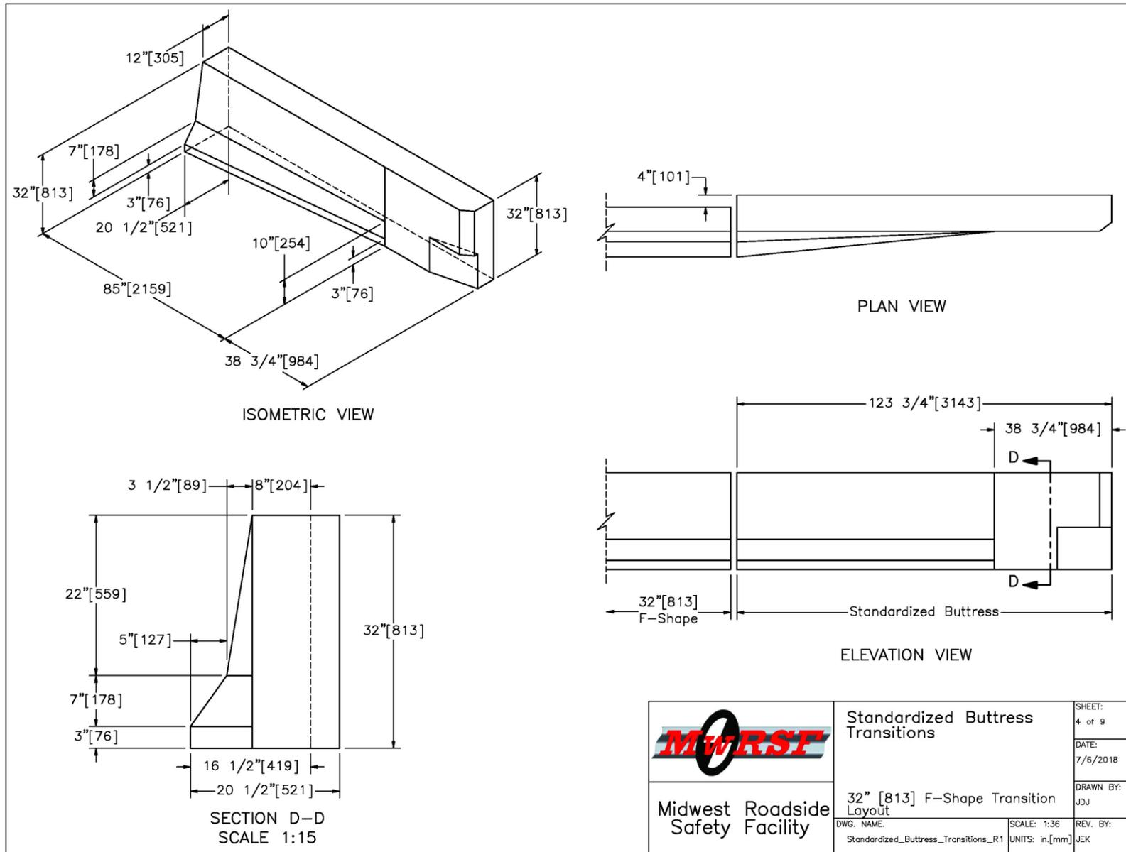
Figure 89. Buttress Shape Transition to 32-in. Tall F-Shape Barrier
