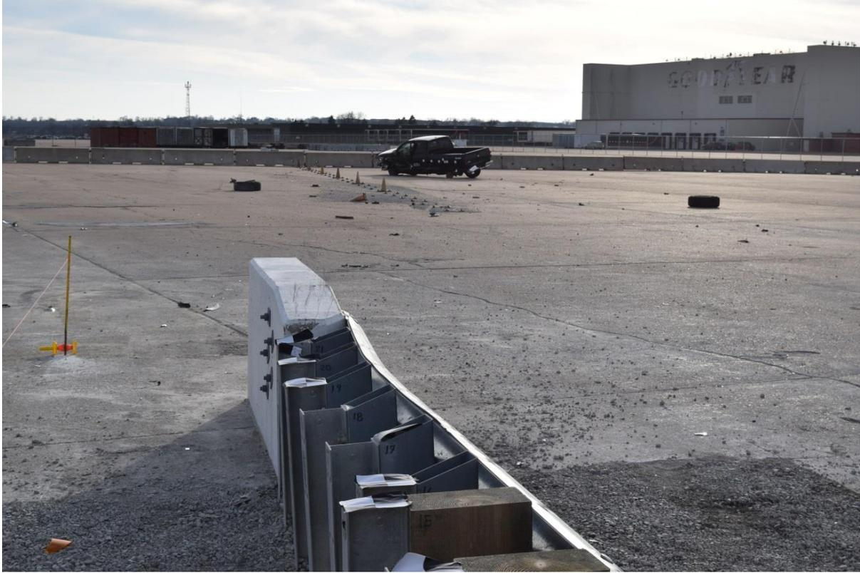
Figure 40. Vehicle Final Position and Trajectory Marks, Test No. AGTB-1
