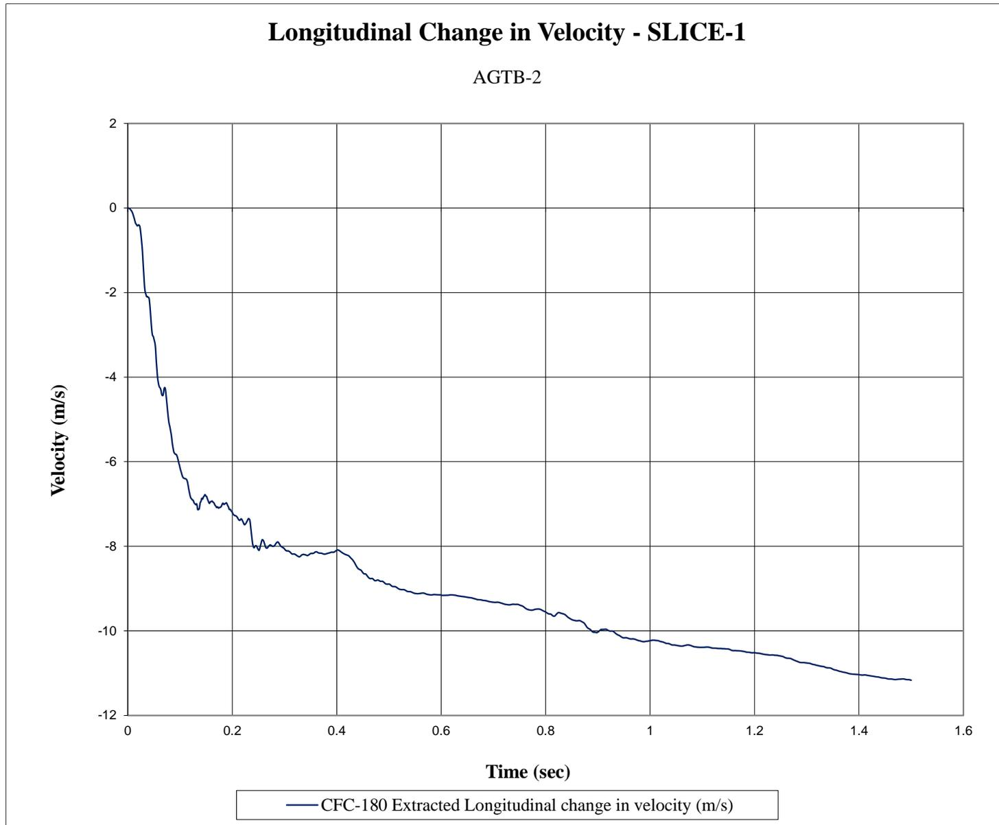
Figure F-2. Longitudinal Occupant Impact Velocity (SLICE-1), Test No. AGTB-2
