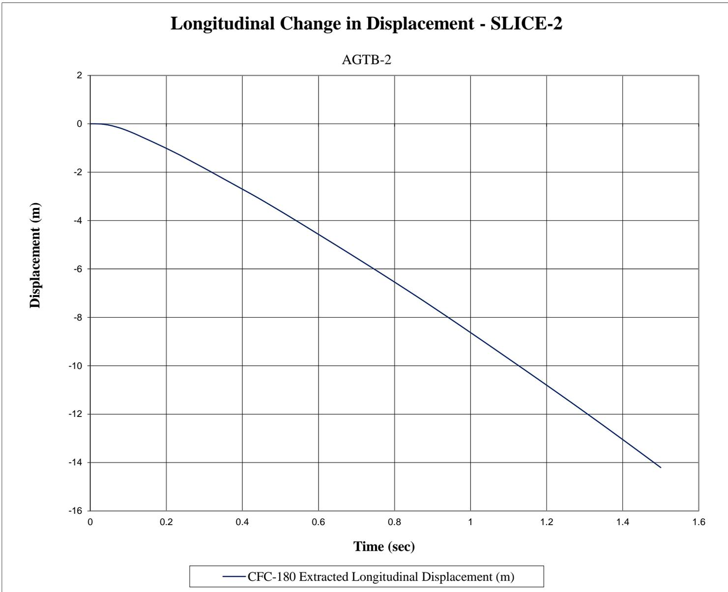
Figure F-11. Longitudinal Occupant Displacement (SLICE-2), Test No. AGTB-2
