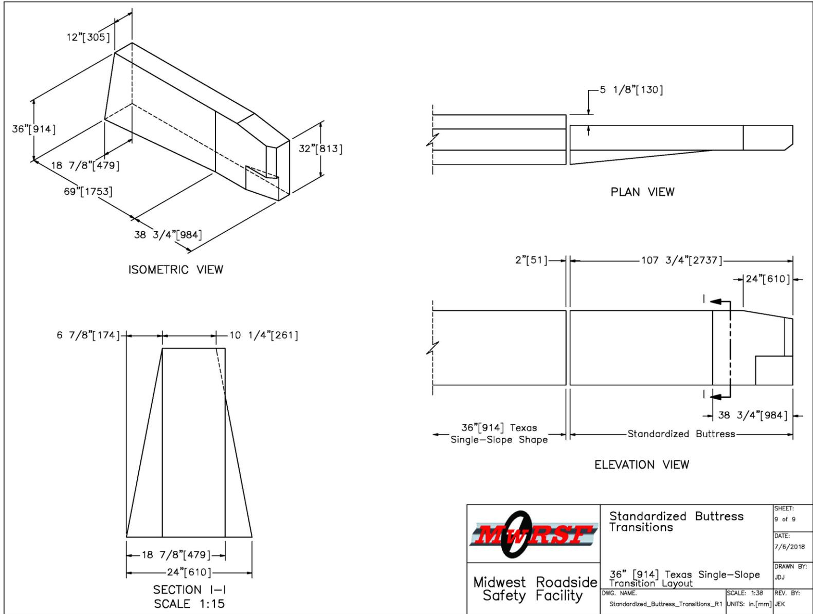
Figure 94. Buttress Shape Transition to 36-in. Tall Texas Single Slope Barrier
