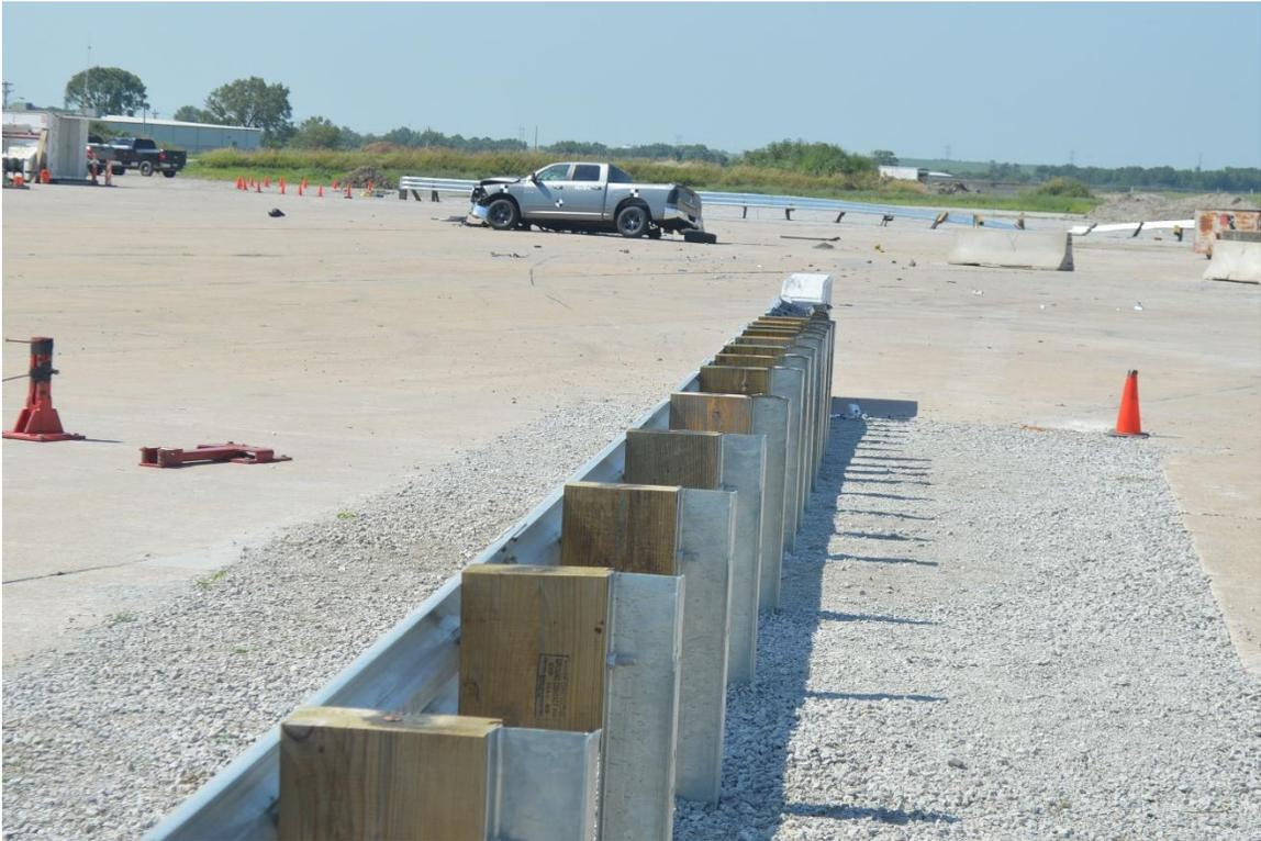
Figure 75. Vehicle Final Position and Trajectory Marks, Test No. AGTB-2
