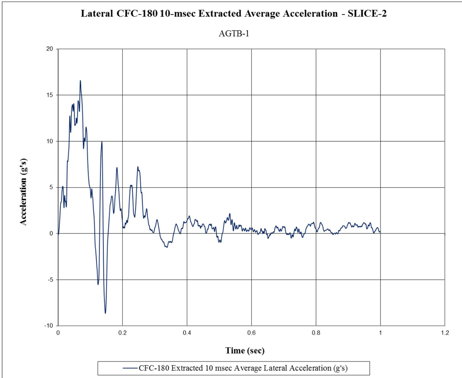
Figure E-12. 10-ms Average Lateral Deceleration (SLICE-2), Test No. AGTB-1
