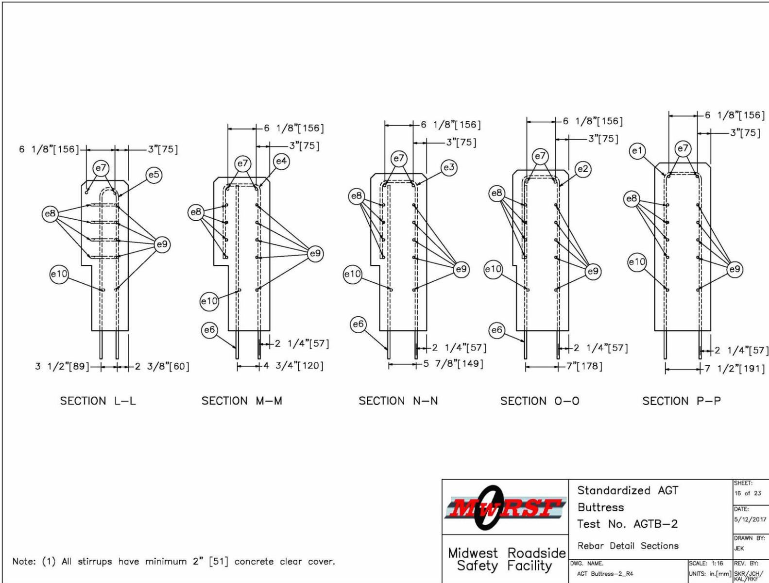
Figure 63. Rebar Detail Sections, Test No. AGTB-2
