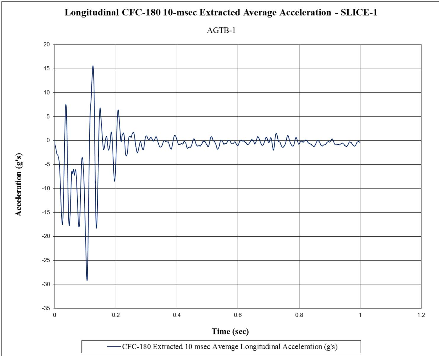
Figure E-1. 10-ms Average Longitudinal Deceleration (SLICE-1), Test No. AGTB-1
