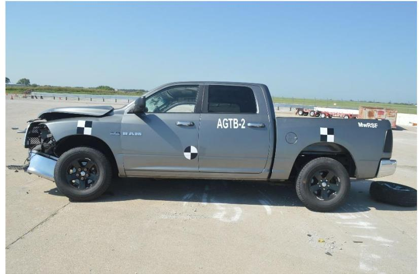
Figure 80. Vehicle Damage, Test No. AGTB-2
