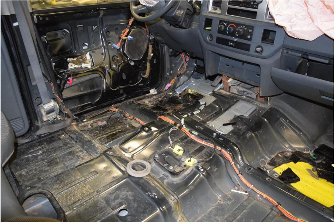
Figure 46. Vehicle Occupant Compartment Damage, Test No. AGTB-1
