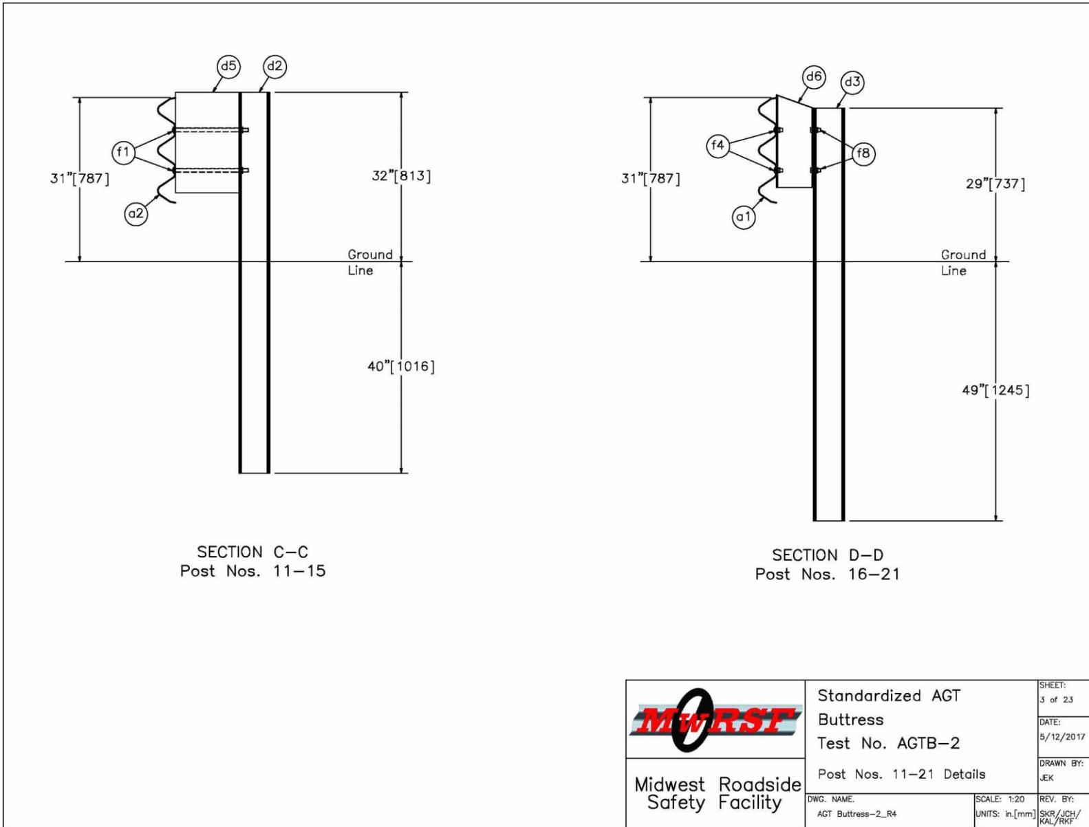
Figure 50. Post Nos. 11 through 21 Details, Test No. AGTB-2
