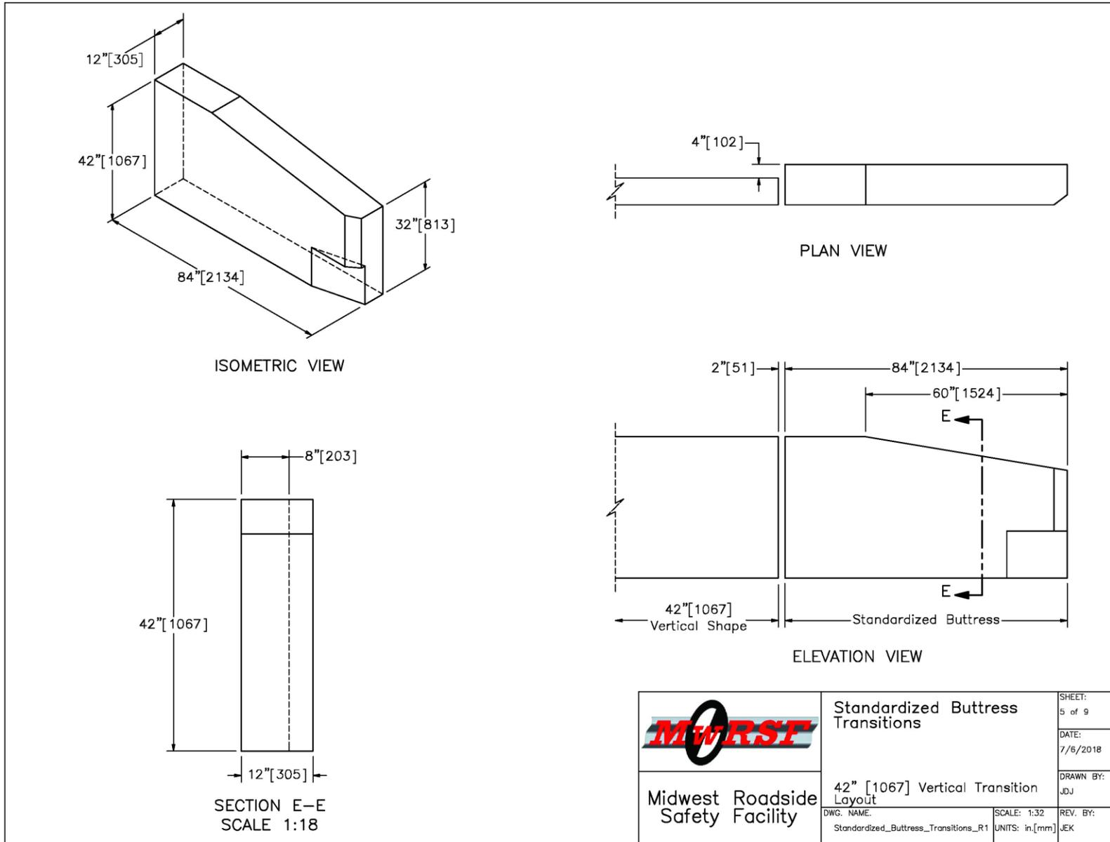
Figure 90. Buttress Shape Transition to 42-in. Tall Vertical Barrier
