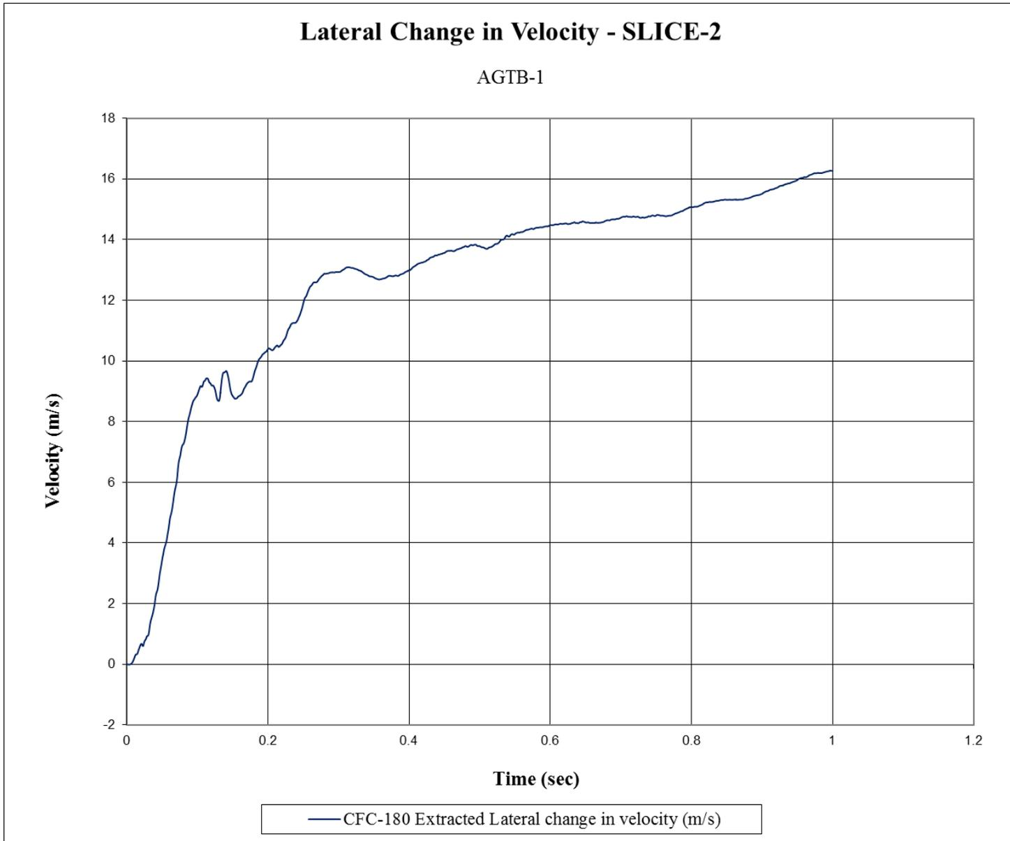
Figure E-13. Lateral Occupant Impact Velocity (SLICE-2), Test No. AGTB-1
