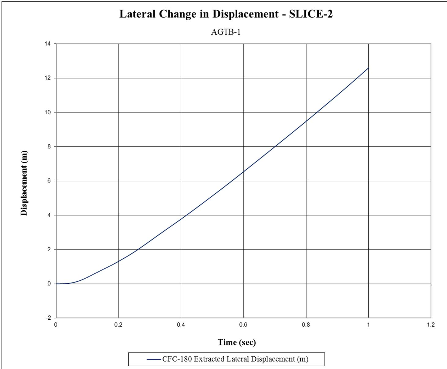
Figure E-14. Lateral Occupant Displacement (SLICE-2), Test No. AGTB-1
