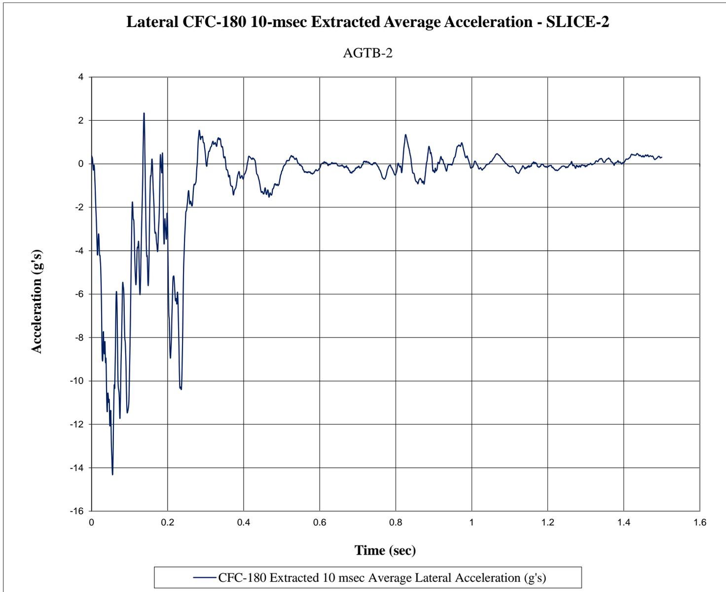
Figure F-12. 10-ms Average Lateral Deceleration (SLICE-2), Test No. AGTB-2
