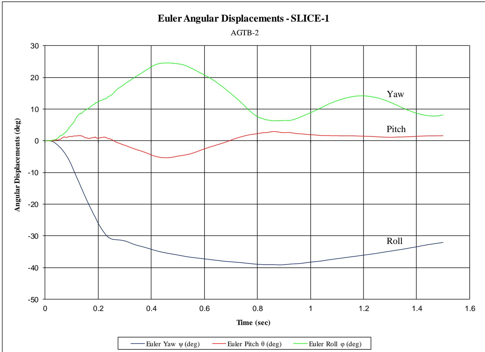
Figure F-7. Vehicle Angular Displacements (SLICE-1), Test No. AGTB-2
