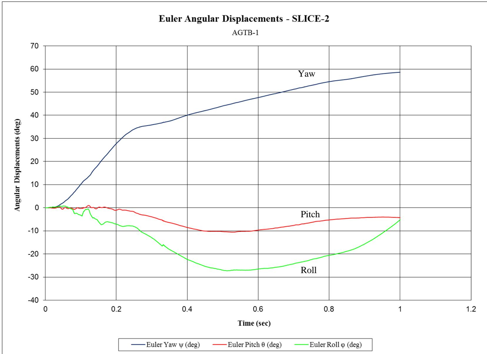
Figure E-15. Vehicle Angular Displacements (SLICE-2), Test No. AGTB-1
