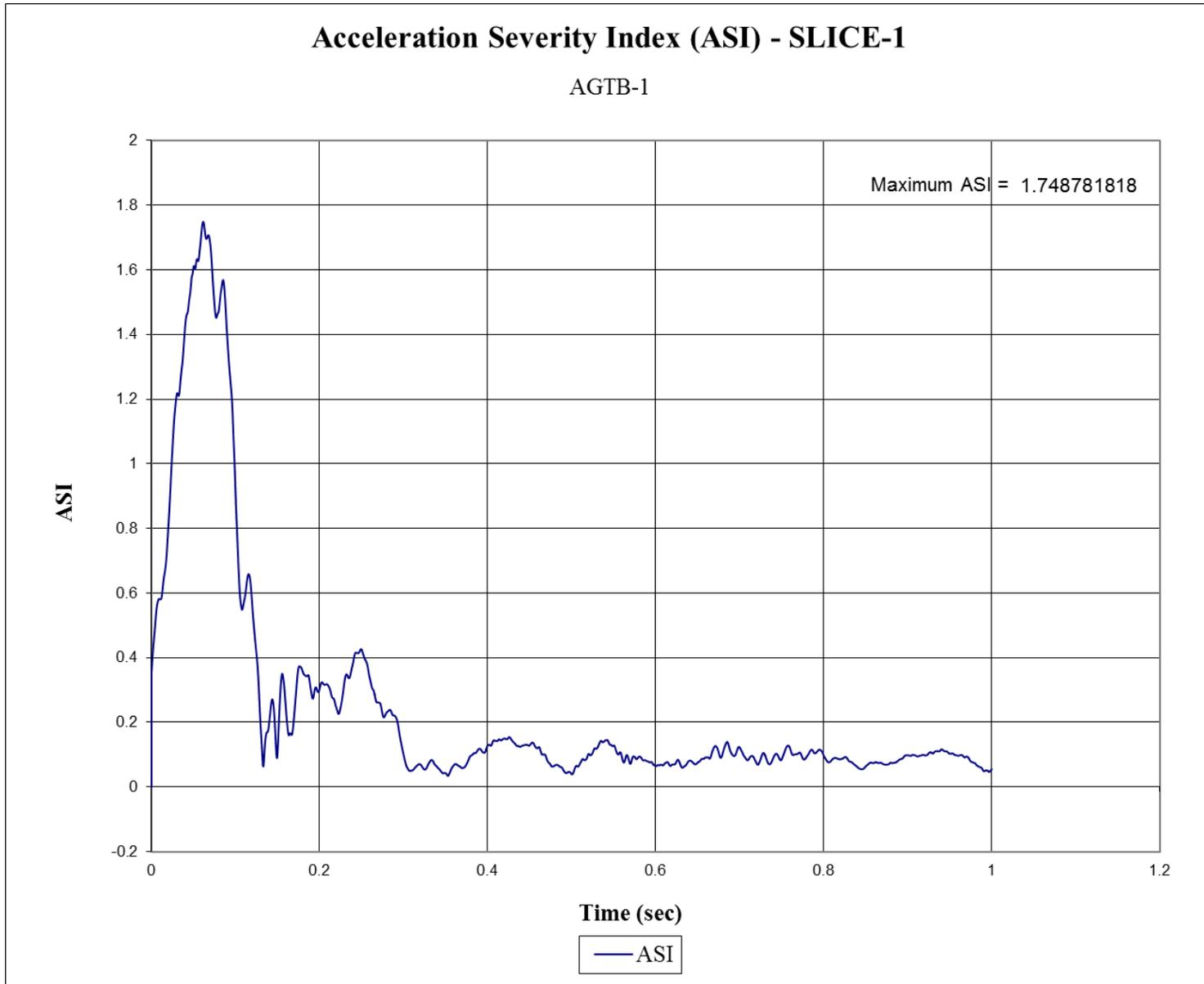
Figure E-8. Acceleration Severity Index (SLICE-1), Test No. AGTB-1
