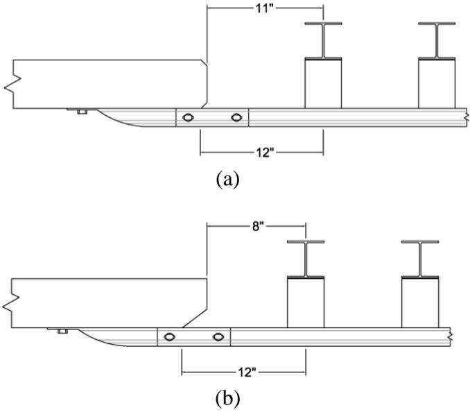
Figure 2. Buttruss to Transition Offset: (a) Original As-tested AGT and (b) AGT in Combination with the Standardized Buttruss
