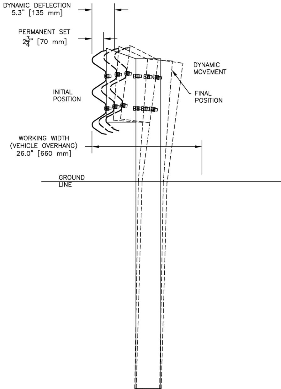
Figure 79. Permanent Set Deflection, Dynamic Deflection, and Working Width, Test No. AGTB-2
