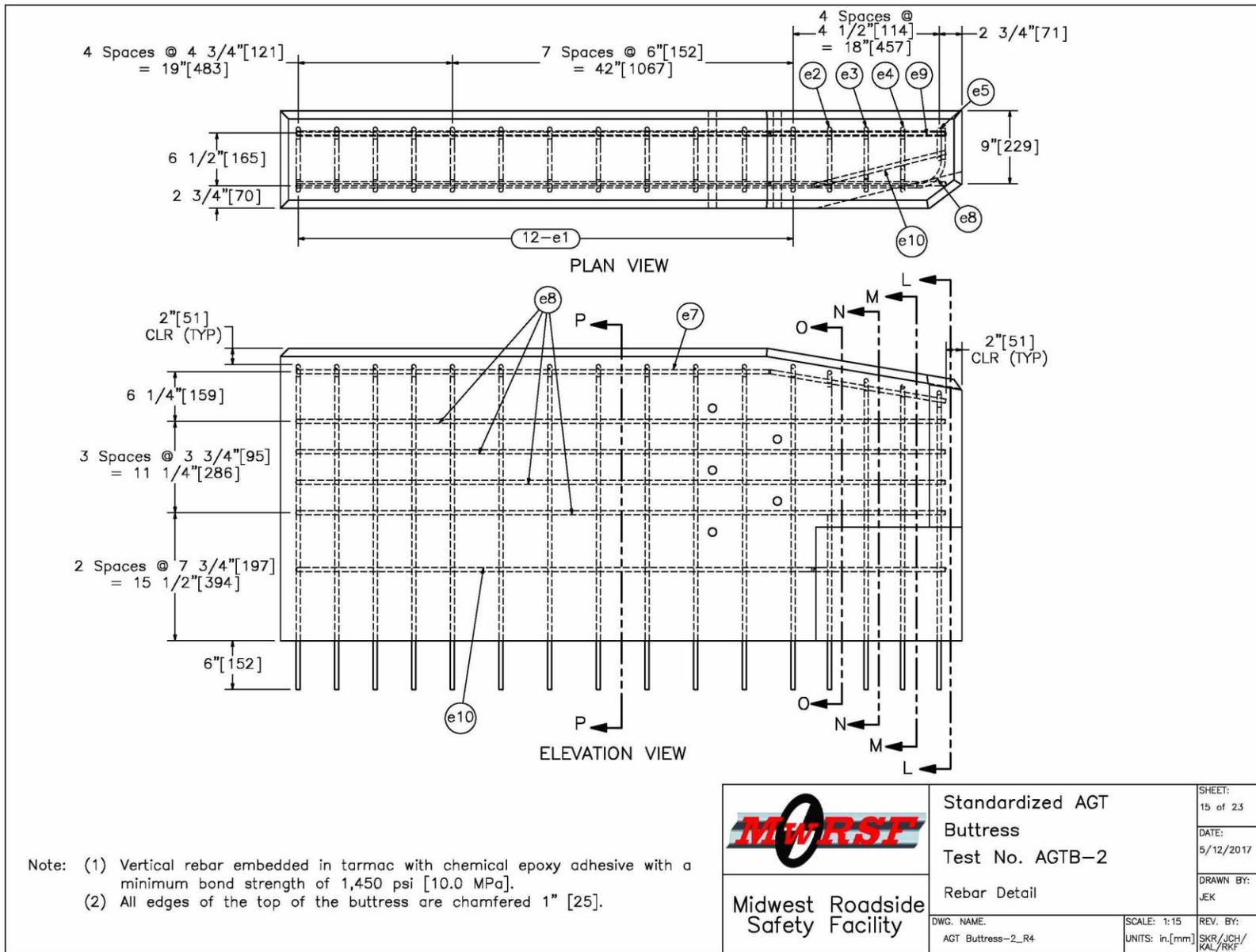
Figure 62. Rebar Detail, Test No. AGTB-2
