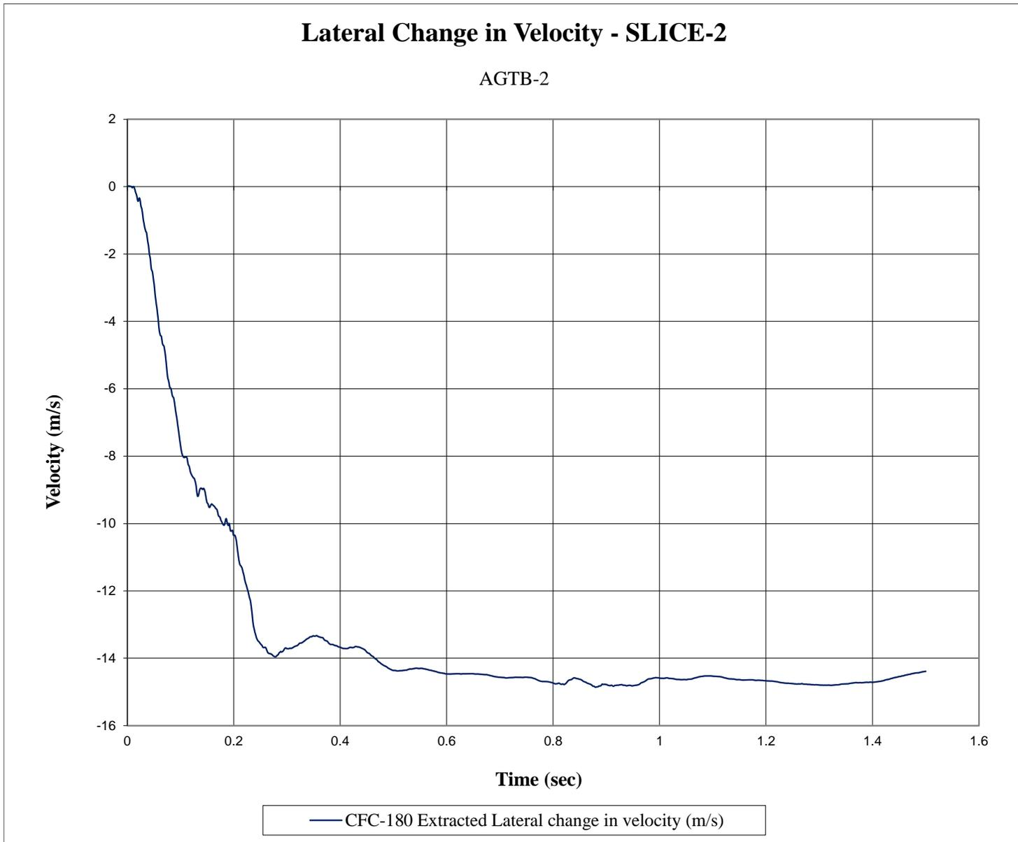
Figure F-13. Lateral Occupant Impact Velocity (SLICE-2), Test No. AGTB-2
