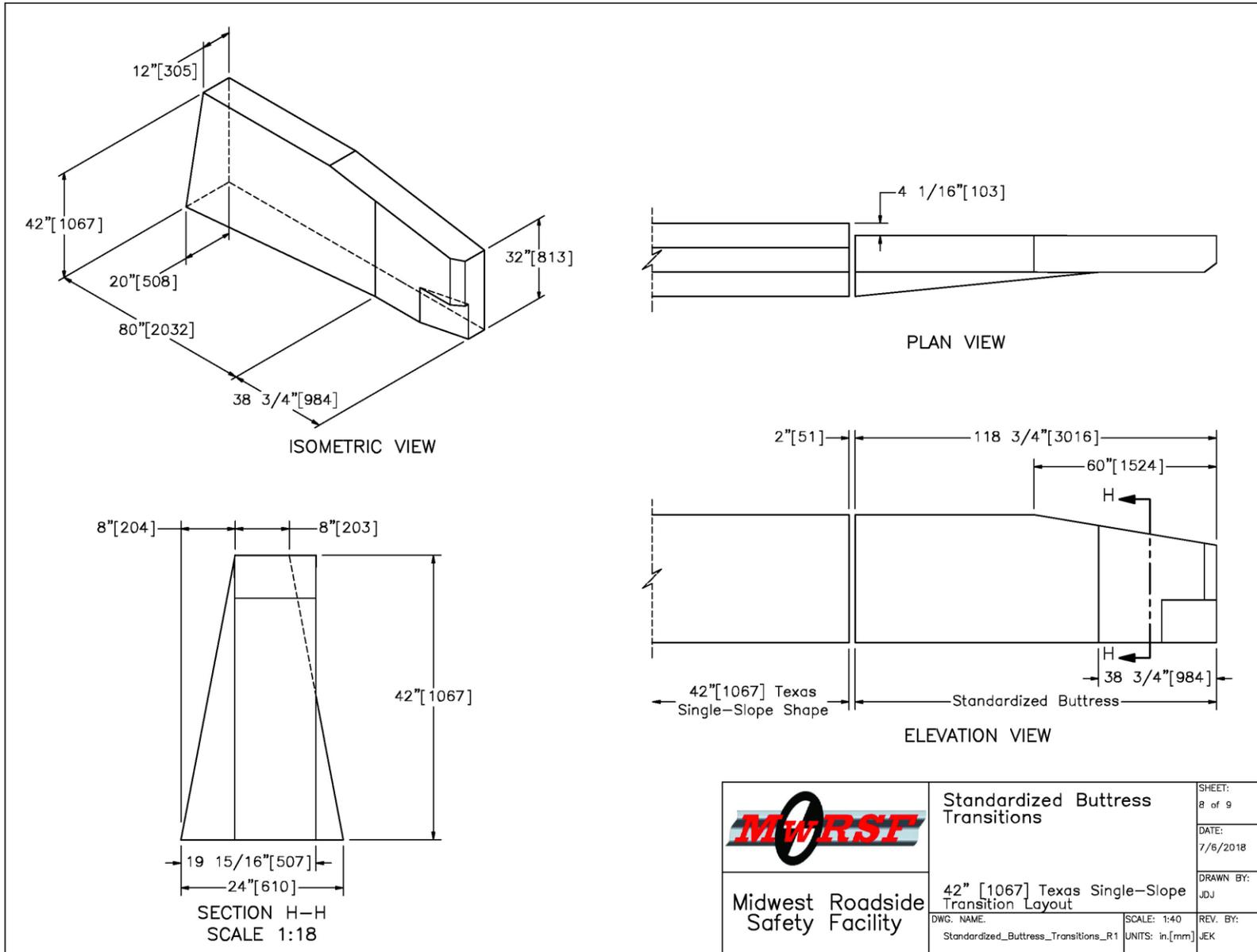
Figure 93. Buttress Shape Transition to 42-in. Tall Texas Single Slope Barrier
