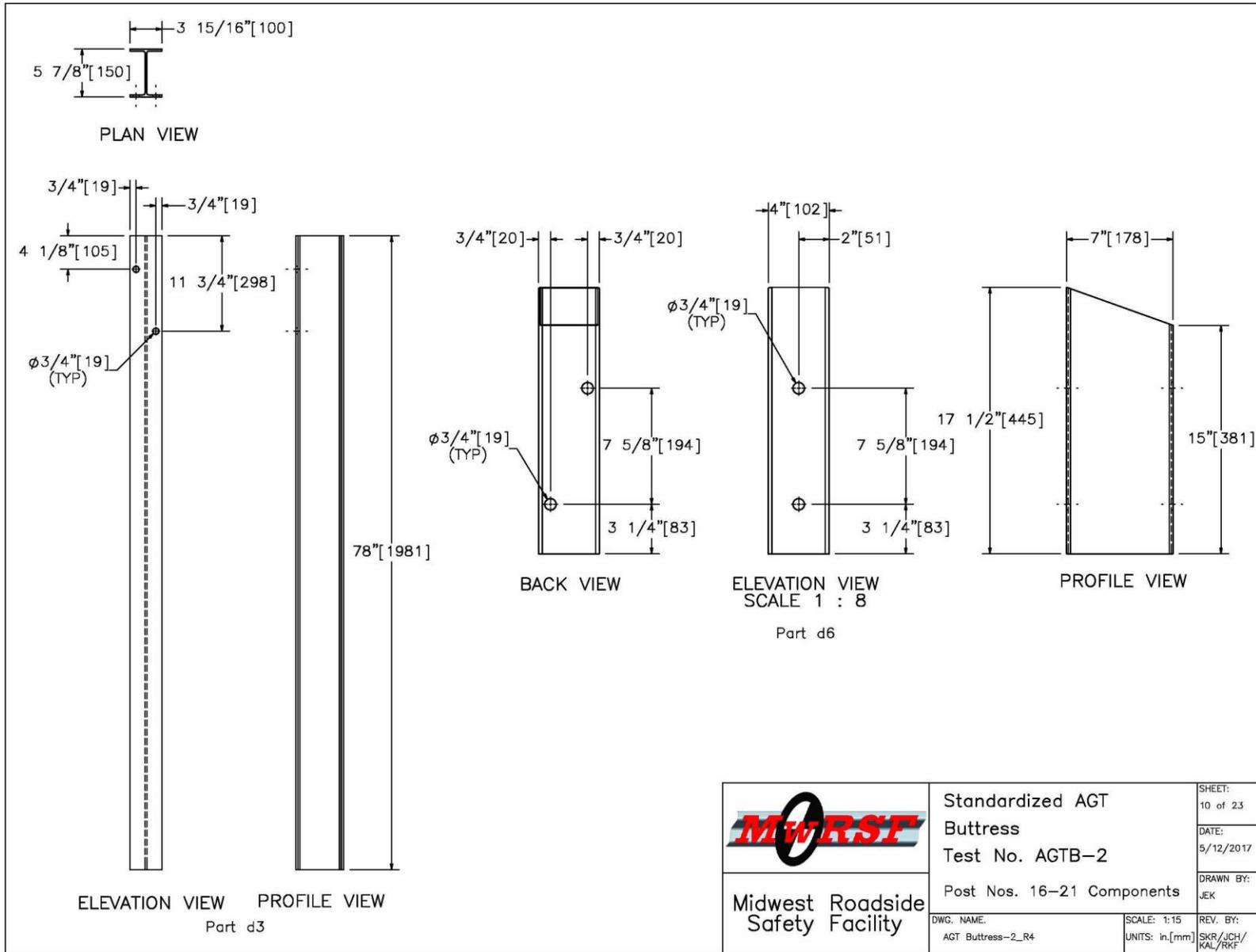
Figure 57. Post Nos. 16 through 21 Components, Test No. AGTB-2
