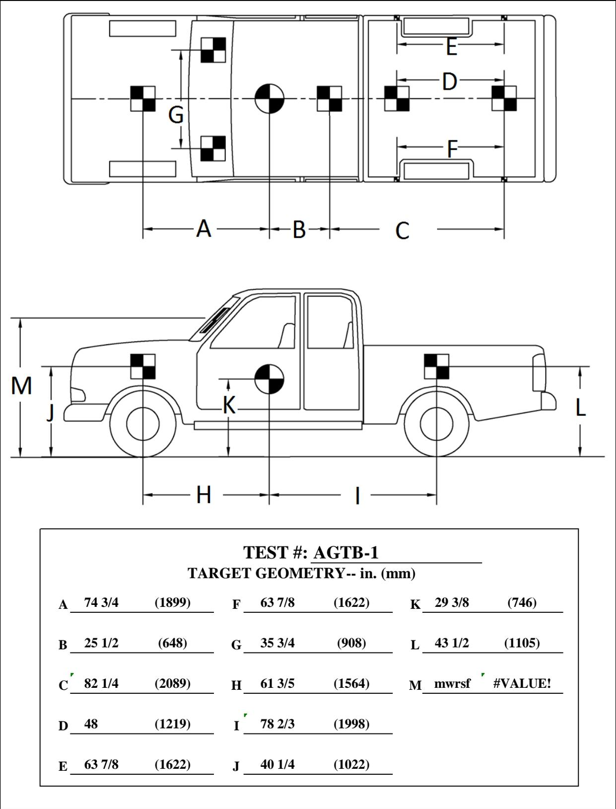
Figure 32. Target Geometry, Test No. AGTB-1
