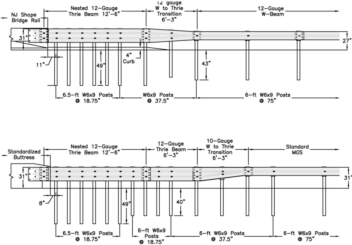
Figure 3. Selected AGT Design in its (a) Original, As-Tested Configuration and (b) Critical Configuration for Evaluating the Standardized Buttruss
