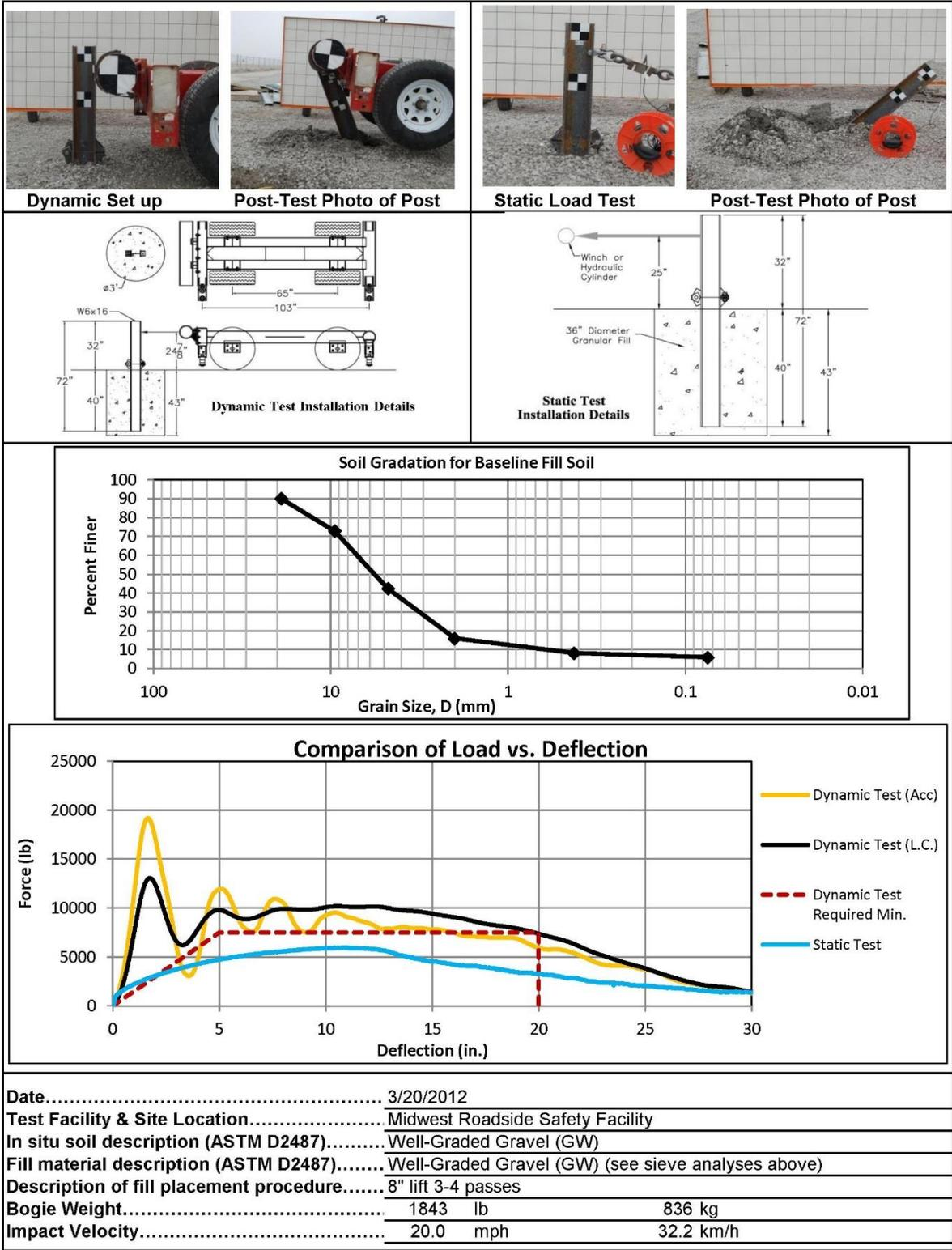
Figure C-3. Soil Strength, Initial Calibration Tests, Test No. AGTB-2
