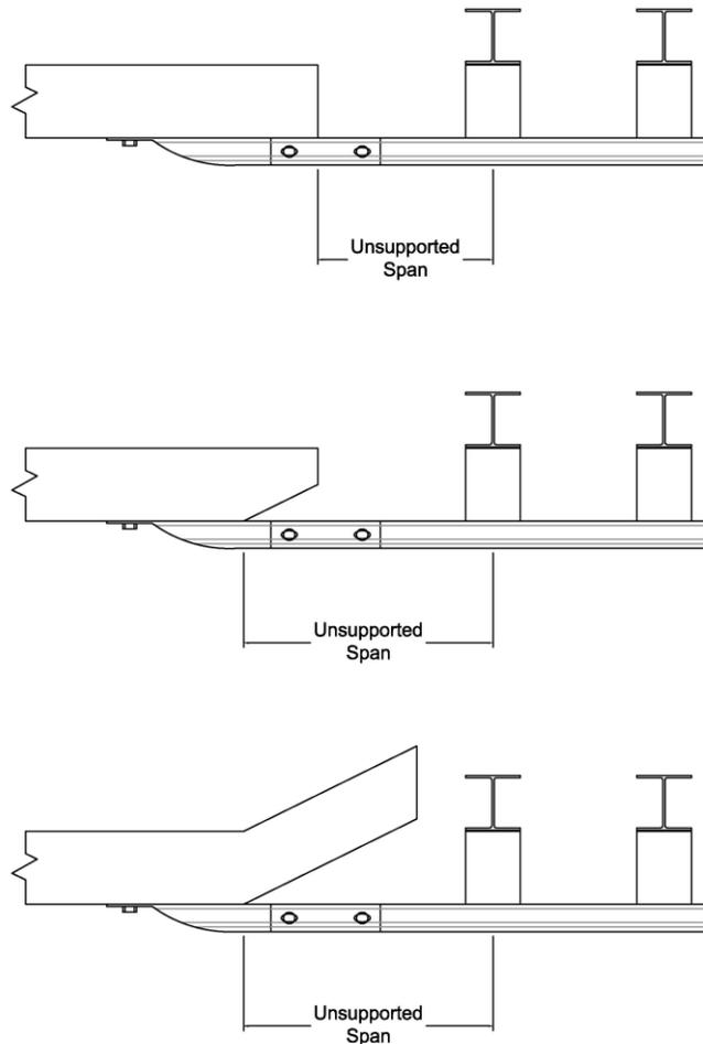
Figure 84. Examples of Unsupported Span Lengths for Various AGT Configurations
