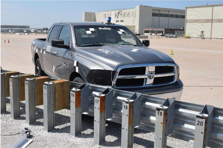
Figure 72. Impact Location, Test No. AGTB-2
