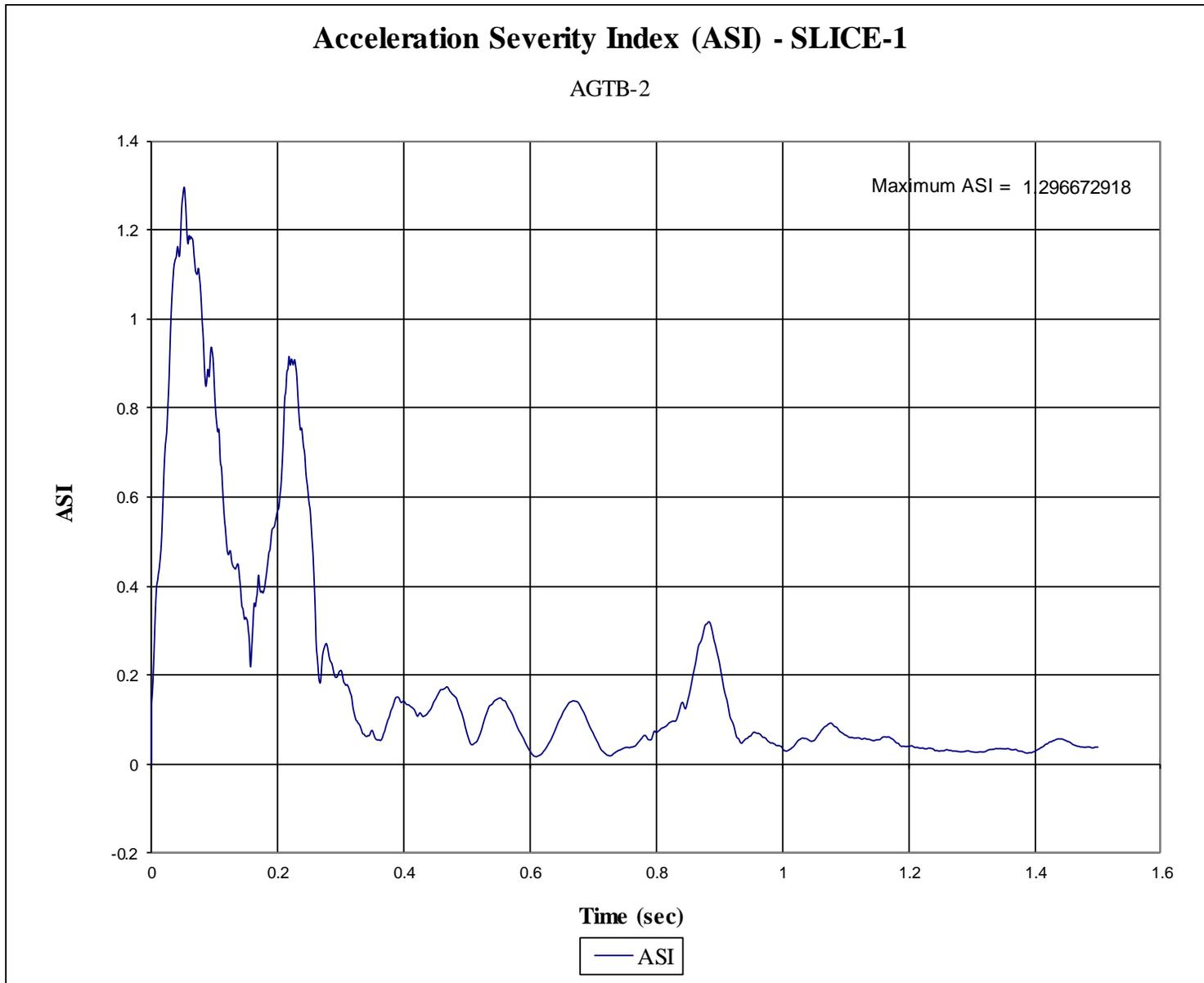
Figure F-8. Acceleration Severity Index (SLICE-1), Test No. AGTB-2
