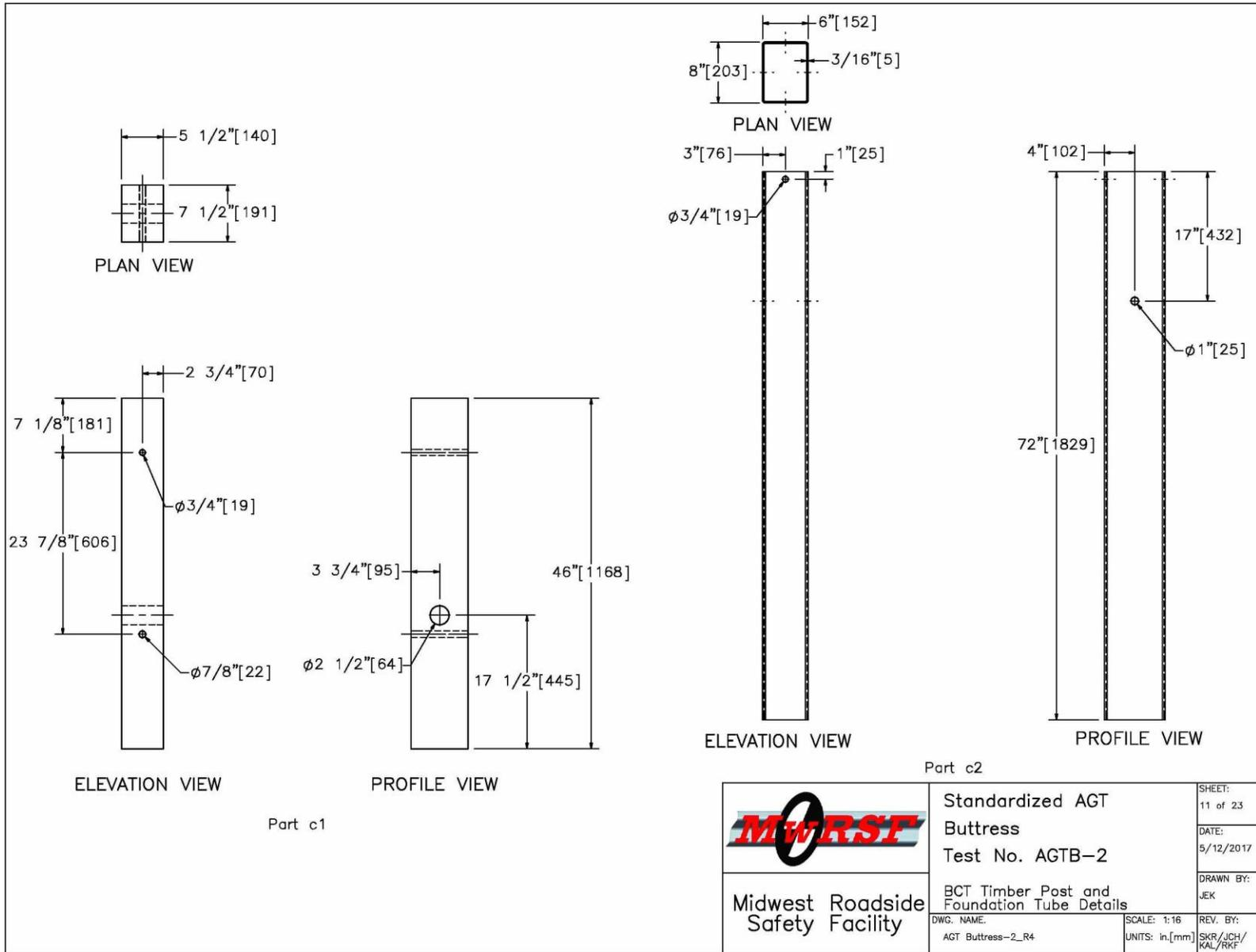
Figure 58. BCT Timber Post and Foundation Tube Details, Test No. AGTB-2
