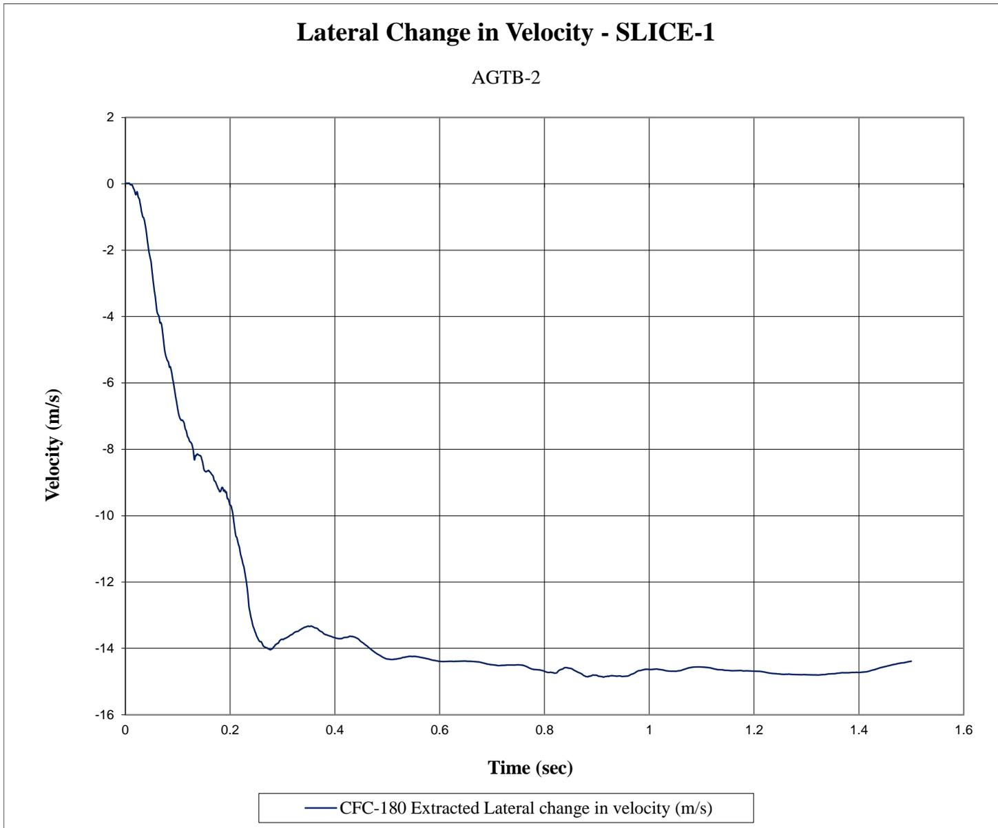
Figure F-5. Lateral Occupant Impact Velocity (SLICE-1), Test No. AGTB-2
