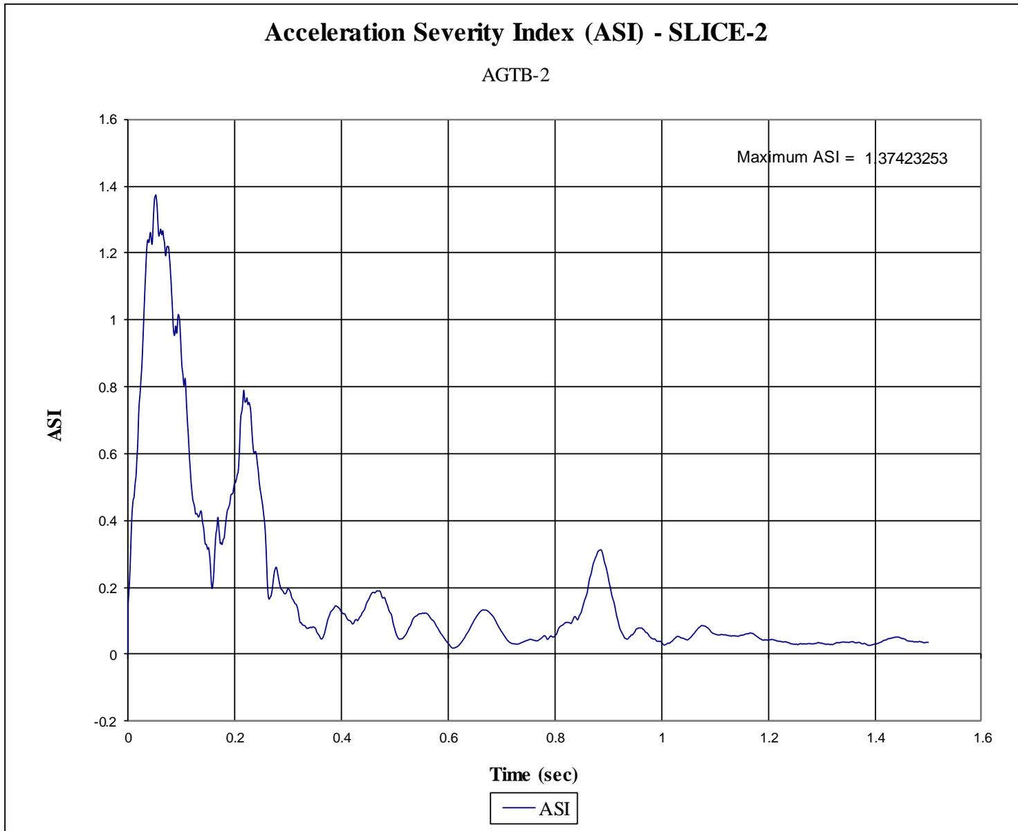
Figure F-16. Acceleration Severity Index (SLICE-2), Test No. AGTB-2
