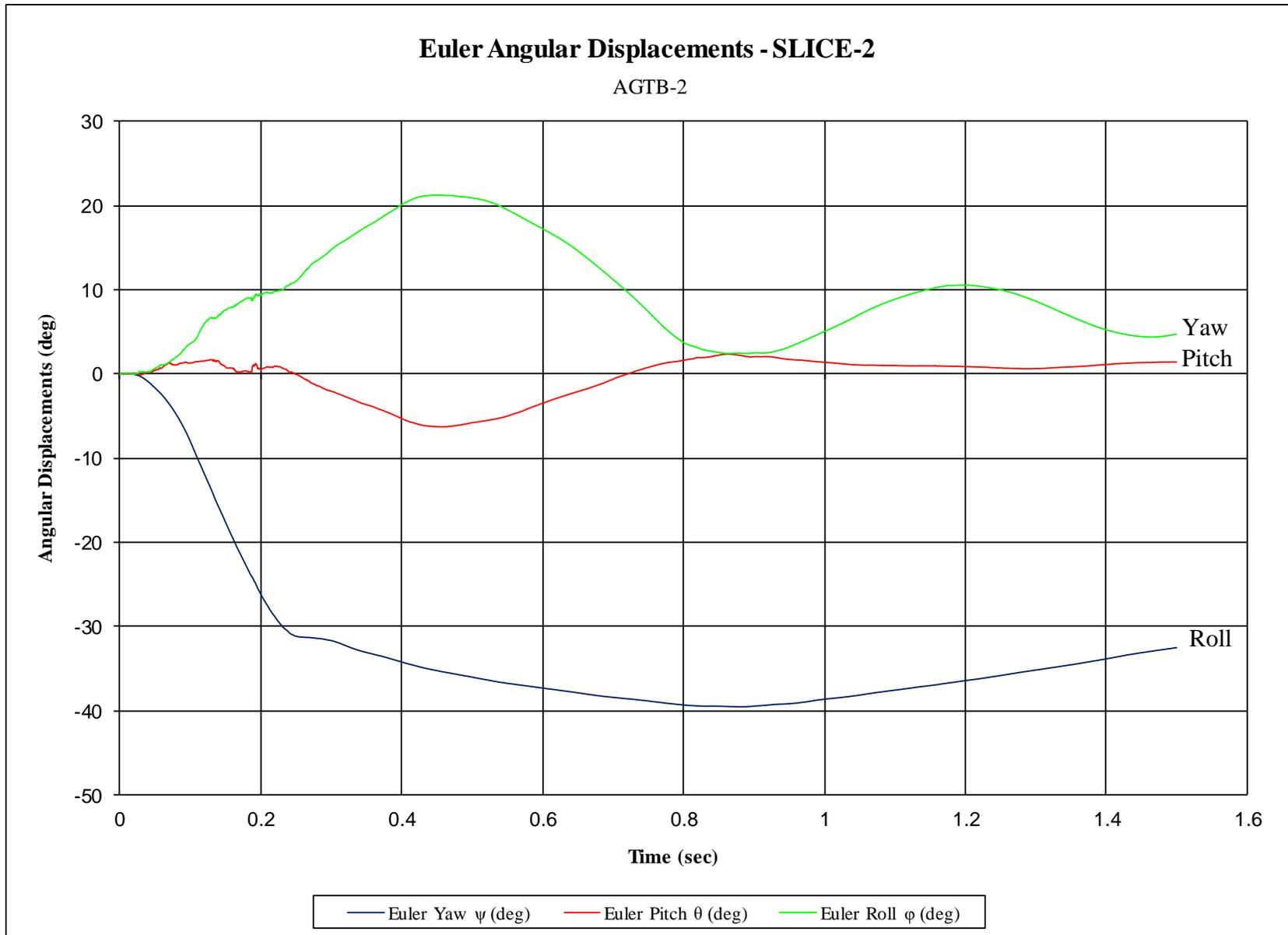
Figure F-15. Vehicle Angular Displacements (SLICE-2), Test No. AGTB-2
