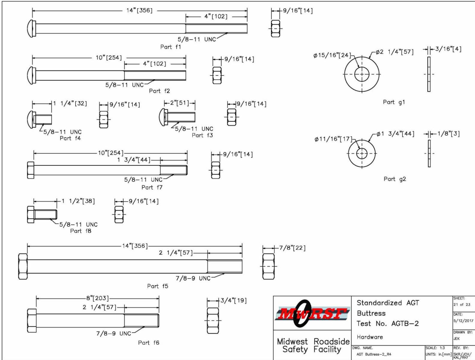
Figure 68. Hardware, Test No. AGTB-2
