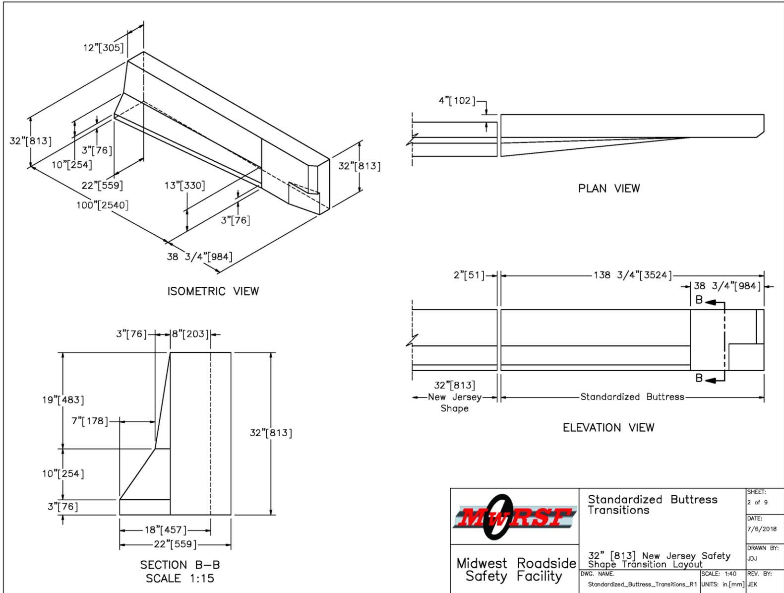
Figure 87. Buttress Shape Transition to 32-in. Tall NJ Shape Barrier
