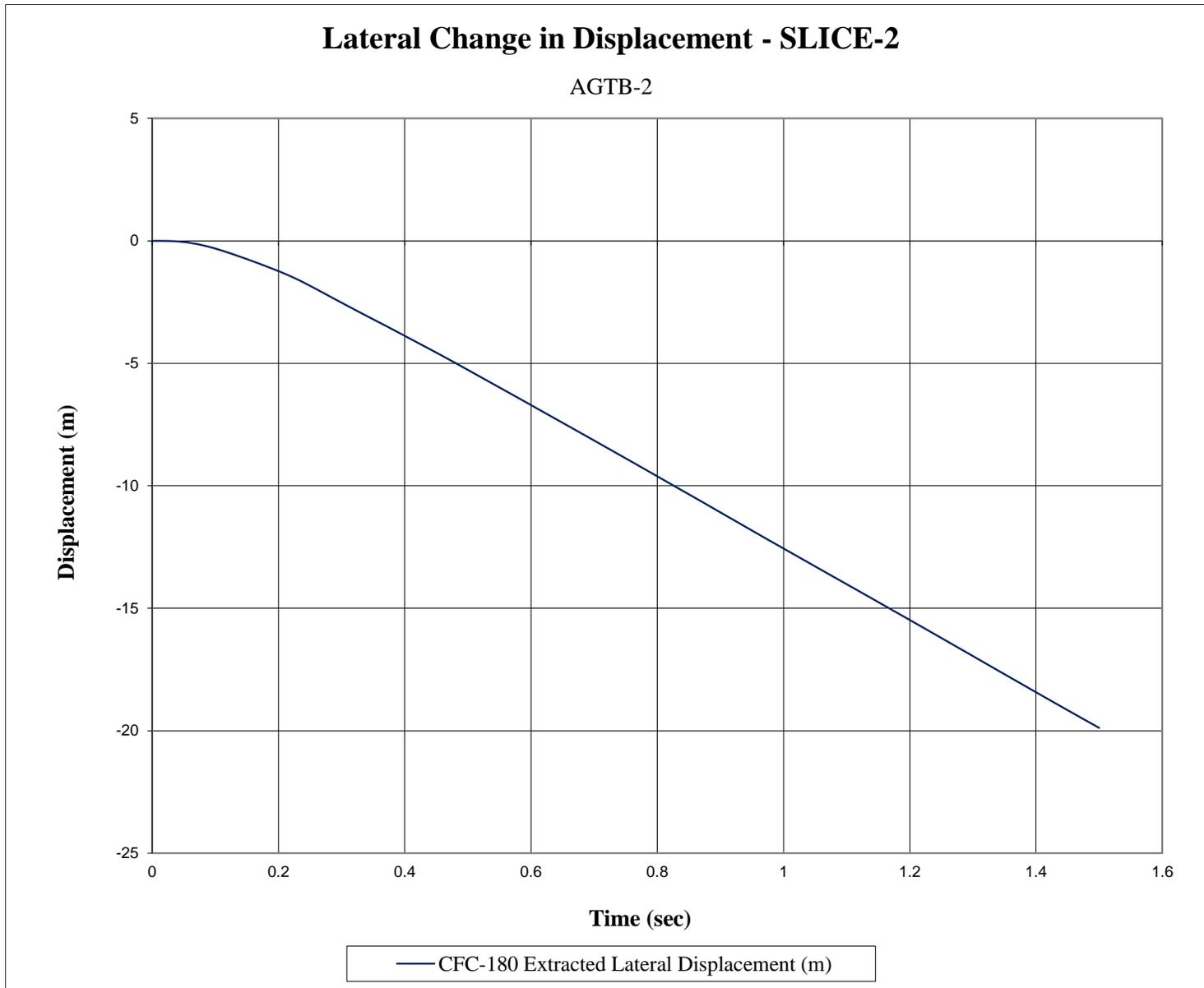
Figure F-14. Lateral Occupant Displacement (SLICE-2), Test No. AGTB-2
