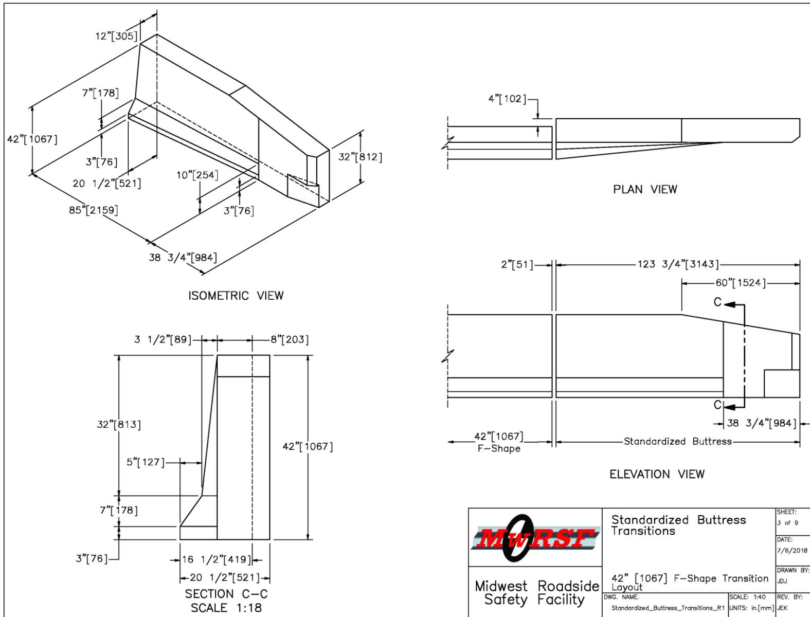
Figure 88. Buttress Shape Transition to 42-in. Tall F-Shape Barrier
