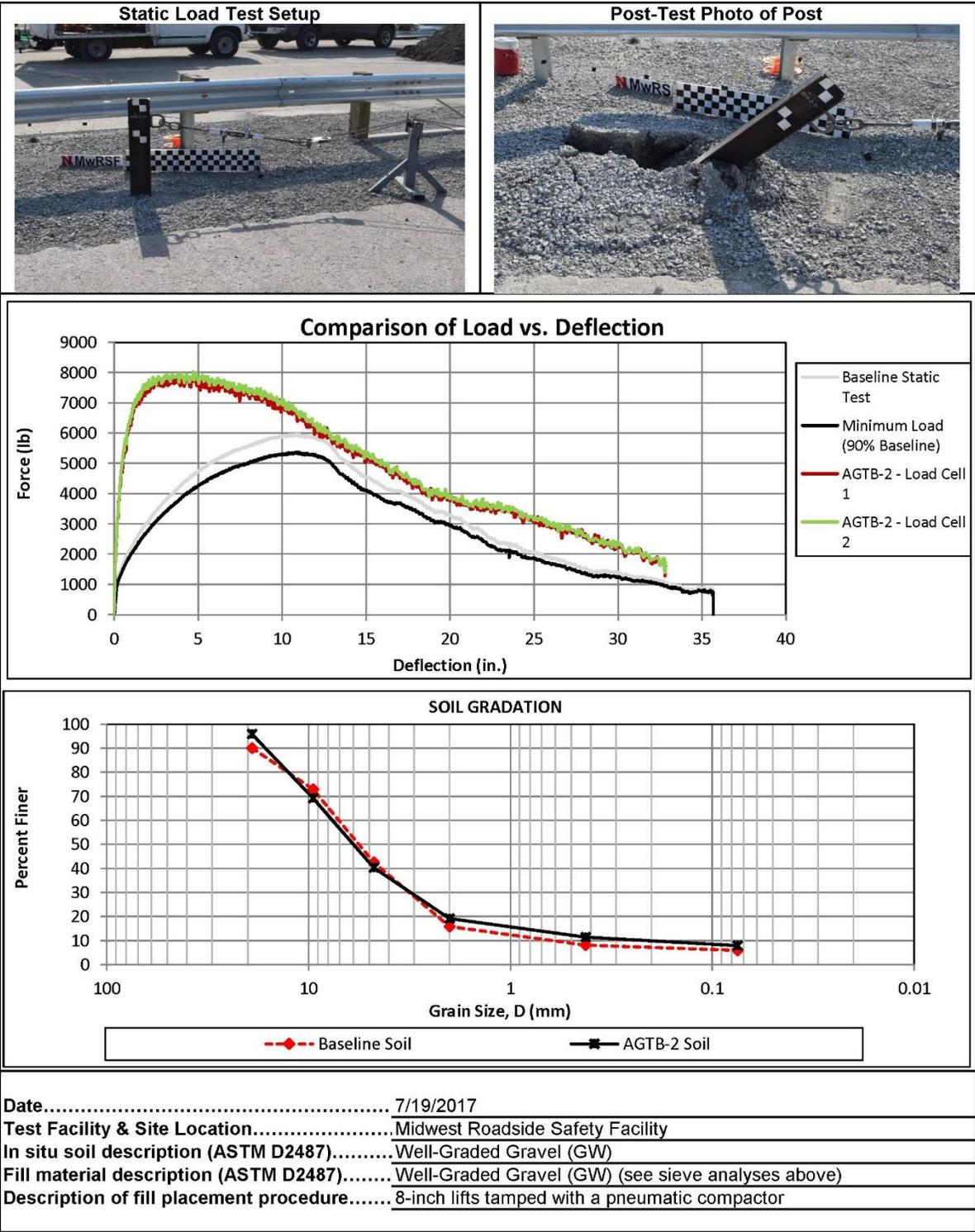
Figure C-4. Soil Strength Test, Test No. AGTB-2
