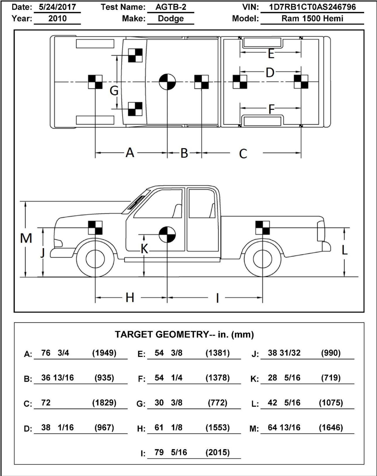
Figure 33. Target Geometry, Test No. AGTB-2
