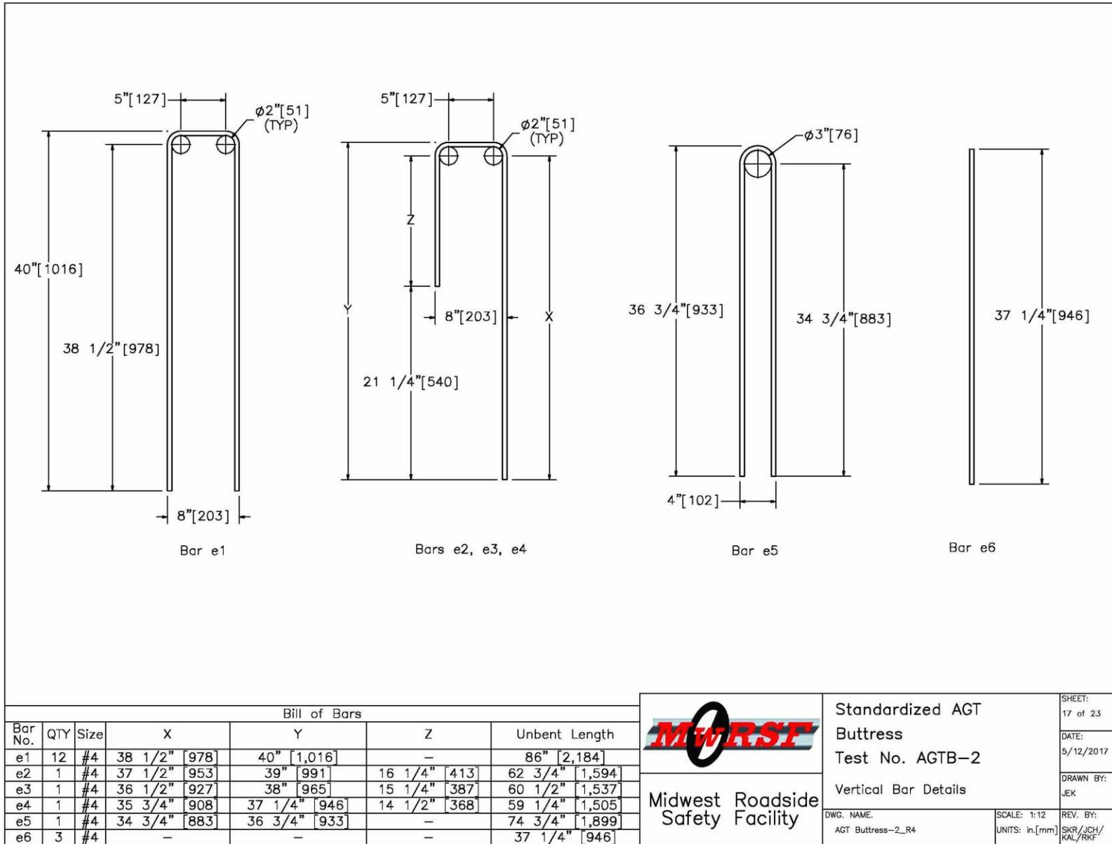
Figure 64. Vertical Bar Details, Test No. AGTB-2
