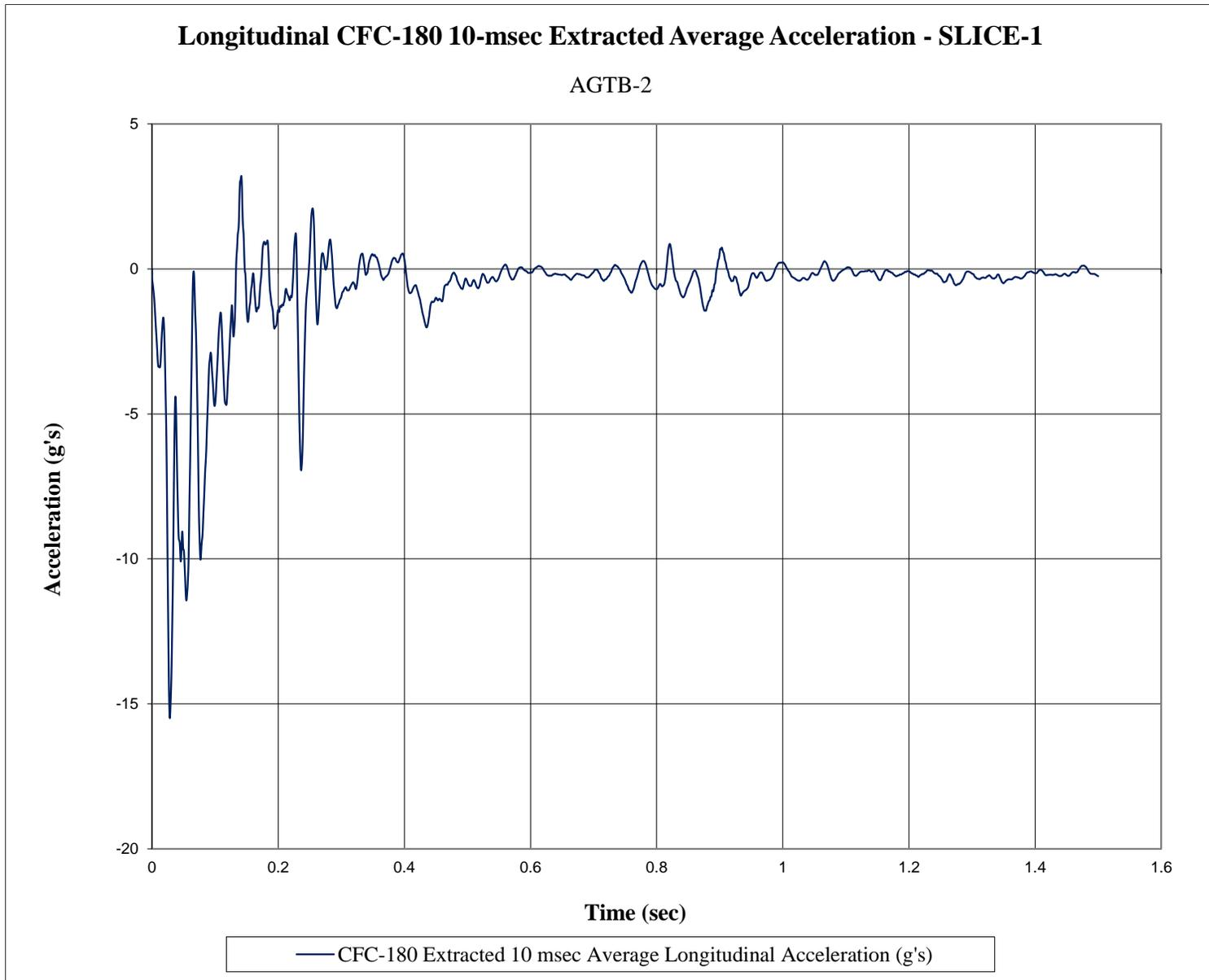
Figure F-1. 10-ms Average Longitudinal Deceleration (SLICE-1), Test No. AGTB-2
