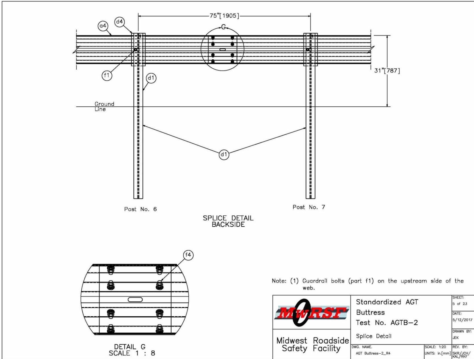
Figure 52. Splice Detail, Test No. AGTB-2
