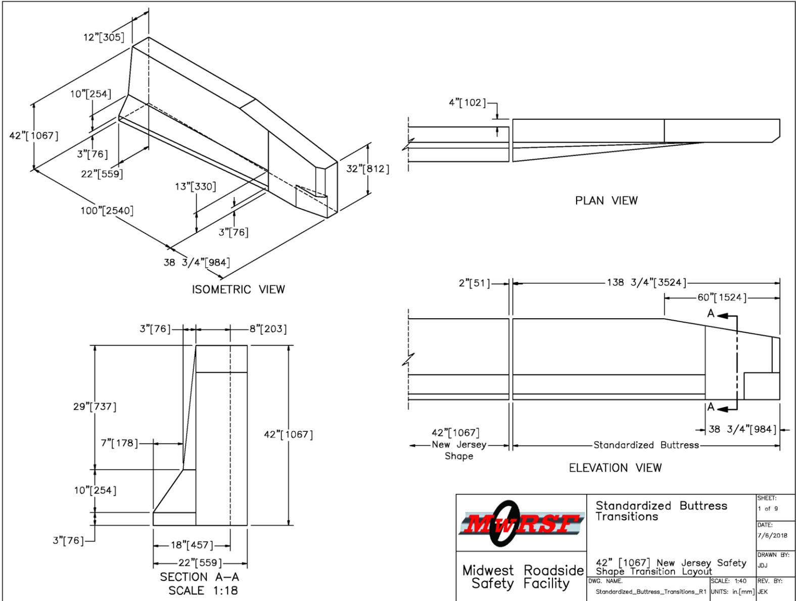
Figure 86. Buttress Shape Transition to 42-in. Tall NJ Shape Barrier
