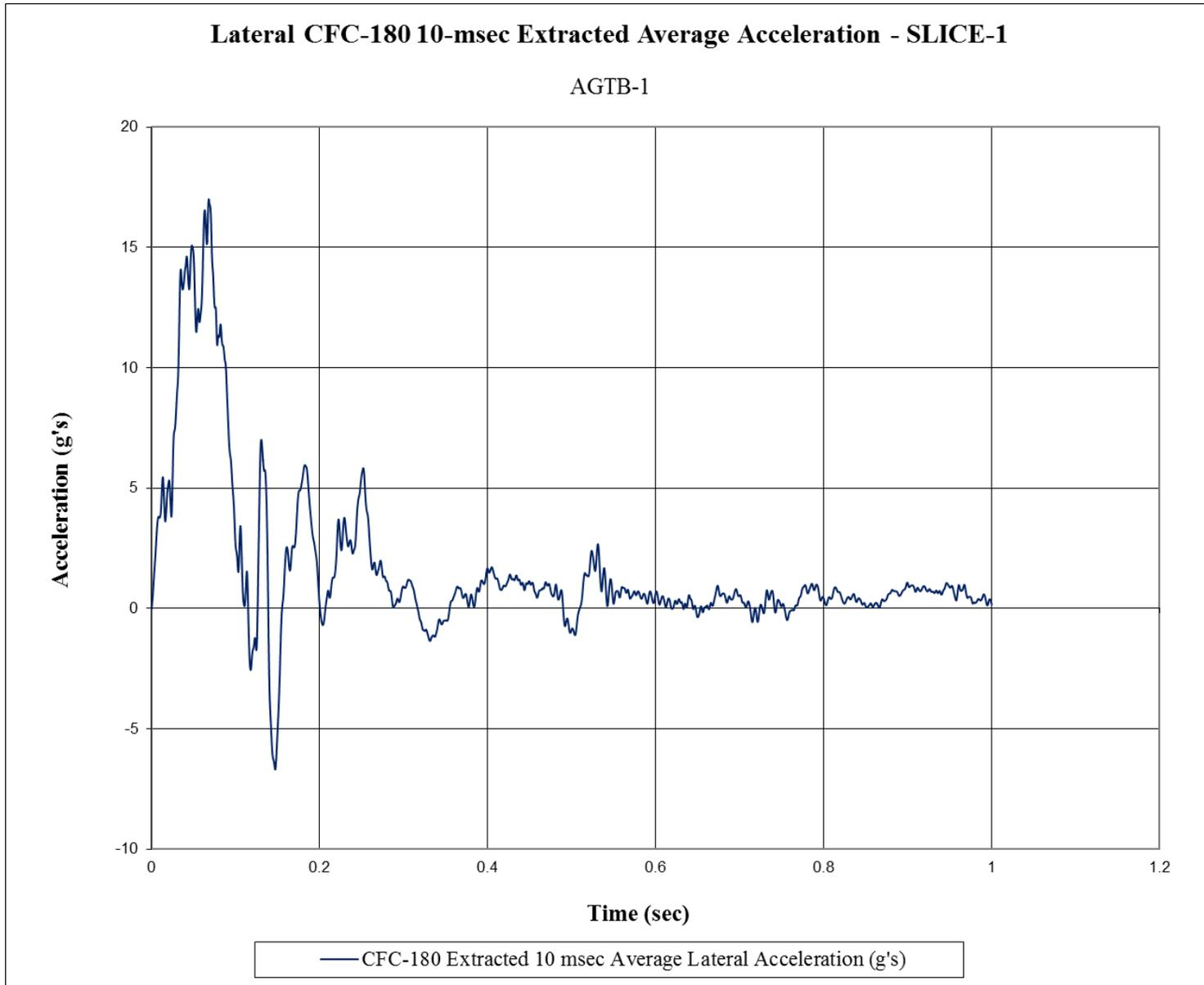
Figure E-4. 10-ms Average Lateral Deceleration (SLICE-1), Test No. AGTB-1
