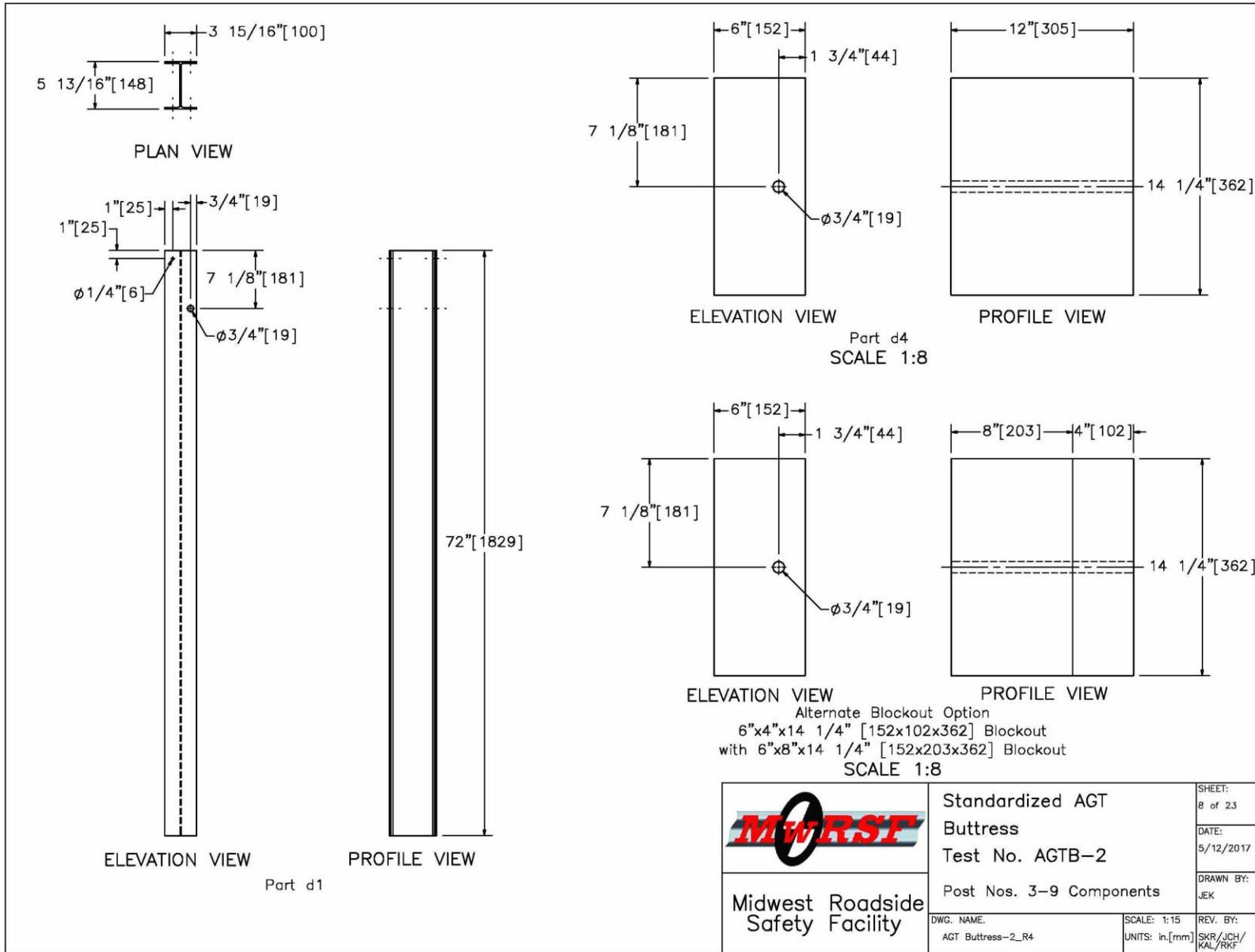
Figure 55. Post Nos. 3 through 9 Components, Test No. AGTB-2
