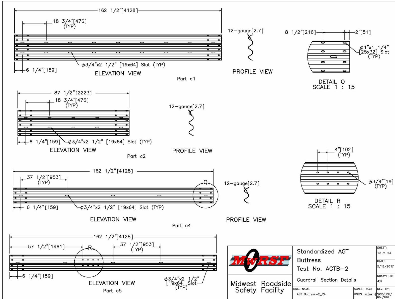
Figure 66. Guardrail Section Details, Test No. AGTB-2
