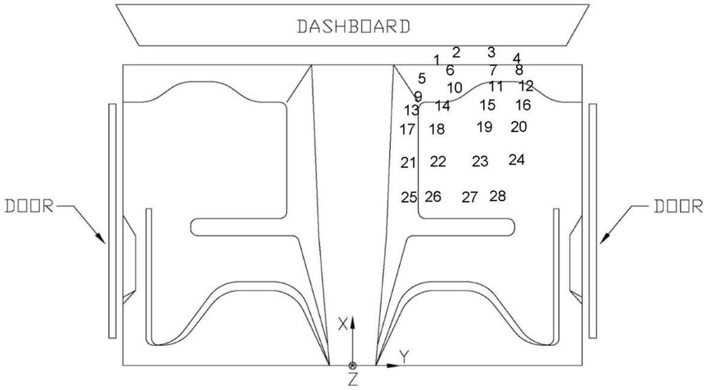
Figure D-8. Floor Pan Deformation Data – Set 2, Test No. AGTB-2
