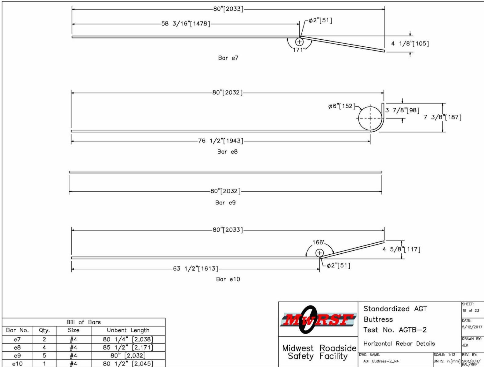
Figure 65. Horizontal Rebar Details, Test No. AGTB-2
