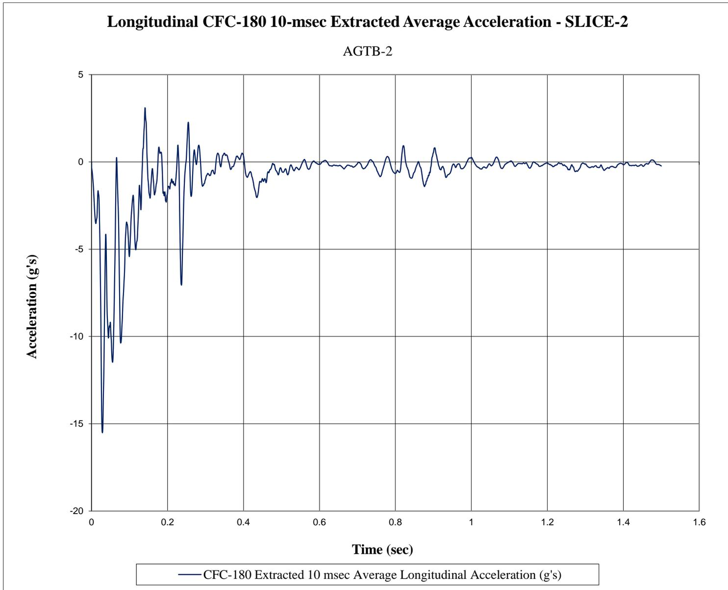
Figure F-9. 10-ms Average Longitudinal Deceleration (SLICE-2), Test No. AGTB-2
