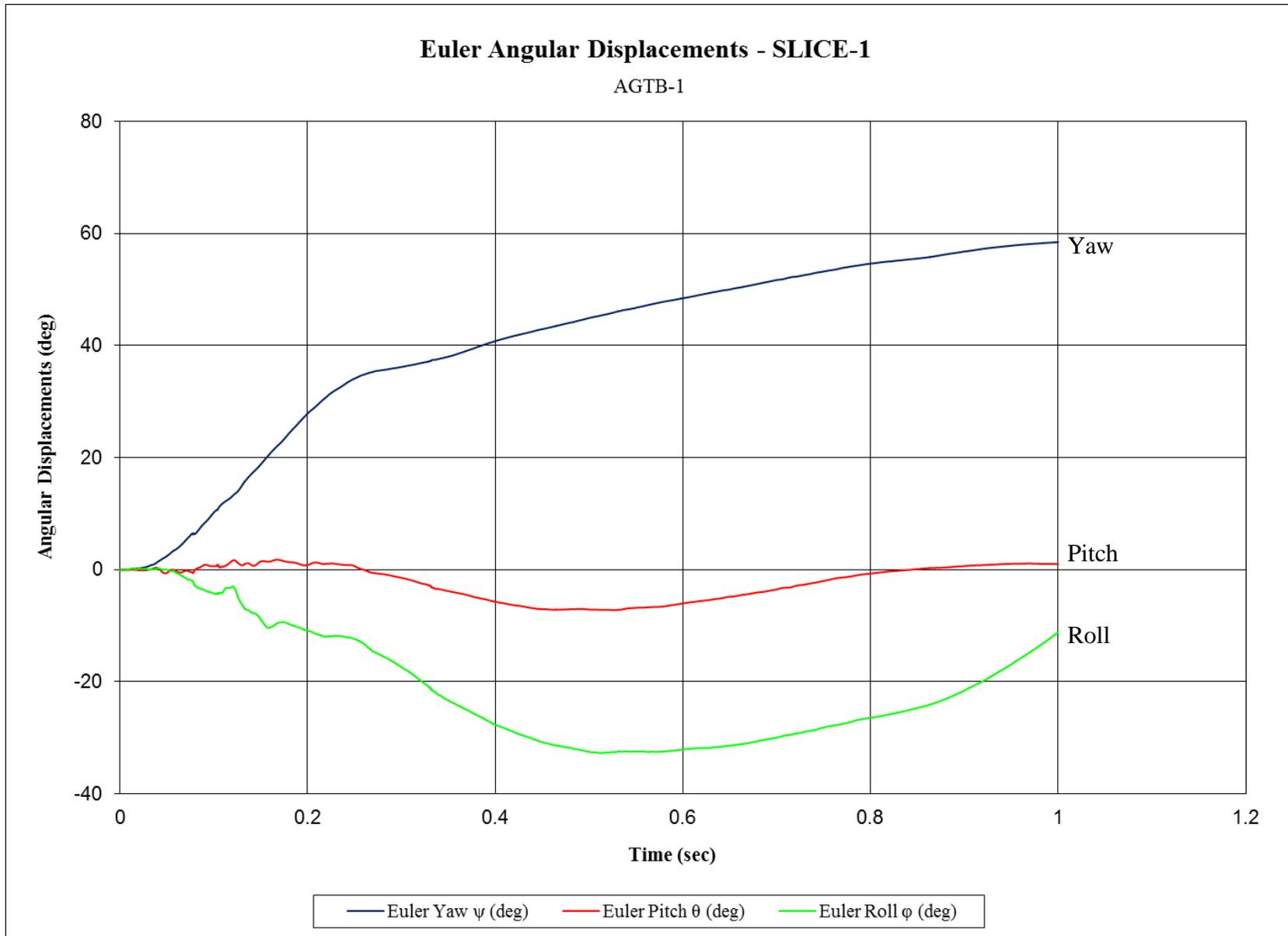
Figure E-7. Vehicle Angular Displacements (SLICE-1), Test No. AGTB-1
