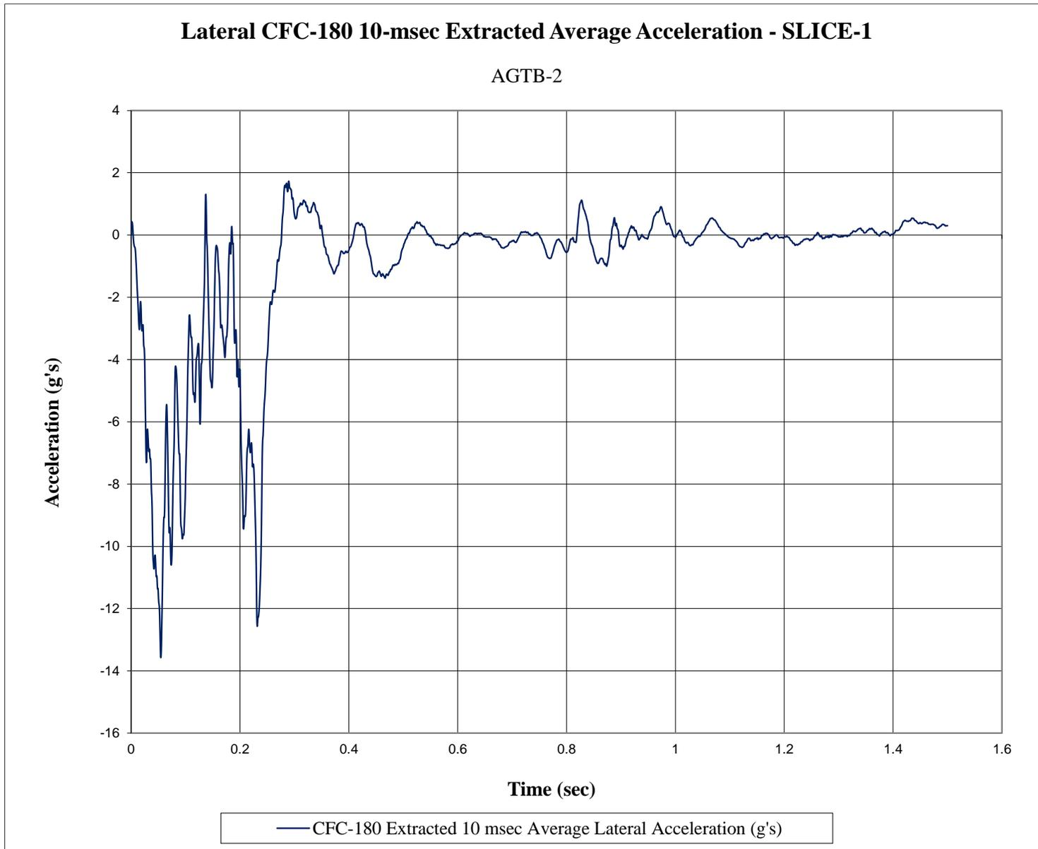
Figure F-4. 10-ms Average Lateral Deceleration (SLICE-1), Test No. AGTB-2
