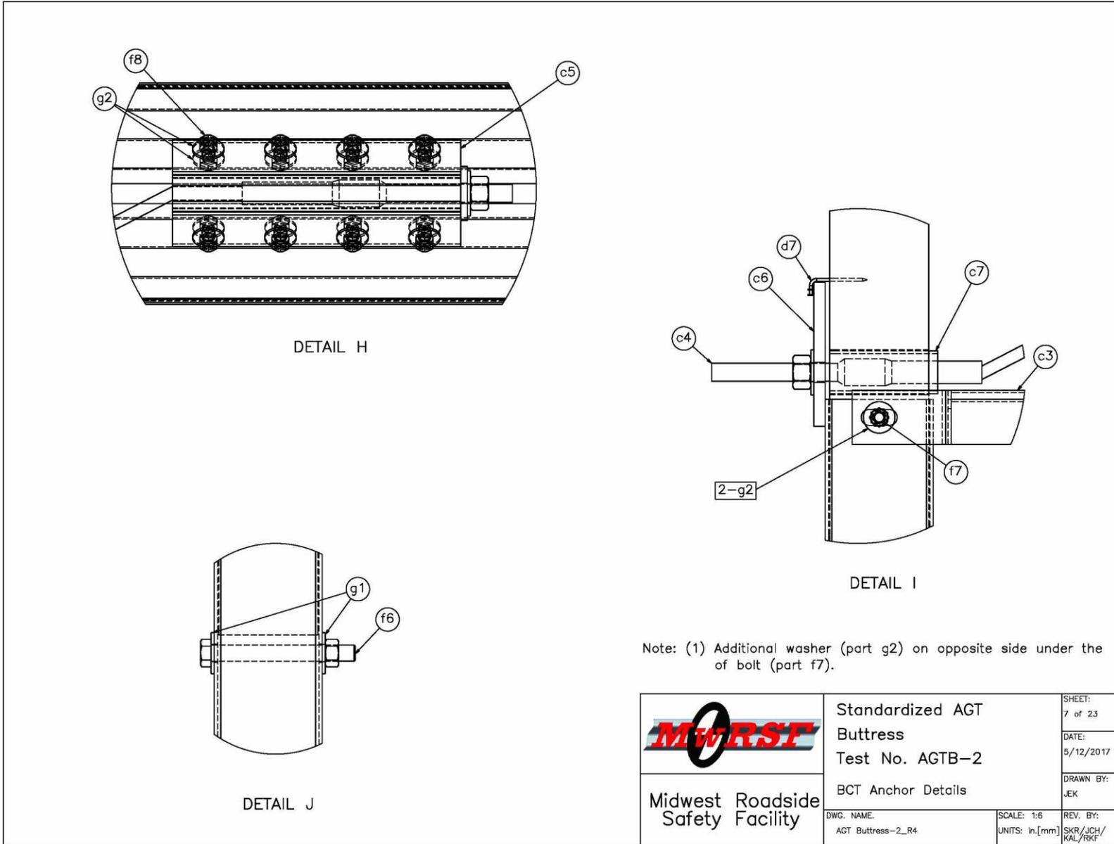
Figure 54. BCT Anchor Details, Test No. AGTB-2
