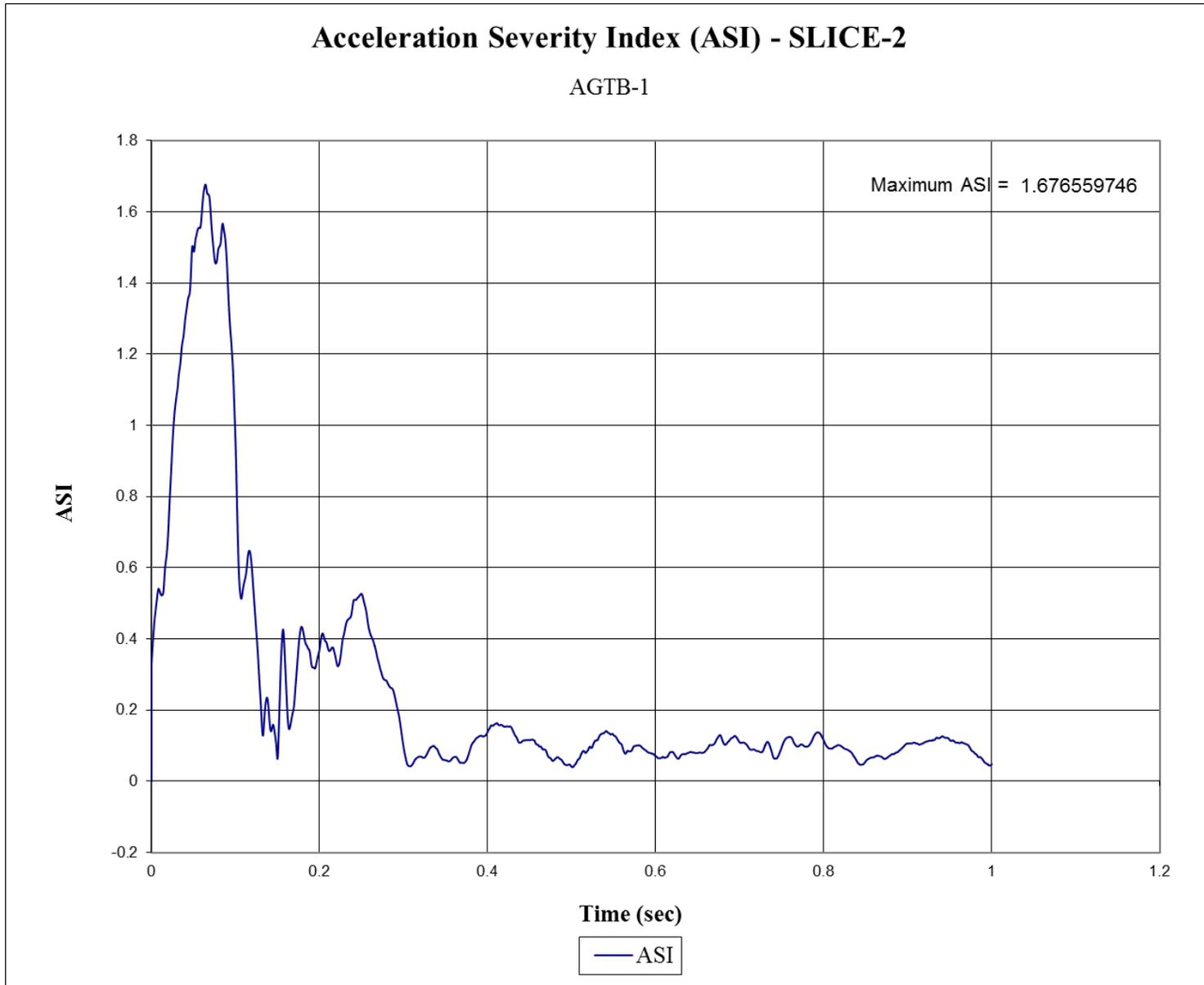
Figure E-16. Acceleration Severity Index (SLICE-2), Test No. AGTB-1
