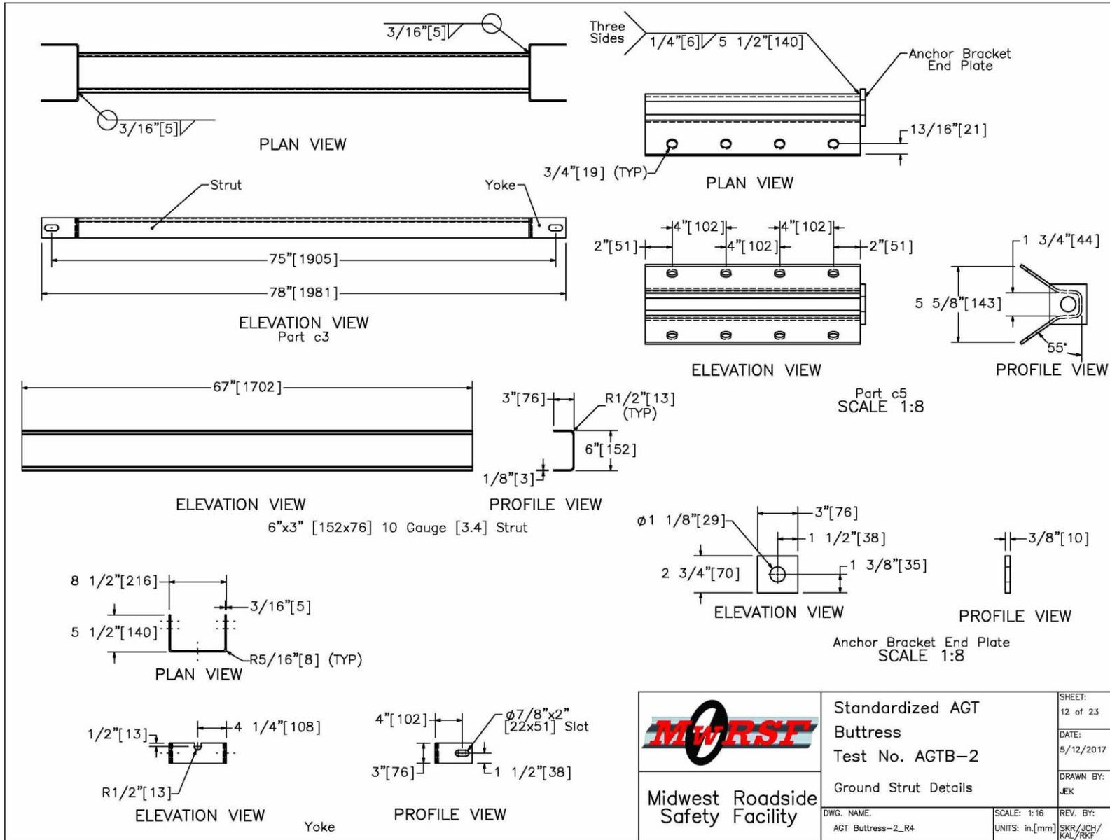
Figure 59. Ground Strut Details, Test No. AGTB-2
