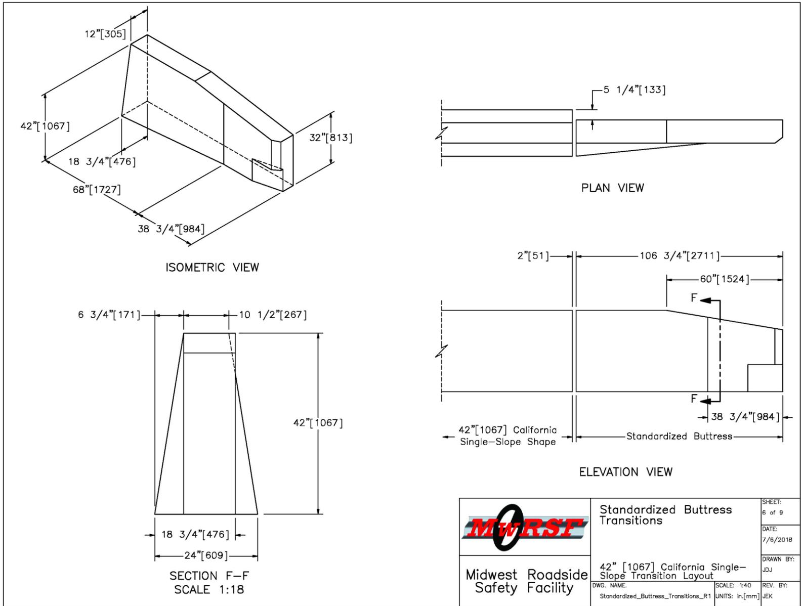
Figure 91. Buttress Shape Transition to 42-in. Tall California Single Slope Barrier
