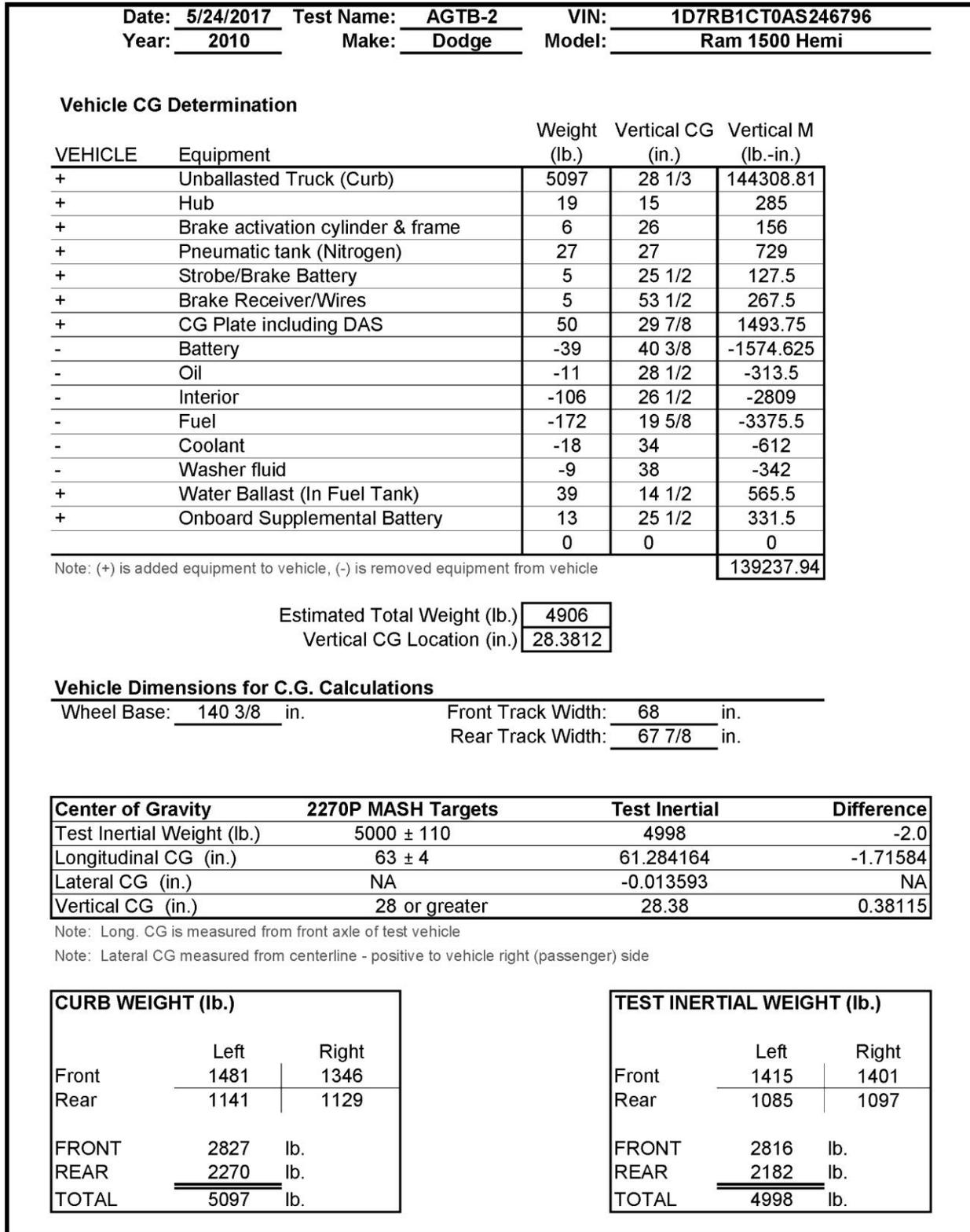
Figure B-2. Vehicle Mass Distribution, Test No. AGTB-2
