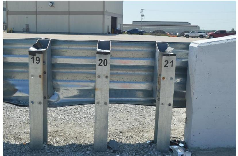
Figure 77. System Damage, Test No. AGTB-2
