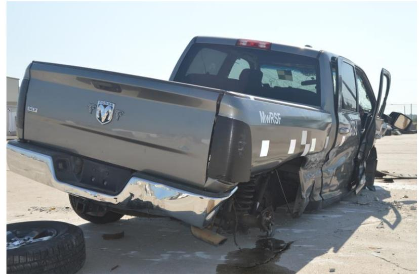
Figure 81. Vehicle Damage, Test No. AGTB-2
