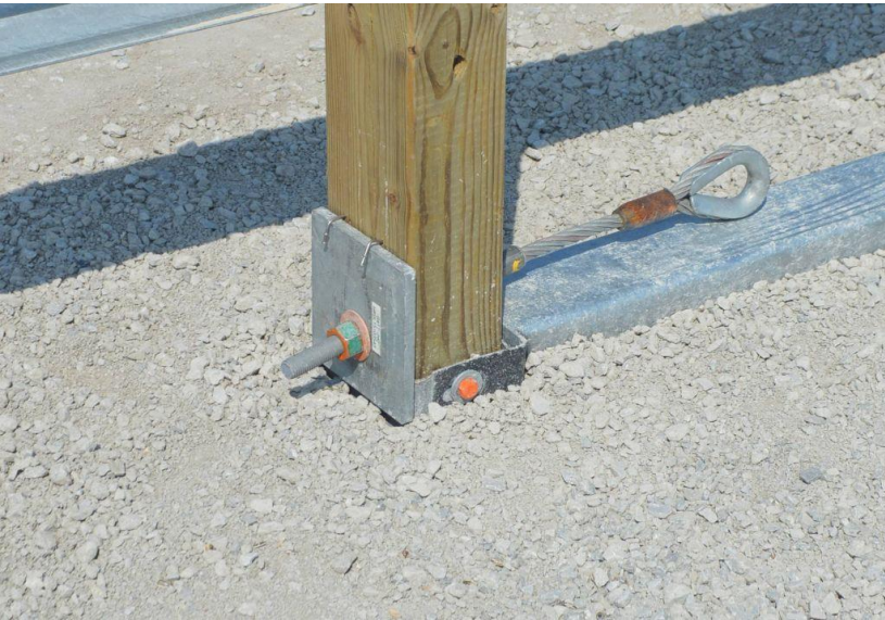
Figure 64. System Damage – Upstream End Anchorage System, Test No. SPTA-1
