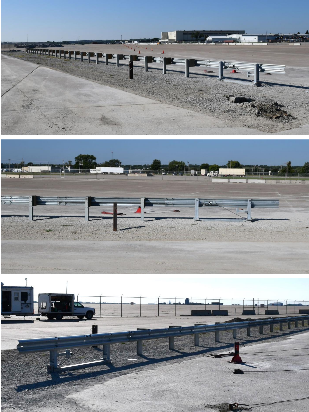
Figure 97. Test Installation Photographs – Trailing-End Anchorage System, Test No. SPTA-2
