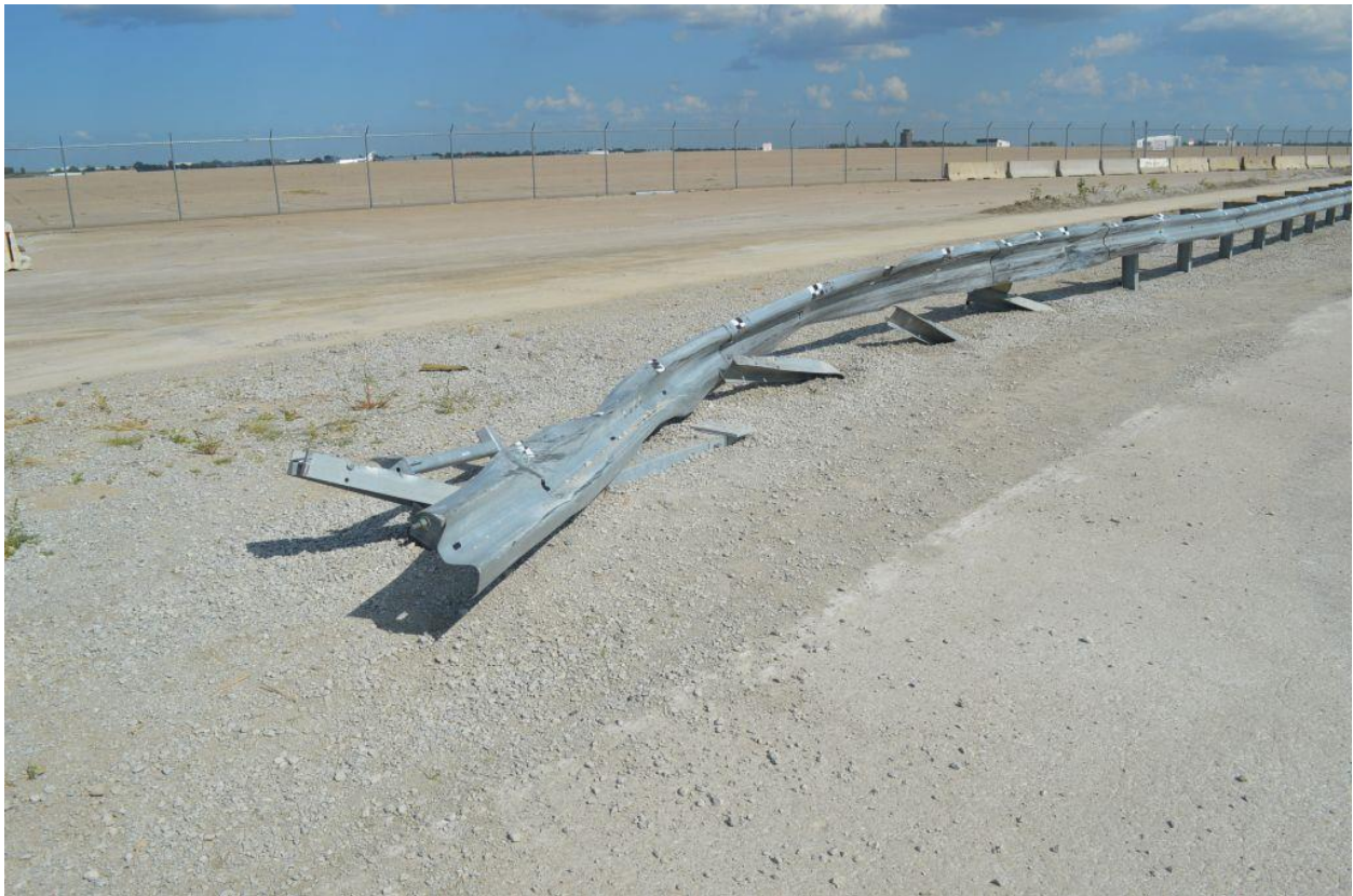
Figure 58. System Damage, Test No. SPTA-1
