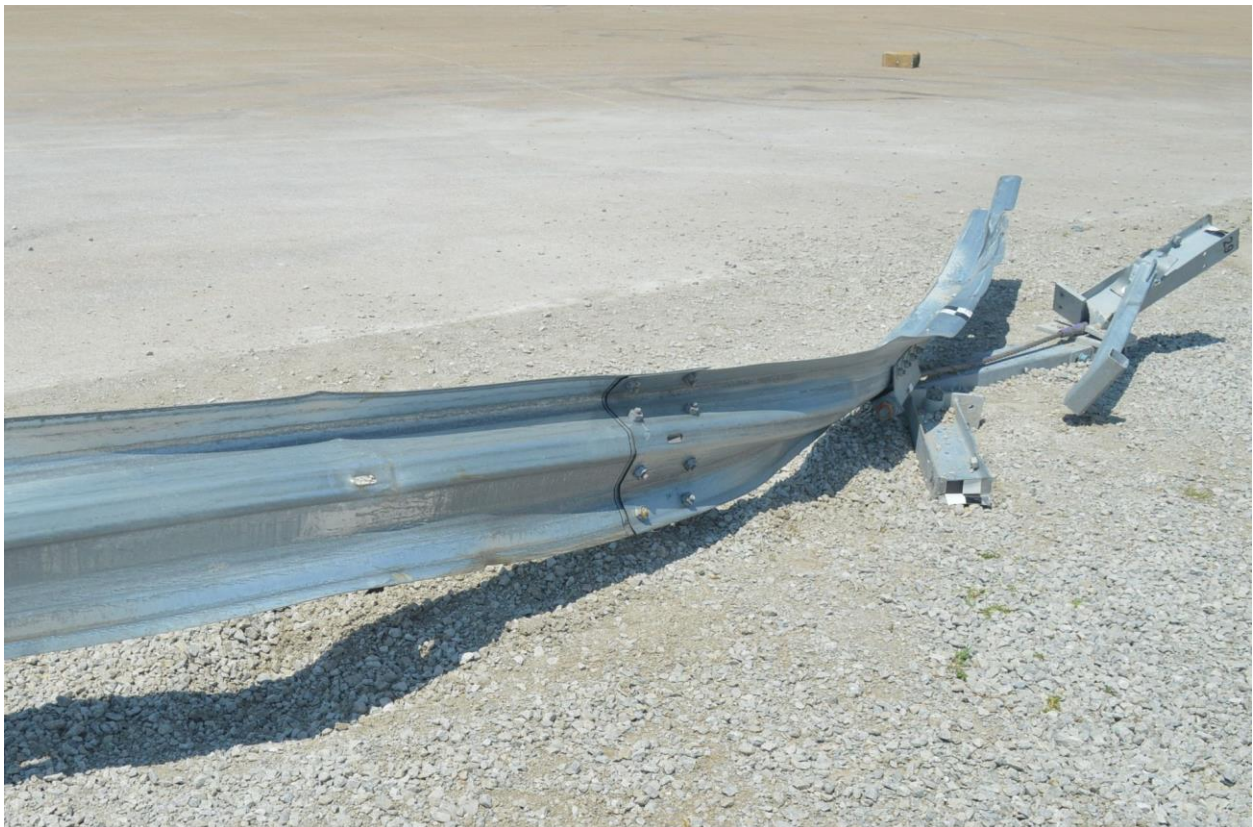
Figure 59. System Damage, Test No. SPTA-1
