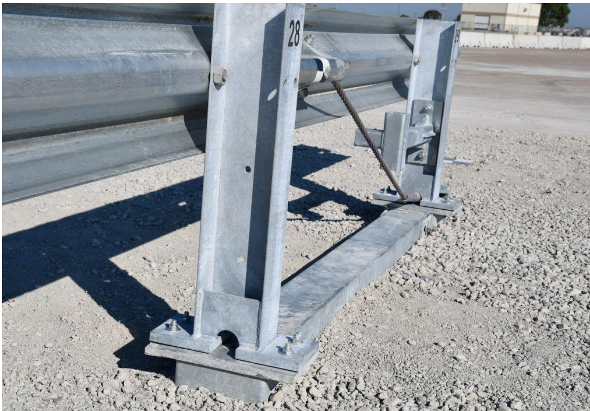
Figure 100. Test Installation Photographs – Trailing-End Anchorage System, Test No. SPTA-2
