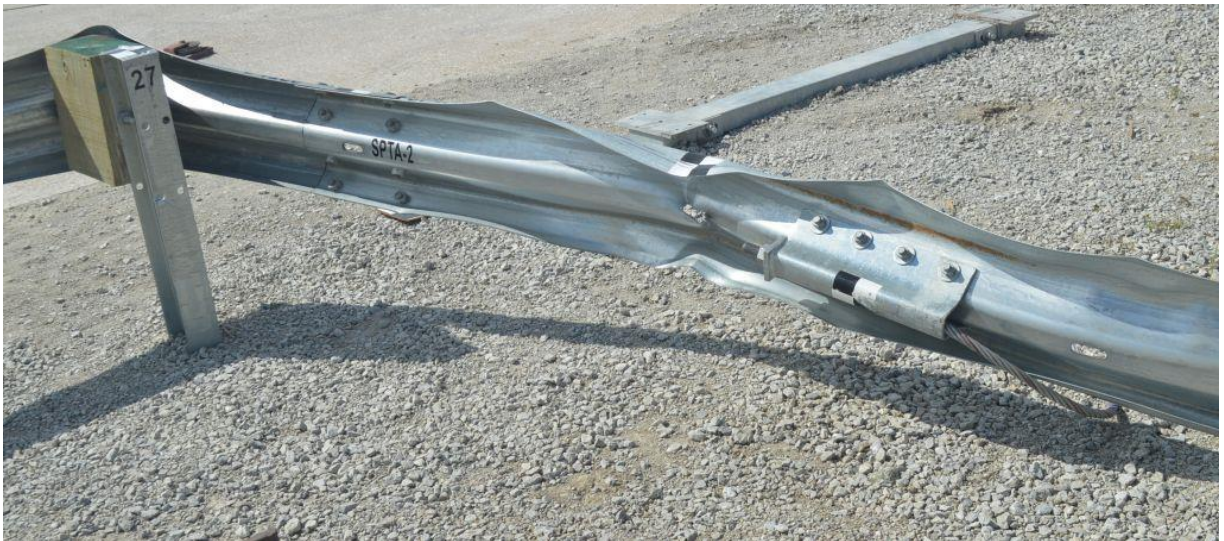
Figure 108. System Damage, Test No. SPTA-2
