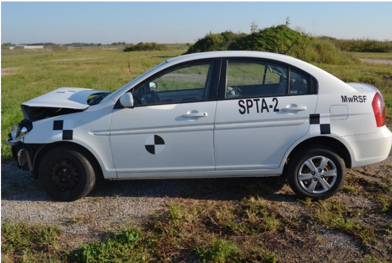
Figure 113. Vehicle Damage, Test No. SPTA-2
