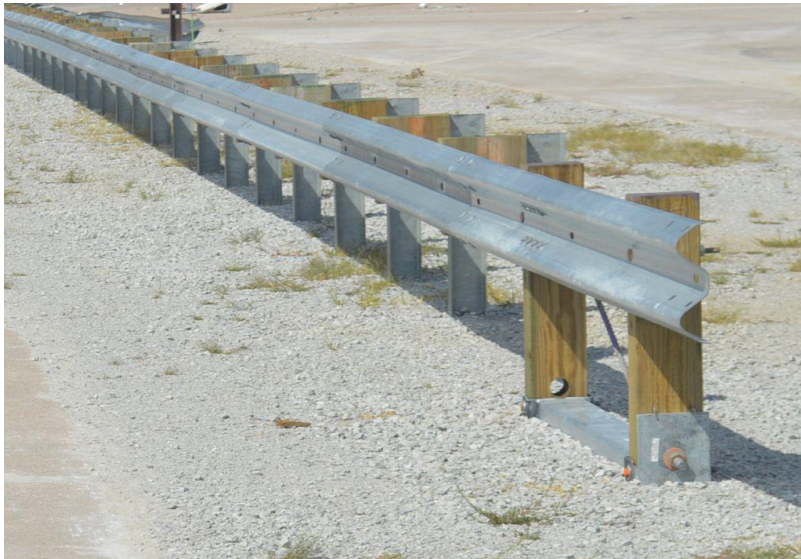
Figure 111. System Damage – Upstream End Anchorage System, Test No. SPTA-2
