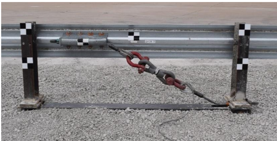
Figure 4. Steel-Post, Trailing-End Anchorage System Prototype
