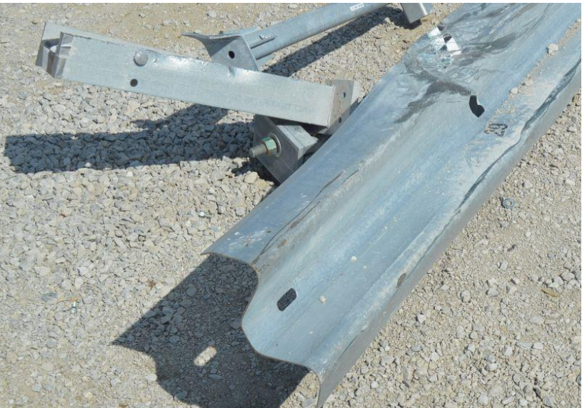
Figure 63. System Damage, Post Nos. 28 and 29, Test No. SPTA-1
