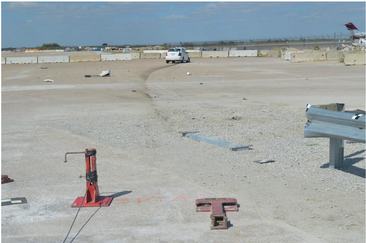
Figure 107. Vehicle Final Position and Trajectory Marks, Test No. SPTA-2
