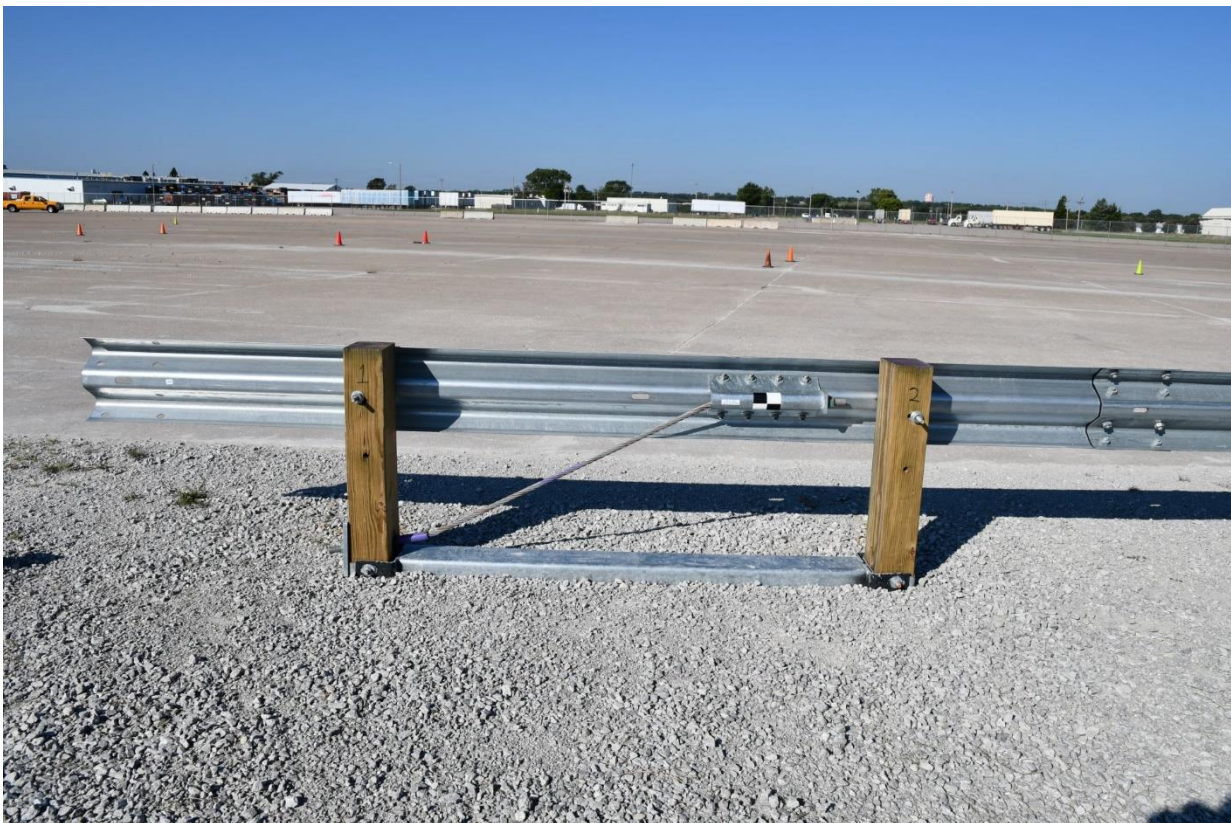
Figure 101. Test Installation Photographs – Upstream End Anchorage System, Test No. SPTA-2
