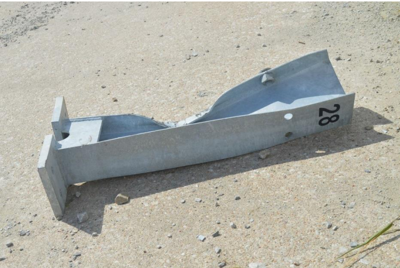
Figure 110. System Damage – Post Nos. 28 and 29, Test No. SPTA-2
