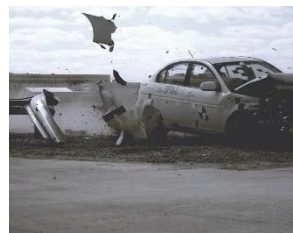
Figure 104. Additional Sequential Photographs, Test No. SPTA-2
