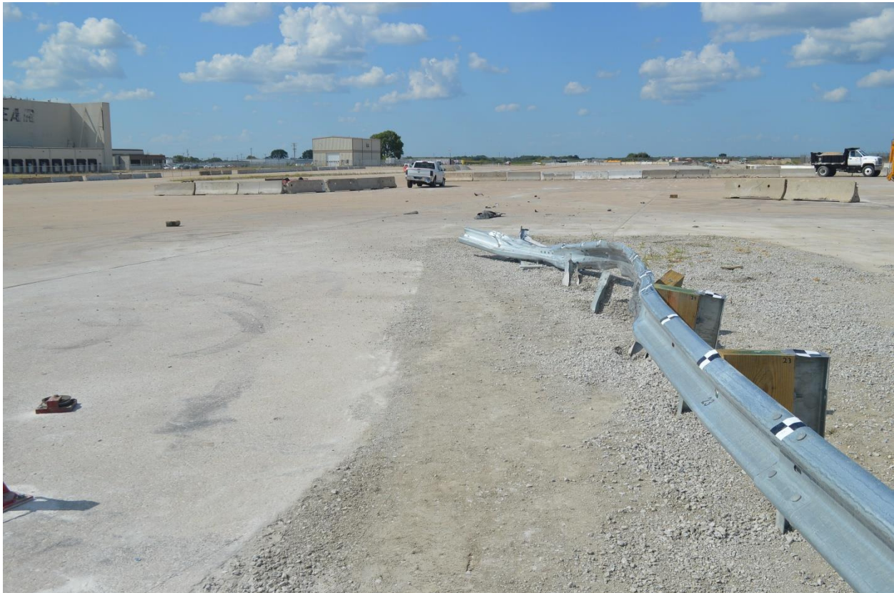
Figure 57. Vehicle Final Position and Trajectory Marks, Test No. SPTA-1
