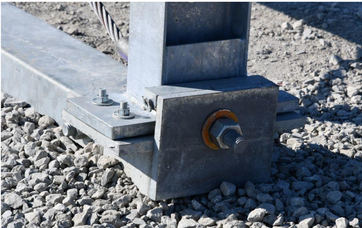
Figure 99. Test Installation Photographs – Trailing-End Anchorage System, Test No. SPTA-2
