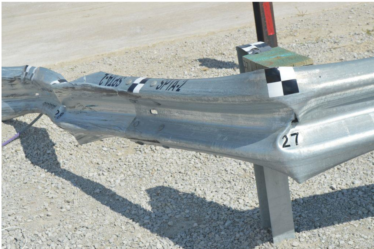
Figure 109. System Damage, Test No. SPTA-2
