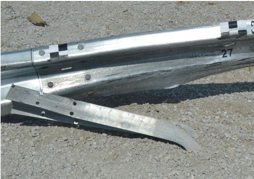
Figure 62. System Damage, Post Nos. 24, 25, 26, and 27, Test No. SPTA-1
