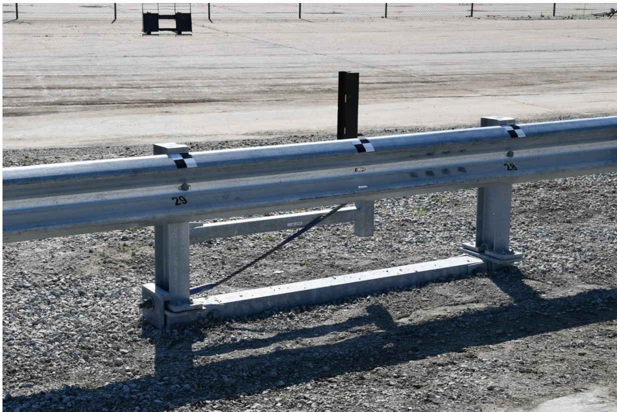
Figure 48. Test Installation Photographs – Trailing-End Anchorage System, Test No. SPTA-1
