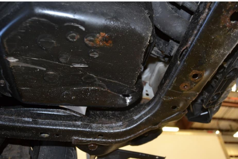
Figure 116. Undercarriage Damage, Test No. SPTA-2
