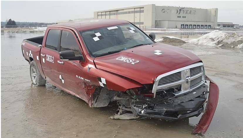
Figure 92. Additional Vehicle Damage, Test No. CMGS-2
