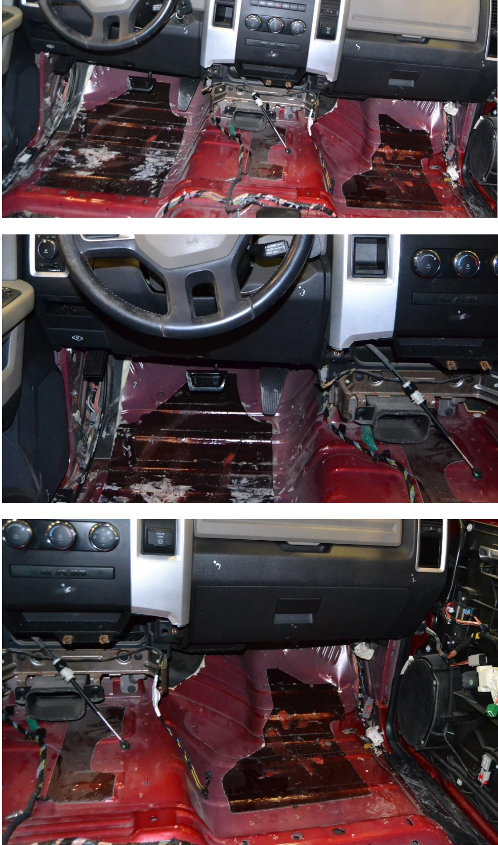
Figure 94. Vehicle Occupant Compartment Damage, Test No. CMGS-2
