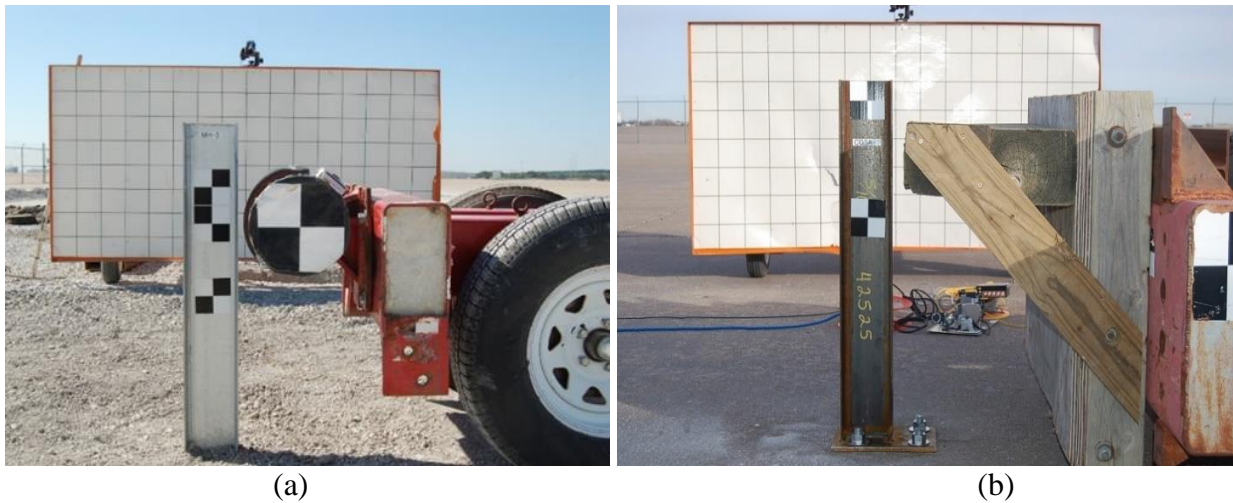
Figure 98. (a) Soil Embedment Post Test Nos. MH-1 and MH-4; (b) Concrete-Mounted Post Test No. CGSA-4
