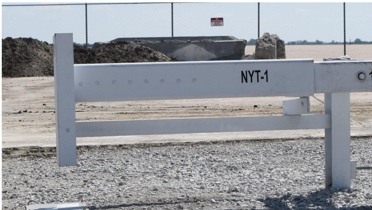
Figure 32. Test Installation-End Terminal, Test No. NYT-1
