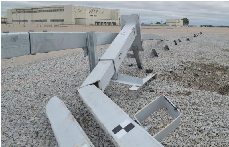
Figure 51. End Terminal Damage, Test No. NYT-1
