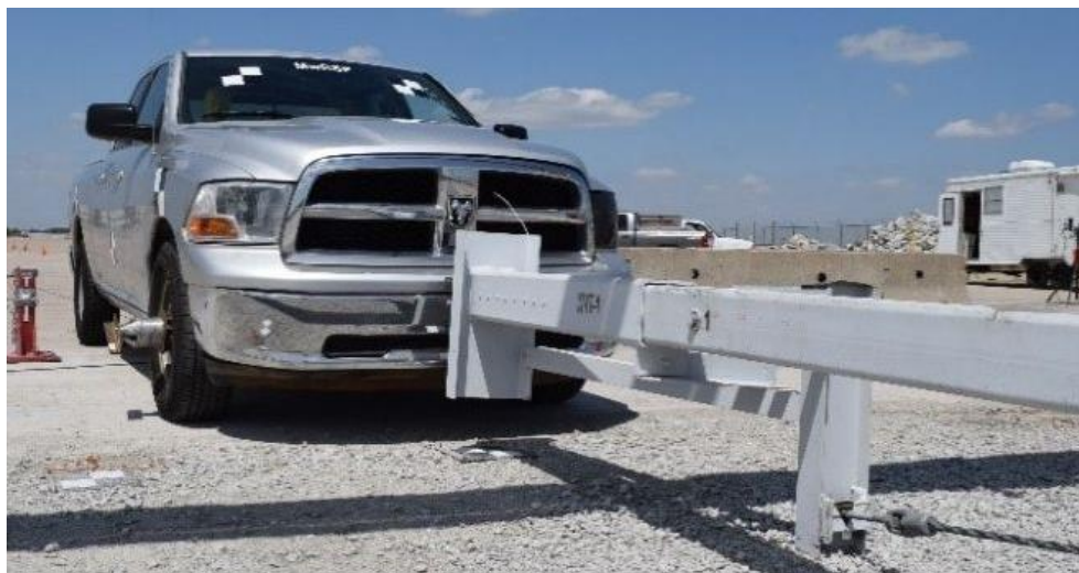
Figure 44. Impact Location, Test No. NYT-1
