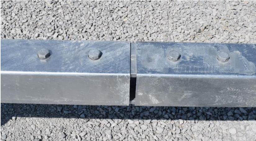
Figure 35. Test Installation, Splice Details, Test No. NYT-1
