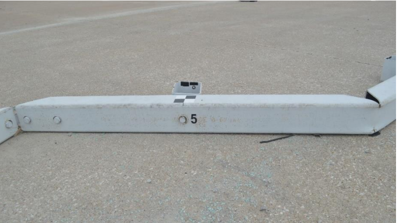
Figure 55. Rail Damage, Test No. NYT-1
