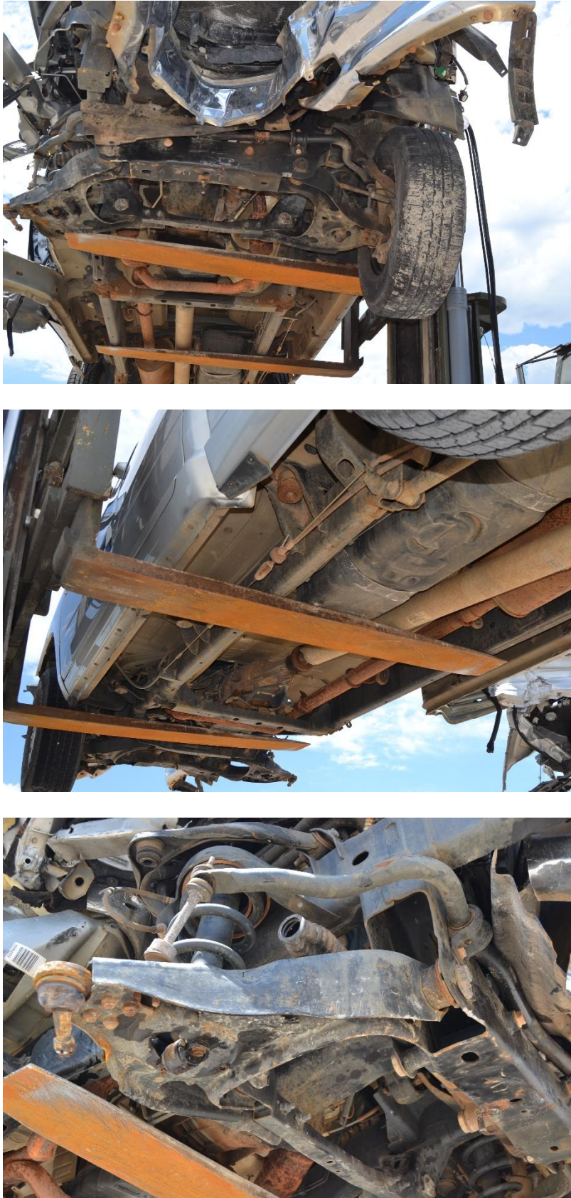
Figure 62. Vehicle Undercarriage Damage, Test No. NYT-1
