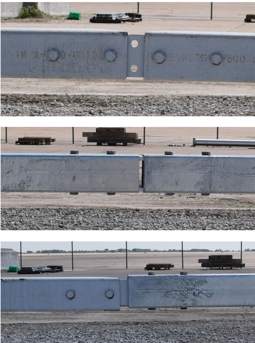
Figure 36. Test Installation, Splice Details; Test No. NYT-1
