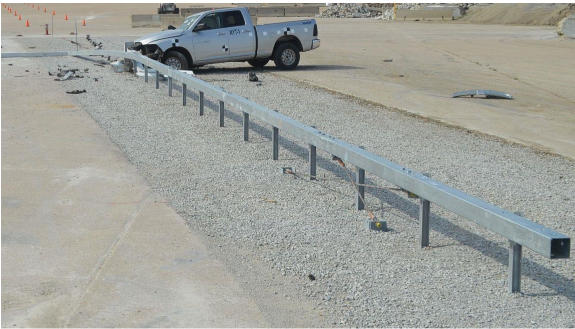
Figure 45. Vehicle Final Position and Trajectory Marks, Test No. NYT-1
