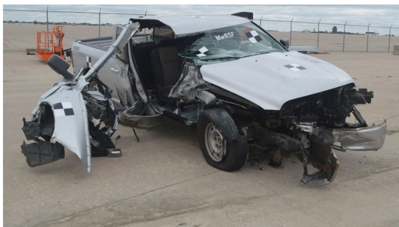
Figure 58. Vehicle Damage, Test No. NYT-1
