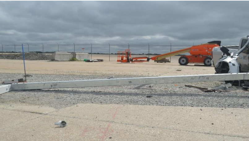
Figure 56. Additional Rail Damage, Test No. NYT-1
