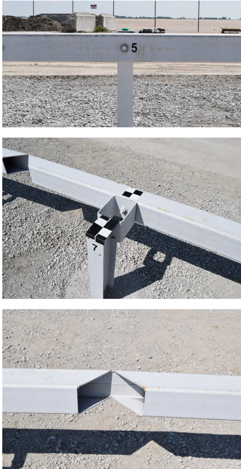
Figure 33. Test Installation Post and Rail Details for Post Nos. 1 through 8, Test No. NYT-1
