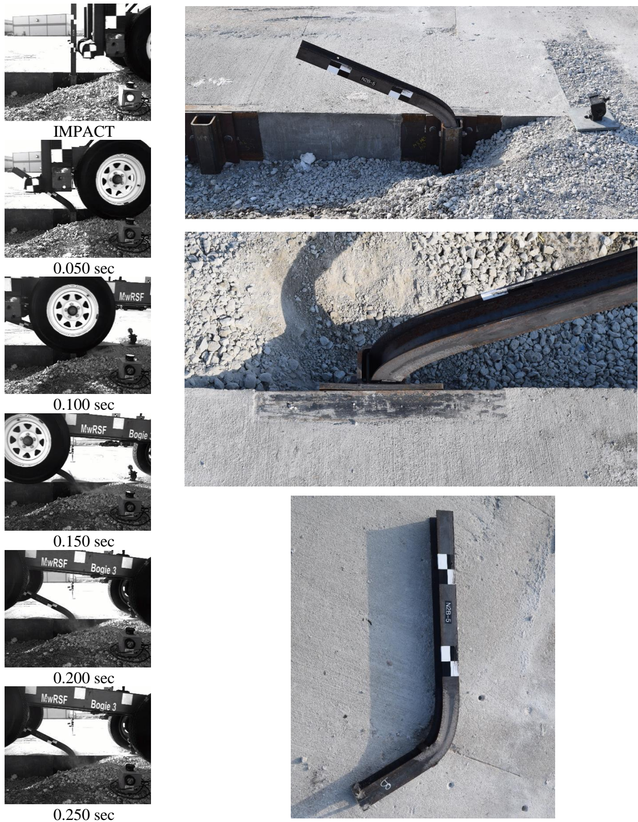
Figure 46. Time-Sequential and Post-Impact Photographs, Test No. N2B-5
