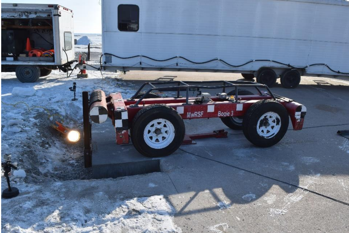
(a) Lateral Impact Head - Test Nos. N2B-1 Through N2B-4
