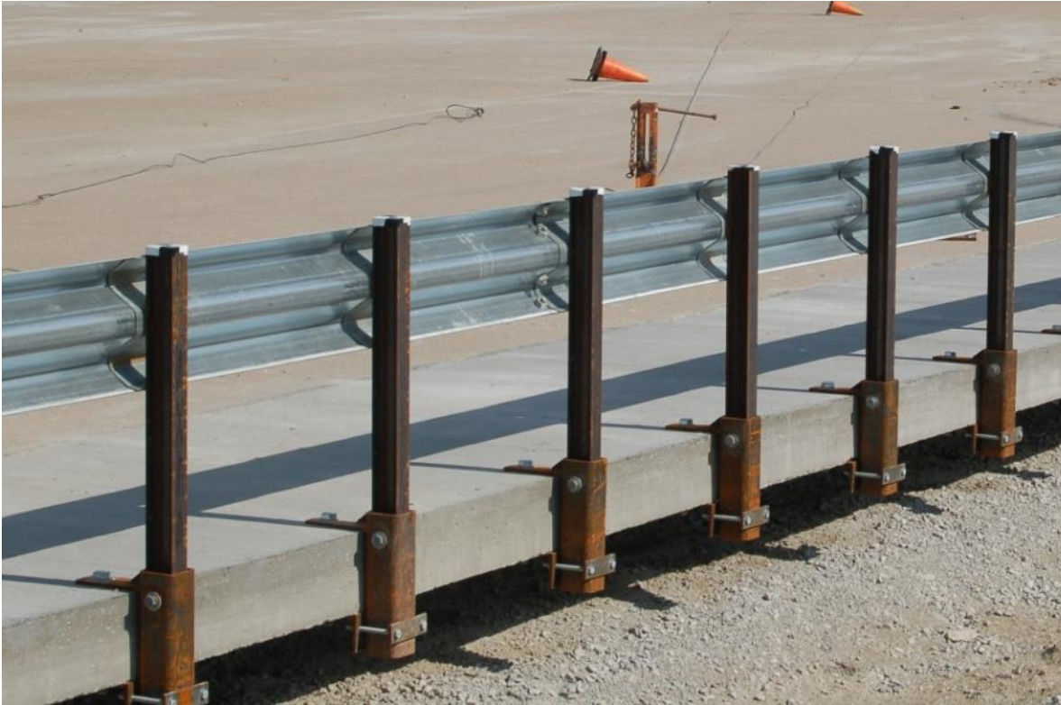
Figure 1. MGS Bridge Rail Test Installation [3]
