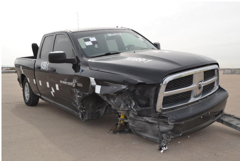
Figure 96. Vehicle Damage, Test No. N2BR-1
