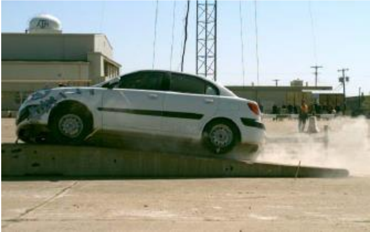
Figure 22. Vehicle Riding Up Sloped End Treatment, Test No. 490023-5 [8]
