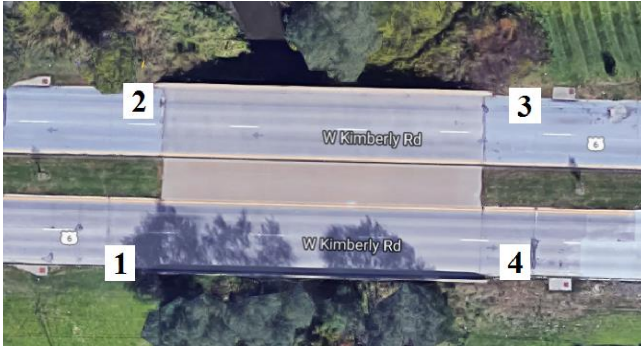
Figure 163. Bridge No. 8204.9S006 with Sloped End Treatments Labeled [1]
