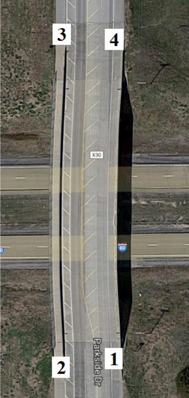
Figure 156. Bridge No. 1654.6O080 with Sloped End Treatments Labeled [1]
