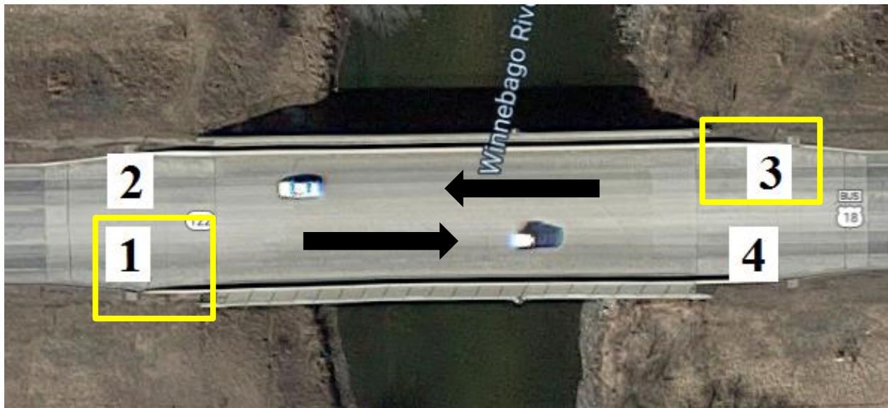
Figure 142. Sloped End Treatments on Two-Way Traffic Road
