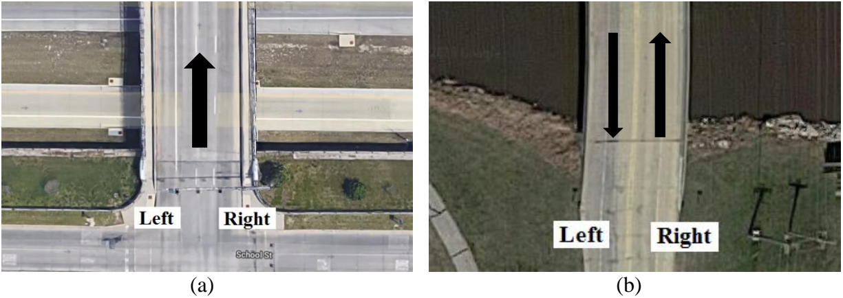
Figure 133. Left- and Right-Side Sloped End Treatments for (a) One-Way and (b) Two-Way Traffic
