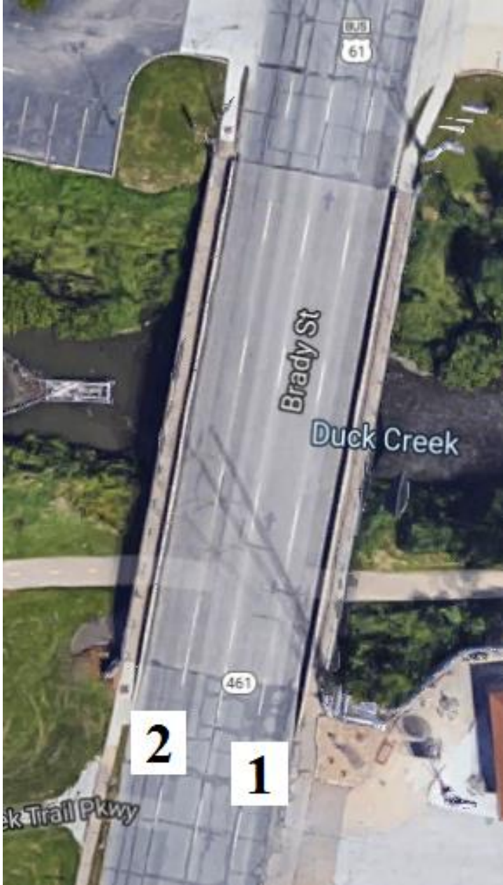
Figure 164. Bridge No. 8220.1R061 with Sloped End Treatments Labeled [1]
