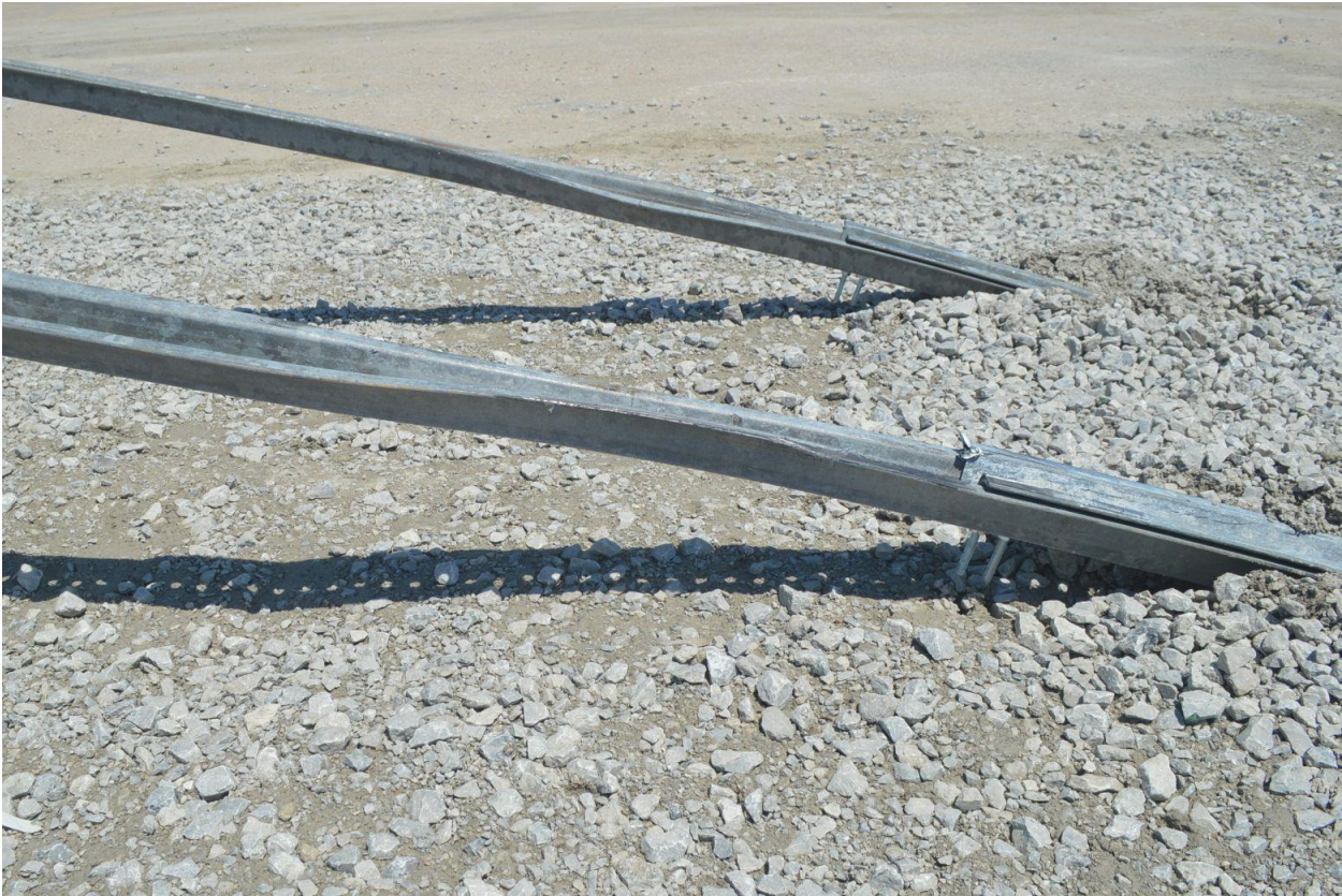
Figure 71. System Damage, U-Channel Posts, Test No. MOS-7
