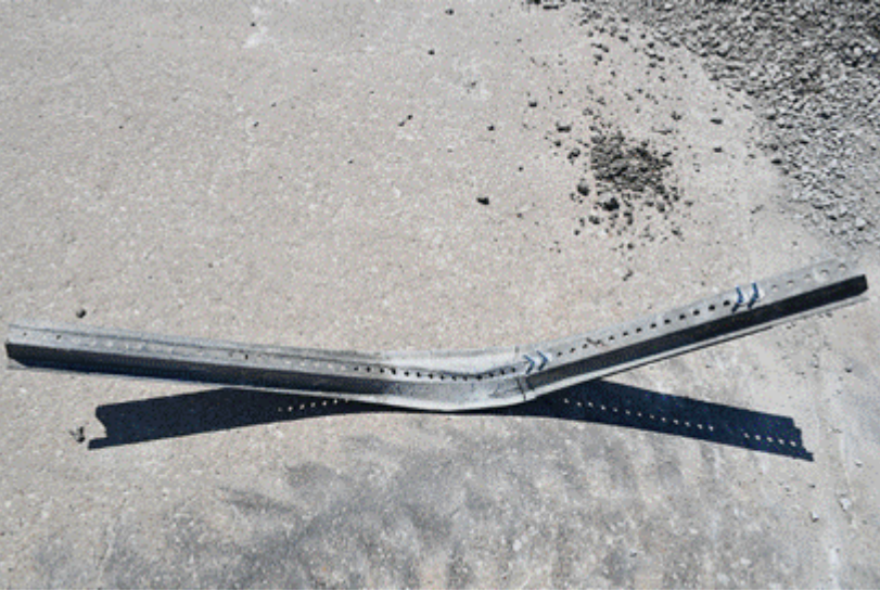
Figure 42. System Damage, Embedded Stubs, Test No. MOS-5
