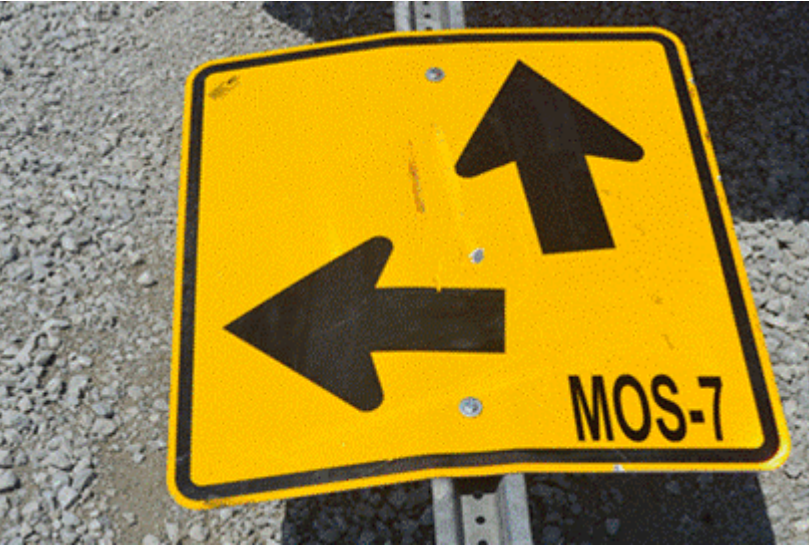
Figure 70. System Damage, Sign Panels, Test No. MOS-7
