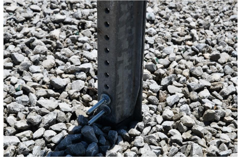
Figure 15. Test Installation Photographs, U-Channel Post and Stub Splice, Test Nos. MOS-5 through MOS-7
