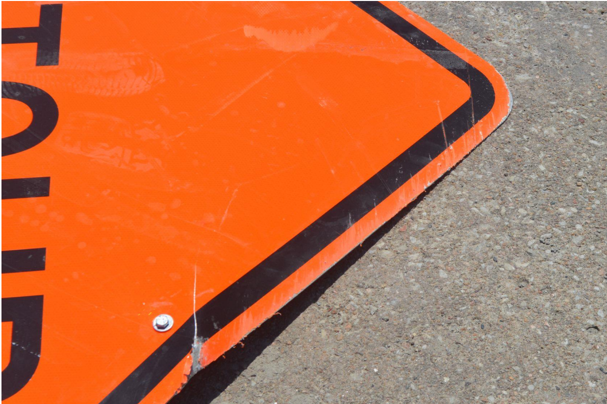
Figure 54. System Damage, Sign Panels, Test No. MOS-6
