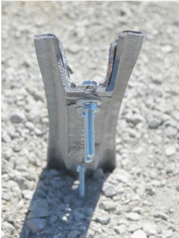
Figure 55. System Damage, U-Channel Posts, Test No. MOS-6
