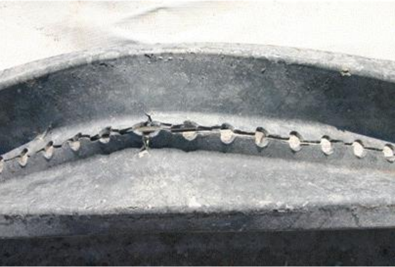
Figure 57. System Damage, Embedded Stubs, Test No. MOS-6
