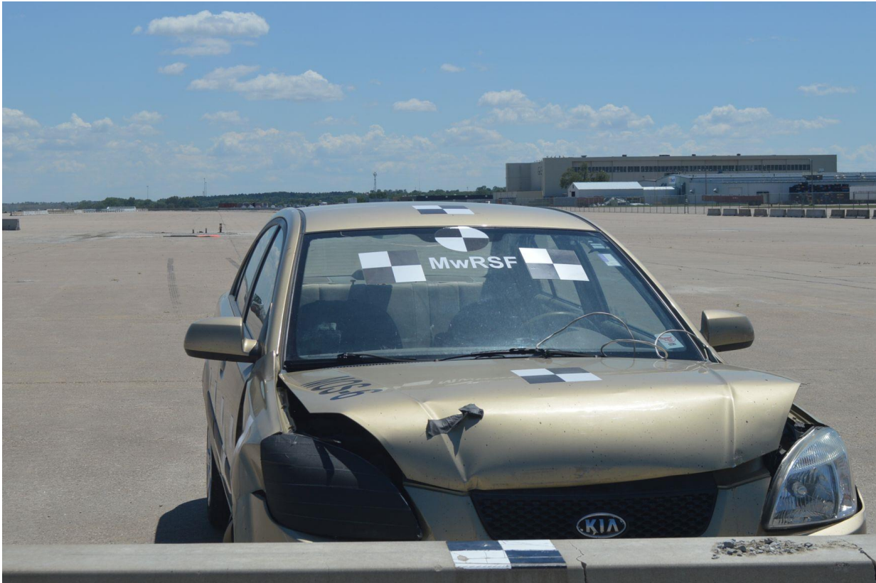
Figure 52. Vehicle Final Position and Trajectory Marks, Test No. MOS-6
