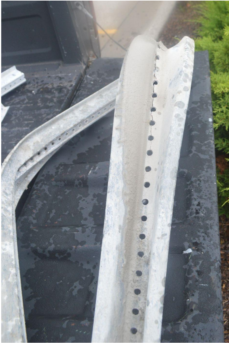
Figure 72. System Damage, Embedded Stubs, Test No. MOS-7
