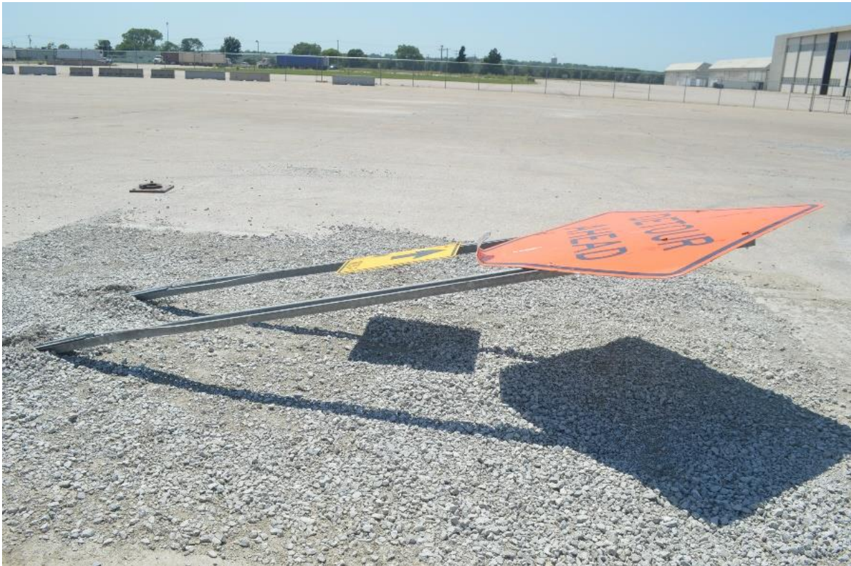
Figure 69. System Damage, Test No. MOS-7
