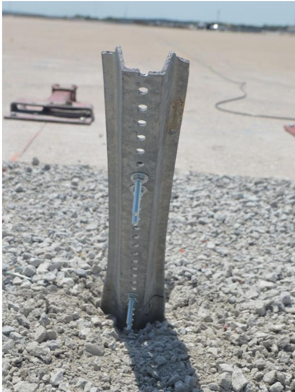
Figure 40. System Damage, U-Channel Posts, Test No. MOS-5
