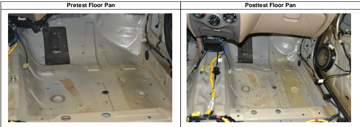
Figure D-15. Floor Pan Deformation – Set 2, Right, Test No. MOS-6
