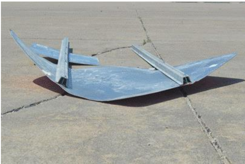
Figure 39. System Damage, Sign Panels, Test No. MOS-5
