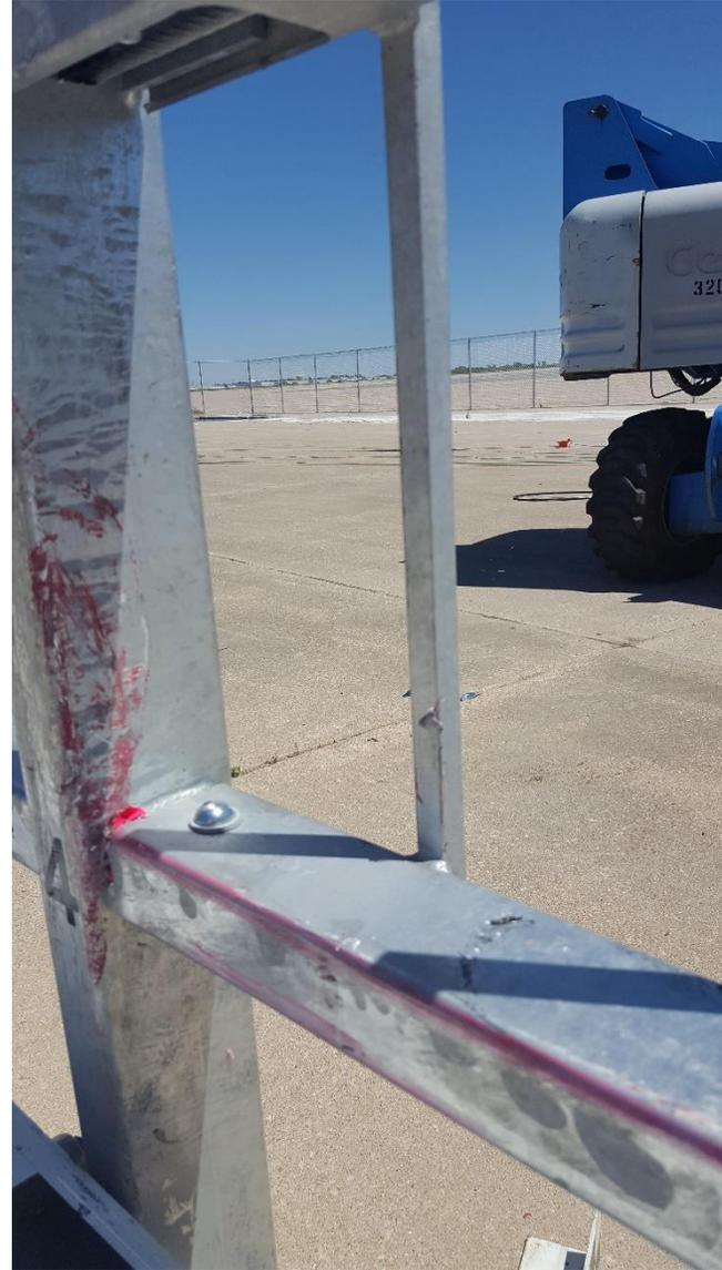
Figure 54. Rail and Post No. 4 Damage, Test No. MNPD-3
