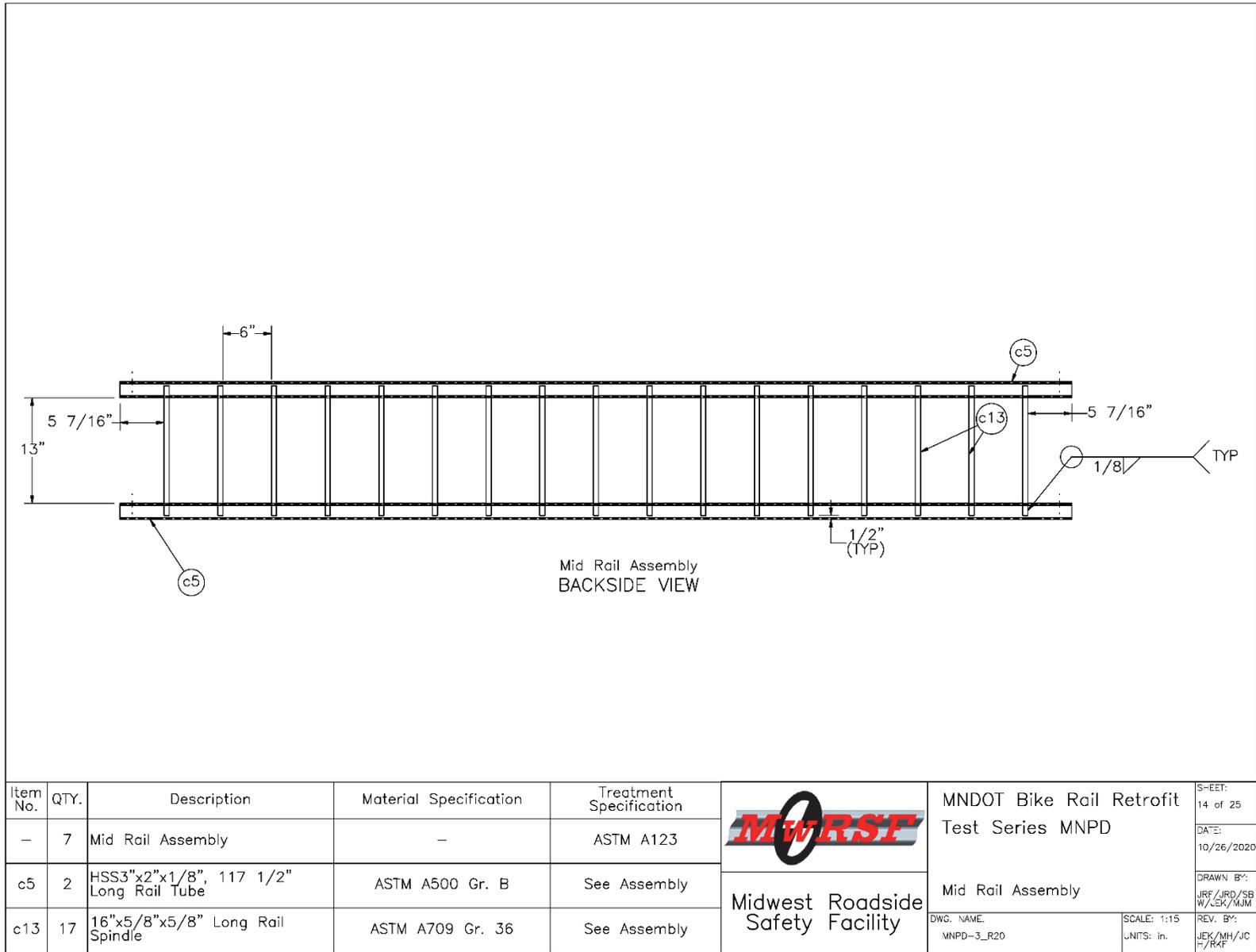
Figure 21. Mid Rail Assembly, Test No. MNPD-3
