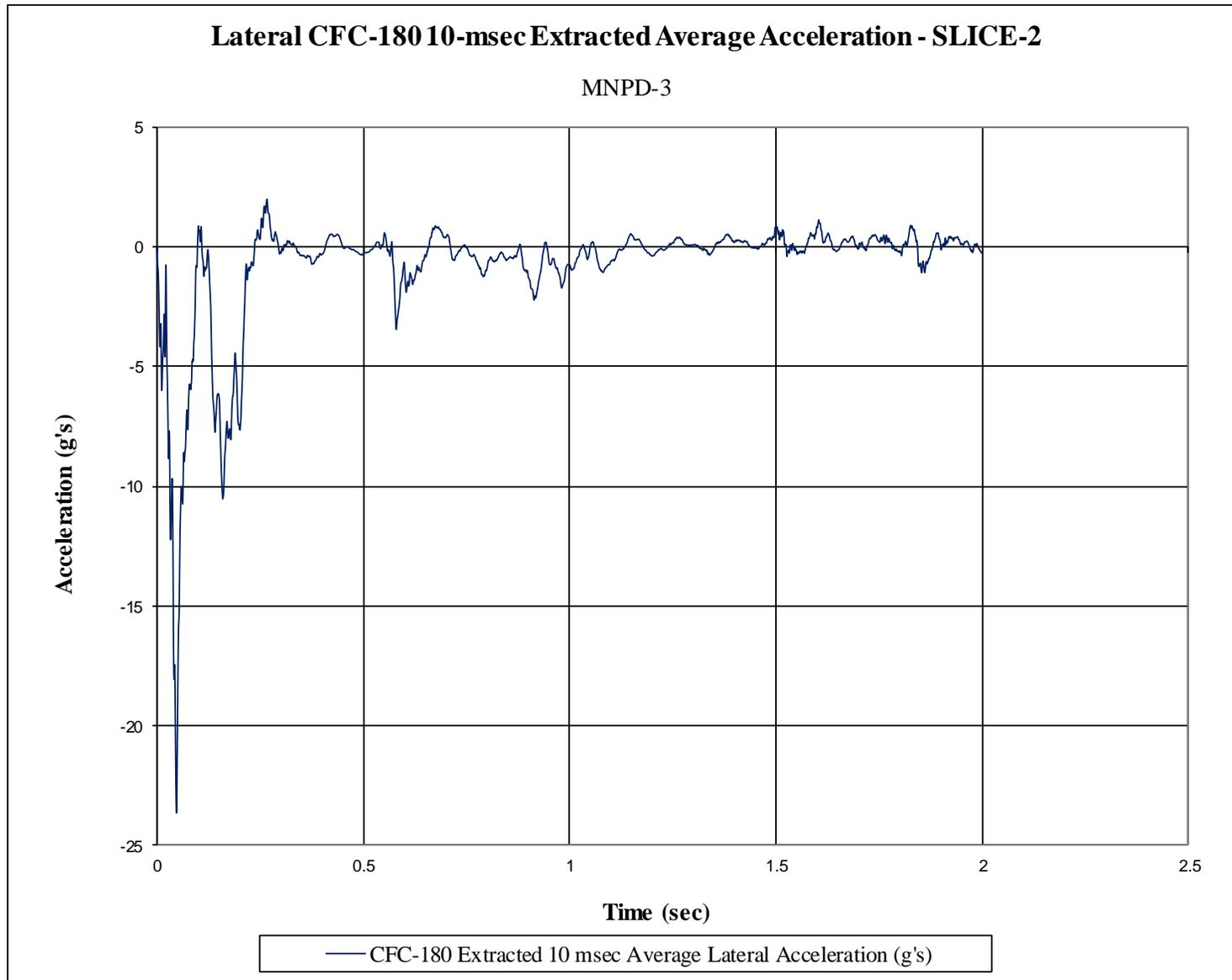
Figure D-4. 10-ms Average Lateral Deceleration (SLICE-2), Test No. MNP3
