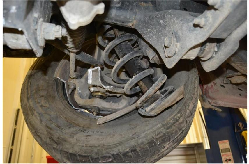
Figure 66. Undercarriage Damage, Test No. MNPD-3
