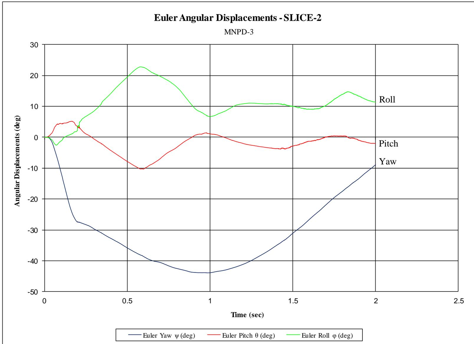
Figure D-7. Vehicle Angular Displacements (SLICE-2), Test No. MNP-3
