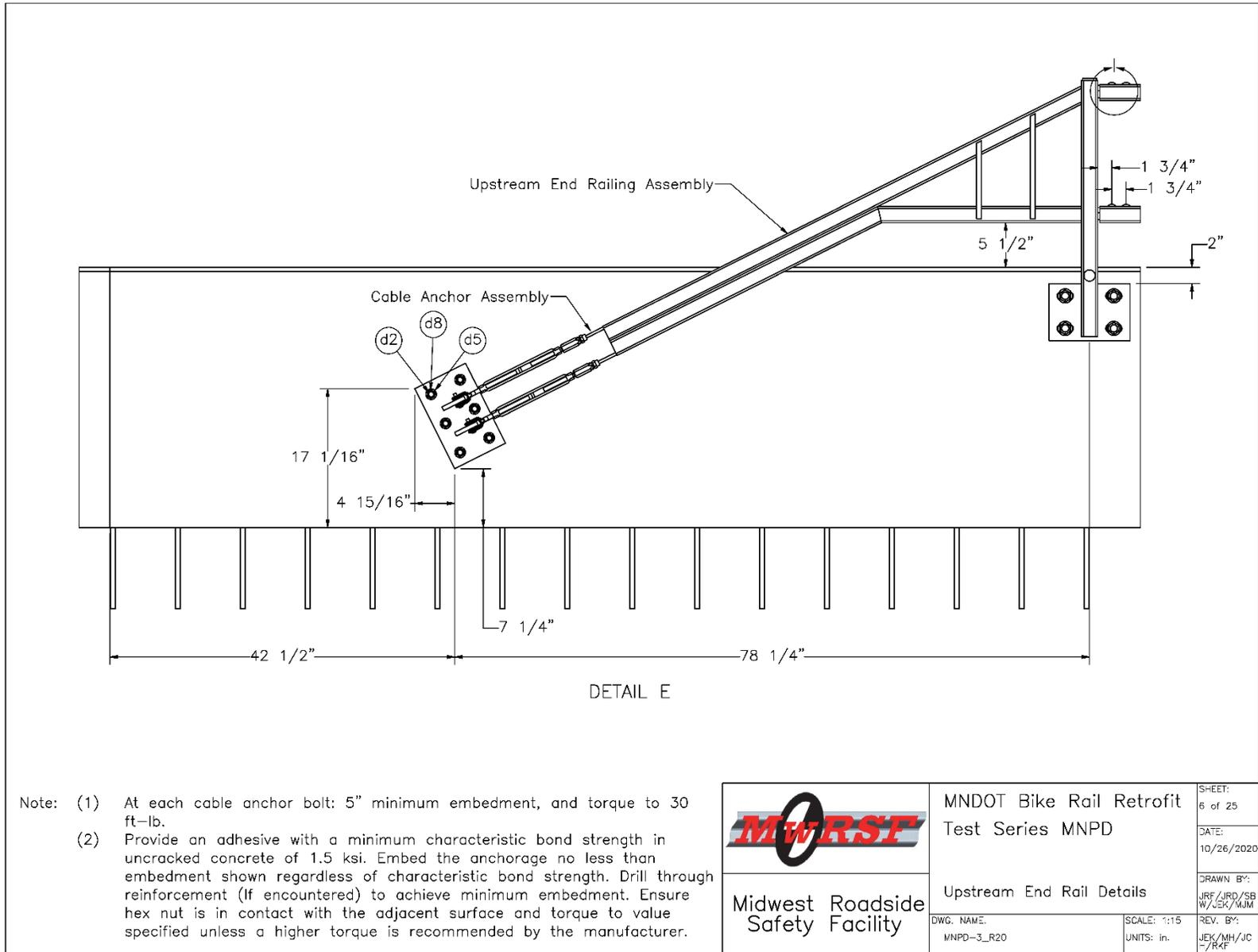
Figure 13. Upstream End Rail Details, Test No. MNPD-3
