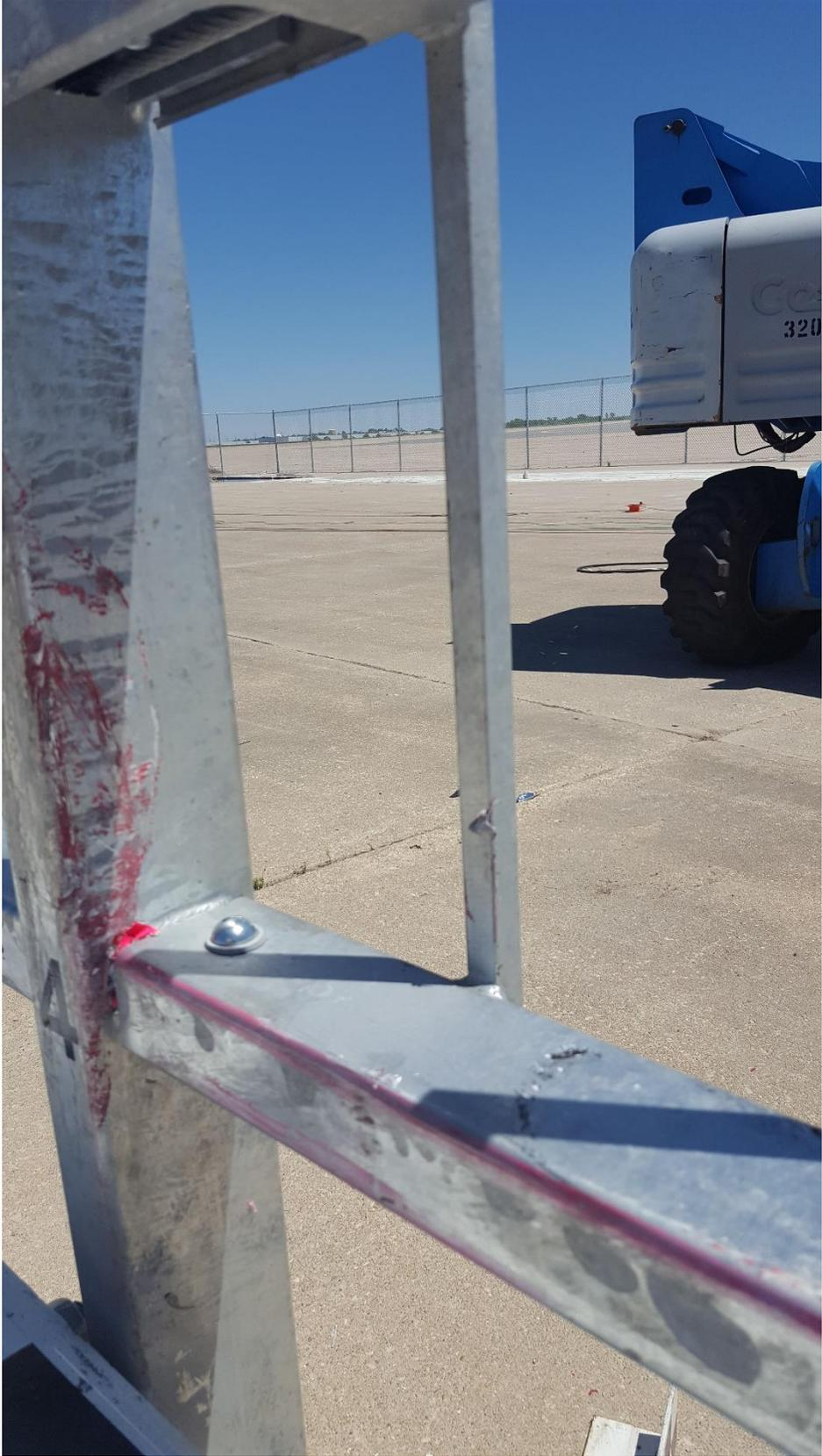
Figure 55. Spindle Contact and Debris, Test No. MNPD-3
