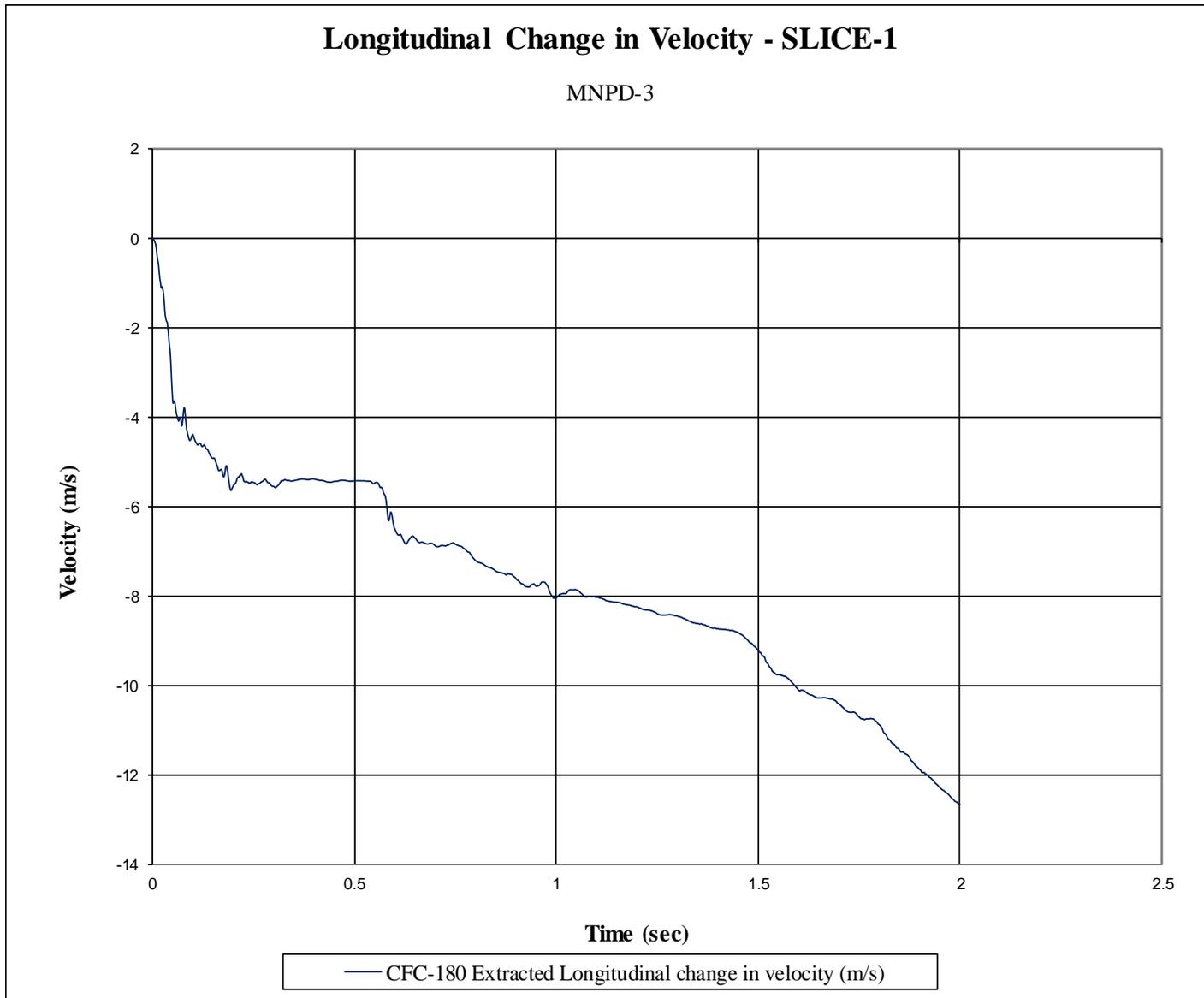
Figure D-10. Longitudinal Occupant Impact Velocity (SLICE-1), Test No. MNPD-3
