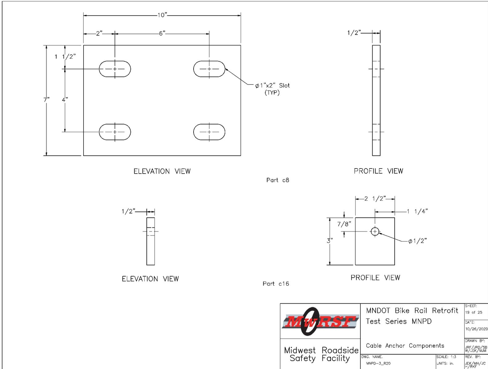
Figure 26. Cable Anchor Components, Test No. MNPD-3
