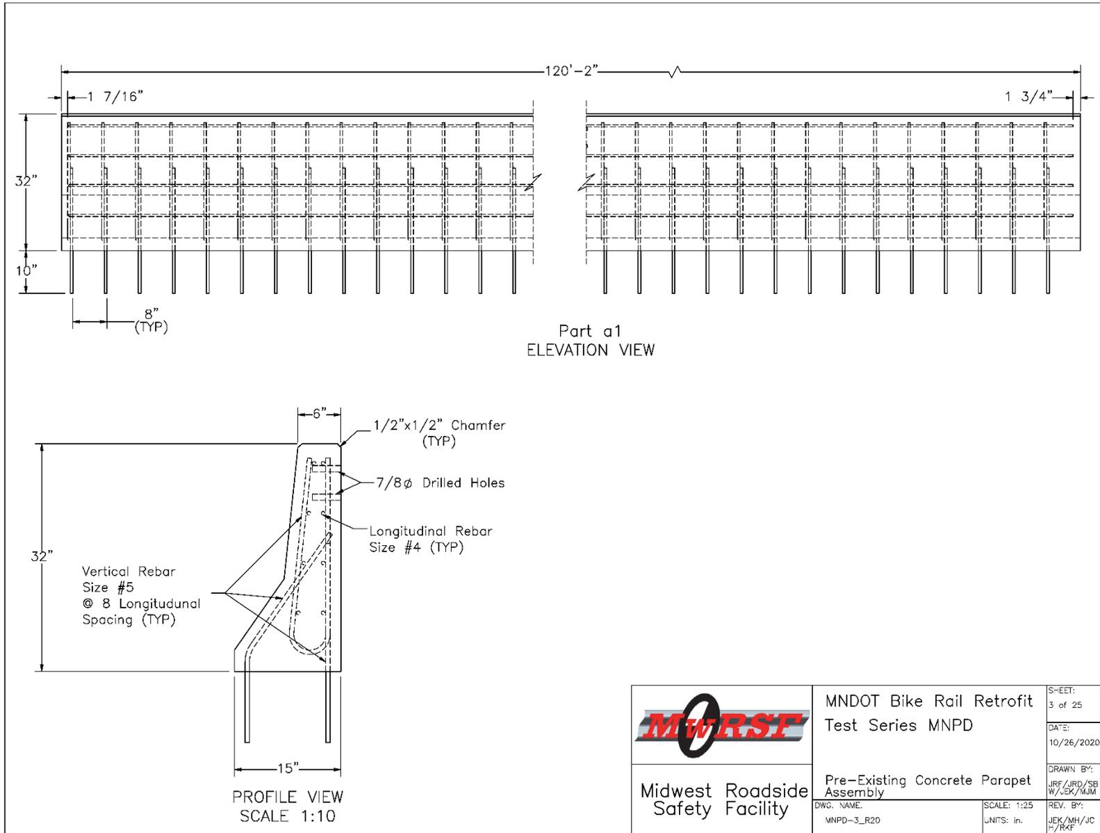
Figure 10. Pre-Existing Concrete Barrier Assembly, Test No. MNP3-3
