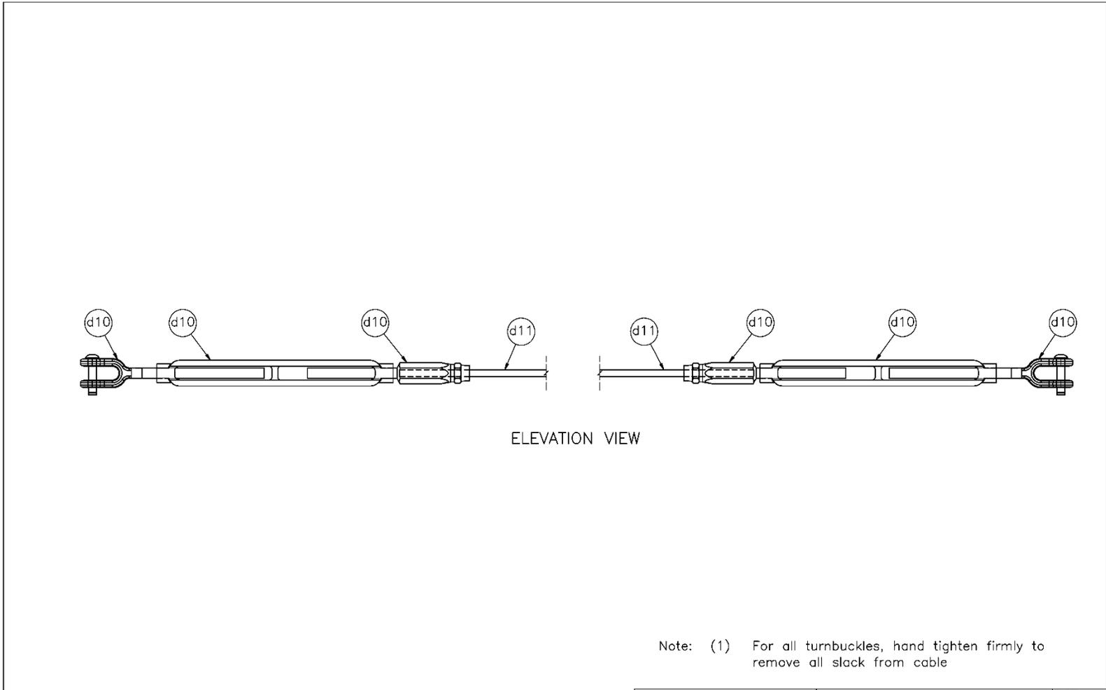
Note: (1) For all turnbuckles, hand tighten firmly to remove all slack from cable
