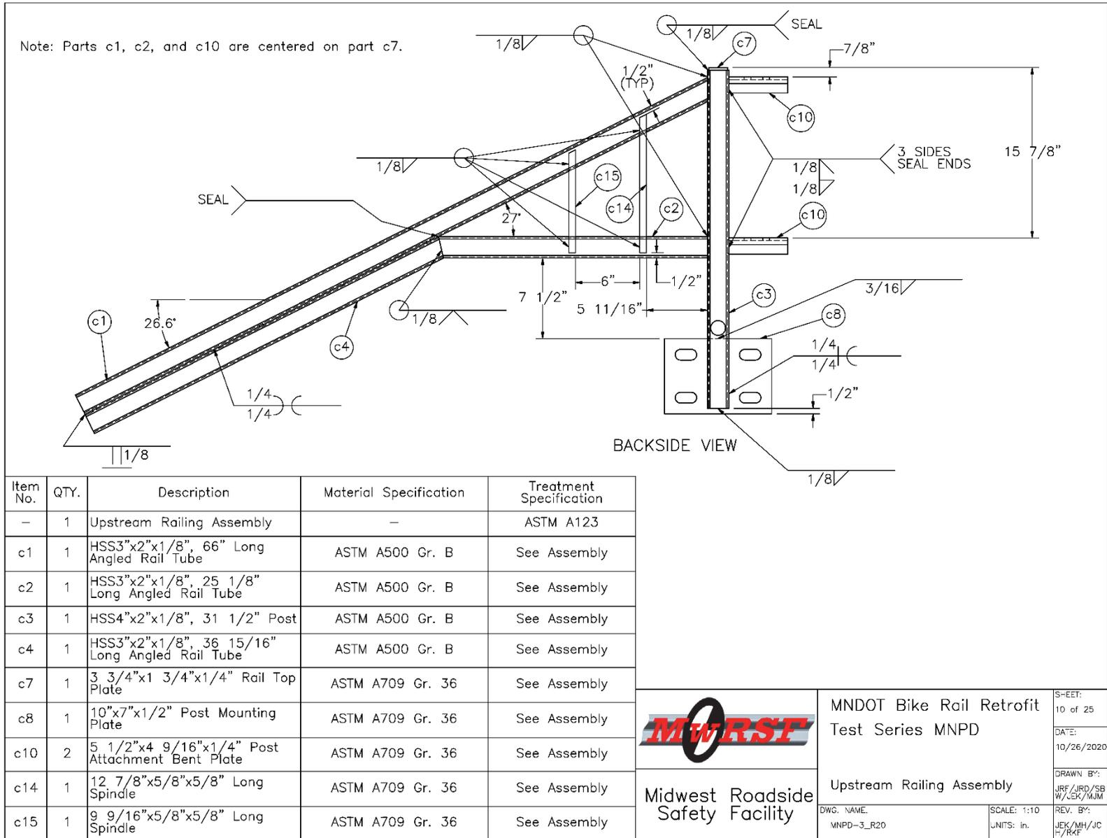
Figure 17. Upstream Railing Assembly, Test No. MNPD-3
