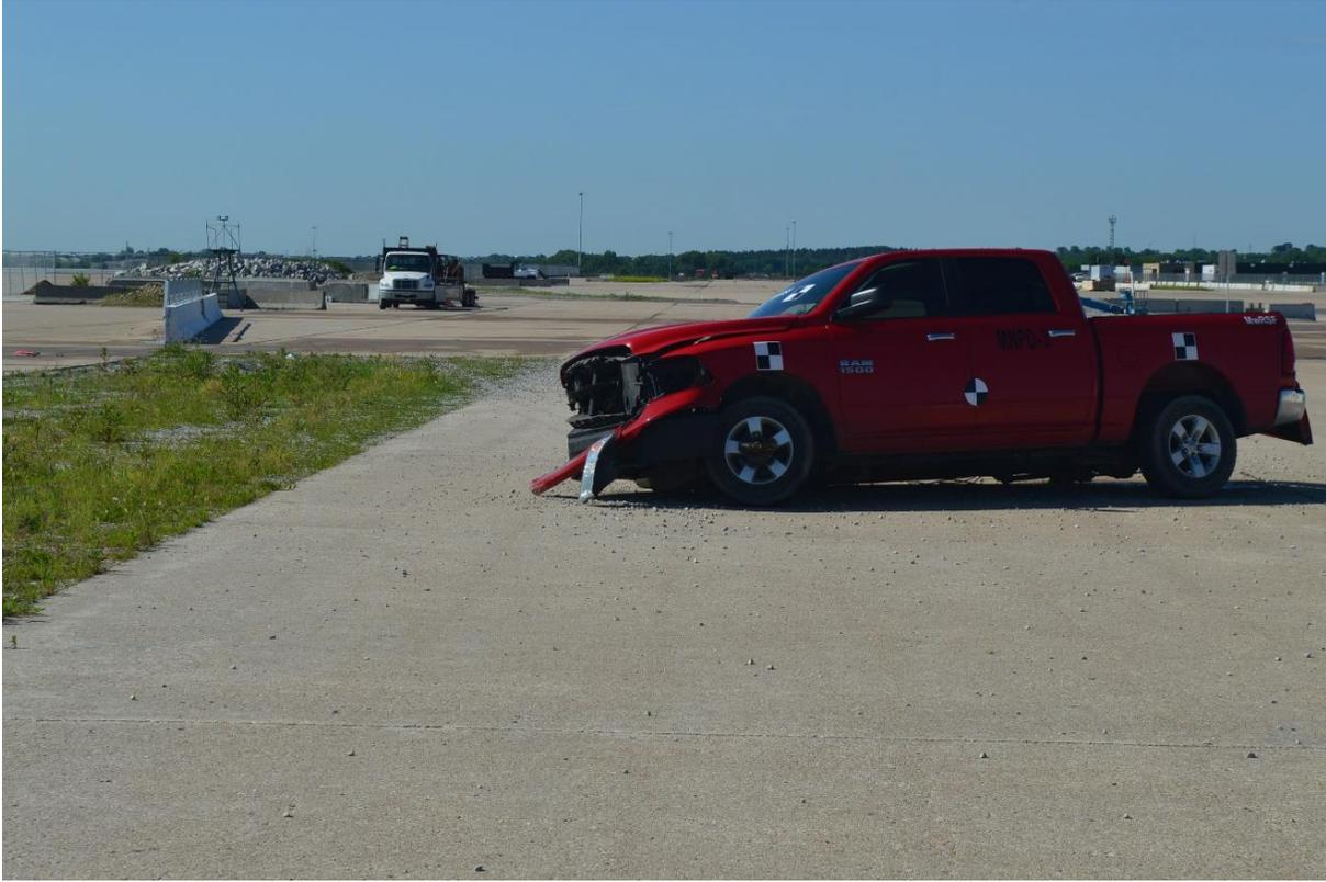
Figure 48. Vehicle Final Position and Trajectory Marks, Test No. MNPD-3.
