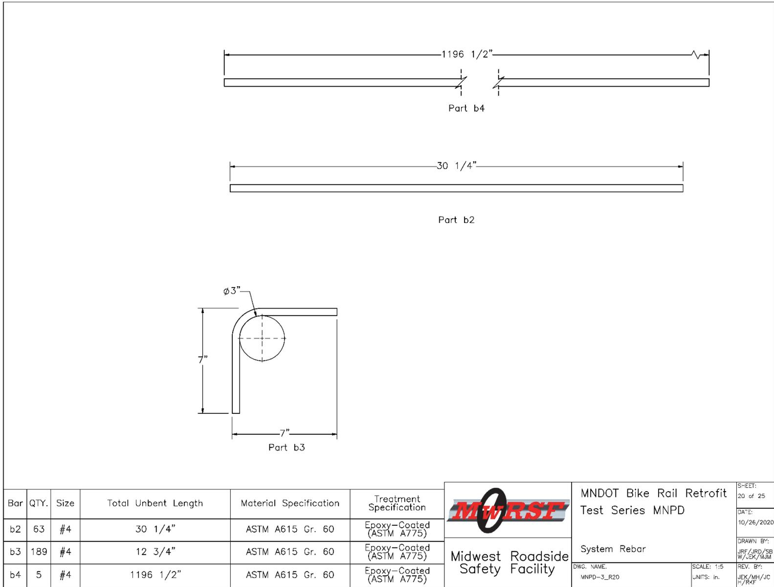
Figure 27. System Rebar, Test No. MNPD-3
