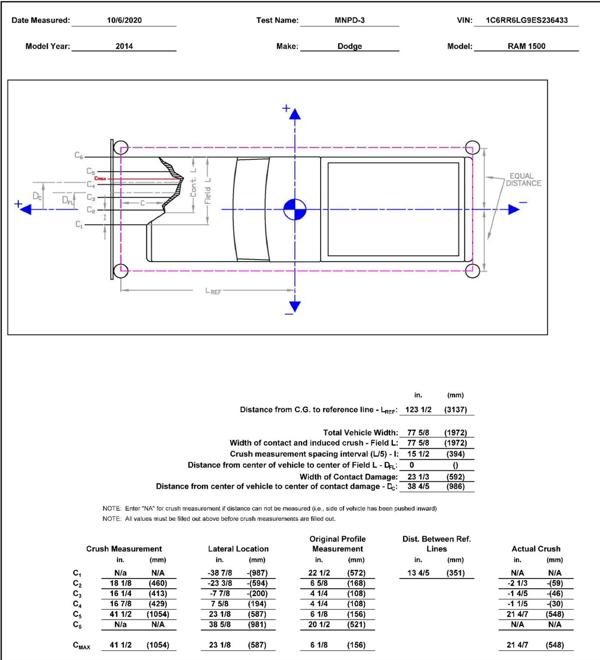
Figure C-5. Exterior Vehicle Crush (NASS) - Front, Test No. MNPD-3
