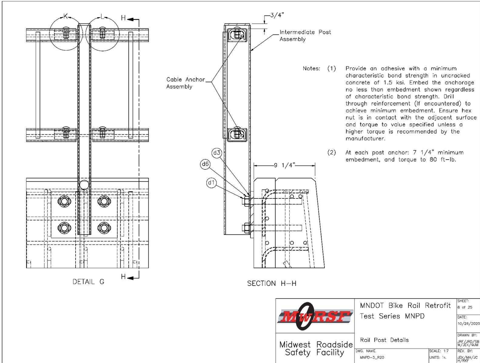
Figure 15. Rail Post Details, Test No. MNPD-3
