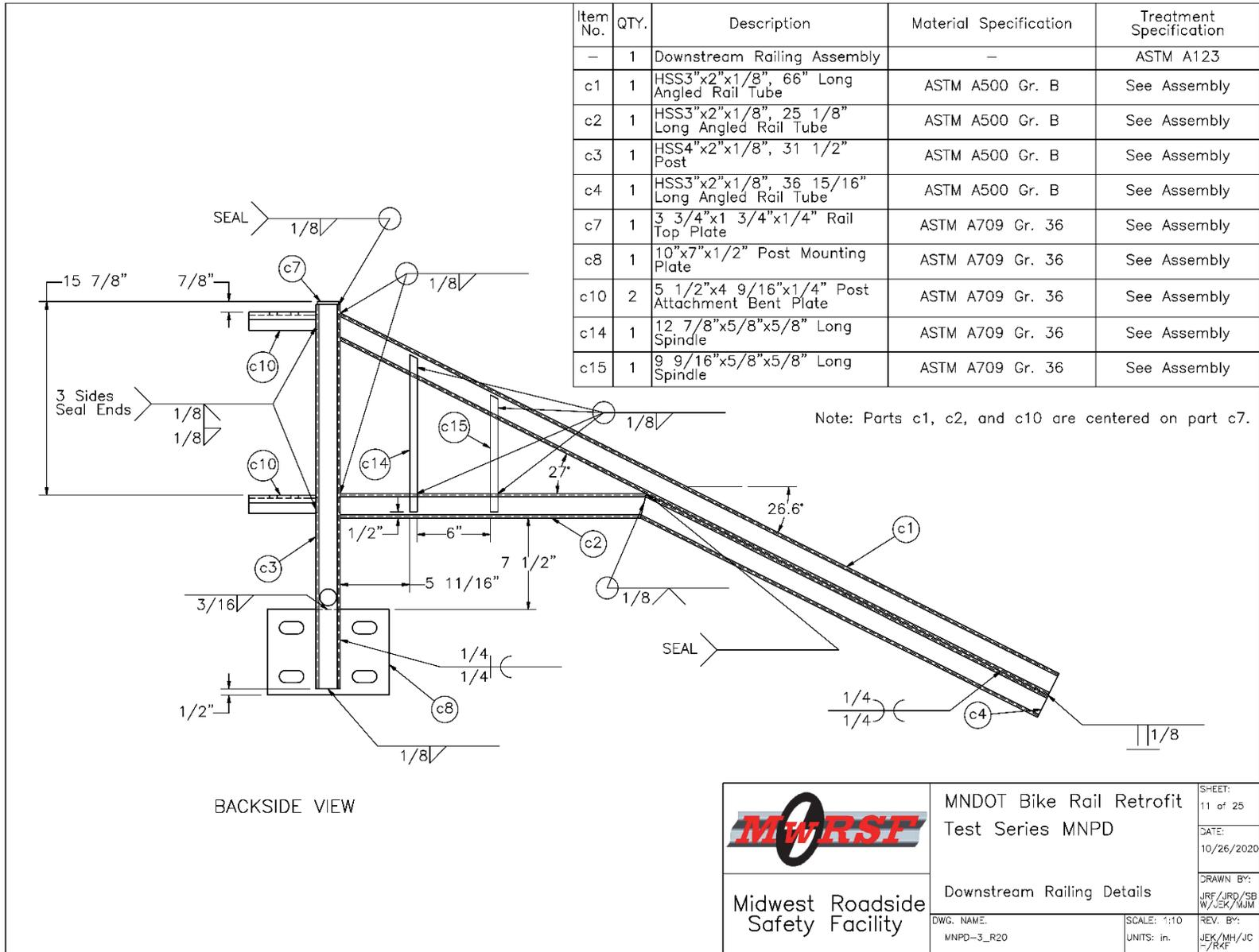
Figure 18. Downstream Railing Details, Test No. MNPD-3
