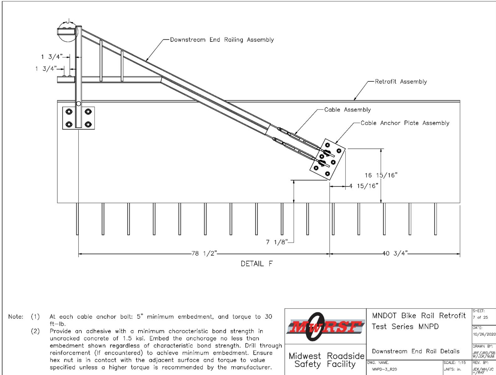
Figure 14. Downstream End Rail Details, Test No. MNPD-3
