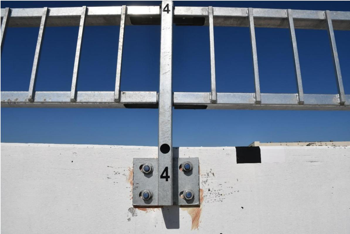
Figure 6. 2020 MnDOT Bicycle and Pedestrian Rail Spindle with Back of Tube Positioning, Test No. MNPD-3
