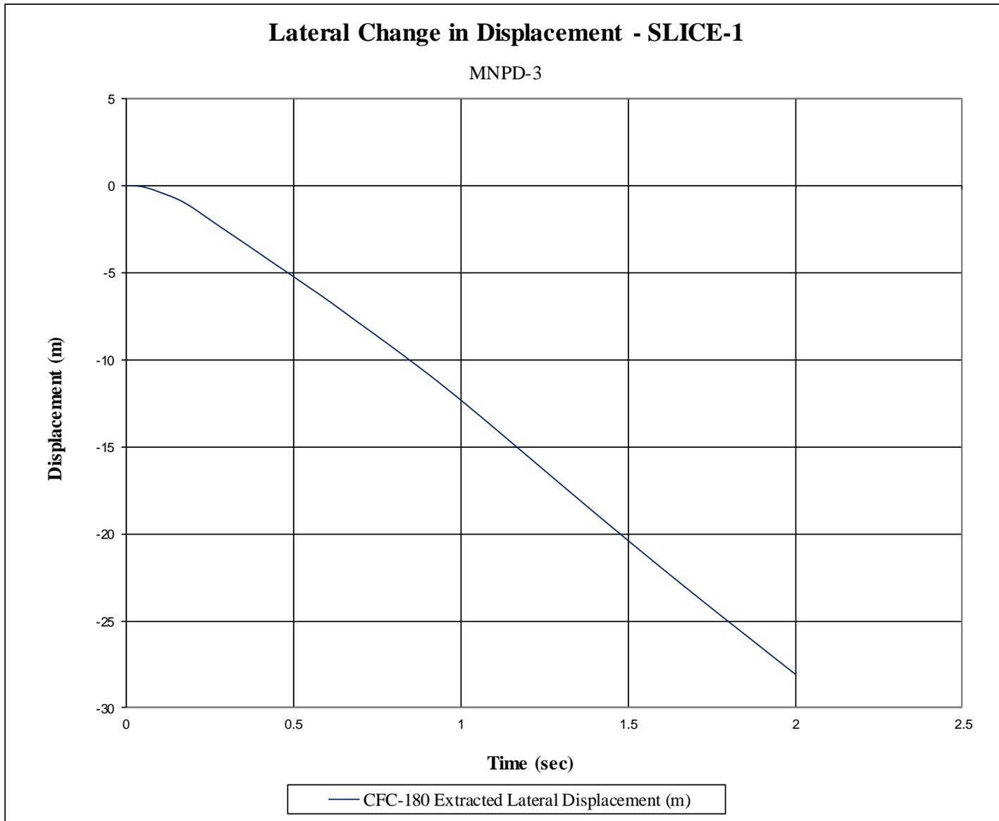
Figure D-14. Lateral Occupant Displacement (SLICE-1), Test No. MNP-3
