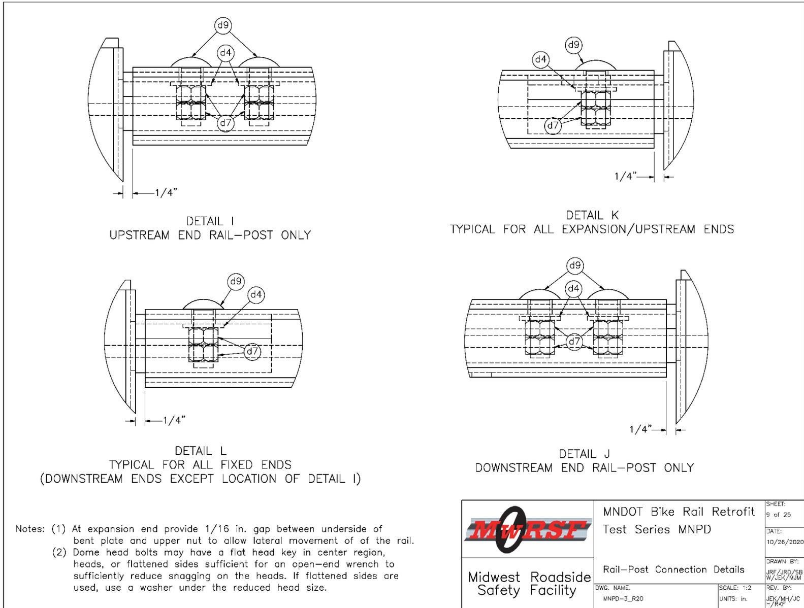
Figure 16. Rail-Post Connection Details, Test No. MNPD-3
