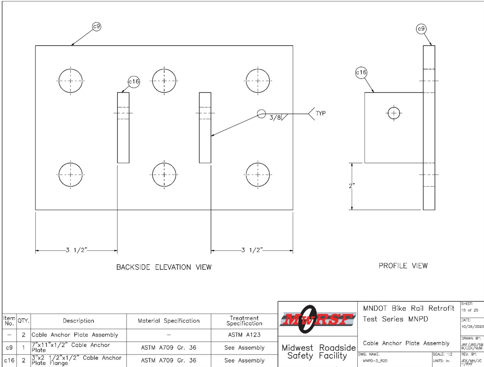
Figure 22. Cable Anchor Plate Assembly, Test No. MNPD-3
