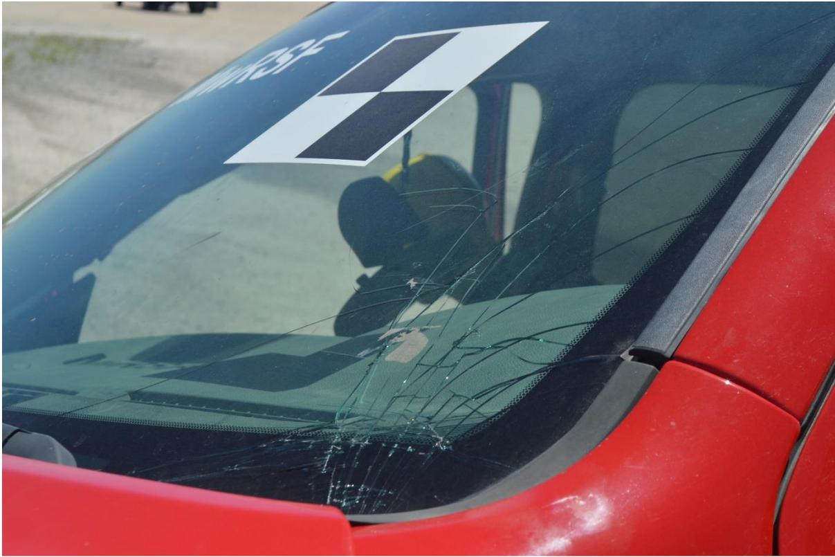
Figure 67. Windshield Damage (Post-Test), Test No. MNPD-3
