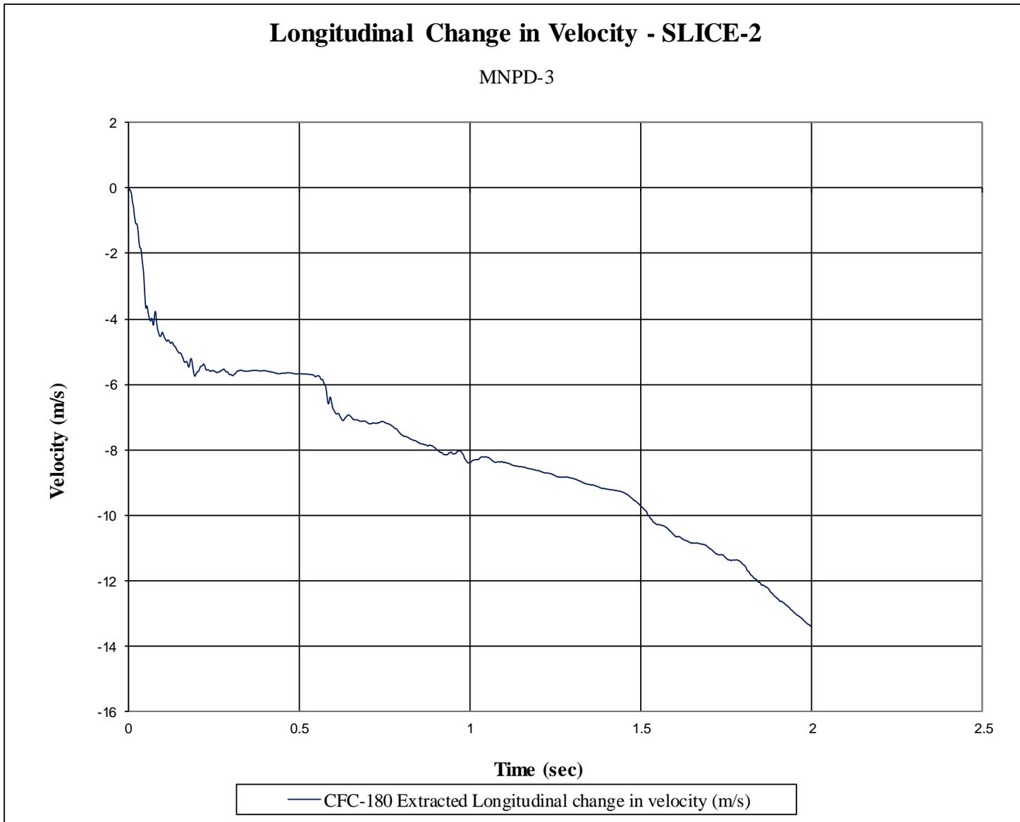
Figure D-2. Longitudinal Occupant Impact Velocity (SLICE-2), Test No. MNPD-3
