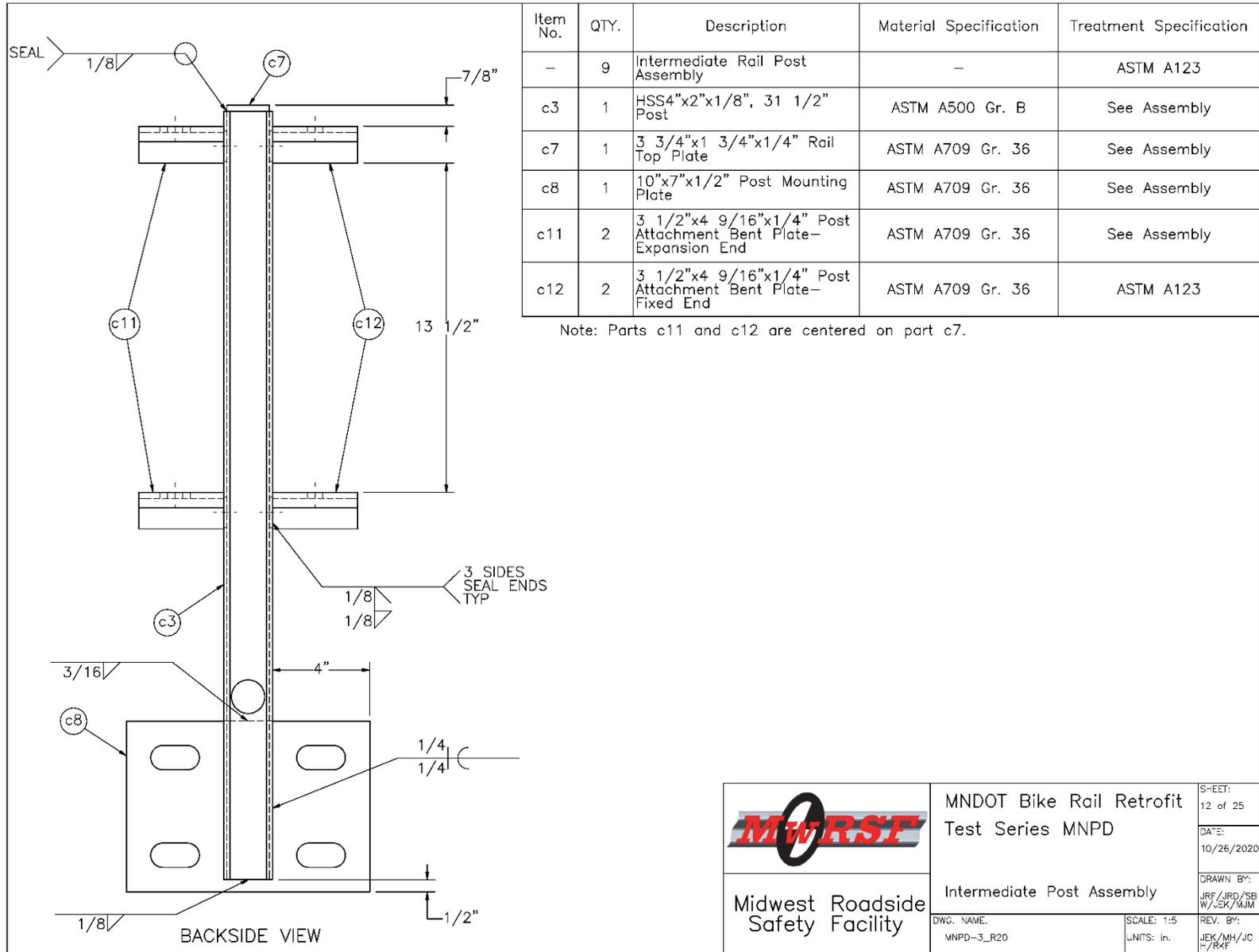
Figure 19. Intermediate Post Assembly, Test No. MNPD-3
