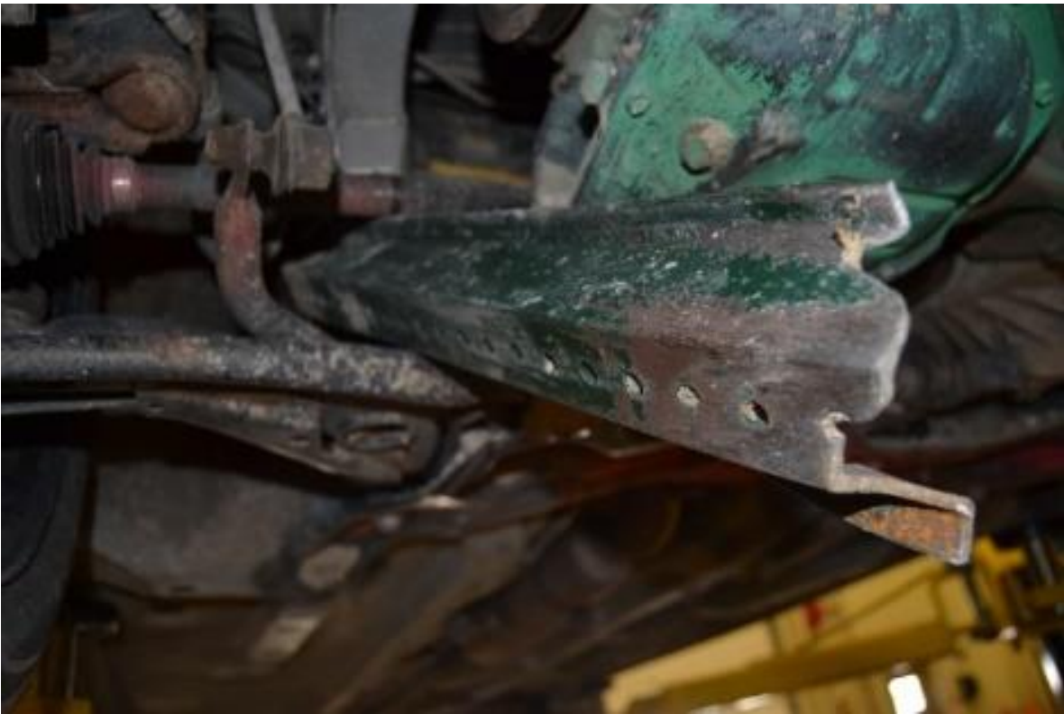
Figure 41. Right-Side Lower A-Arm Damage, Test No.UCSS-1
